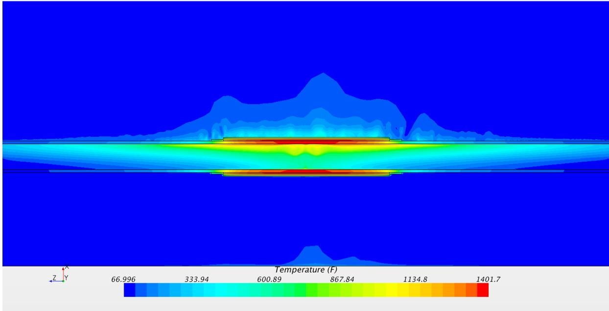
**Figure B-90: Temperature contours, cross section of all regions, close-up (°F). 24 inch schedule 160**
