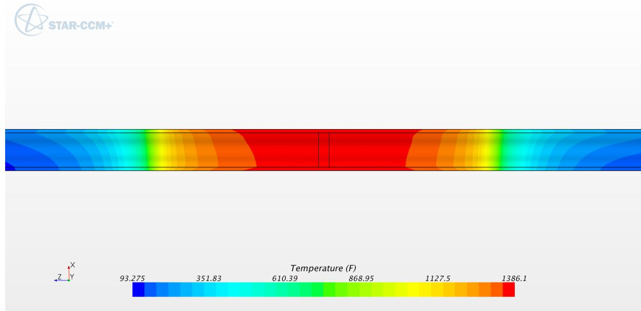
**Figure B-116: Temperature contours in pipe wall, close-up (°F). 30 inch schedule 160**
