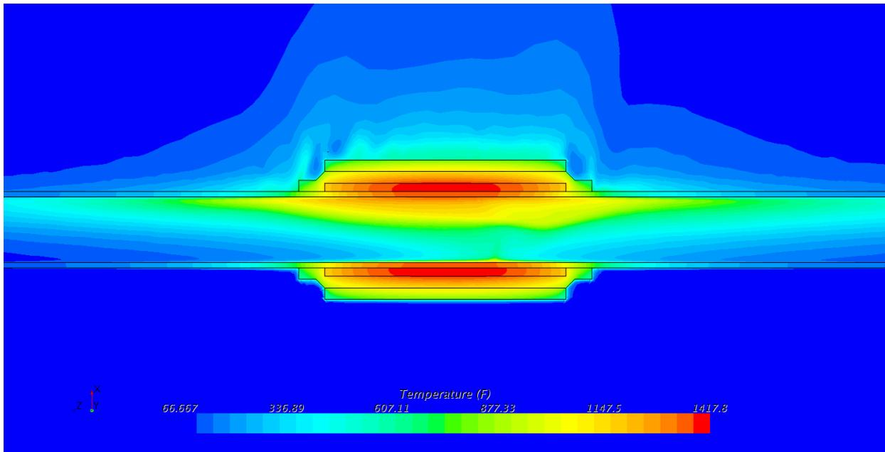
**Figure B-3: Temperature contours in pipe wall (°F). 6 inch schedule 80**
