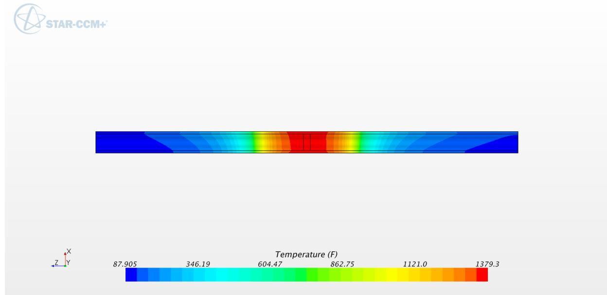
**Figure B-44: Temperature contours in pipe wall, close-up (°F). 10 inch schedule 160**
