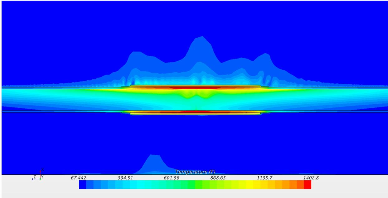
**Figure B-106: Temperature contours, cross section of all regions, close-up (°F). 30 inch schedule 120**
