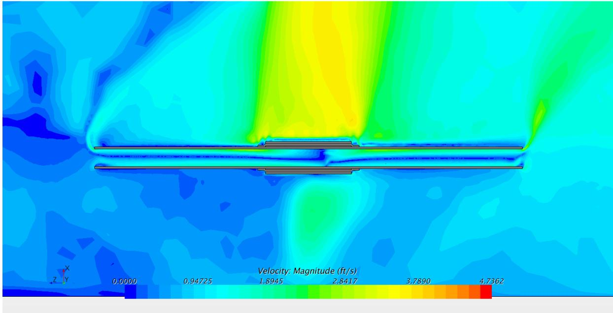
**Figure B-40: Velocity contours, cross section of all regions, isometric view (ft/s). 10 inch schedule 120**
