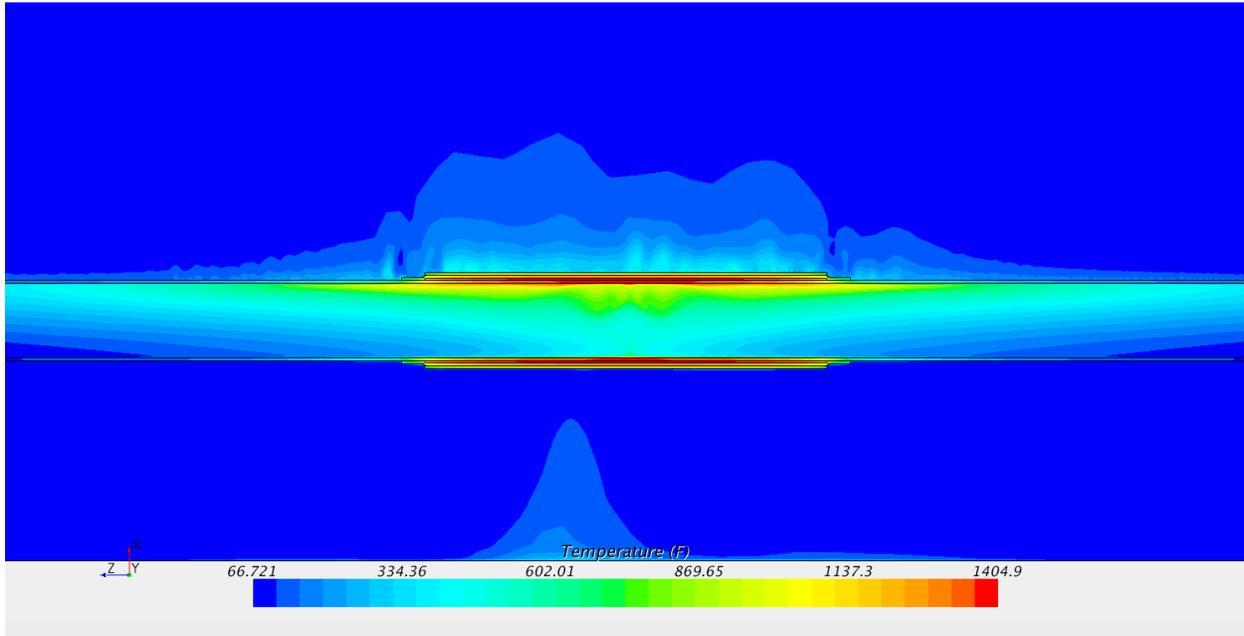
**Figure B-98: Temperature contours, cross section of all regions, close-up (°F). 30 inch schedule 80**
