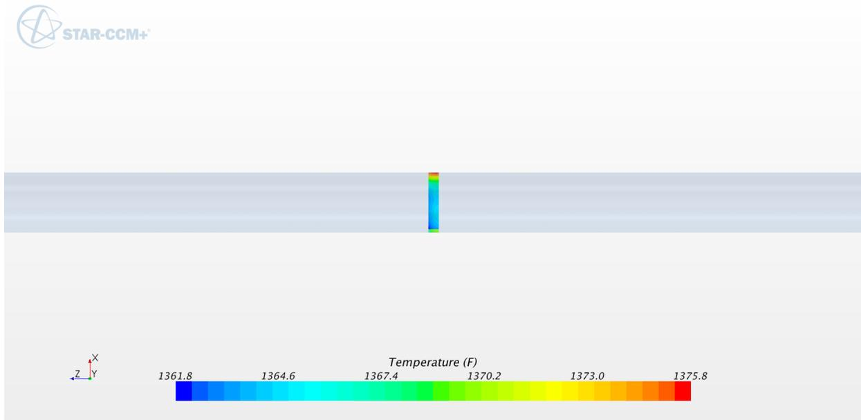
**Figure B-30: Temperature contours in SB, isometric view (°F). 10 inch schedule 80**
