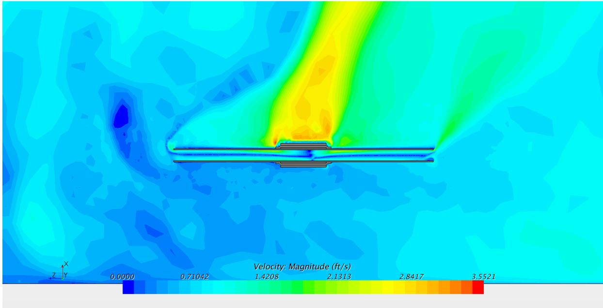
**Figure B-16: Velocity contours, cross section of all regions, isometric view (ft/s). 6 inch schedule 120**
