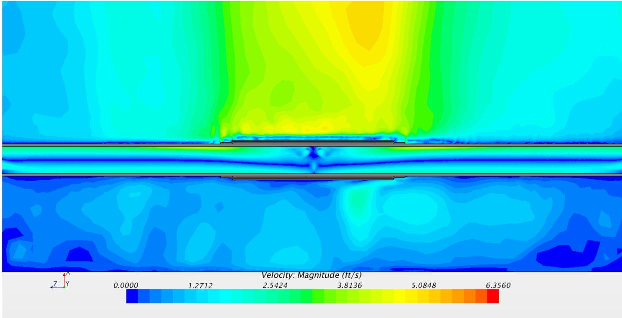
**Figure B-88: Velocity contours, cross section of all regions, isometric view (ft/s). 24 inch schedule 120**
