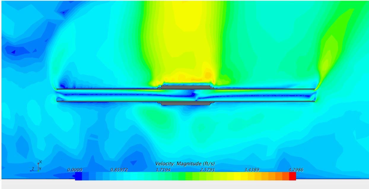
**Figure B-32: Velocity contours, cross section of all regions, isometric view (ft/s). 10 inch schedule 80**
