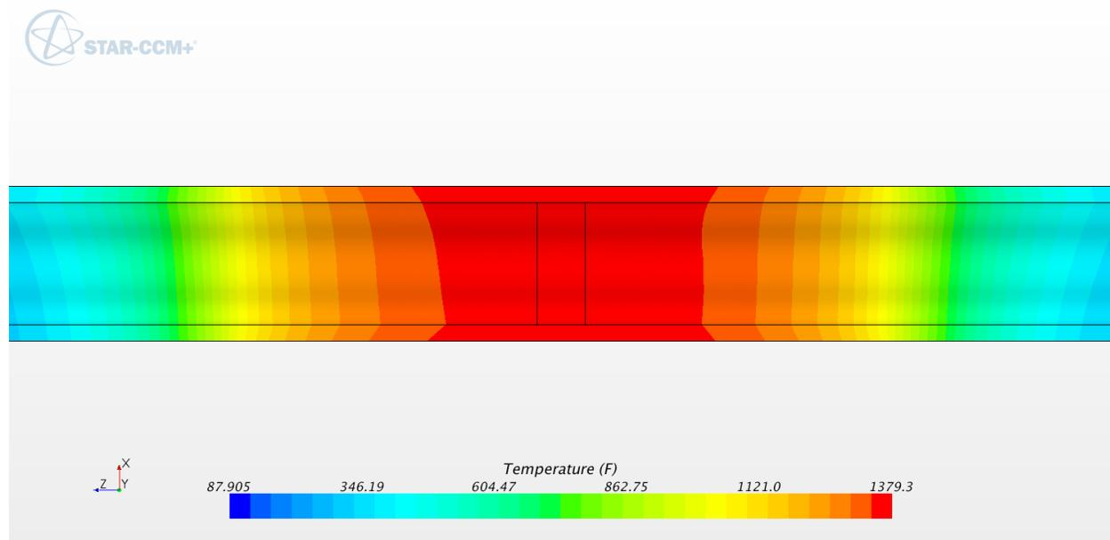
**Figure B-45: Temperature contours in SB (°F). 10 inch schedule 160**
