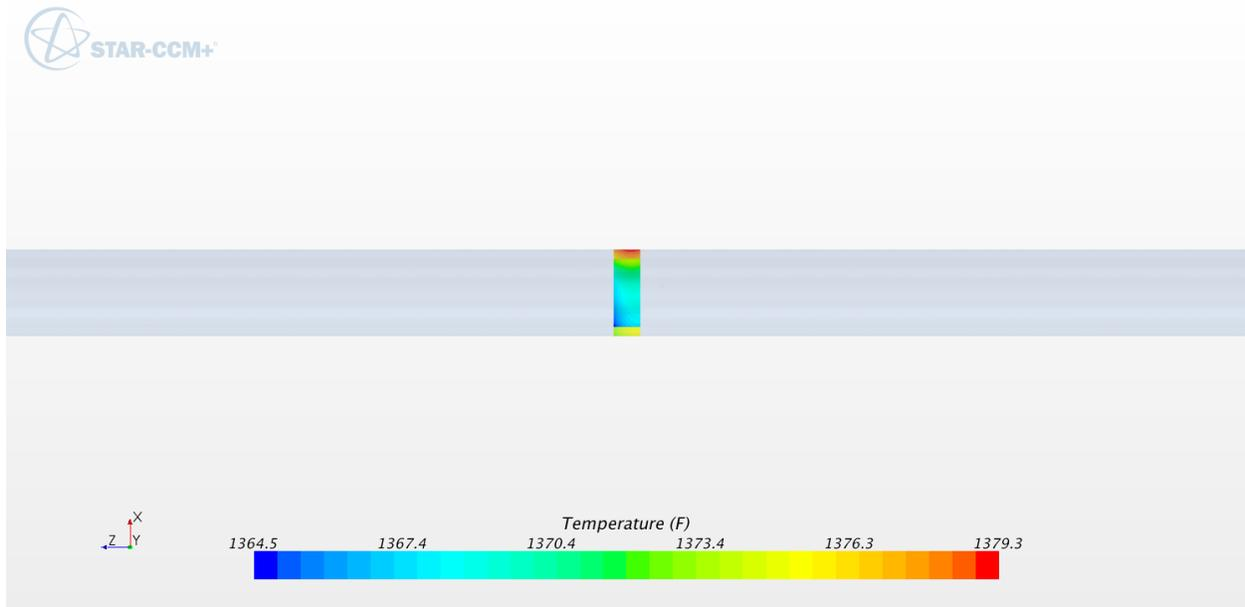
**Figure B-46: Temperature contours in SB, isometric view (°F). 10 inch schedule 160**
