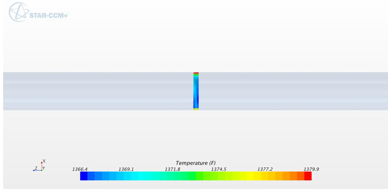
**Figure B-102: Temperature contours in SB, isometric view (°F). 30 inch schedule 80**
