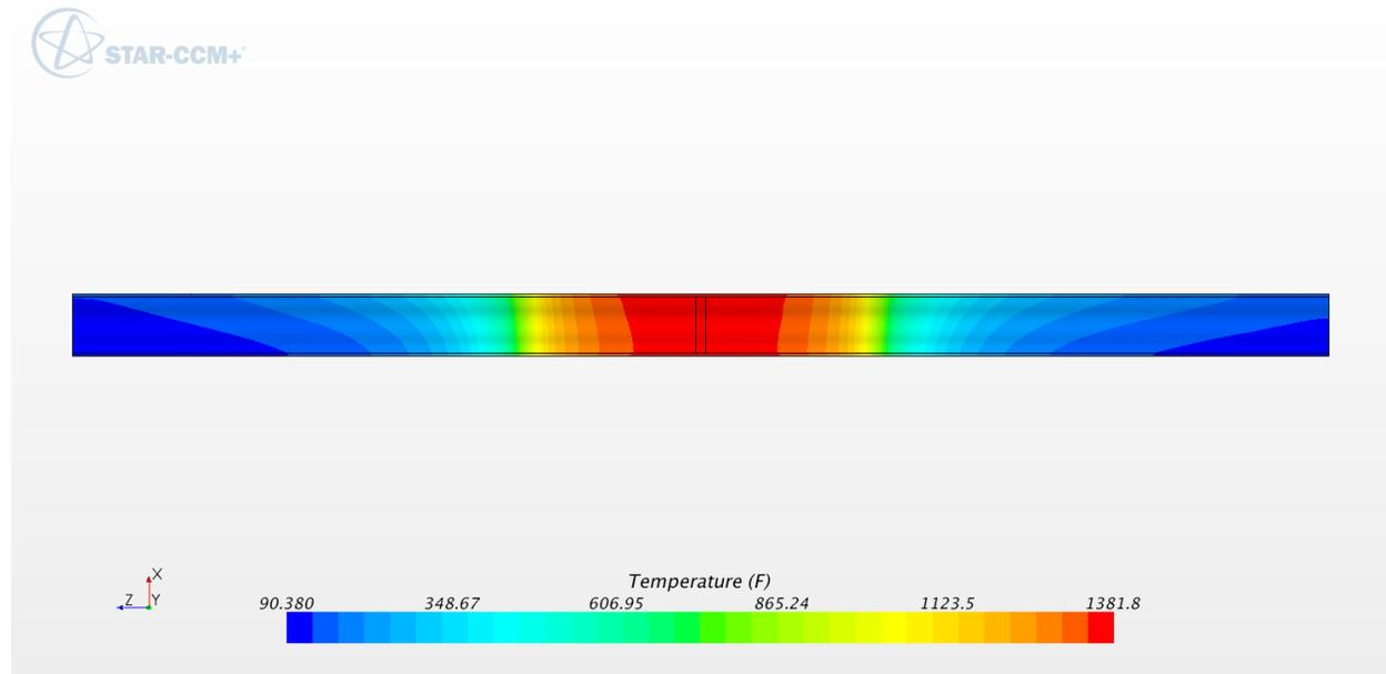
**Figure B-52: Temperature contours in pipe wall, close-up (°F). 14 inch schedule 80**
