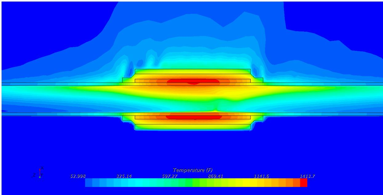
**Figure B-11: Temperature contours in pipe wall (°F). 6 inch schedule 120**
