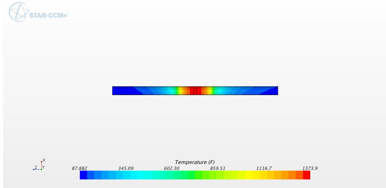
**Figure B-12: Temperature contours in pipe wall, close-up (°F). 6 inch schedule 120**
