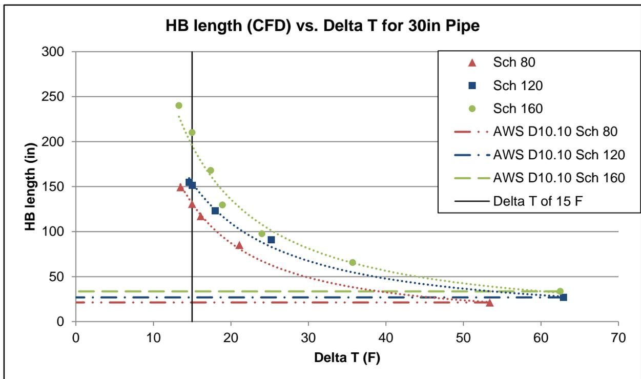
If a larger temperature gradient than 15°F is deemed acceptable, the required HB length can be interpolated using the power fit curves. The coefficients for those curves are in Figure 3-7 and take the form of Equation 1.
