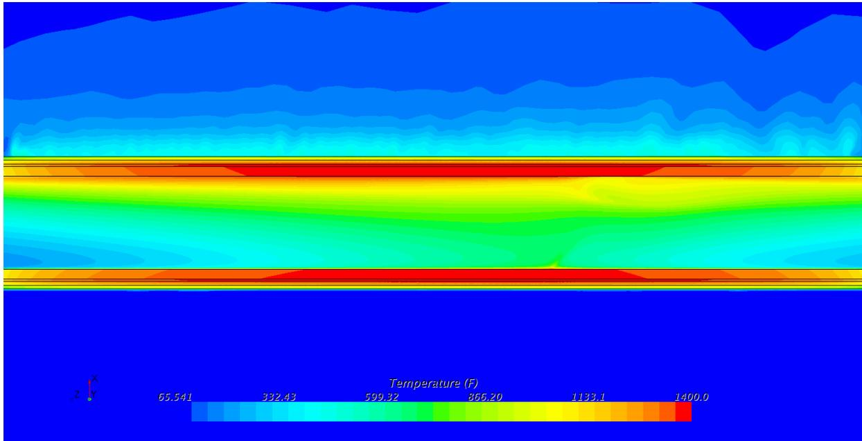
**Figure B-115: Temperature contours in pipe wall (°F). 30 inch schedule 160**
