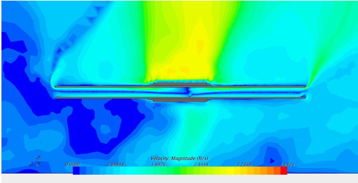
**Figure B-48: Velocity contours, cross section of all regions, isometric view (ft/s). 10 inch schedule 160**
