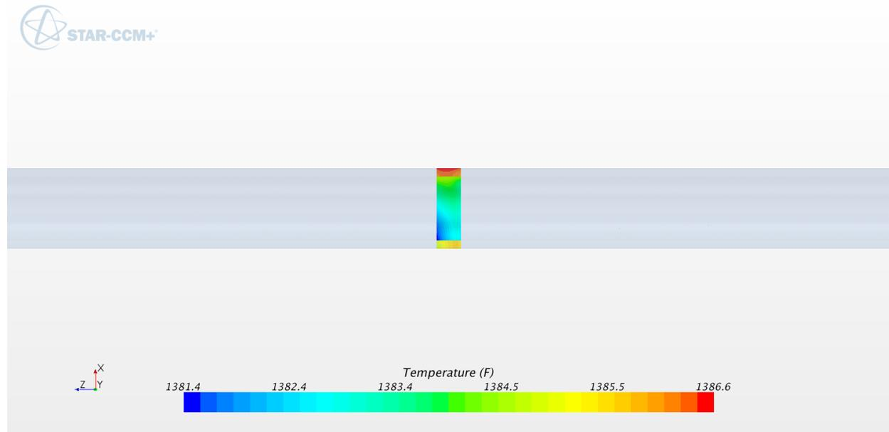
**Figure B-70: Temperature contours in SB, isometric view (°F). 14 inch schedule 160**
