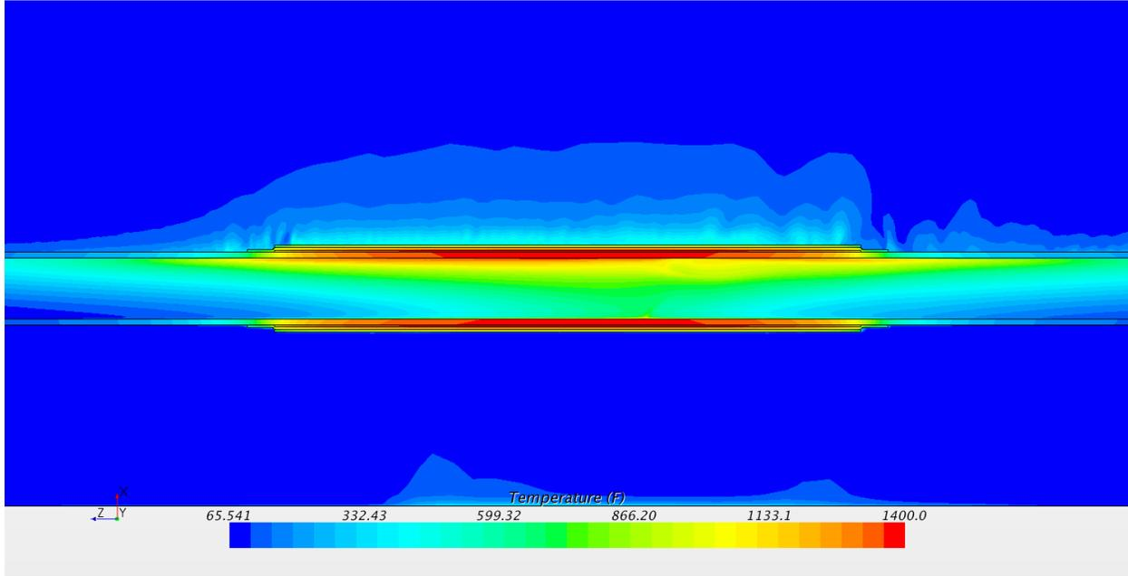
**Figure B-114: Temperature contours, cross section of all regions, close-up (°F). 30 inch schedule 160**
