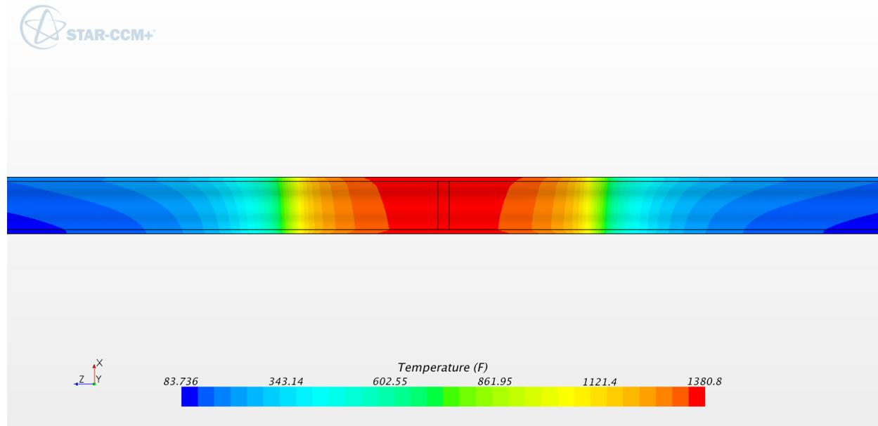
**Figure B-108: Temperature contours in pipe wall, close-up (°F). 30 inch schedule 120**
