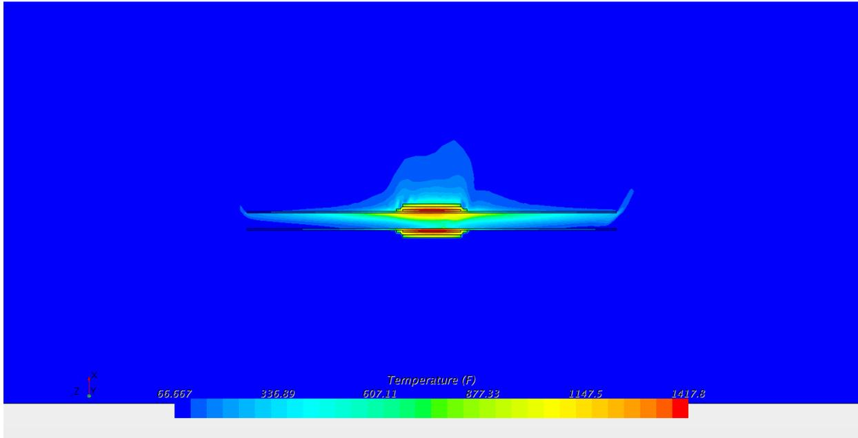
**Figure B-2: Temperature contours, cross section of all regions, close-up (°F). 6 inch schedule 80**
