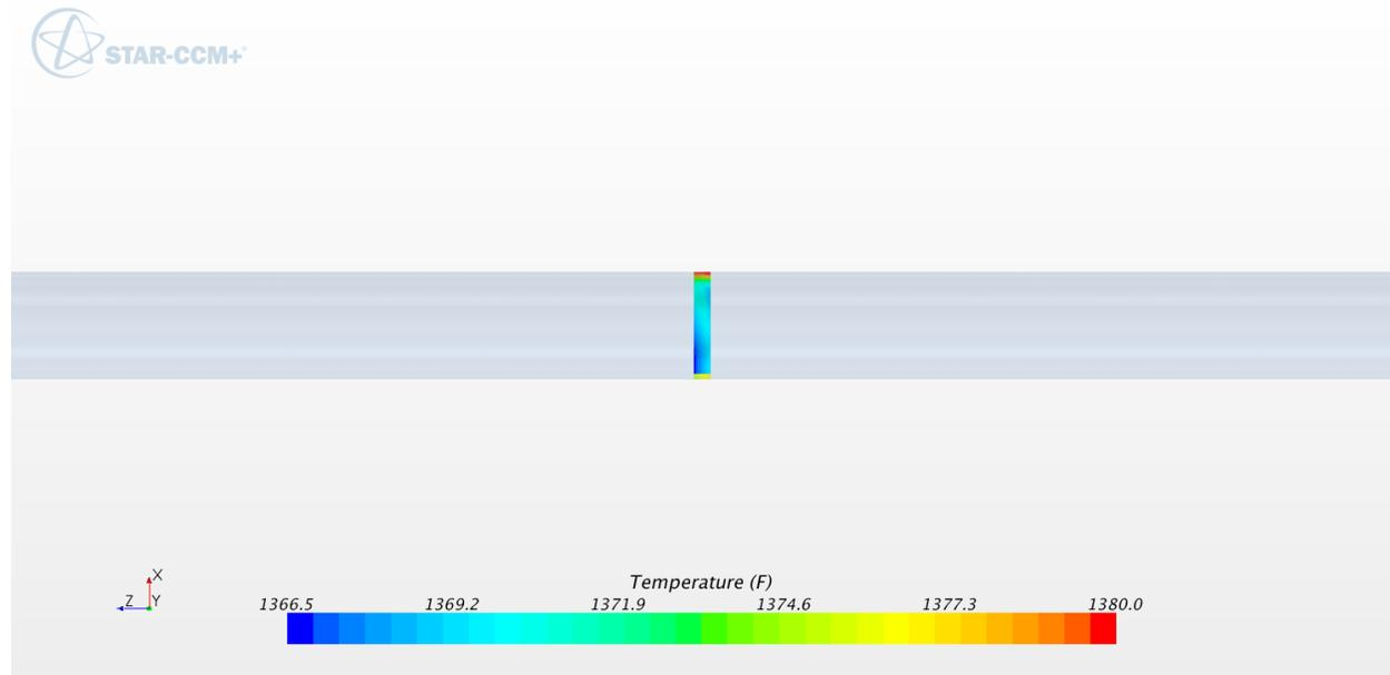
**Figure B-78: Temperature contours in SB, isometric view (°F). 24 inch schedule 80**
