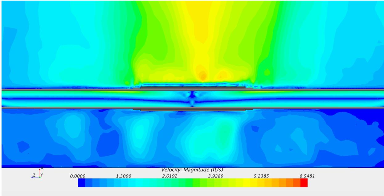
**Figure B-96: Velocity contours, cross section of all regions, isometric view (ft/s). 24 inch schedule 160**
