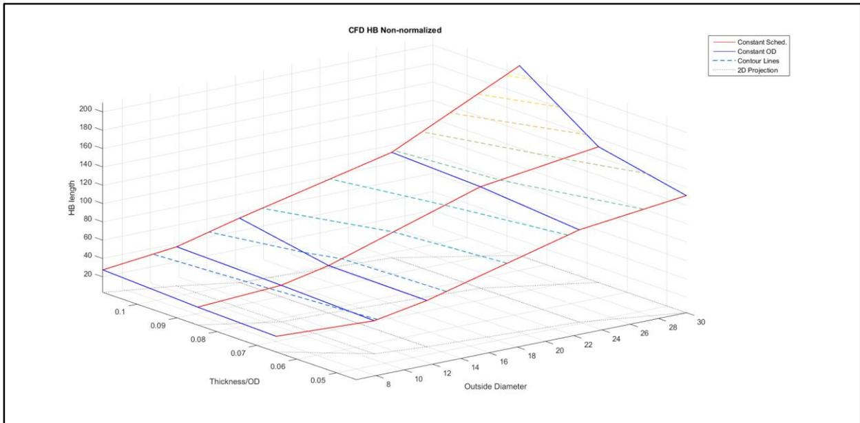
**Figure 3-10: CFD HB results for SB temperature difference of 15°F plotted against OD and t/OD. Viewed from in-plane direction**
