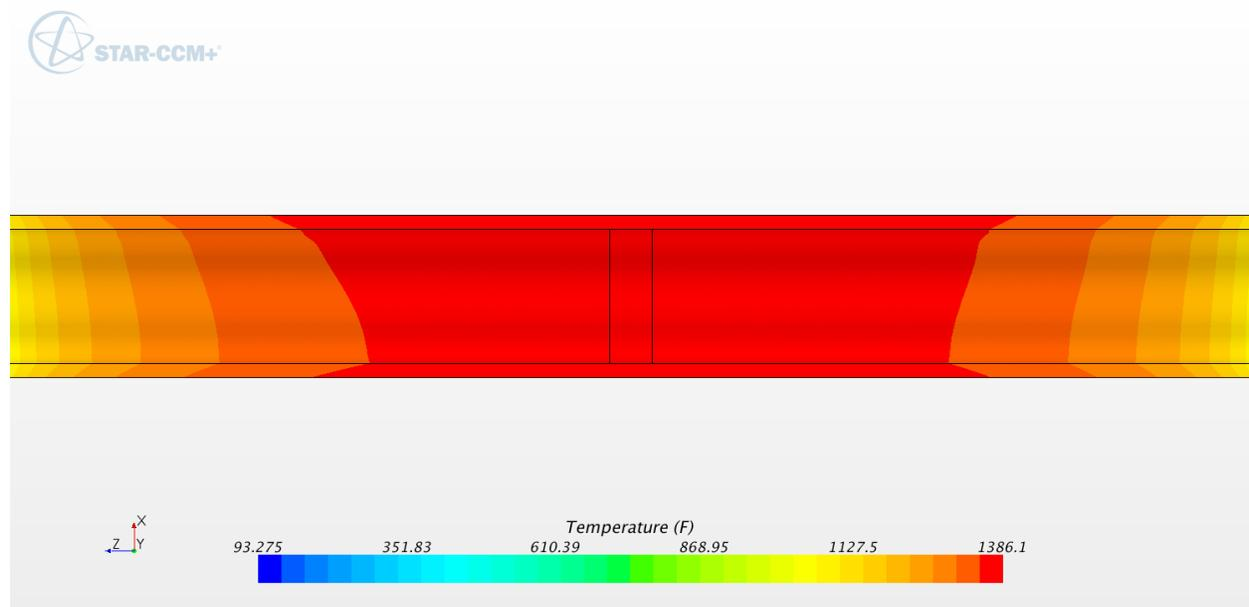
**Figure B-117: Temperature contours in SB (°F). 30 inch schedule 160**
