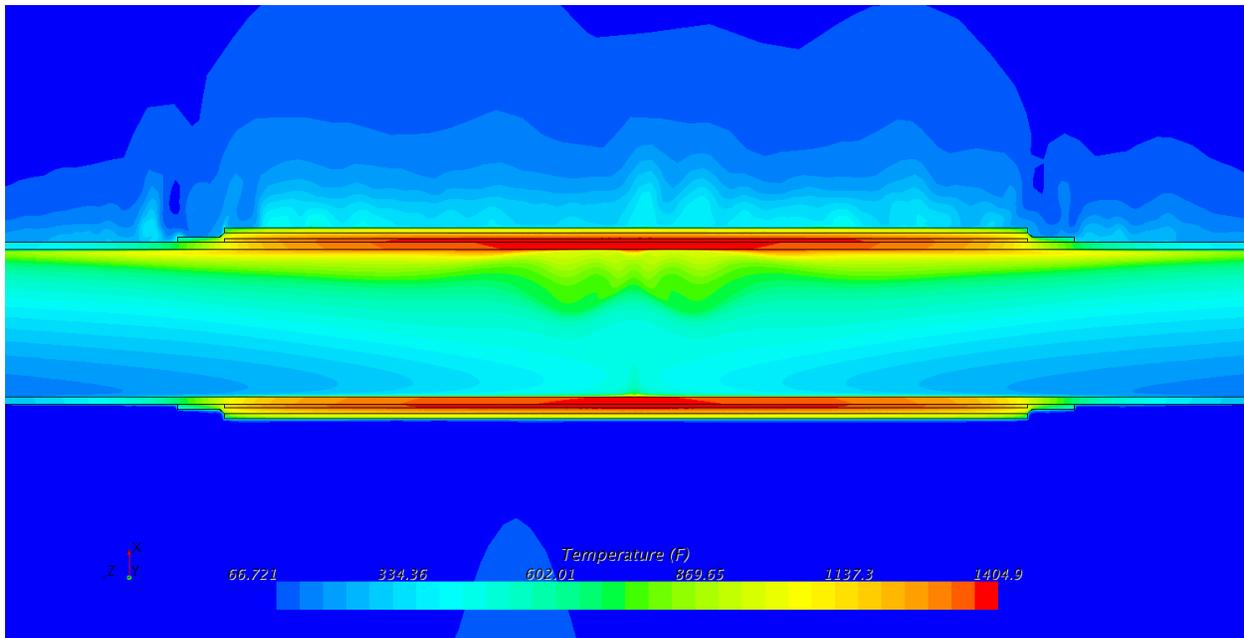
**Figure B-99: Temperature contours in pipe wall (°F). 30 inch schedule 80**
