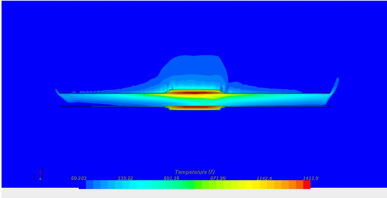
**Figure B-26: Temperature contours, cross section of all regions, close-up (°F). 10 inch schedule 80**
