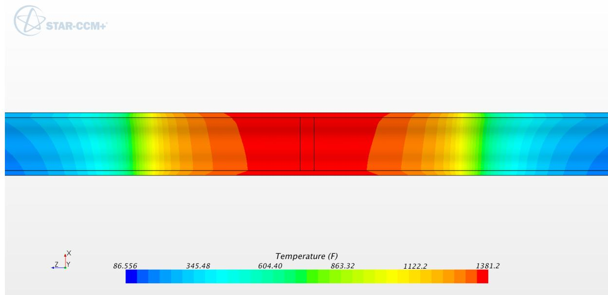
**Figure B-85: Temperature contours in SB (°F). 24 inch schedule 120**
