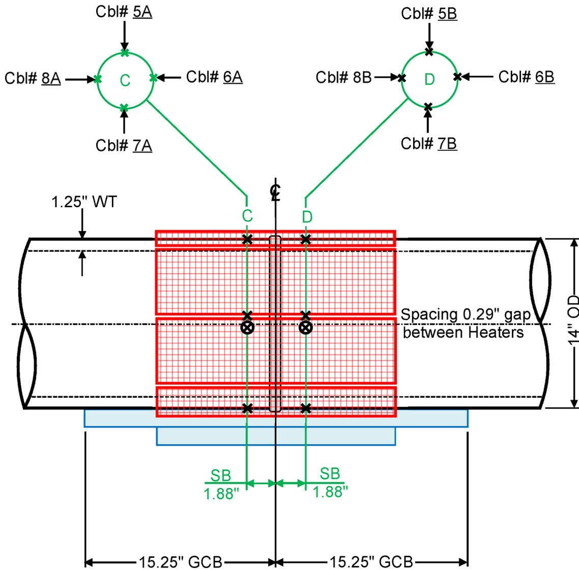
1" 6# density Insulation Double Layer over Heaters
