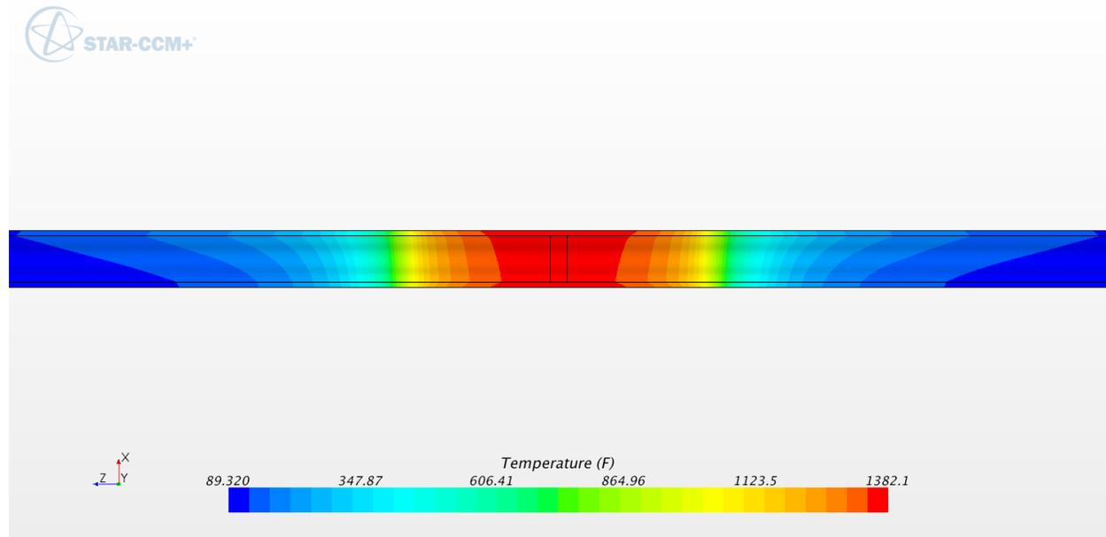
**Figure B-92: Temperature contours in pipe wall, close-up (°F). 24 inch schedule 160**
