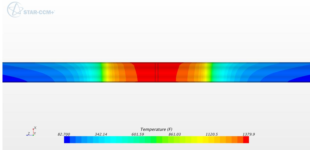
**Figure B-100: Temperature contours in pipe wall, close-up (°F). 30 inch schedule 80**
