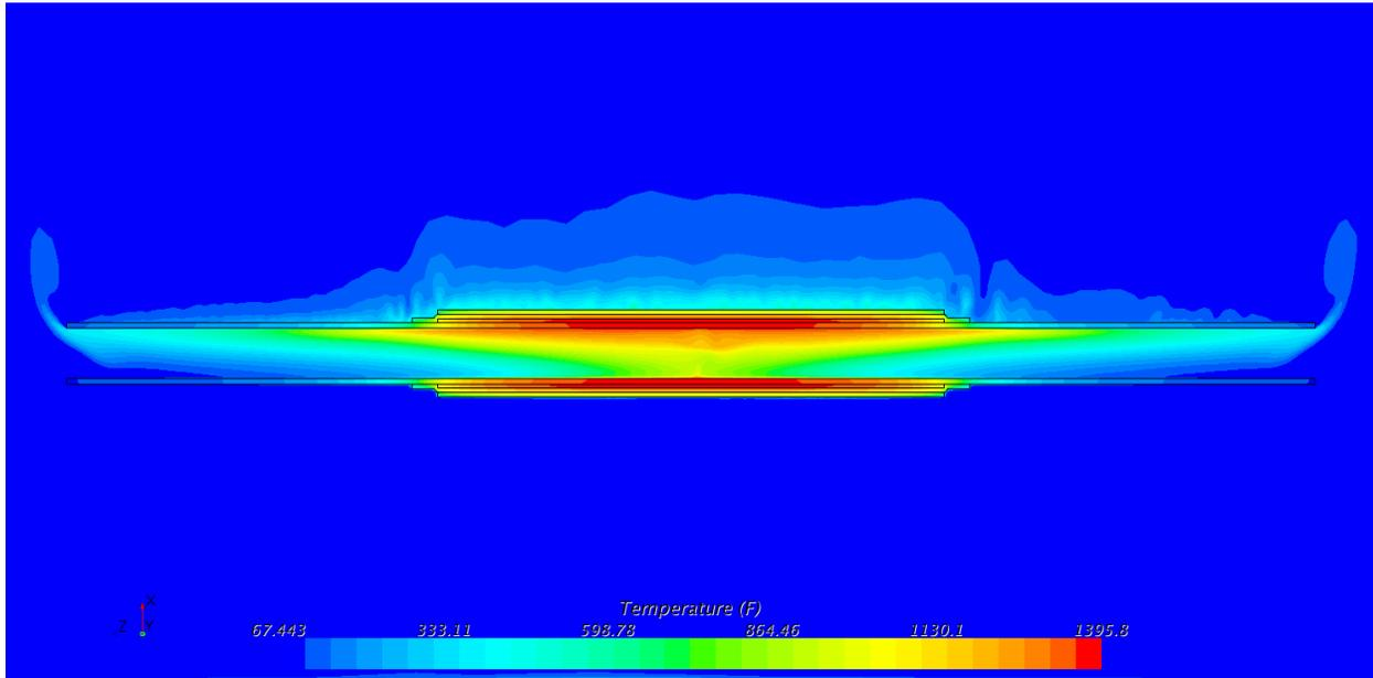
**Figure B-66: Temperature contours, cross section of all regions, close-up (°F). 14 inch schedule 160**
