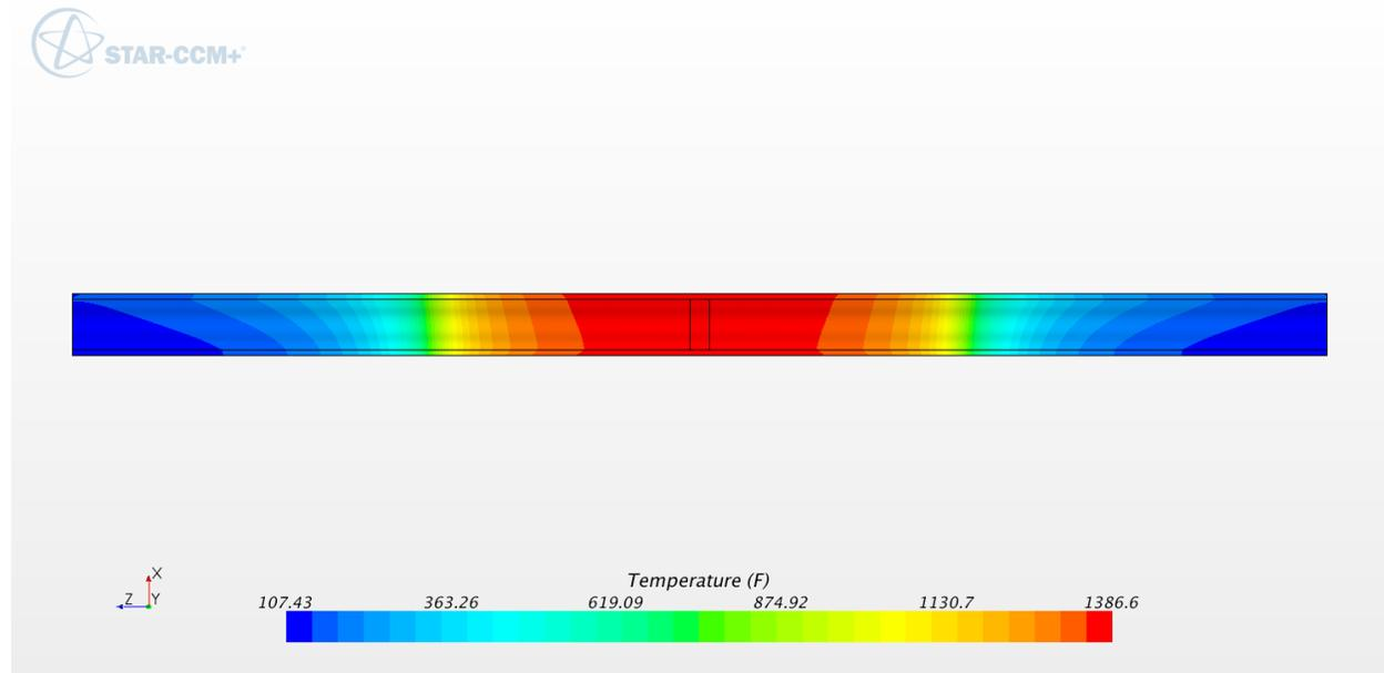
**Figure B-68: Temperature contours in pipe wall, close-up (°F). 14 inch schedule 160**
