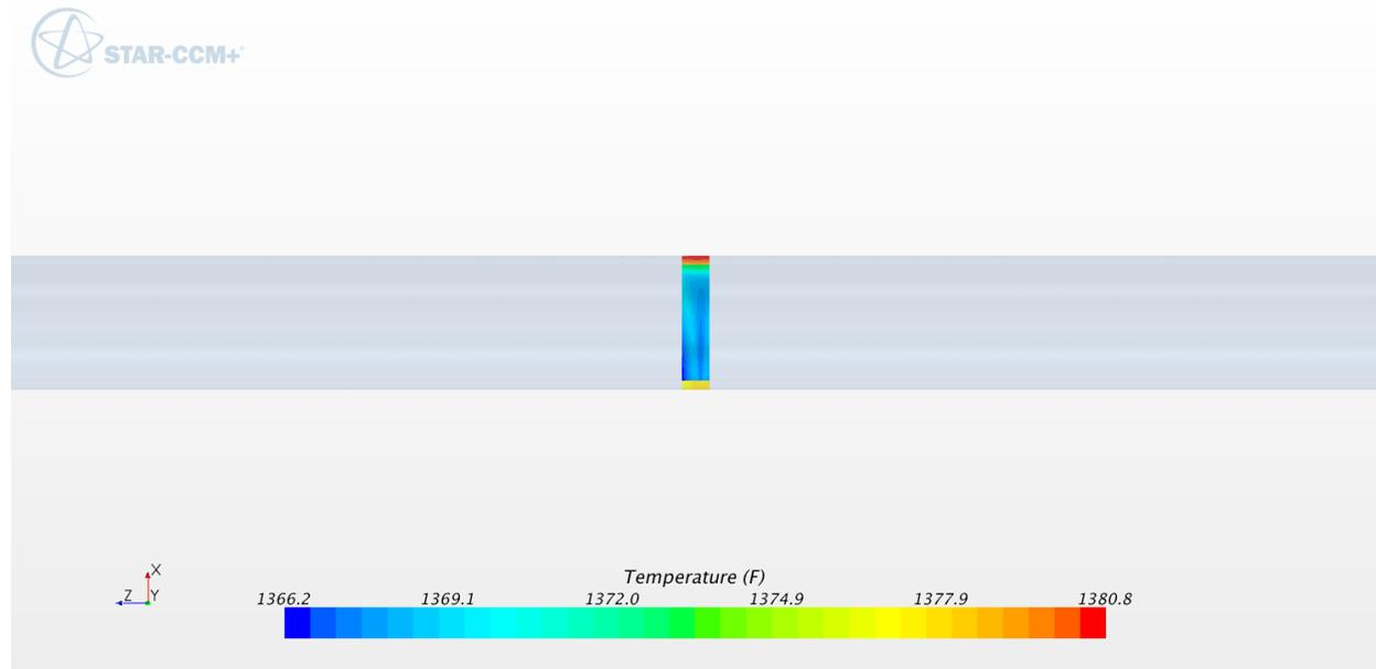
**Figure B-110: Temperature contours in SB, isometric view (°F). 30 inch schedule 120**
