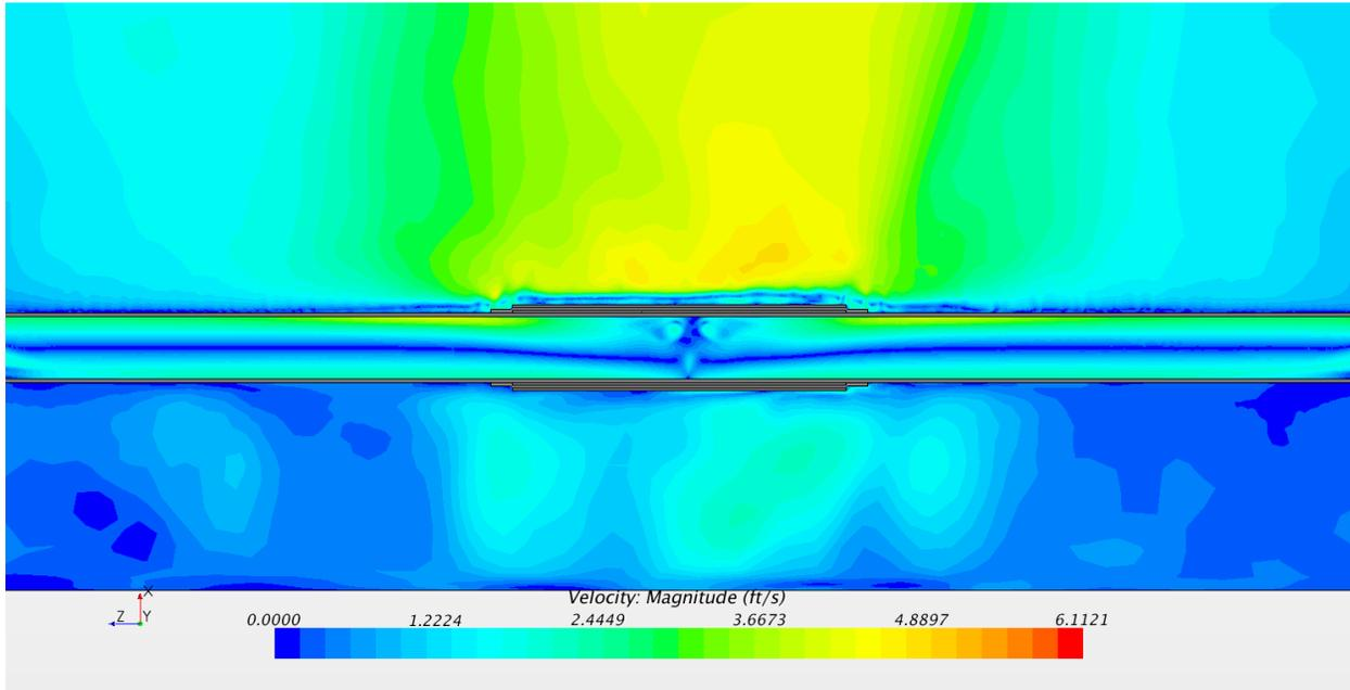
**Figure B-80: Velocity contours, cross section of all regions, isometric view (ft/s). 24 inch schedule 80**
