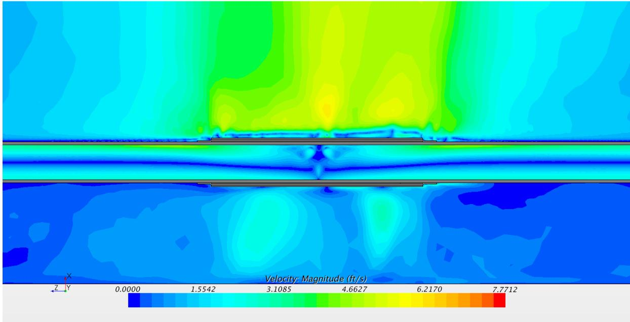
**Figure B-112: Velocity contours, cross section of all regions, isometric view (ft/s). 30 inch schedule 120**
