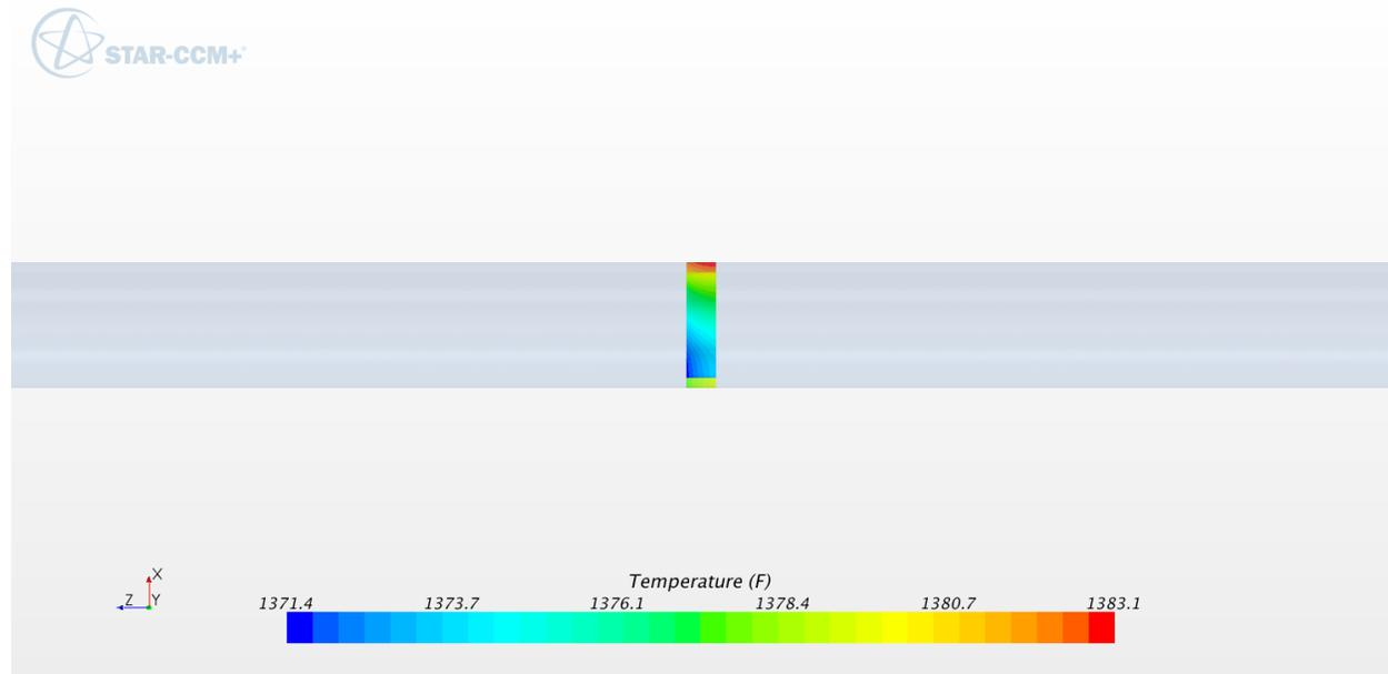
**Figure B-62: Temperature contours in SB, isometric view (°F). 14 inch schedule 120.**
