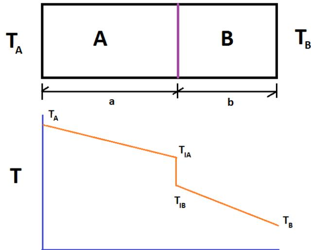
Note that the contact between bodies create a discontinuity in the temperature distribution. The heat flow across a contact boundary can be written as
