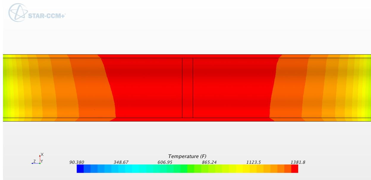
**Figure B-53: Temperature contours in SB (°F). 14 inch schedule 80**
