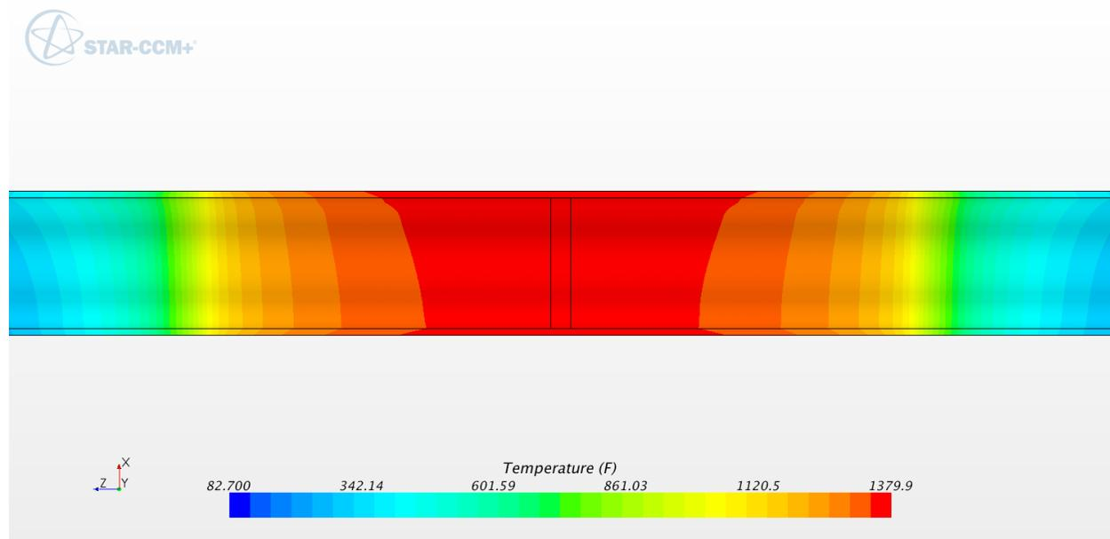
**Figure B-101: Temperature contours in SB (°F). 30 inch schedule 80**
