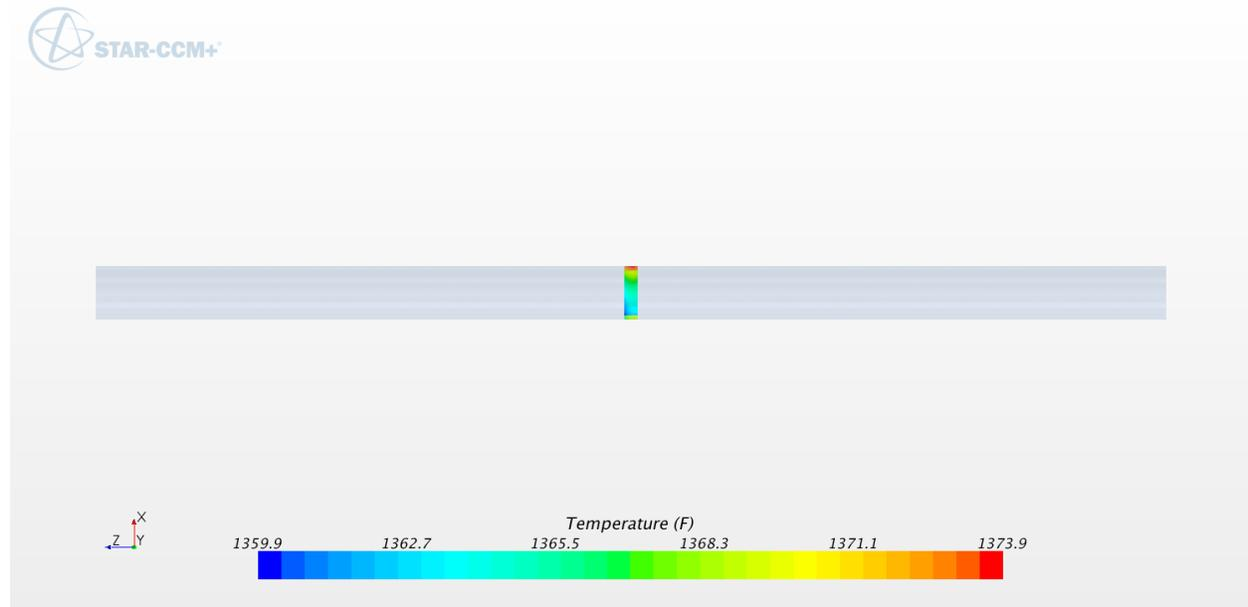
**Figure B-14: Temperature contours in SB, isometric view (°F). 6 inch schedule 120**
