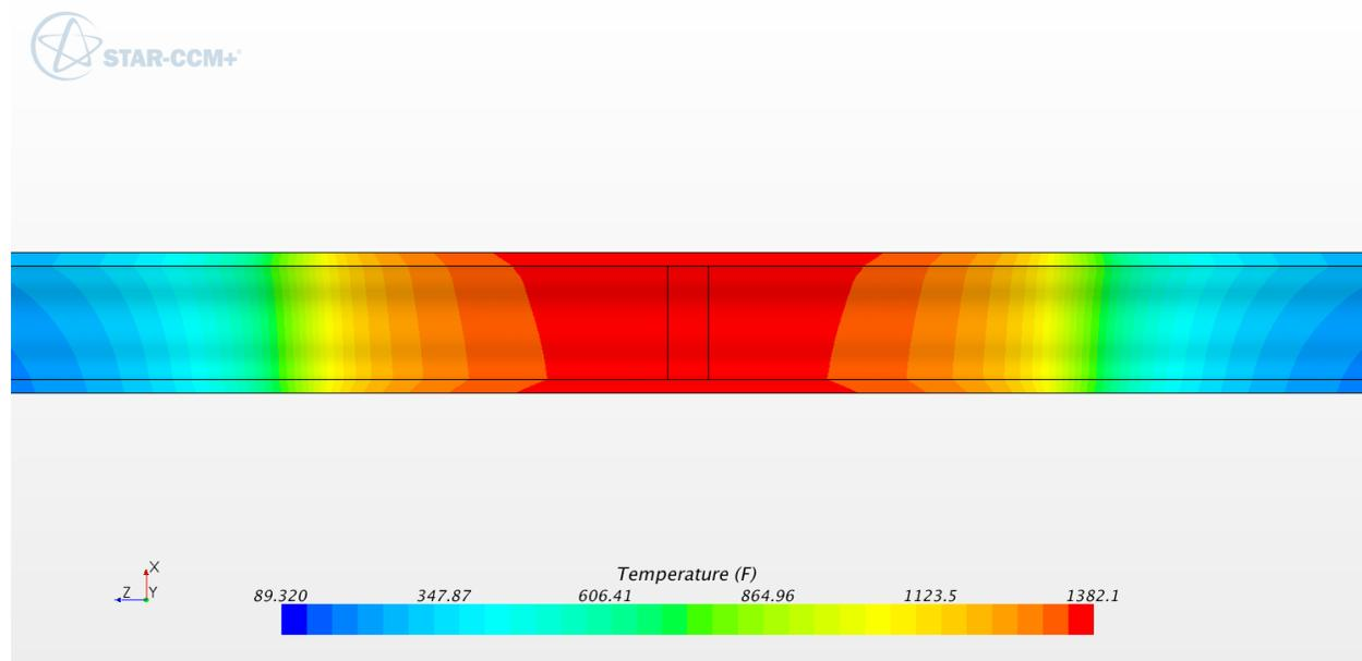
**Figure B-93: Temperature contours in SB (°F). 24 inch schedule 160**
