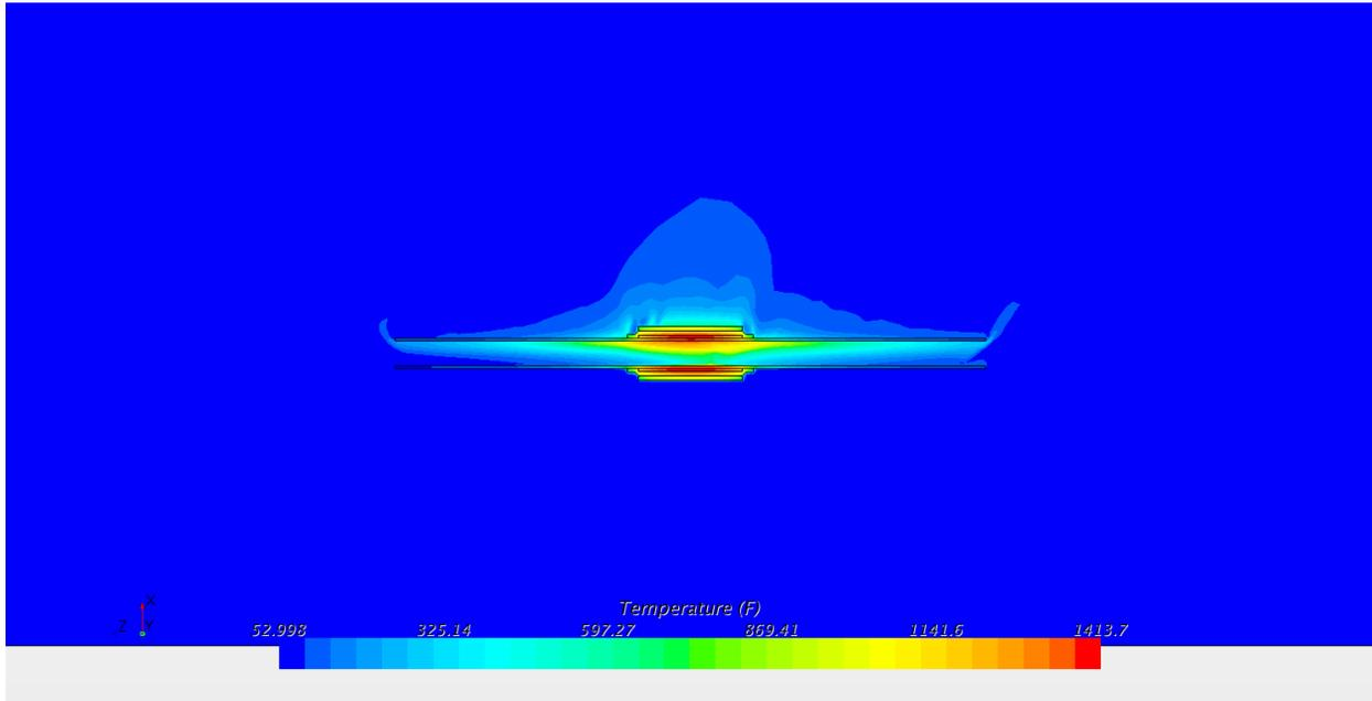
**Figure B-10: Temperature contours, cross section of all regions, close-up (°F). 6 inch schedule 120**
