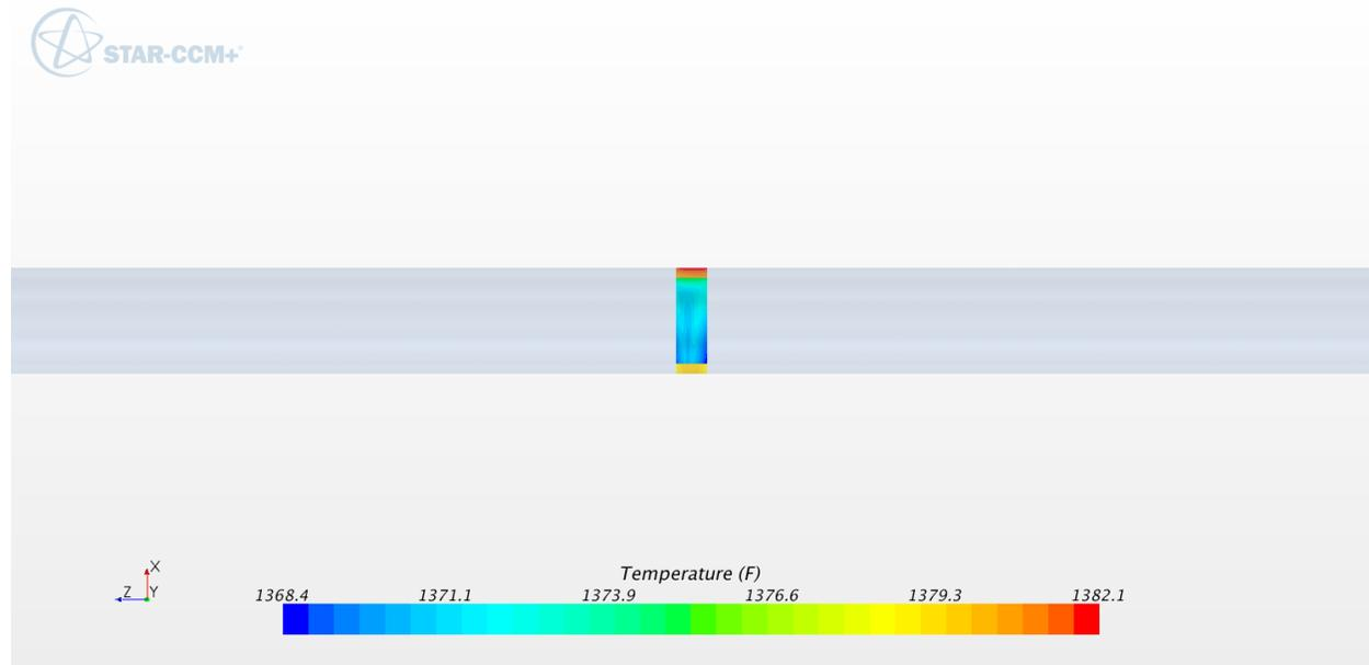
**Figure B-94: Temperature contours in SB, isometric view (°F). 24 inch schedule 160**
