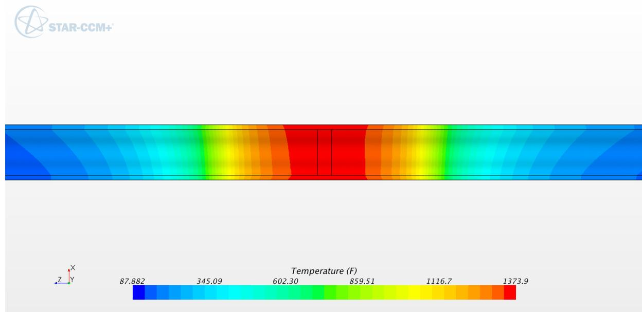
**Figure B-13: Temperature contours in SB (°F). 6 inch schedule 120**
