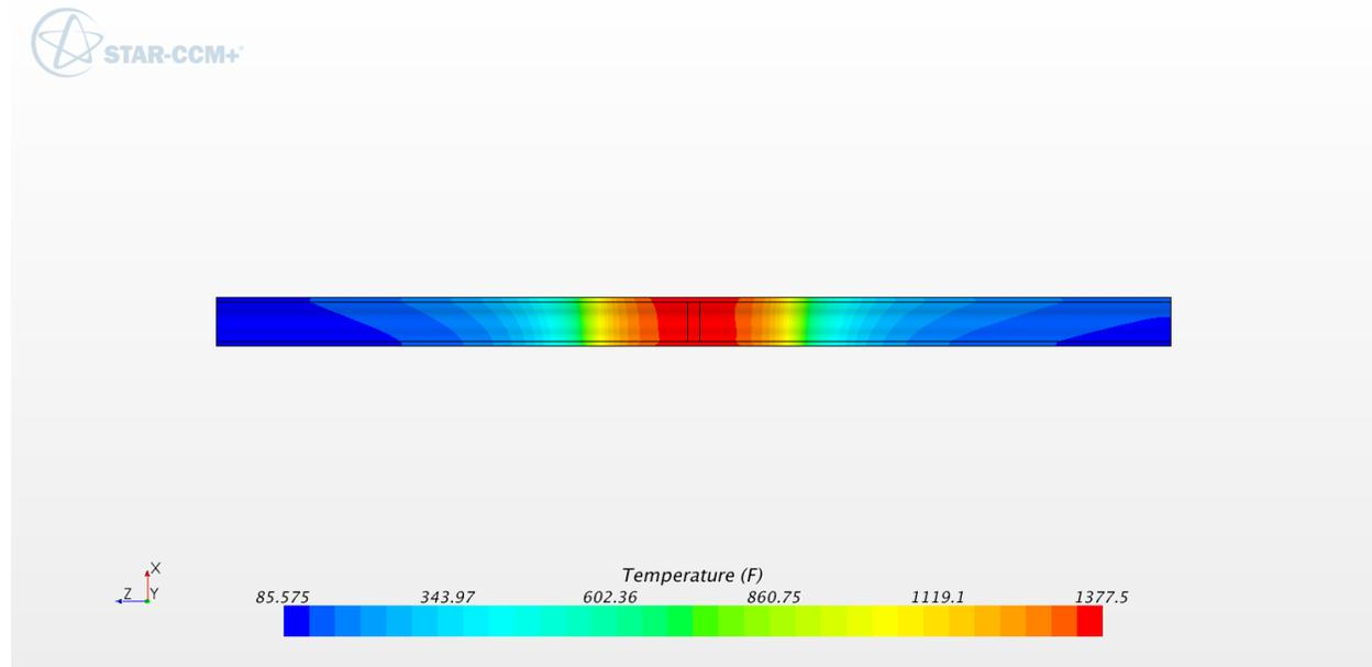
**Figure B-36: Temperature contours in pipe wall, close-up (°F). 10 inch schedule 120**
