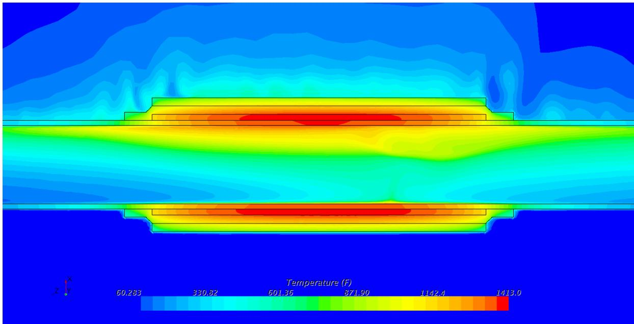
**Figure B-27: Temperature contours in pipe wall (°F). 10 inch schedule 80**
