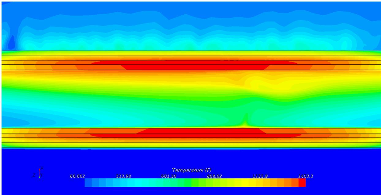
**Figure B-59: Temperature contours in pipe wall (°F). 14 inch schedule 120**
