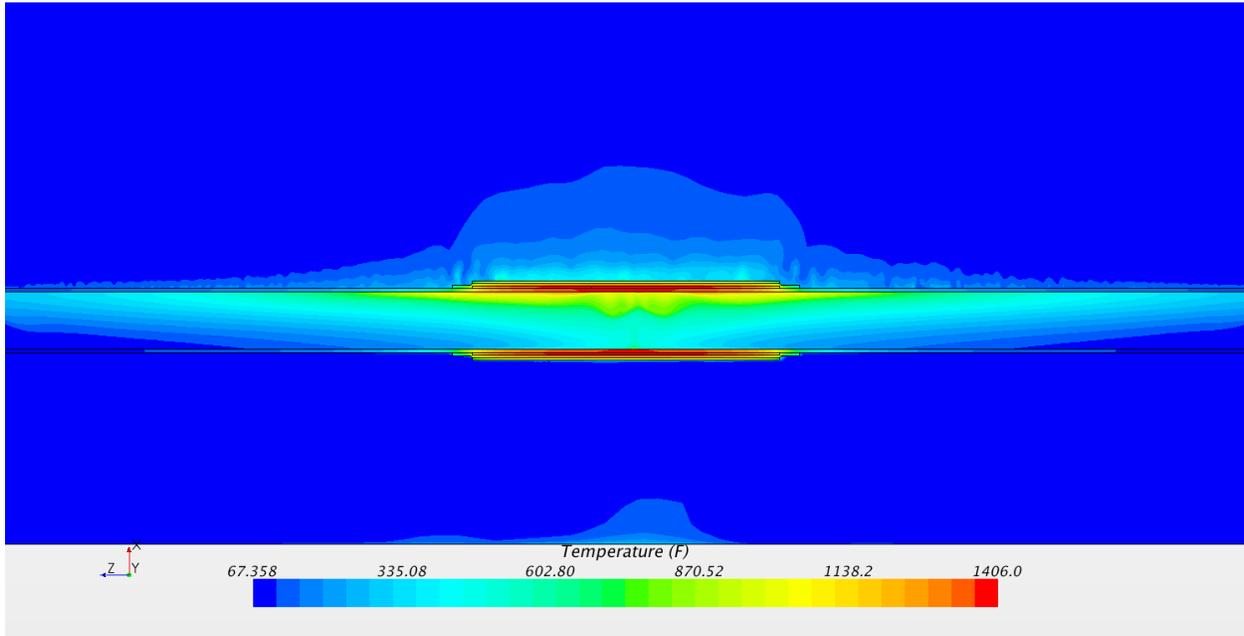
**Figure B-74: Temperature contours, cross section of all regions, close-up (°F). 24 inch schedule 80**
