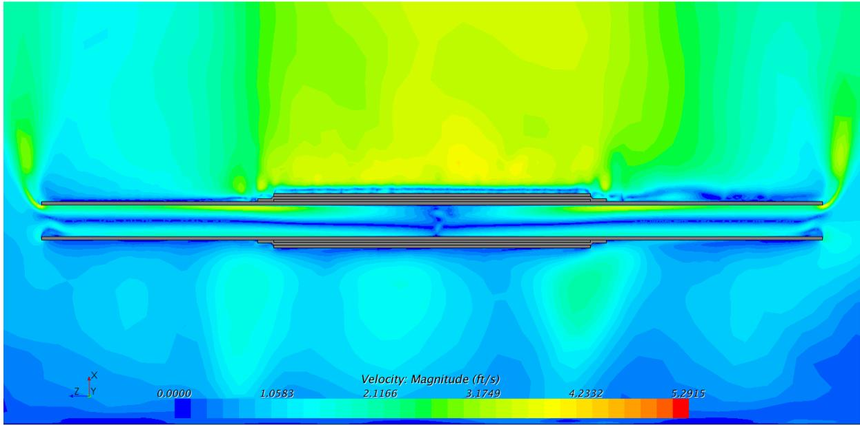
**Figure B-72: Velocity contours, cross section of all regions, isometric view (ft/s). 14 inch schedule 160**
