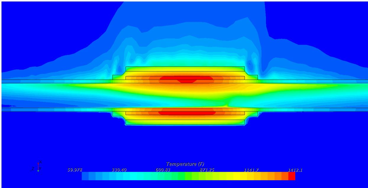
**Figure B-19: Temperature contours in pipe wall (°F). 6 inch schedule 160**
