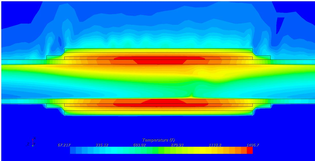
**Figure B-43: Temperature contours in pipe wall (°F). 10 inch schedule 160**
