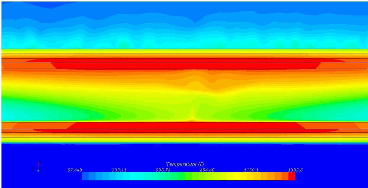
**Figure B-67: Temperature contours in pipe wall (°F). 14 inch schedule 160**
