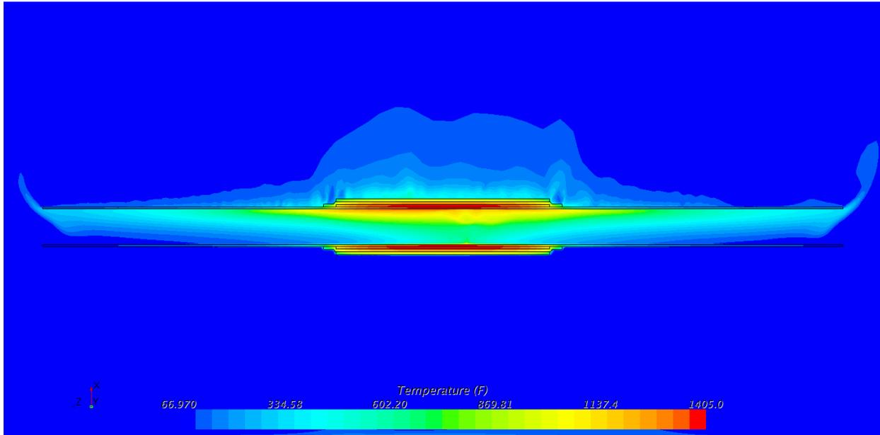
**Figure B-50: Temperature contours, cross section of all regions, close-up (°F). 14 inch schedule 80**
