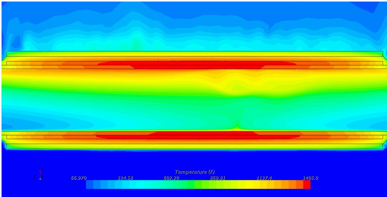
**Figure B-51: Temperature contours in pipe wall (°F). 14 inch schedule 80**
