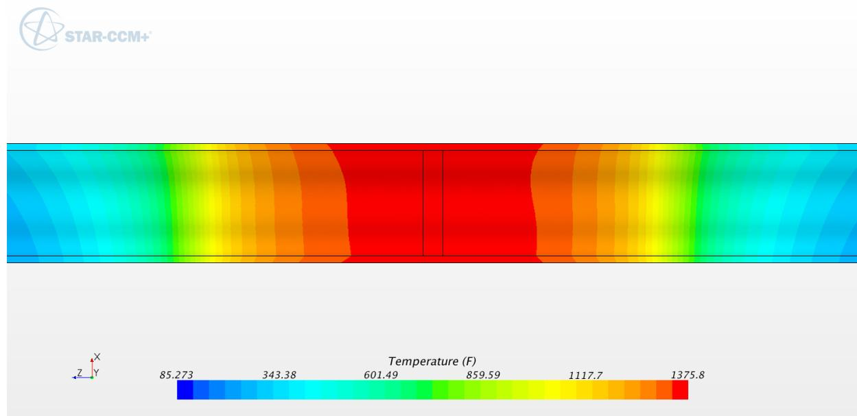
**Figure B-29: Temperature contours in SB (°F). 10 inch schedule 80**
