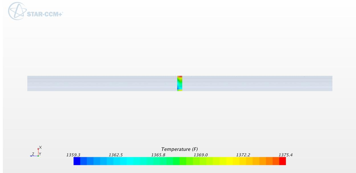
**Figure B-22: Temperature contours in SB, isometric view (°F). 6 inch schedule 160**
