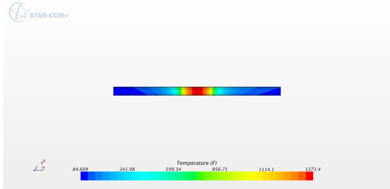
**Figure B-4: Temperature contours in pipe wall, close-up (°F). 6 inch schedule 80**
