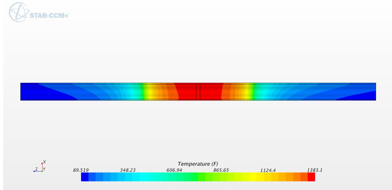
**Figure B-60: Temperature contours in pipe wall, close-up (°F). 14 inch schedule 120**
