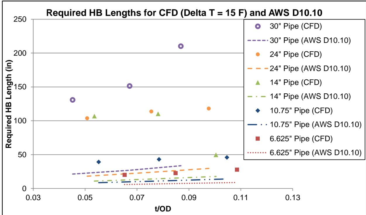
**Figure 3-12: Ratio of CFD HB length for SB delta T=15°F over HB length from AWS D10.10**
