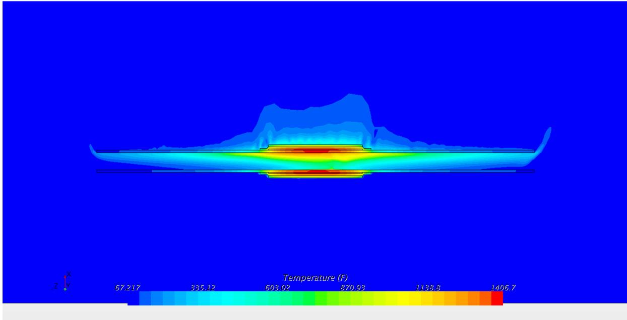
**Figure B-42: Temperature contours, cross section of all regions, close-up (°F). 10 inch schedule 160**
