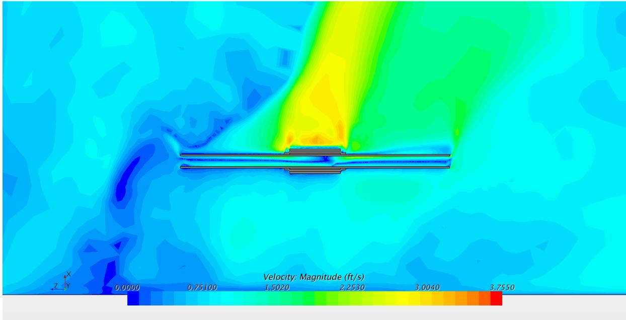
**Figure B-24: Velocity contours, cross section of all regions, isometric view (ft/s). 6 inch schedule 160**
