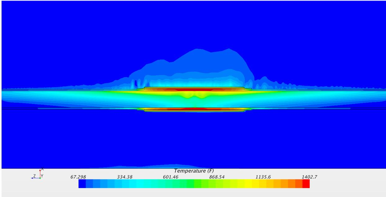
**Figure B-82: Temperature contours, cross section of all regions, close-up (°F). 24 inch schedule 120**
