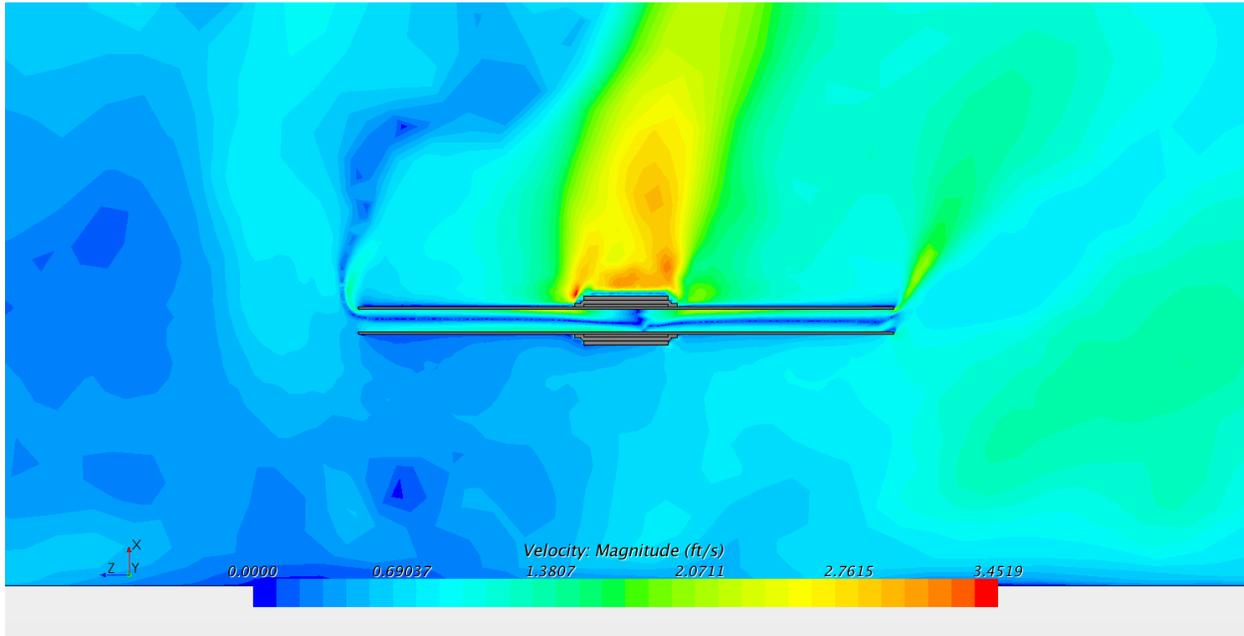
**Figure B-8: Velocity contours, cross section of all regions, isometric view (ft/s). 6 inch schedule 80**
