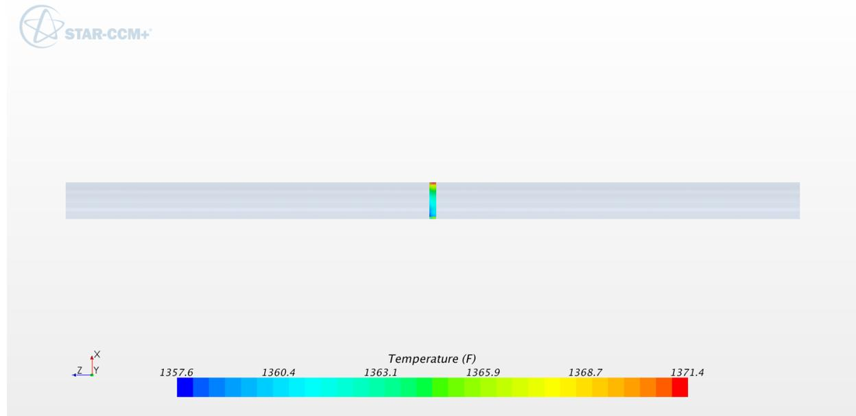
**Figure B-6: Temperature contours in SB, isometric view (°F). 6 inch schedule 80**
