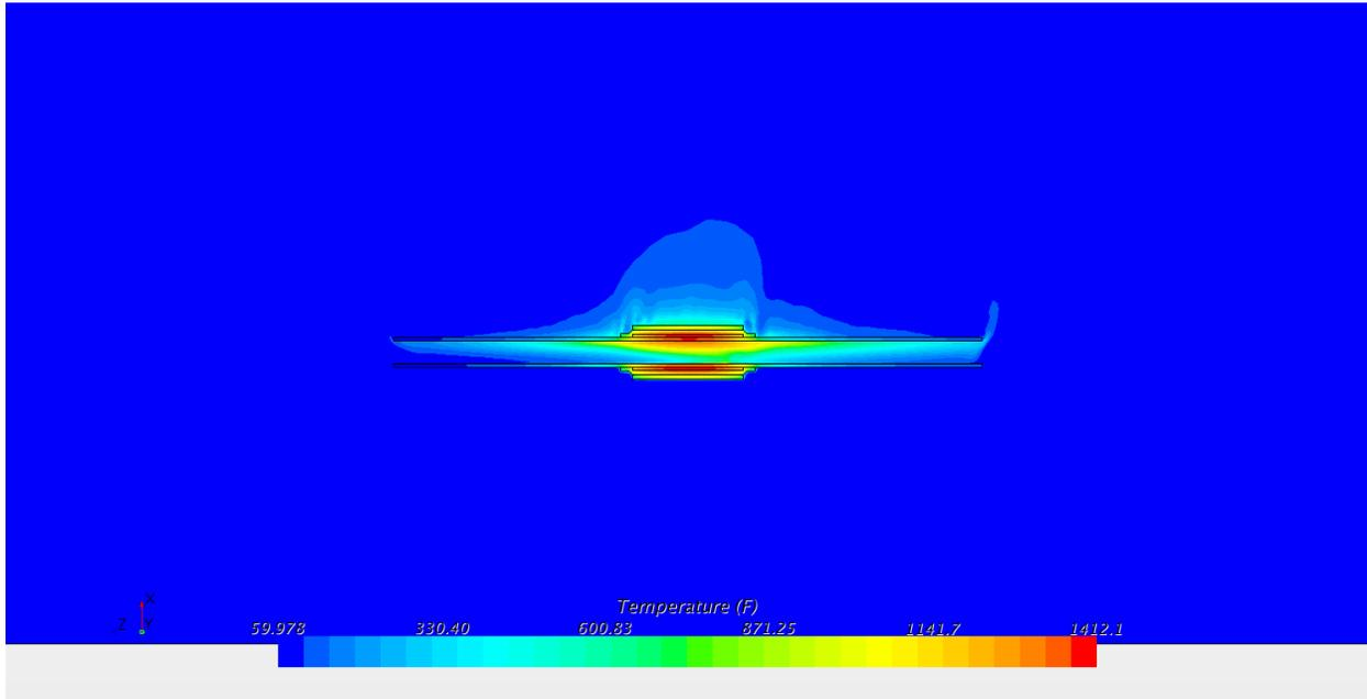
**Figure B-18: Temperature contours, cross section of all regions, close-up (°F). 6 inch schedule 160**
