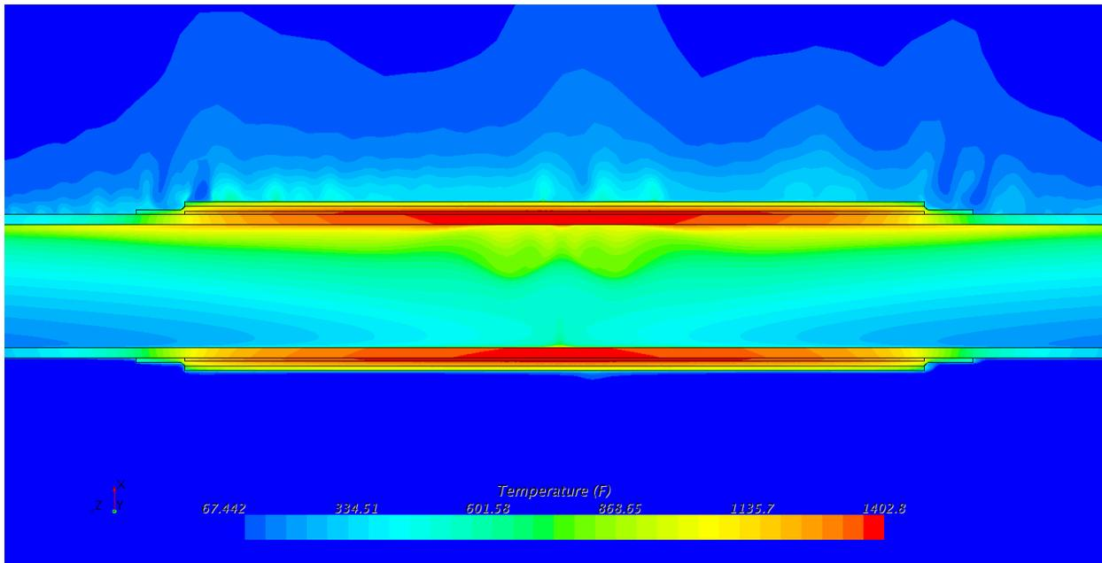
**Figure B-107: Temperature contours in pipe wall (°F). 30 inch schedule 120**
