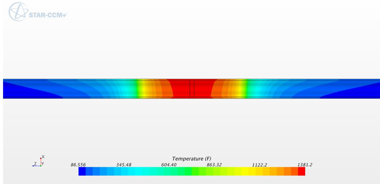
**Figure B-84: Temperature contours in pipe wall, close-up (°F). 24 inch schedule 120**
