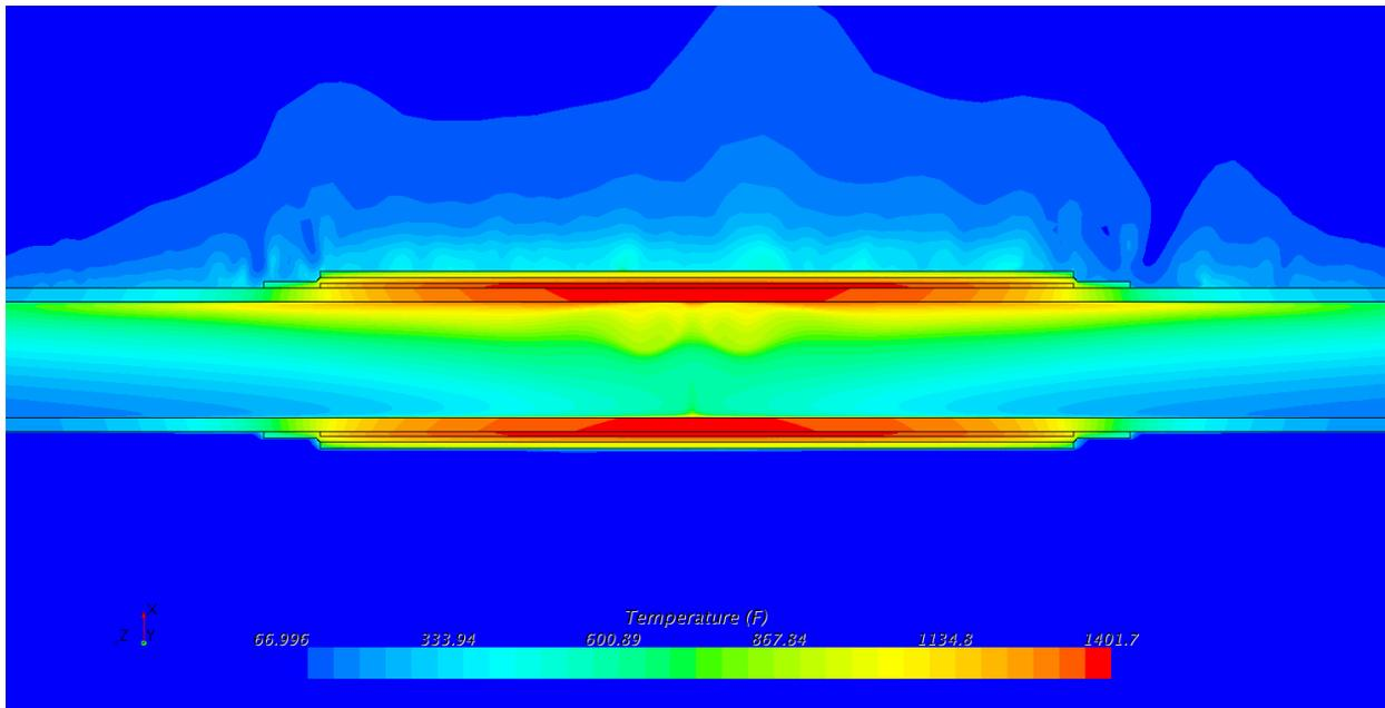
**Figure B-91: Temperature contours in pipe wall (°F). 24 inch schedule 160**
