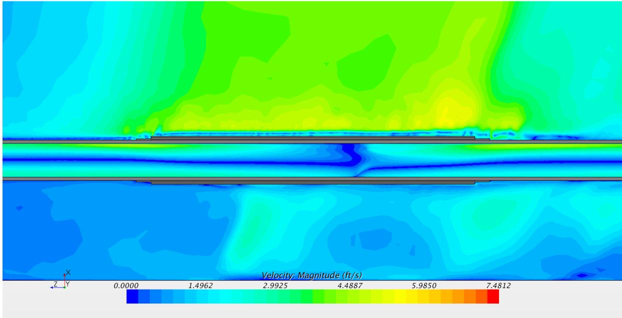
**Figure B-120: Velocity contours, cross section of all regions, isometric view (ft/s). 30 inch schedule 160**
