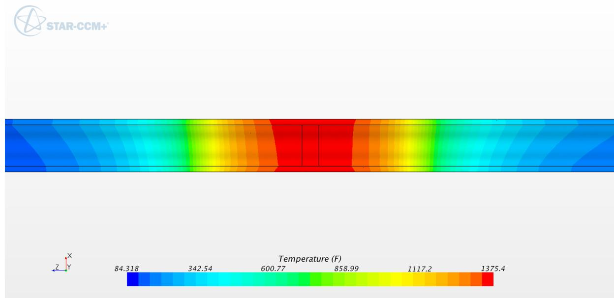
**Figure B-21: Temperature contours in SB (°F). 6 inch schedule 160**
