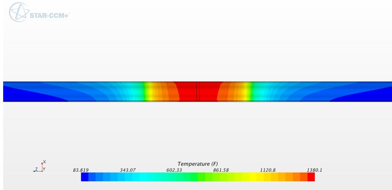
**Figure B-76: Temperature contours in pipe wall, close-up (°F). 24 inch schedule 80**
