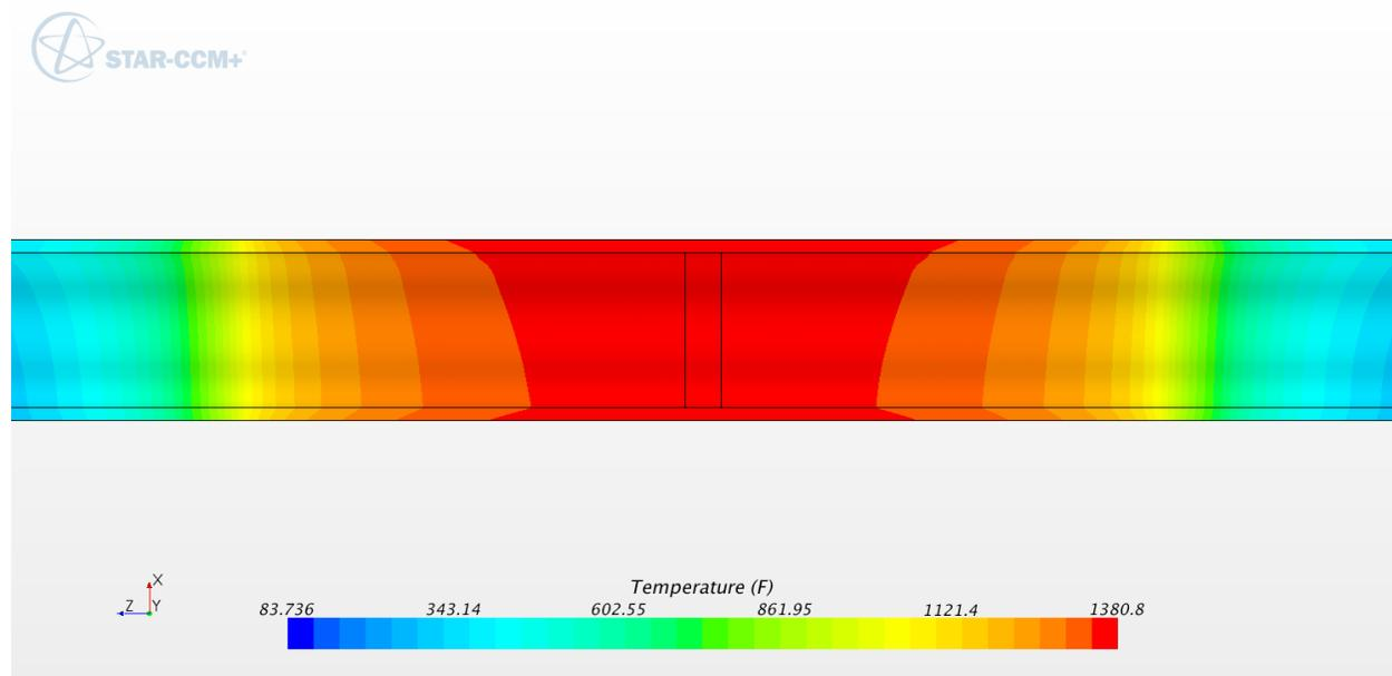
**Figure B-109: Temperature contours in SB (°F). 30 inch schedule 120**
