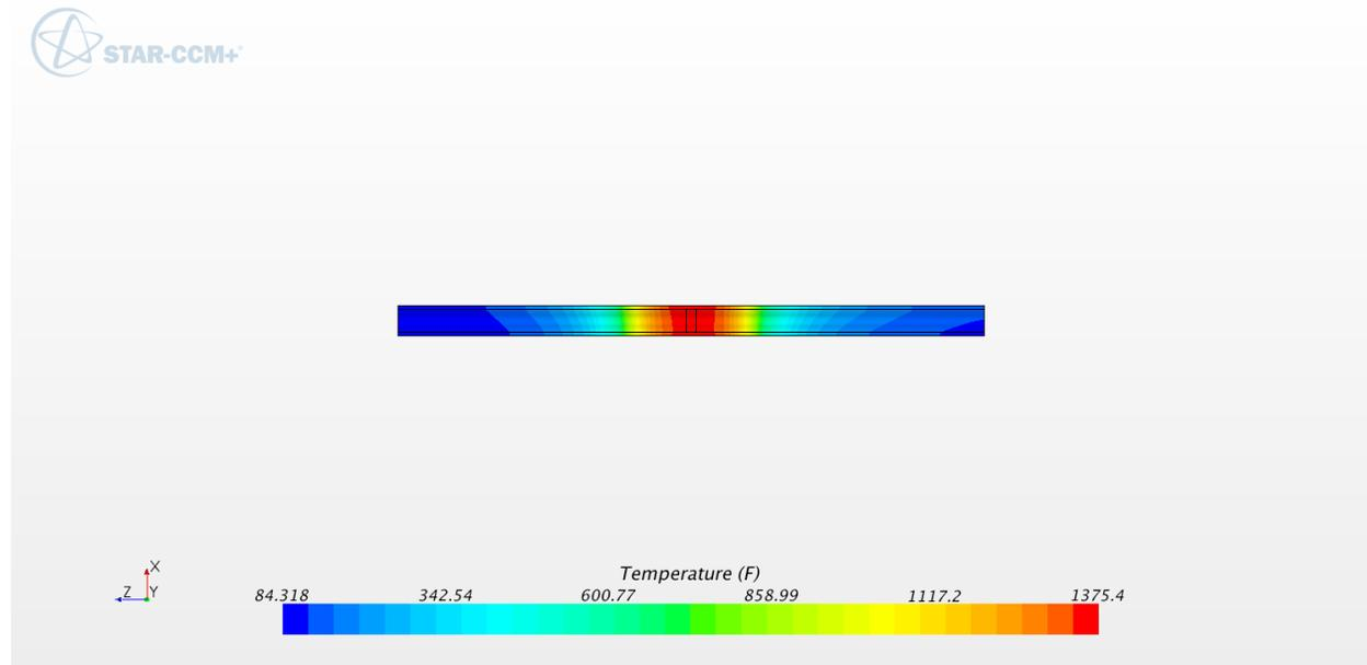
**Figure B-20: Temperature contours in pipe wall, close-up (°F). 6 inch schedule 160**
