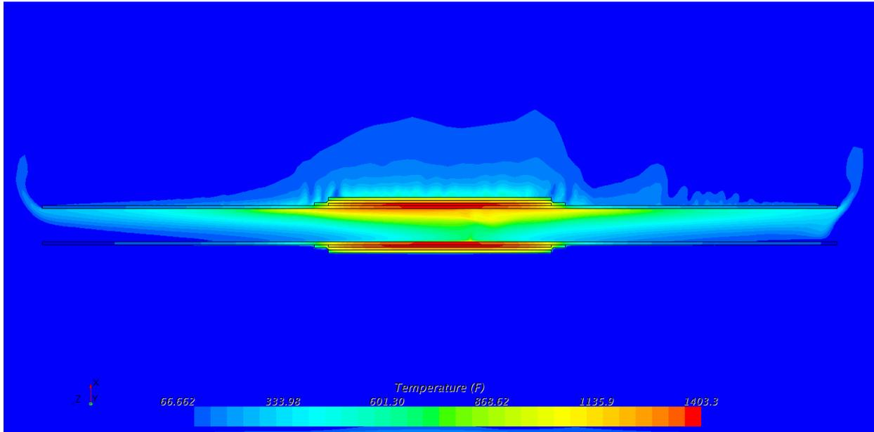
**Figure B-58: Temperature contours, cross section of all regions, close-up (°F). 14 inch schedule 120**
