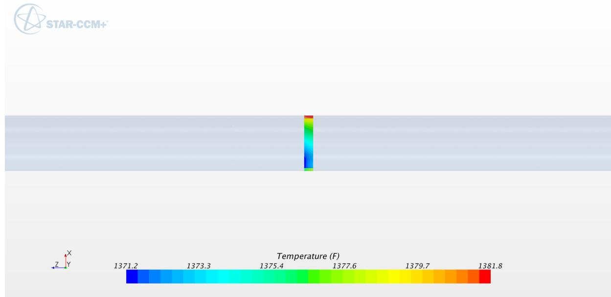
**Figure B-54: Temperature contours in SB, isometric view (°F). 14 inch schedule 80**
