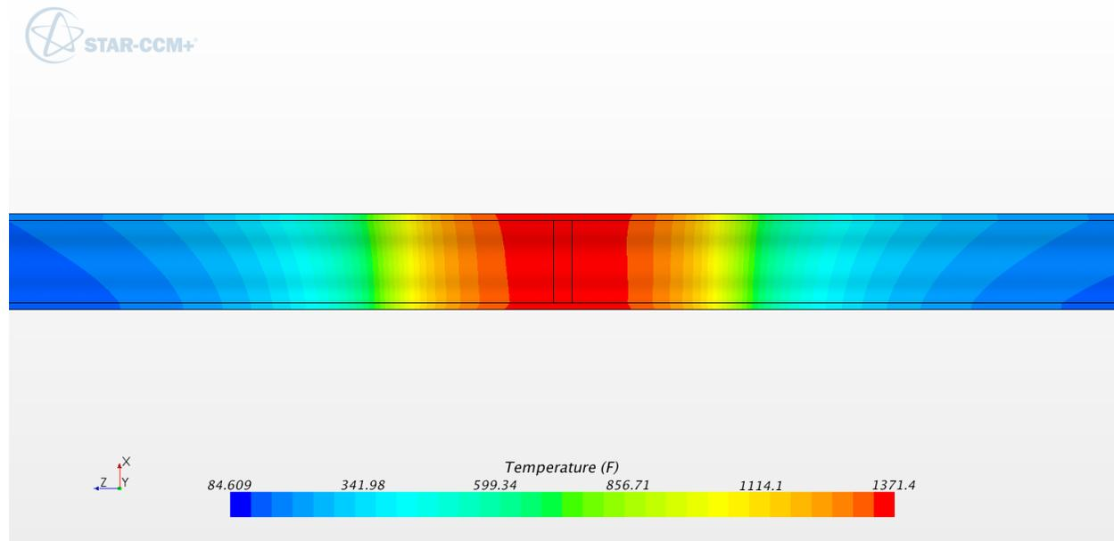
**Figure B-5: Temperature contours in SB (°F). 6 inch schedule 80**
