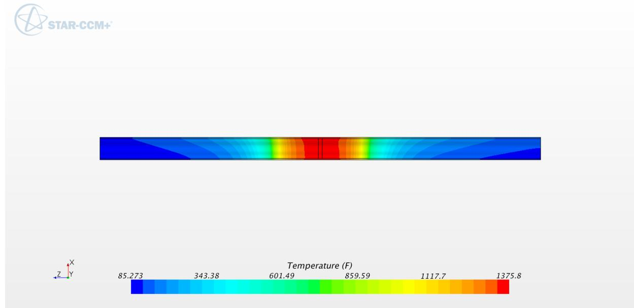
**Figure B-28: Temperature contours in pipe wall, close-up (°F). 10 inch schedule 80**
