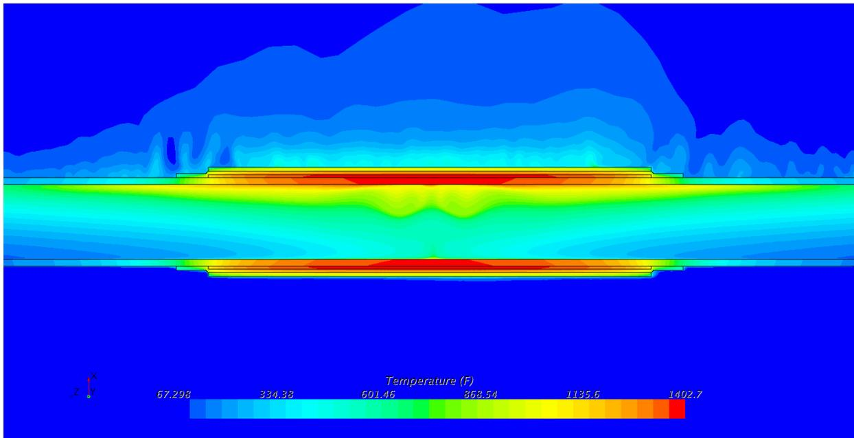
**Figure B-83: Temperature contours in pipe wall (°F). 24 inch schedule 120**
