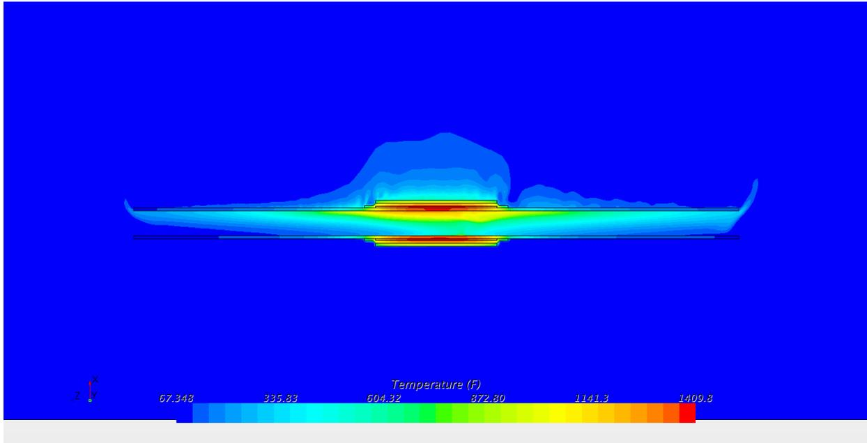
**Figure B-34: Temperature contours, cross section of all regions, close-up (°F). 10 inch schedule 120**
