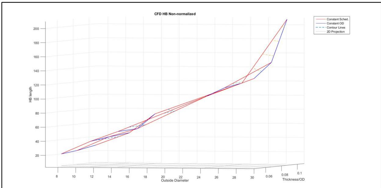
The ratio between the prescribed HB length given in AWS D10.10 [1] and the HB length calculated in this study shows an increasing disparity as the pipe diameter increases. This is due to the increased presence of natural convection on the ID surface of the larger diameter pipes. This disparity can be seen in Figure 3-11 and Figure 3-12. In all cases, a much larger HB length is likely required to obtain the target temperature distribution as compared to AWS guidelines.
