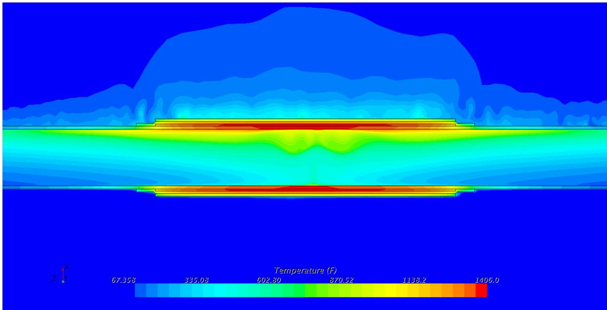
**Figure B-75: Temperature contours in pipe wall (°F). 24 inch schedule 80**
