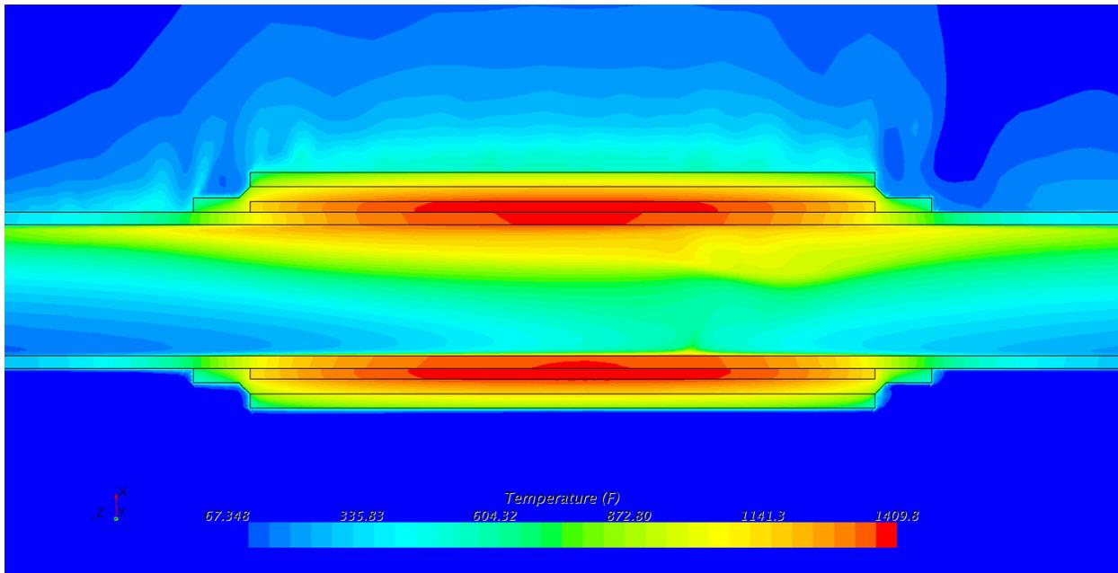
**Figure B-35: Temperature contours in pipe wall (°F). 10 inch schedule 120**
