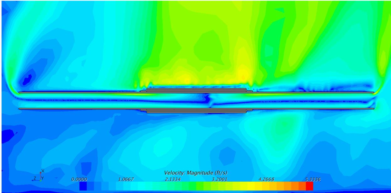
**Figure B-64: Velocity contours, cross section of all regions, isometric view (ft/s). 14 inch schedule 120**
