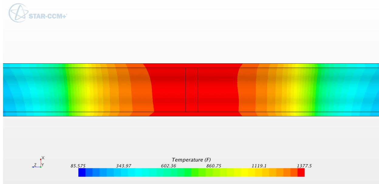
**Figure B-37: Temperature contours in SB (°F). 10 inch schedule 120**
