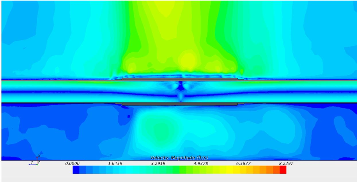
**Figure B-104: Velocity contours, cross section of all regions, isometric view (ft/s). 30 inch schedule 80**
