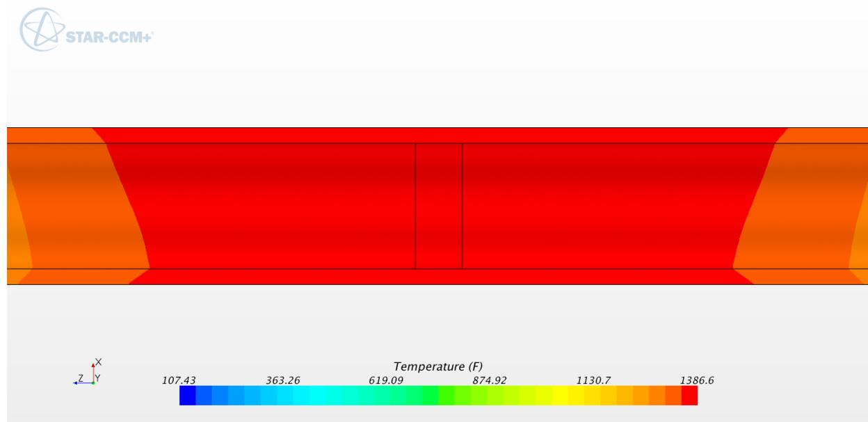
**Figure B-69: Temperature contours in SB (°F). 14 inch schedule 160**
