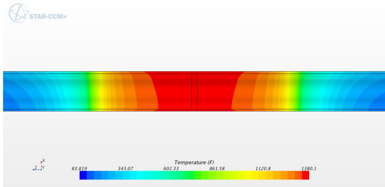
**Figure B-77: Temperature contours in SB (°F). 24 inch schedule 80**
