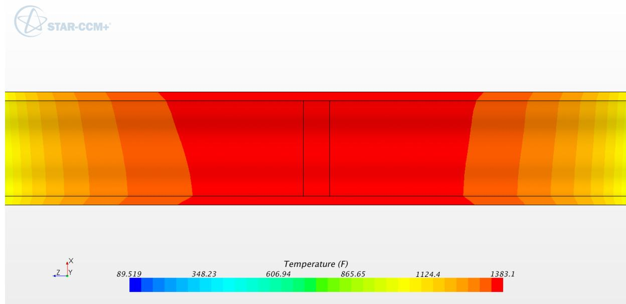
**Figure B-61: Temperature contours in SB (°F). 14 inch schedule 120**
