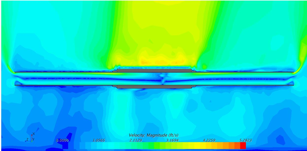
**Figure B-56: Velocity contours, cross section of all regions, isometric view (ft/s). 14 inch schedule 80**
