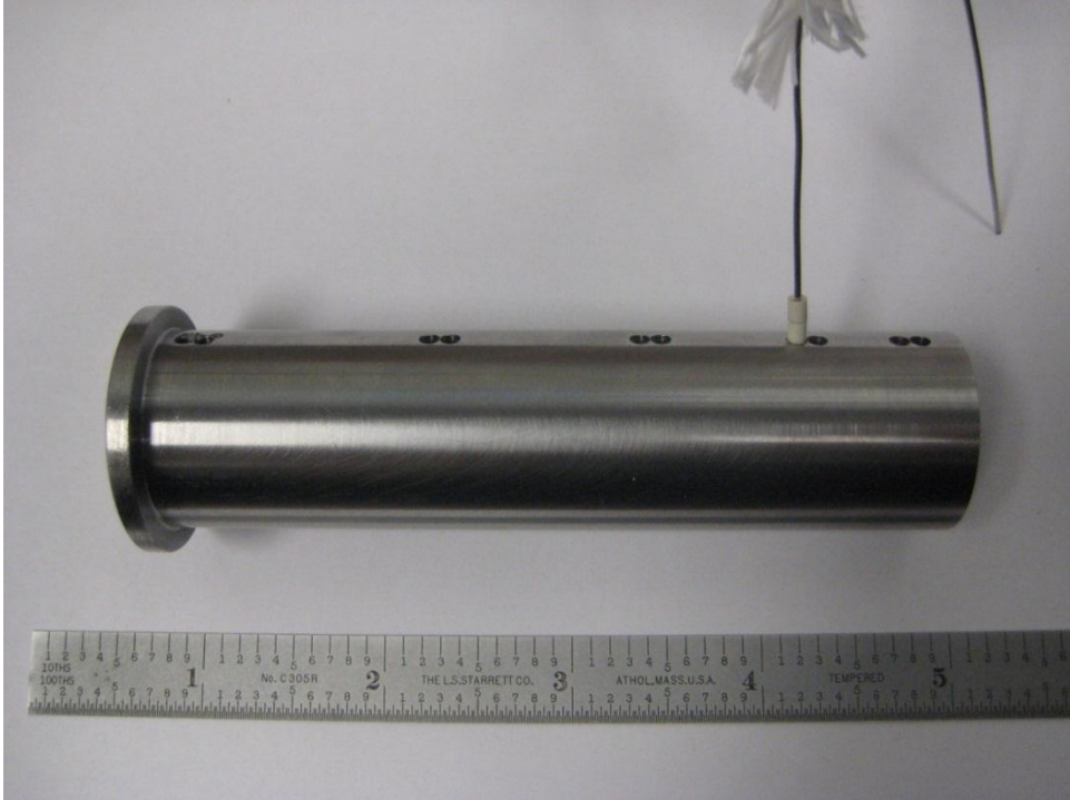
Figure 2-3: Thermocouple Locations, 0.25 in., 1.5 in., 2.5 in., and 3.75 in. from Quenched End of Jominy Bar
