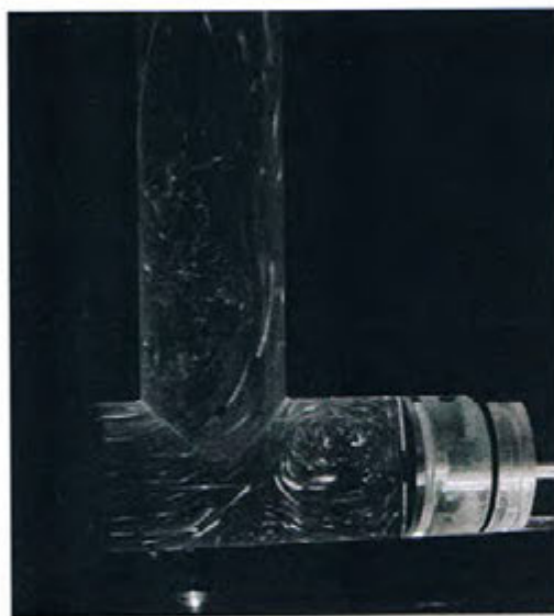
(b) Flow visualizations; L/D = 1
