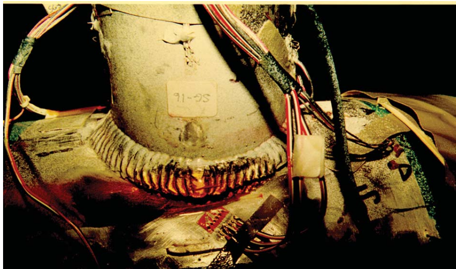
Figure 9 - EPRI Test Vessel-Pipe Nozzle Weld Failure
