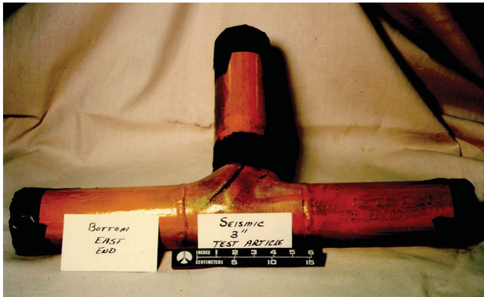
Figure 12 - EPRI System Test 2 Tee Failure
