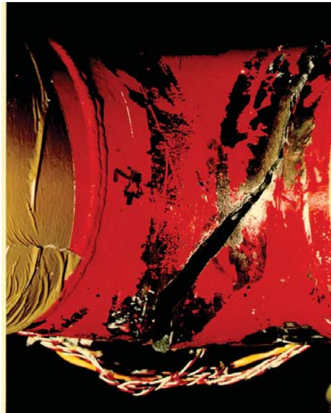
Figure 8 - EPRI Test Elbow Failure
