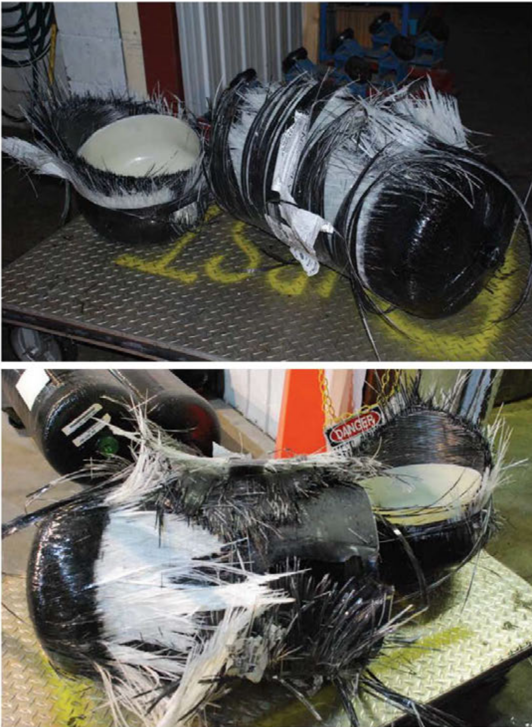
Figure C15: Tank 2C Burst Carcass
