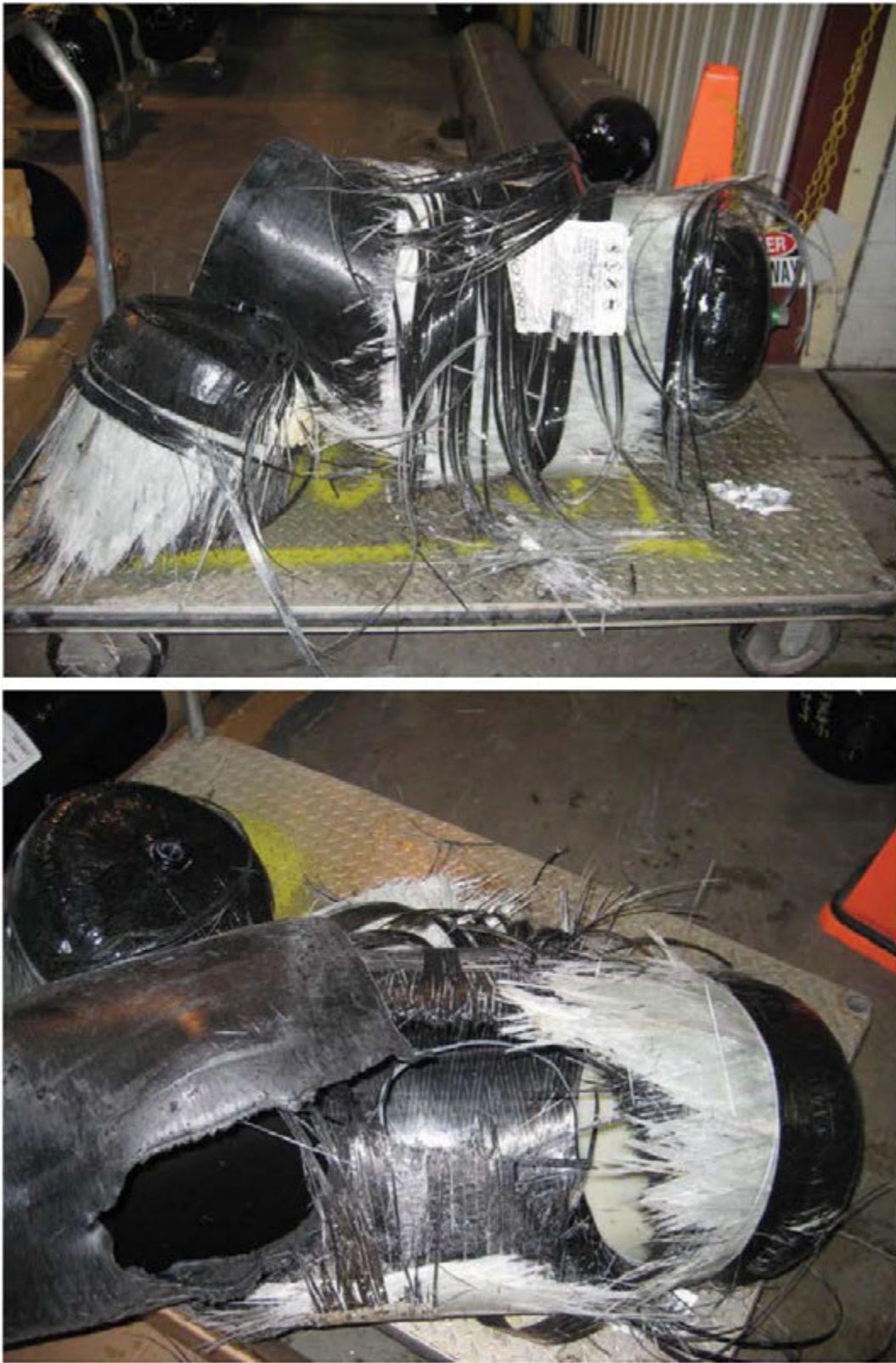
Figure C21: Tank 1B Burst Carcass
