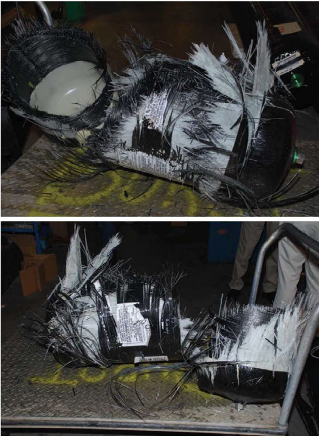
Figure C5: Tank 1A Burst Carcass
