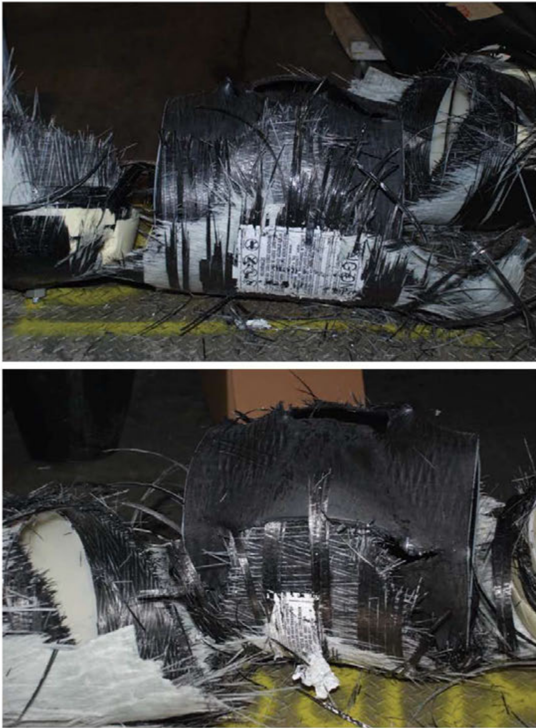
Figure C4: Tank 4A Burst Carcass
