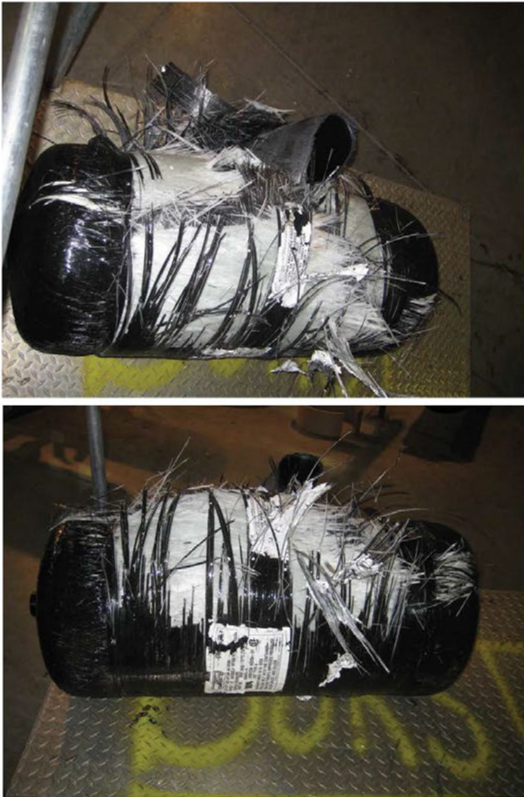
Figure C25: Tank 3B Burst Carcass
