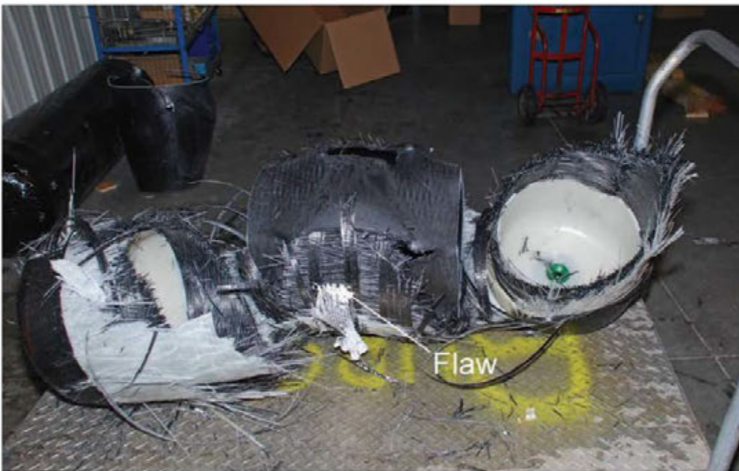
Figure C3: Tank 4A Burst Carcass
