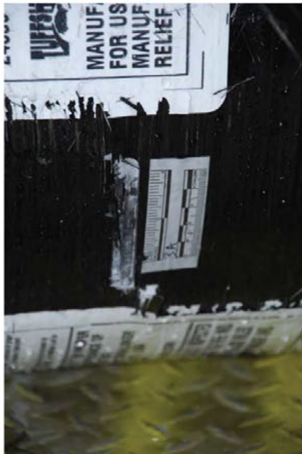
Figure C10: Tank 3A Burst Carcass
