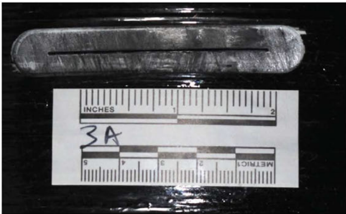
Figure A14: Tank 3A, Transverse Flaw Direction
