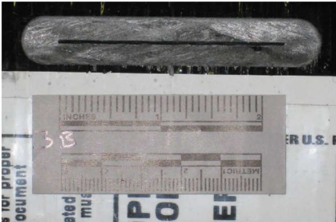
Figure 6 - Longitudinal Flaw in Tank 3B Before Cycling
