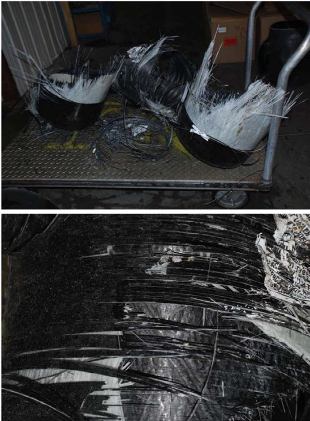
Figure C12: Tank 4C Burst Carcass
