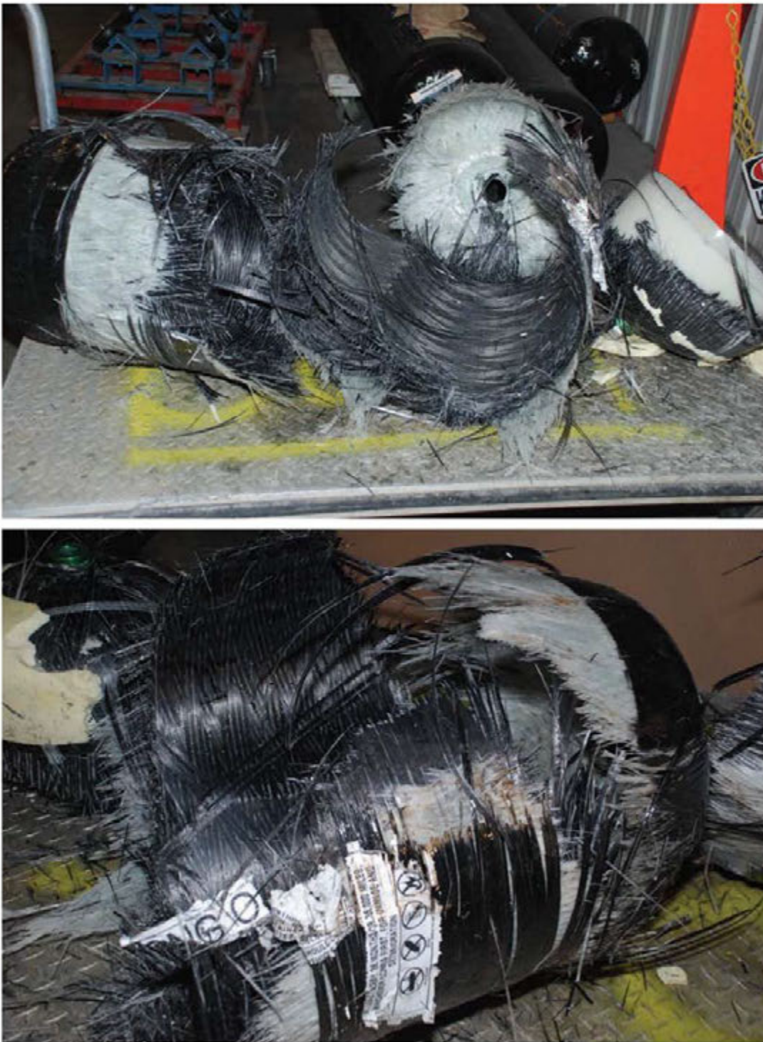
Figure C1: Tank 5 Burst Carcass
