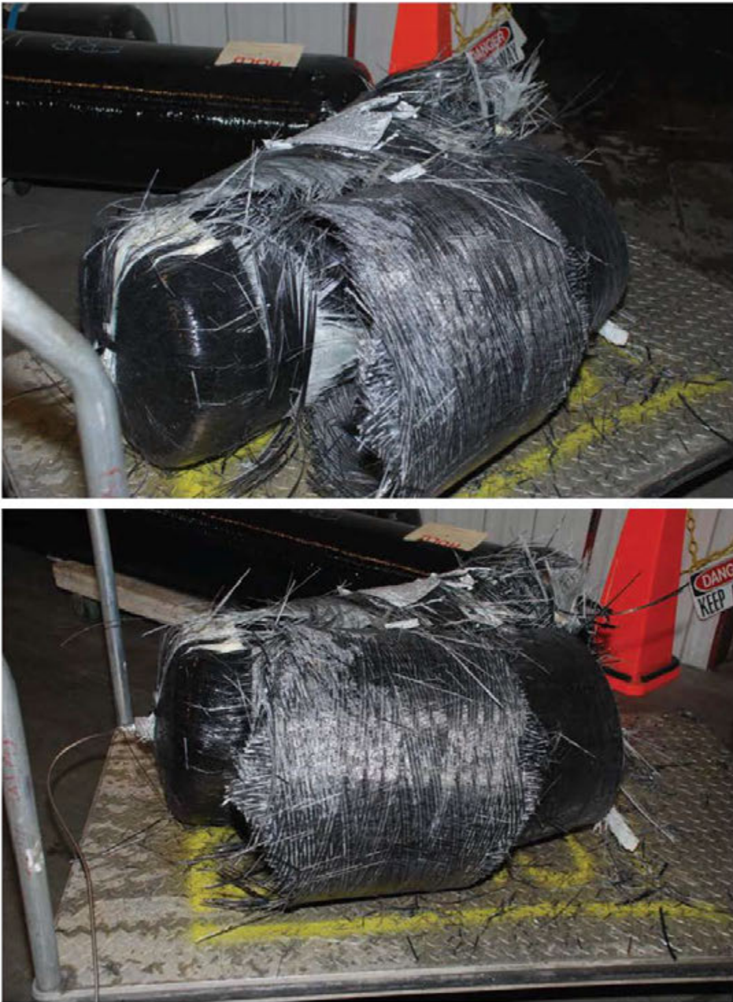
Figure C7: Tank 2A Burst Carcass
