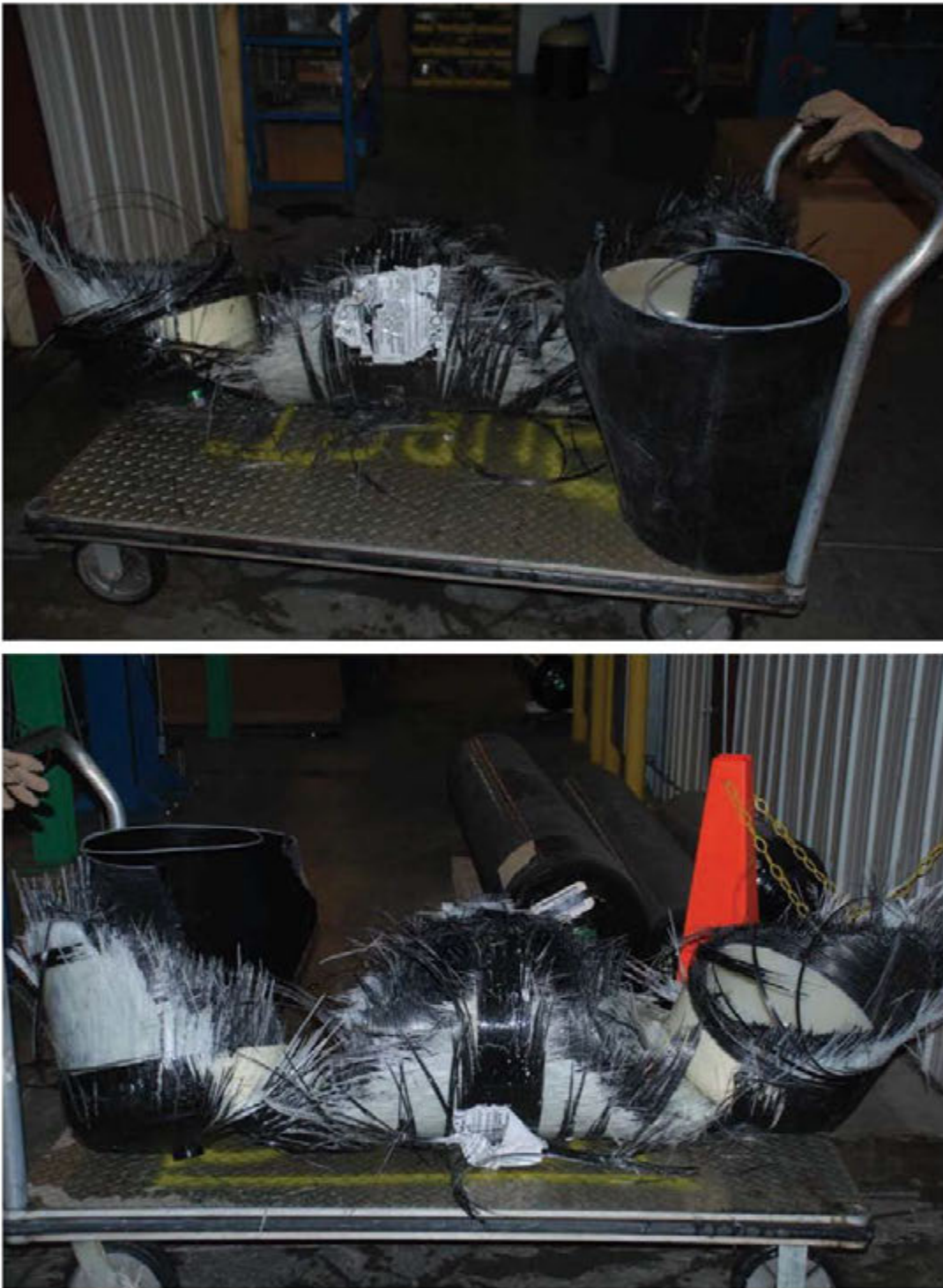
Figure C13: Tank 1C Burst Carcass
