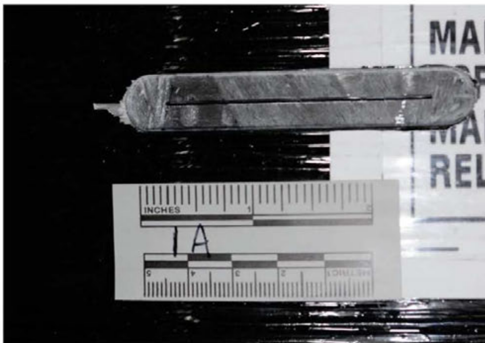
Figure A2: Tank 1A, Transverse Flaw Direction
