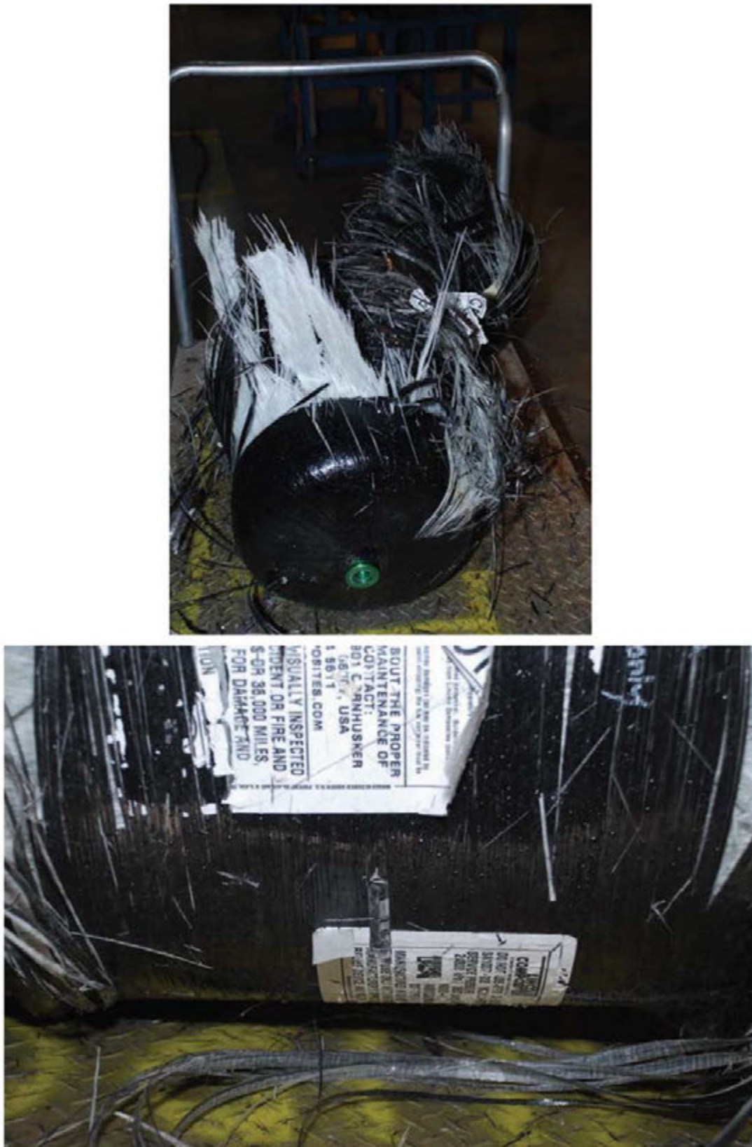
Figure C6: Tank 1A Burst Carcass
