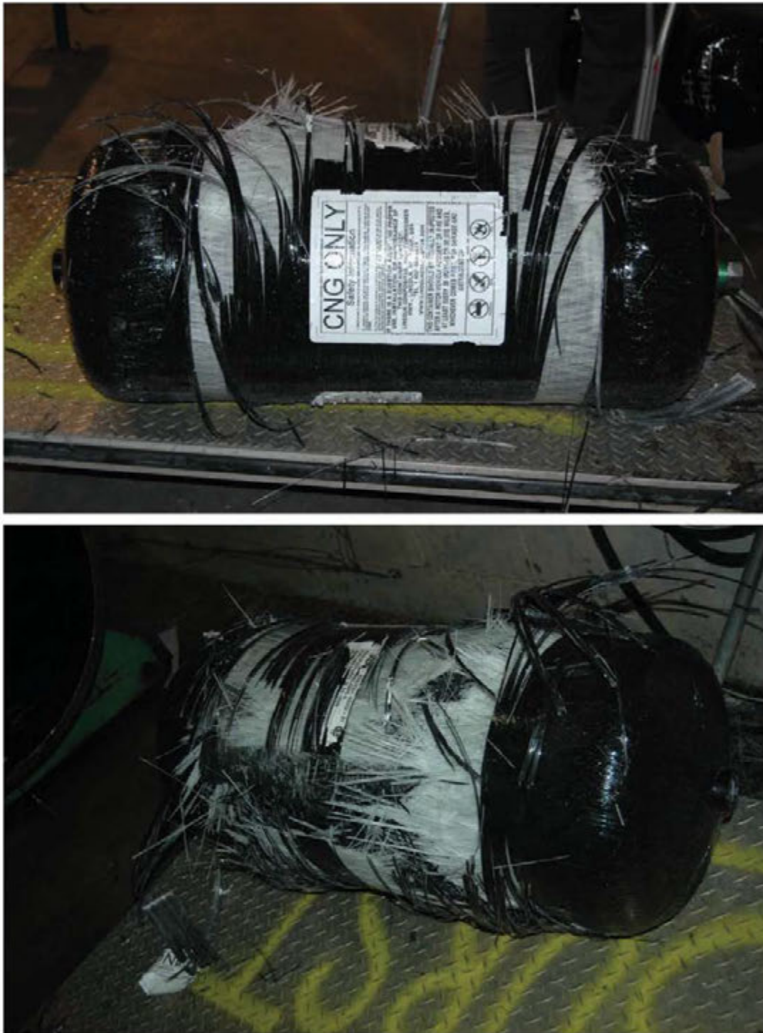
Figure C17: Tank 3C Burst Carcass
