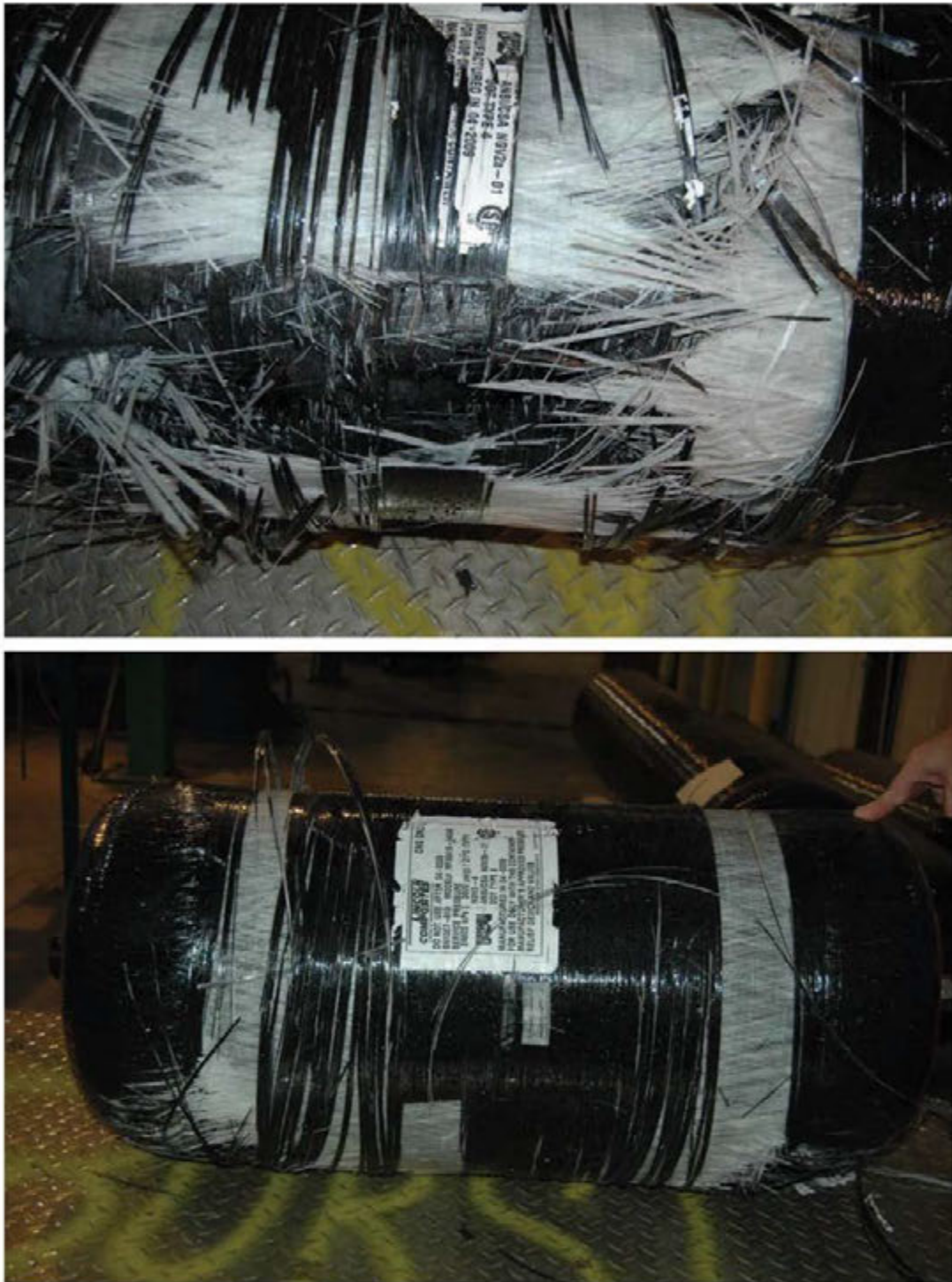
Figure C18: Tank 3C Burst Carcass
