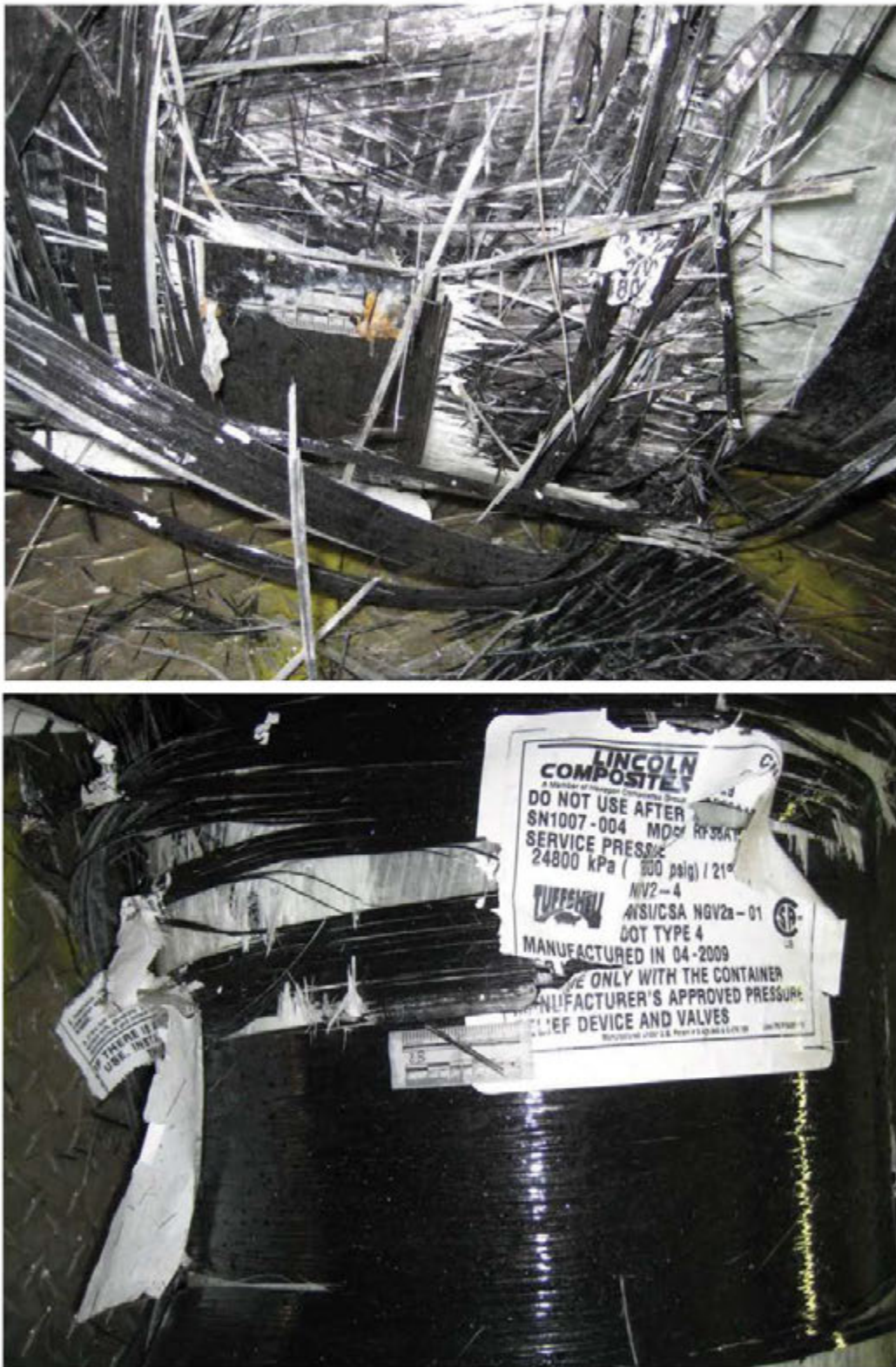
Figure C24: Tank 2B Burst Carcass
