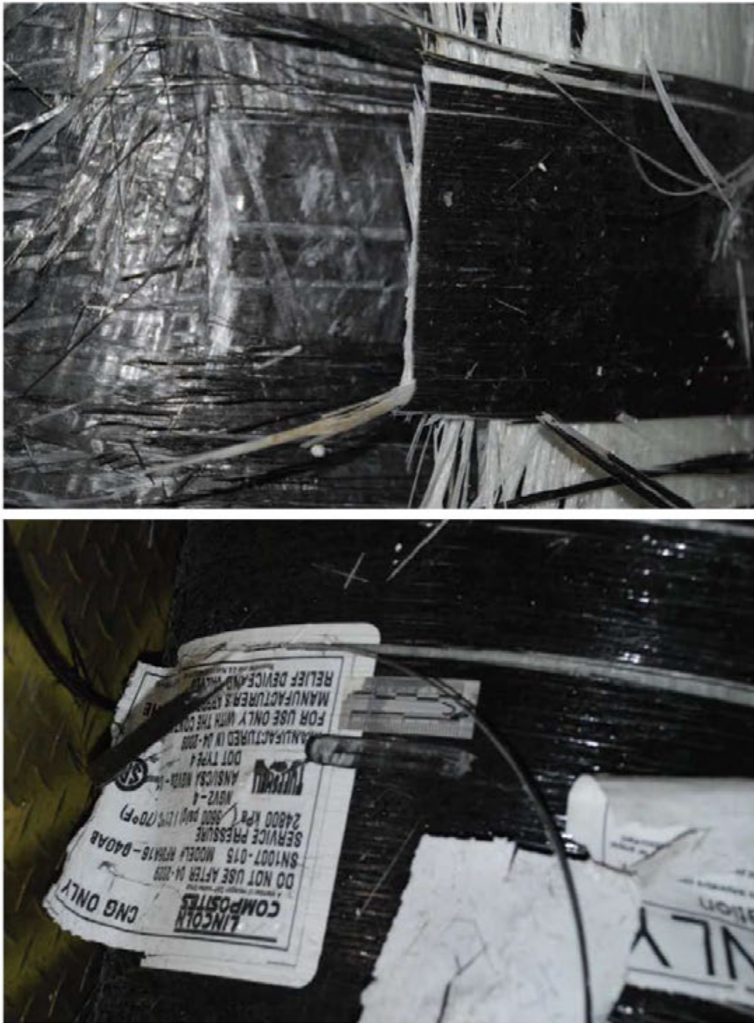
Figure C16: Tank 2C Burst Carcass
