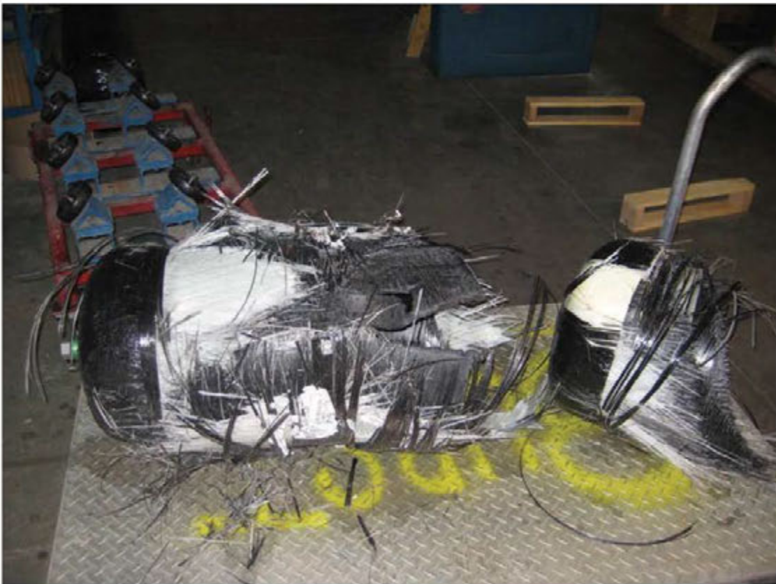
Figure C19: Tank 4B Burst Carcass
