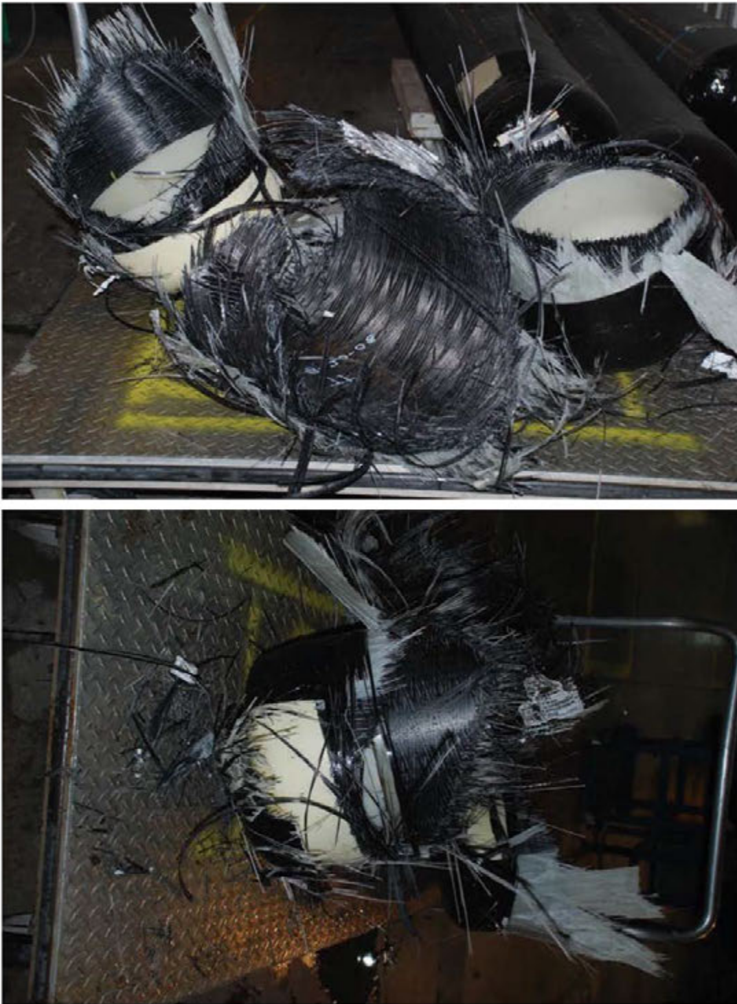
Figure C11: Tank 4C Burst Carcass
