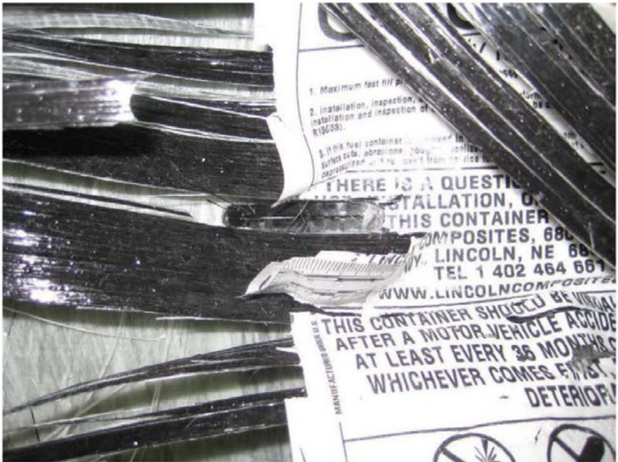
Figure C22: Tank 1B Burst Carcass
