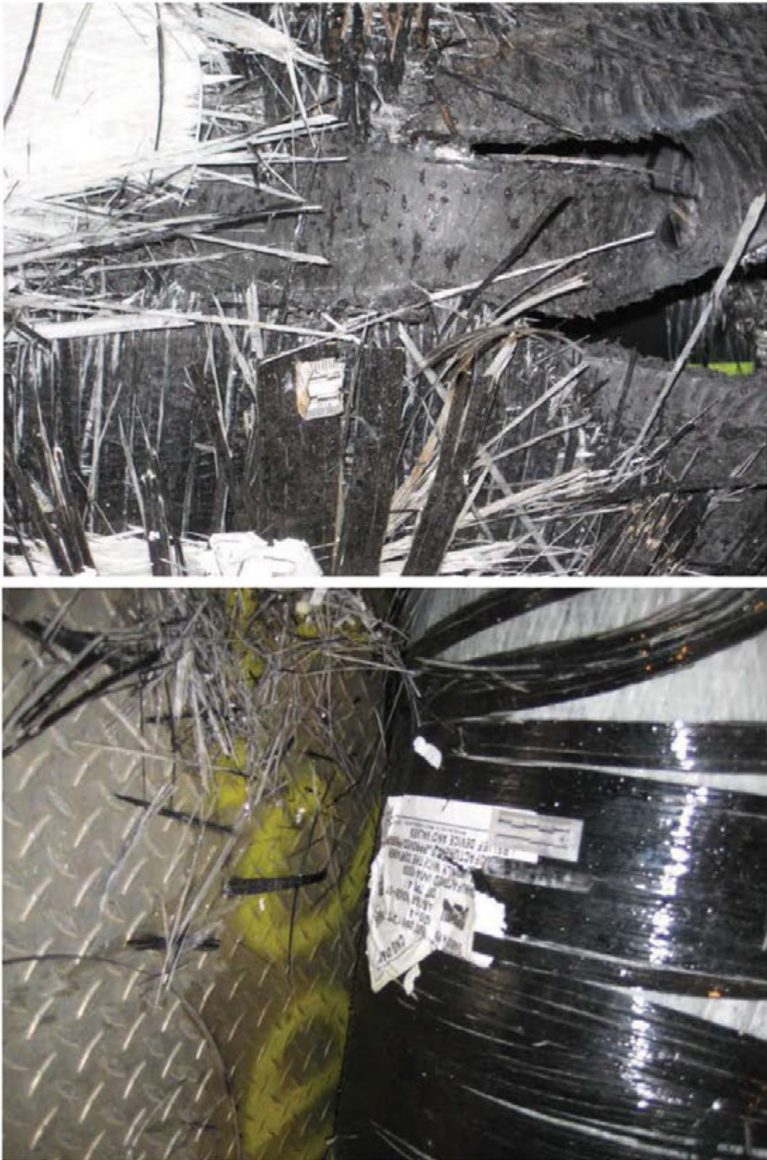
Figure C20: Tank 4B Burst Carcass
