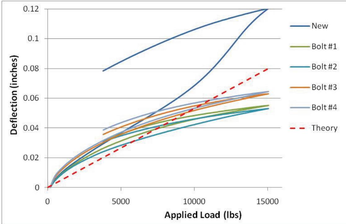
Figure 63 – 6 Belleville Washer Stack Load-Deformation Results
