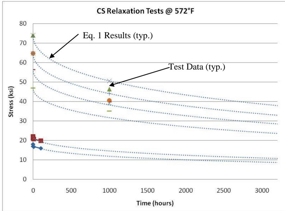
Figure 21 – Equation (1) Carbon Steel Relaxation Results at 572°F
