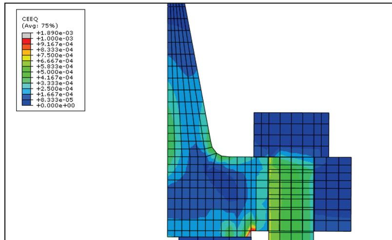
Figure 44 – NPS 6, cl. 150 Creep Strain @ 217 hrs
