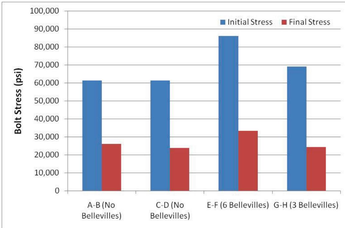
**Figure 61 – NPS 3, cl.150 Remaining Bolt Stress Results**
