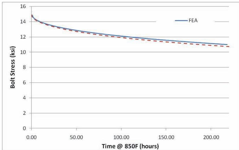
Figure 48 – NPS 2, cl. 900 Bolt Stress vs. Time
