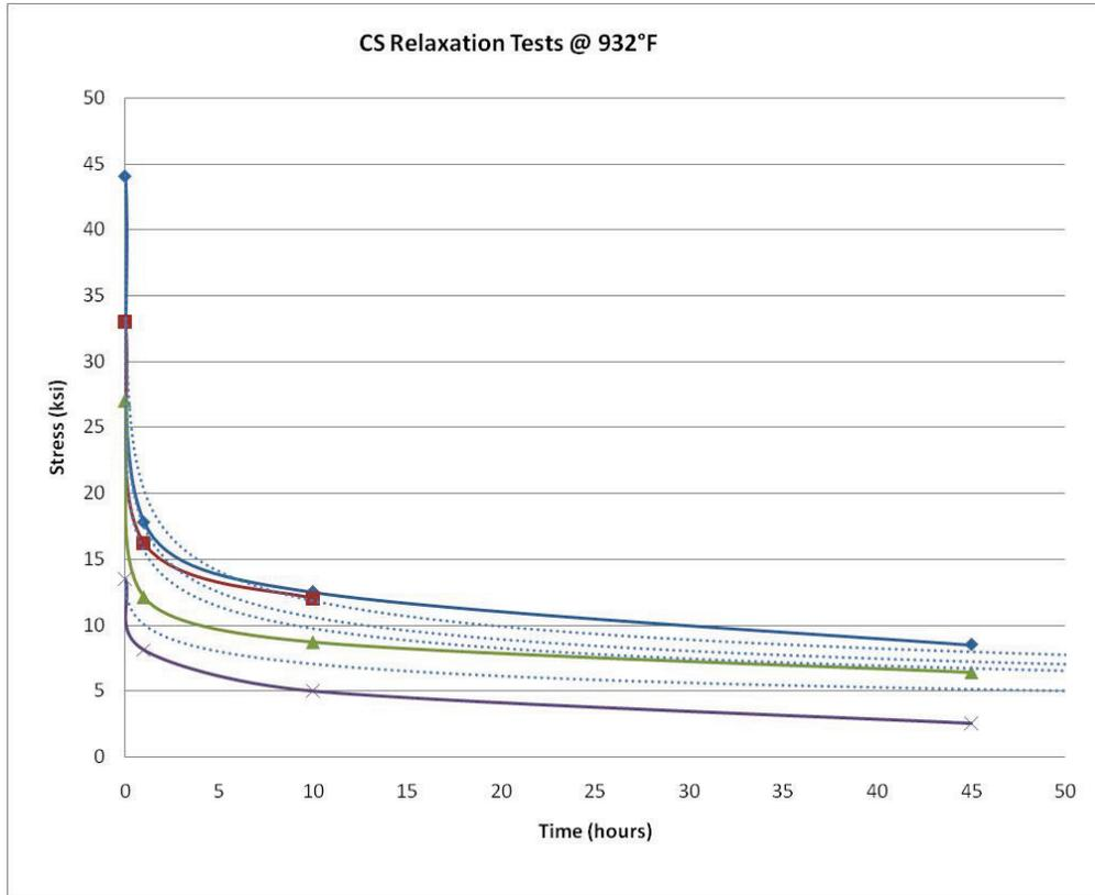
Figure 23 – Equation (1) Carbon Steel Relaxation Results at 932°F
