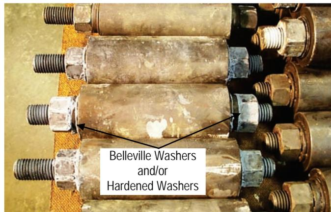
Figure 49 – Bolt Load Relaxation Arrangement
