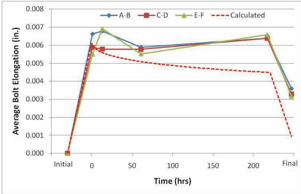
Figure 57 – NPS 2, cl.900 Bolt Deformation Results
