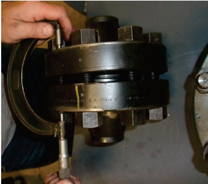
**Figure 52 – Joint Measurement Arrangement**
