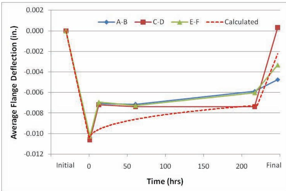
Figure 65 – NPS 3, cl.300 Flange Deformation Results
