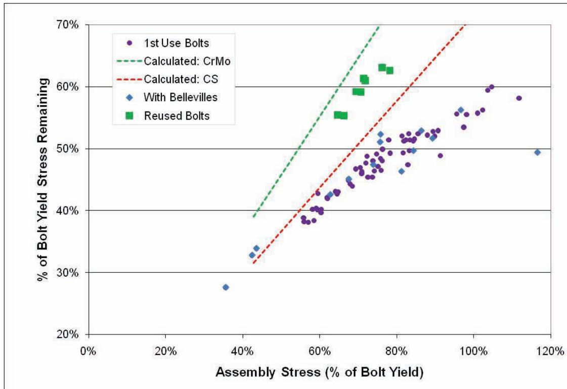
Figure 56 – Bolt Load Relaxation vs. Assembly Load (% of Ambient Bolt Yield Stress)
