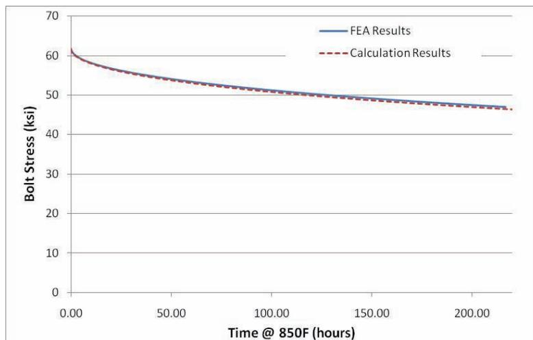
**Figure 45 – NPS 3, cl. 150 Bolt Stress vs. Time**
