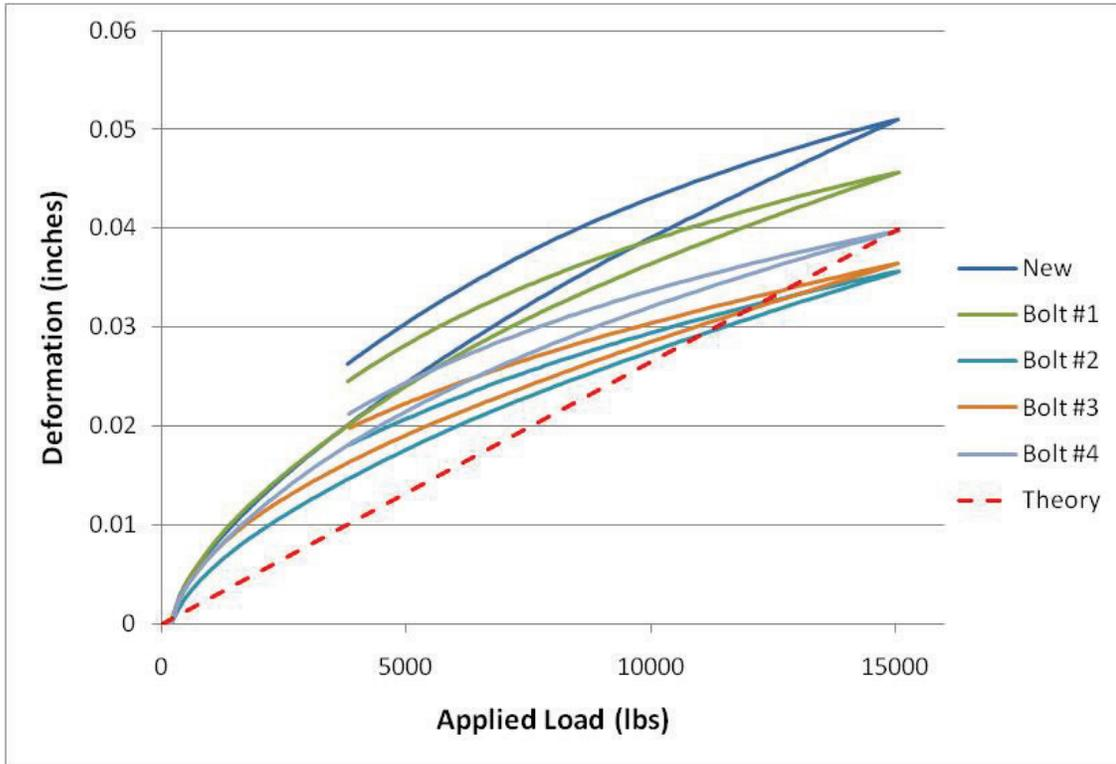
Figure 62 – 3 Belleville Washer Stack Load-Deformation Results
