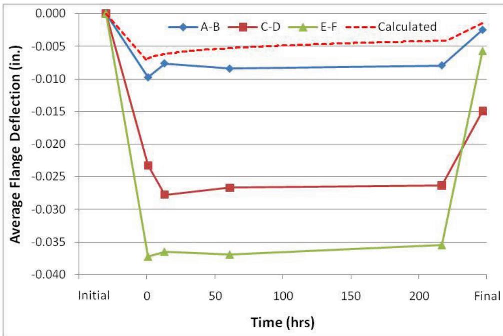
Figure 58 – NPS 2, cl.900 Flange Deformation Results
