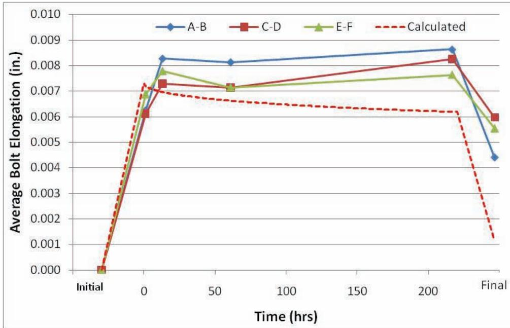
Figure 64 – NPS 3, cl.300 Bolt Deformation Results
