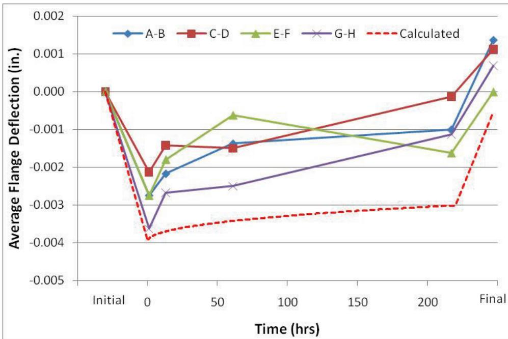
Figure 60 – NPS 3, cl.150 Flange Deformation Results
