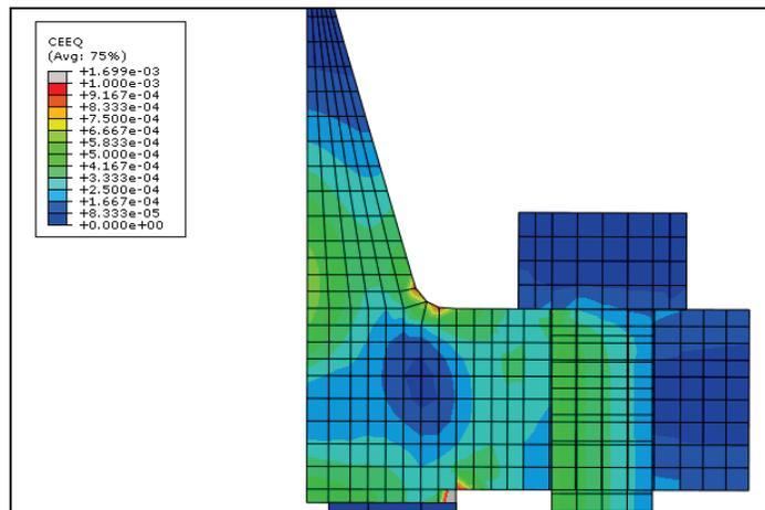
Figure 42 – NPS 3, cl. 300 Creep Strain @ 217hrs
