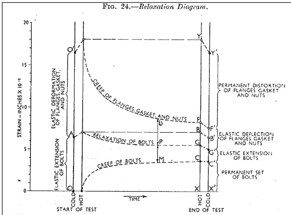
Figure 3 – Relaxation Diagram from Gough [5], Fig. 24, page 263
