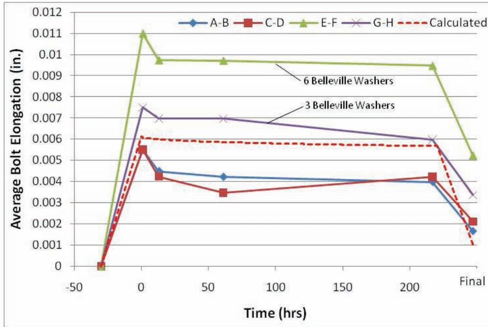
Figure 59 – NPS 3, cl.150 Bolt Deformation Results
