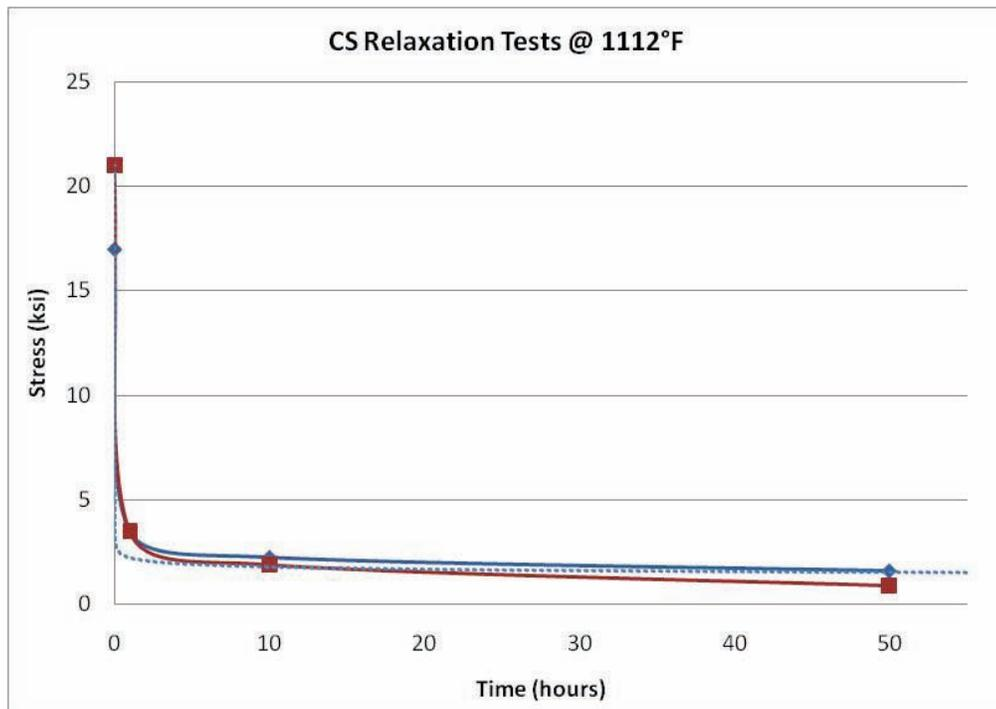
Figure 24 – Equation (1) Carbon Steel Relaxation Results at 1112°F
