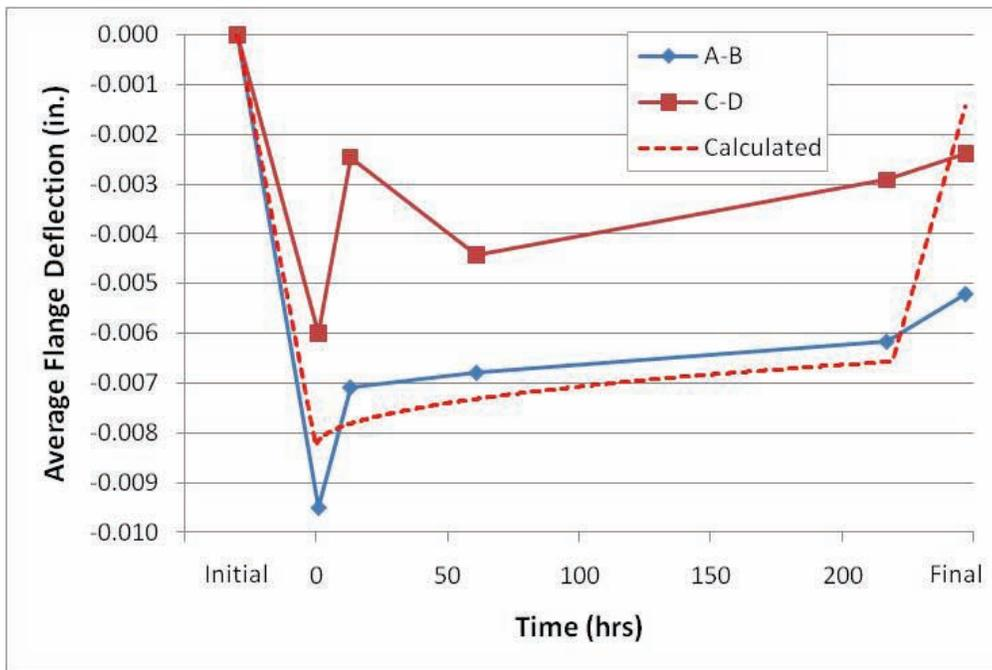
Figure 67 – NPS 6, cl.150 Flange Deformation Results
