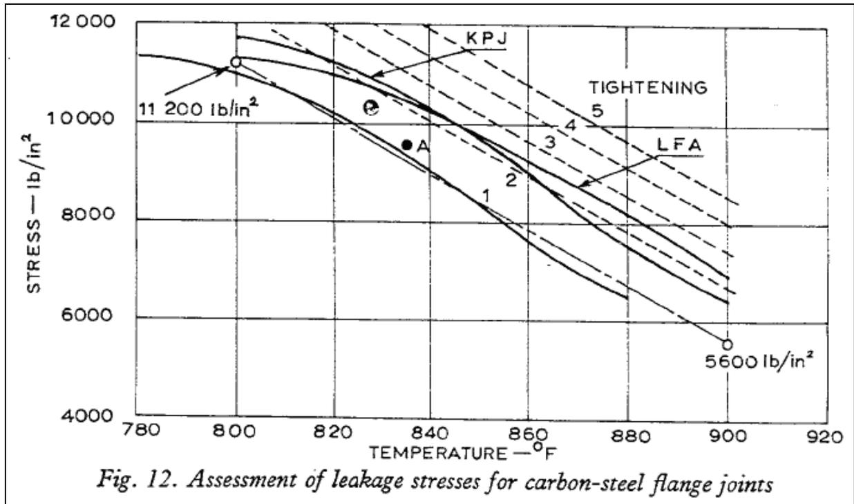
*Fig. 12. Assessment of leakage stresses for carbon-steel flange joints*
