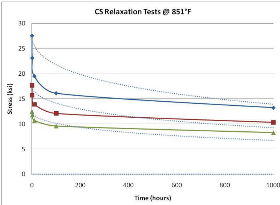
Figure 26 – Equation (1) Carbon Steel Relaxation Results at 851°F
