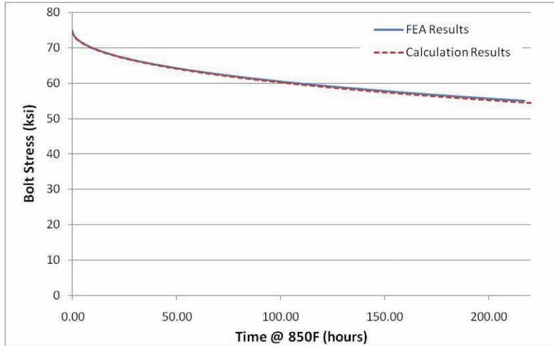
Figure 47 – NPS 6, cl. 150 Bolt Stress vs. Time
