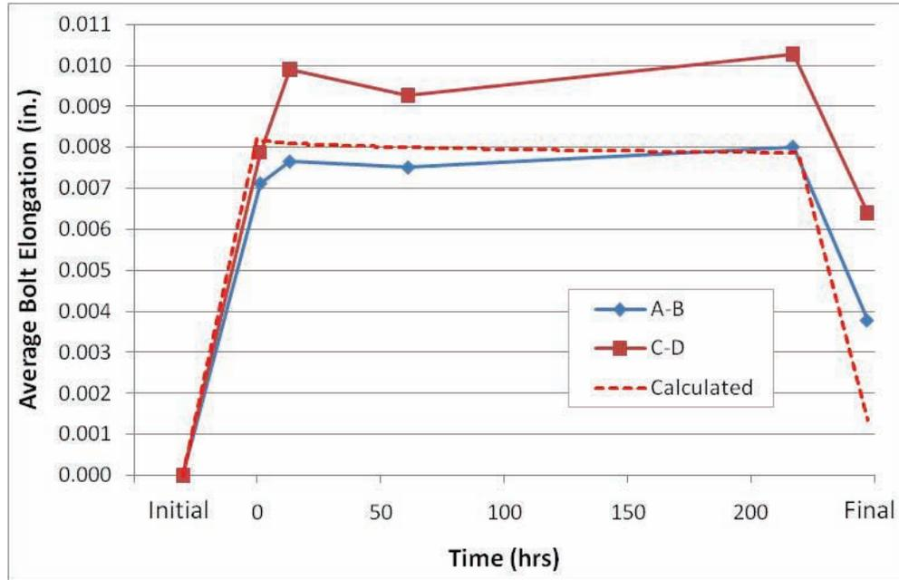
Figure 66 – NPS 6, cl.150 Bolt Deformation Results
