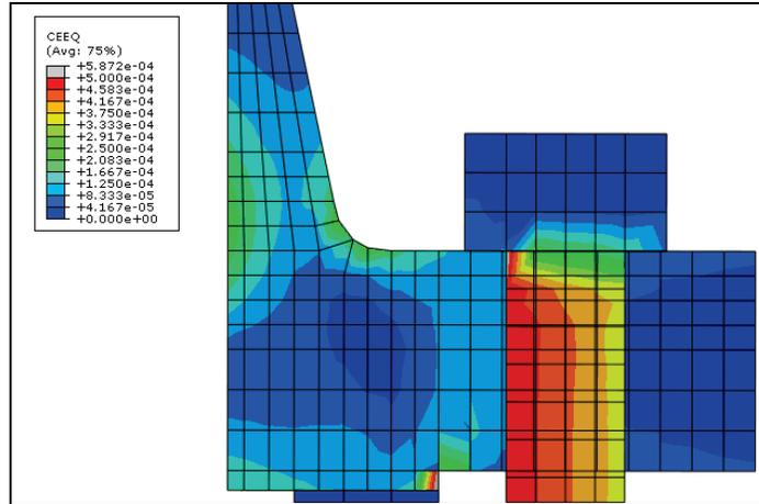
Figure 40 – NPS 3, cl. 150 Creep Strain @ 217 hrs
