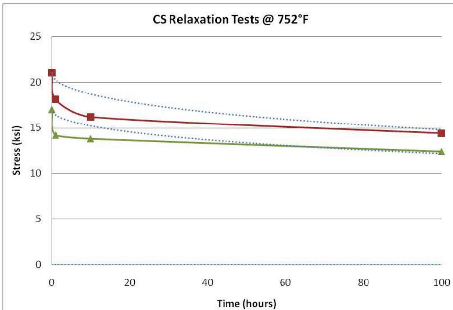
Figure 22 – Equation (1) Carbon Steel Relaxation Results at 752°F
