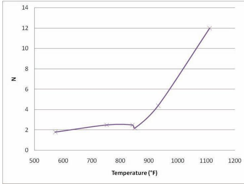
**Figure 27 – Equation (1) Carbon Steel “N” vs. Temperature**
