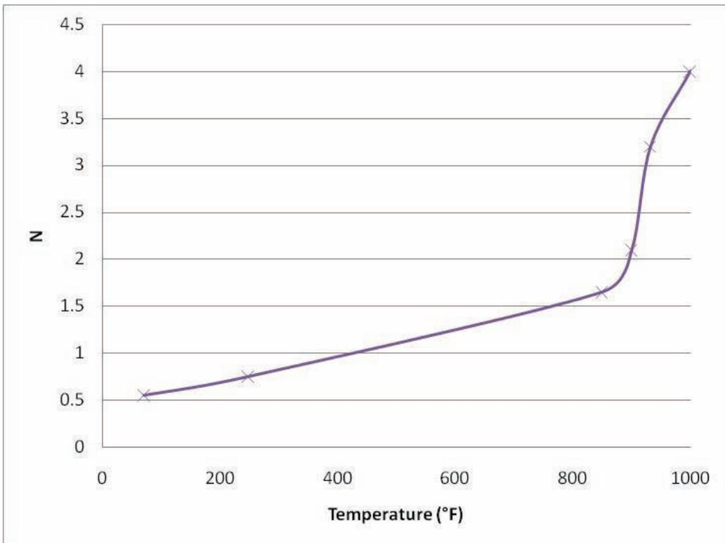
Figure 34 – Equation (1) CrMo "N" vs. Temperature
