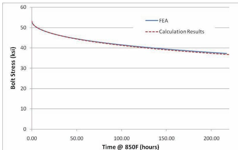
**Figure 46 – NPS 3, cl. 300 Bolt Stress vs. Time**
