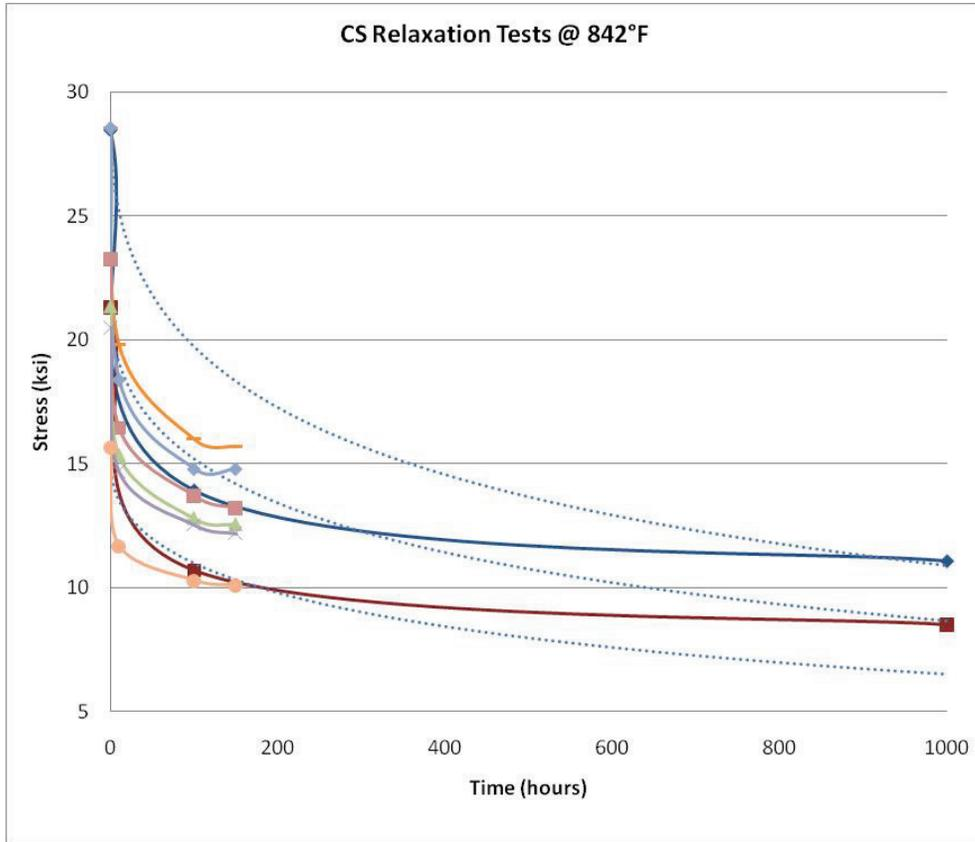
Figure 25 – Equation (1) Carbon Steel Relaxation Results at 842°F
