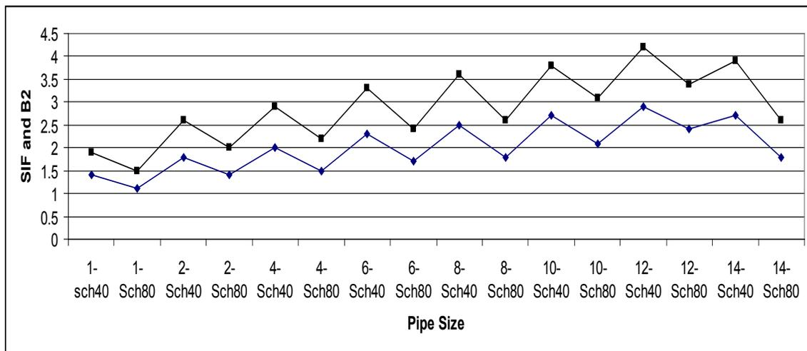
Figure 2 - SIF i (Lower Curve) and Stress Index B<sub>2</sub> for 1.5D B16.9 Elbow
