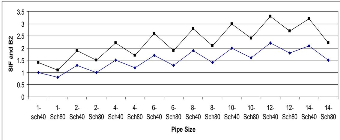
Figure 3 - SIF i (Lower Curve) and Stress Index B<sub>2</sub> for Equal Leg Tee
