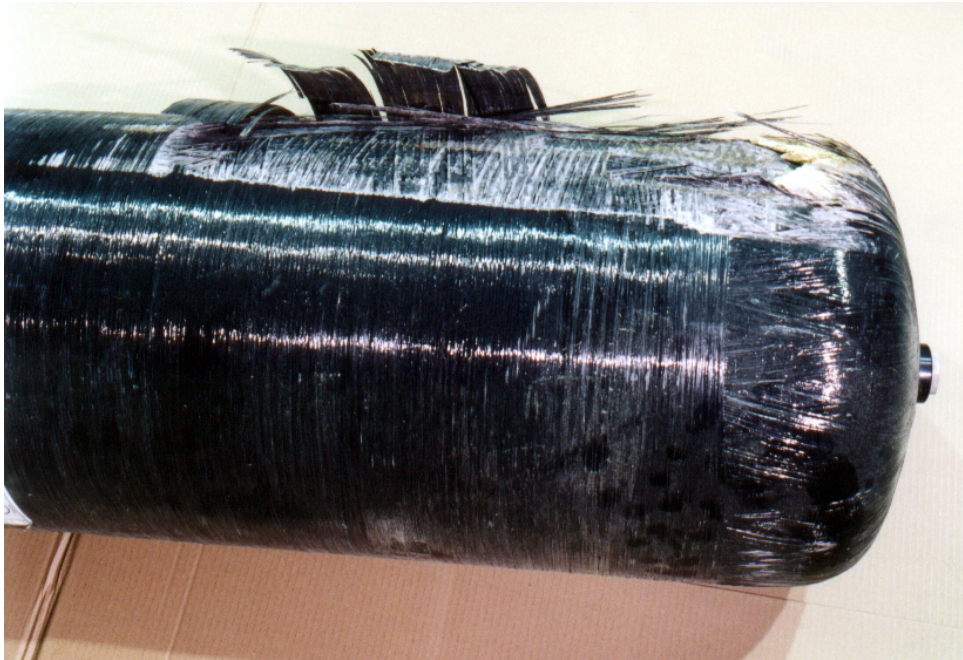
Figure 6 - All-composite fuel tank impacted by bridge (front view)
