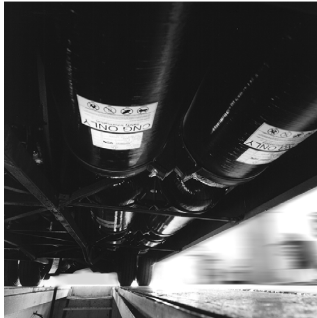
Figure 15 - All-Composite Fuel Containers that are Floor Mounted on Buses
