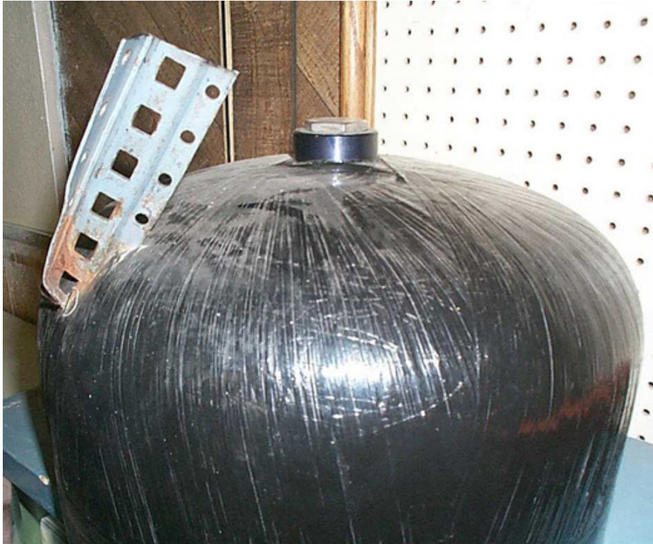
Figure 10 - All-Composite Tank with Embedded Debris
