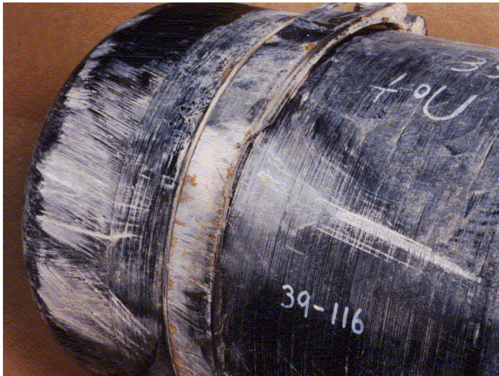
Figure 9 - All-Composite Fuel Tank Dropped from Vehicle
