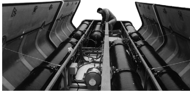
Figure 14 - All-Composite Fuel Containers that are Roof Mounted in Buses
