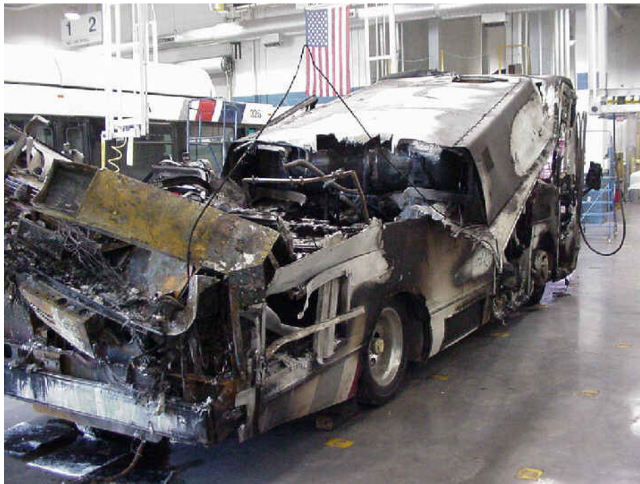
Figure 13 - NGV Bus with Fire Damage
