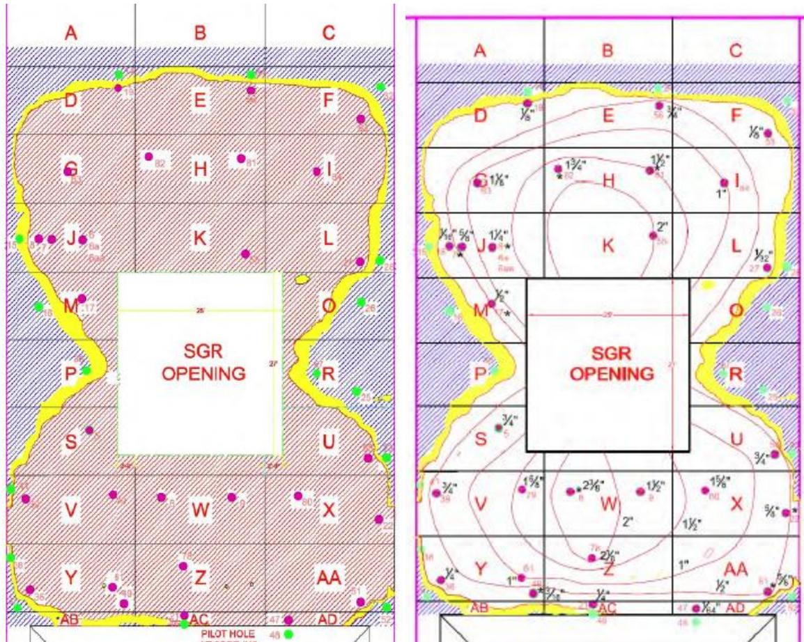
Note: Shaded blue shows non-delaminated area; yellow shows transition zone; shaded red (left) or white (right) shows delaminated area
