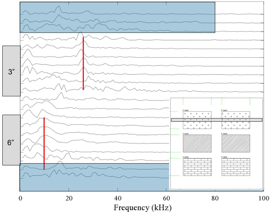
**Note: shaded areas denote boundary affected area; red lines denote characteristic frequencies for each depth; the lower right corner shows the area of the mockup tested**
