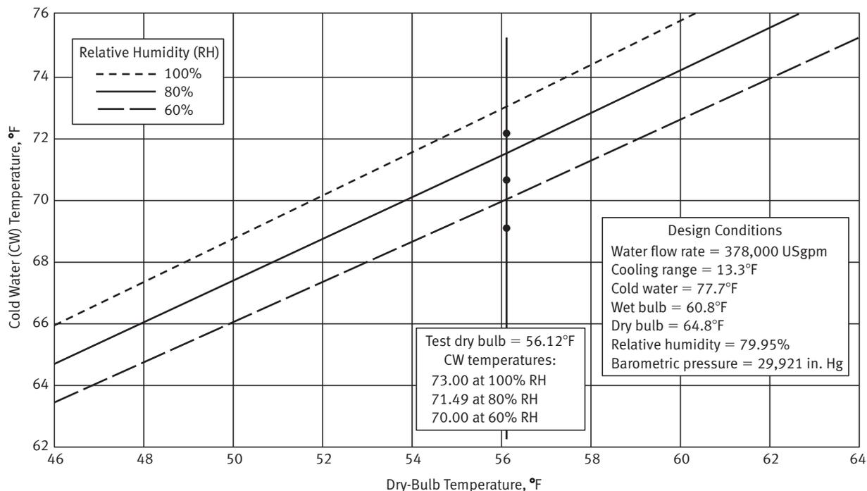
**Fig. F1-4 Cold Water Temperature Versus Dry-Bulb Temperature**
