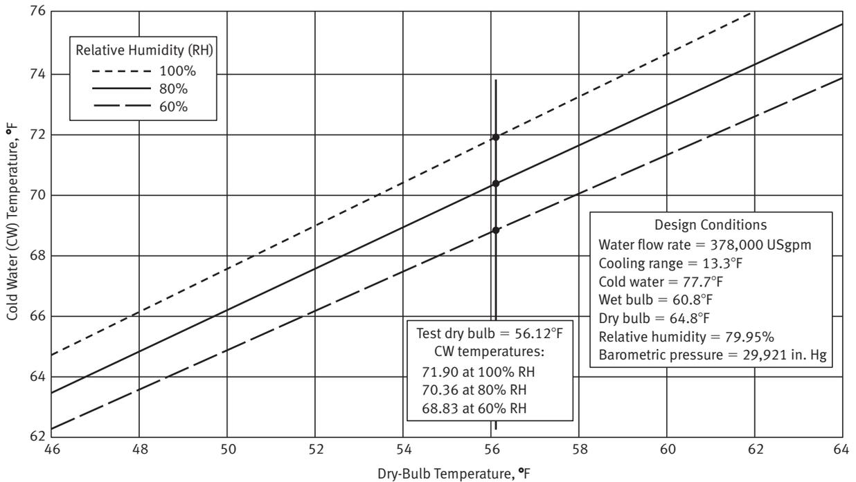
**Fig. F1-2 Cold Water Temperature Versus Dry-Bulb Temperature**
