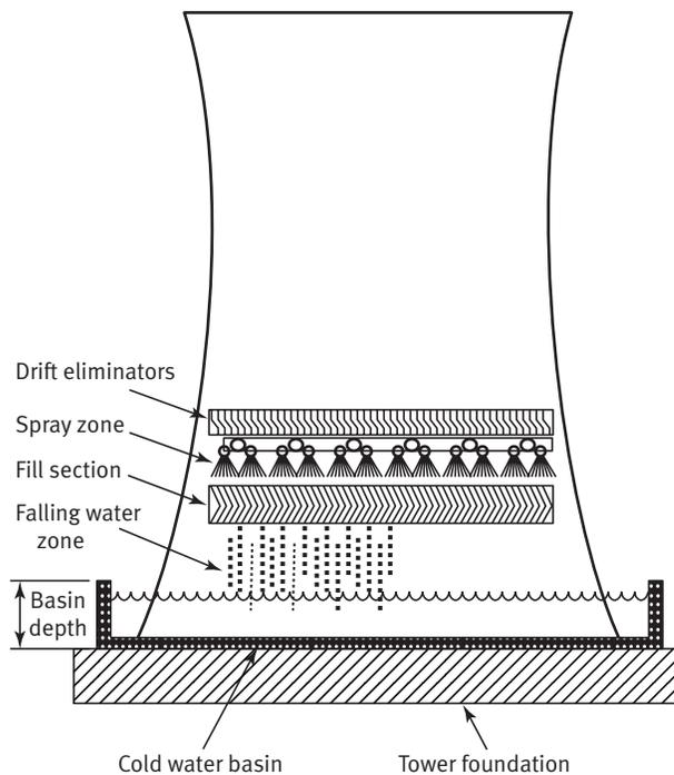
**Fig. J5 Natural Draft: Counterflow Cooling Tower**
