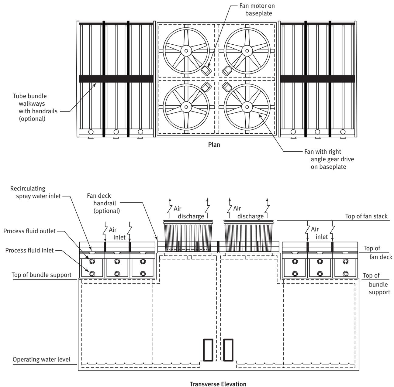
**Fig. J11 Closed-Circuit Evaporative Cooler — Parallel Flow Design**
