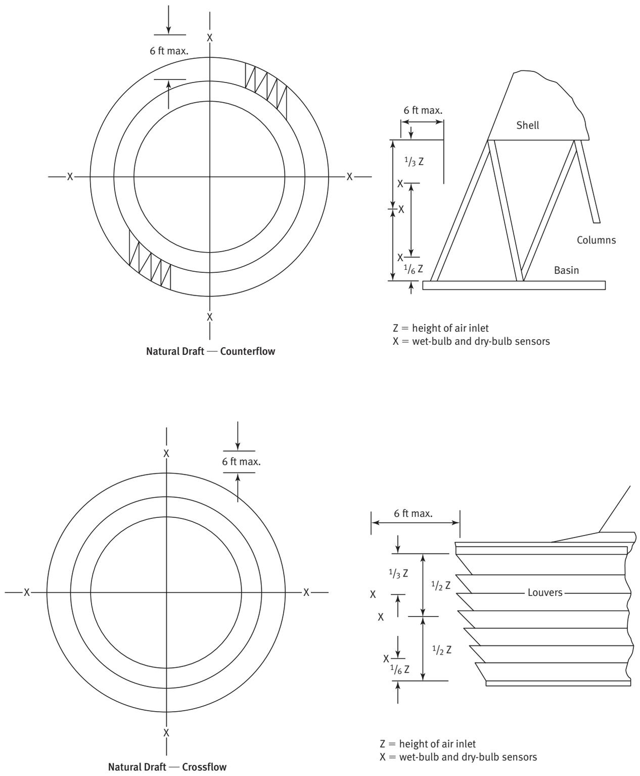
**Fig. J7 Air Temperature Sensors: Quantity and Position in Large Towers**
