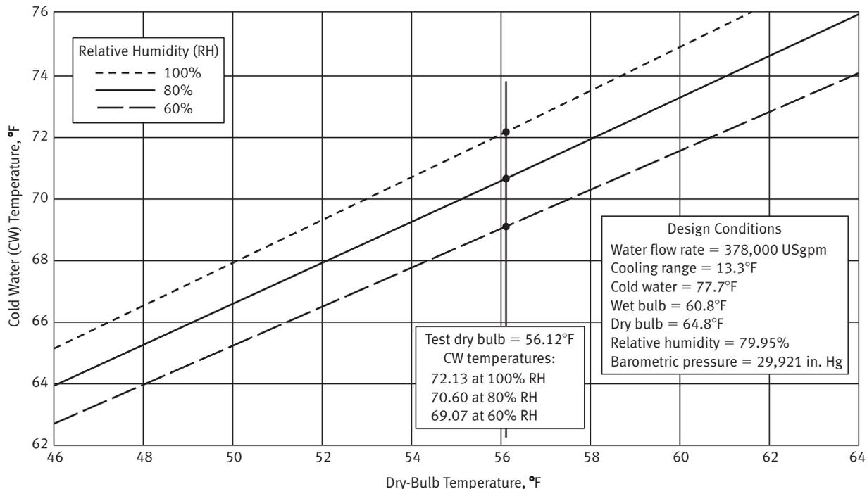
**Fig. F1-3 Cold Water Temperature Versus Dry-Bulb Temperature**
