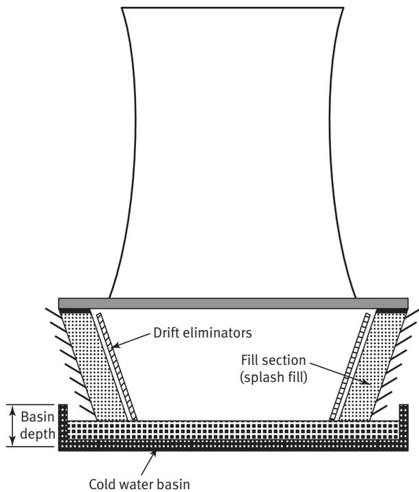
**Fig. J4 Natural Draft: Crossflow Cooling Tower**
