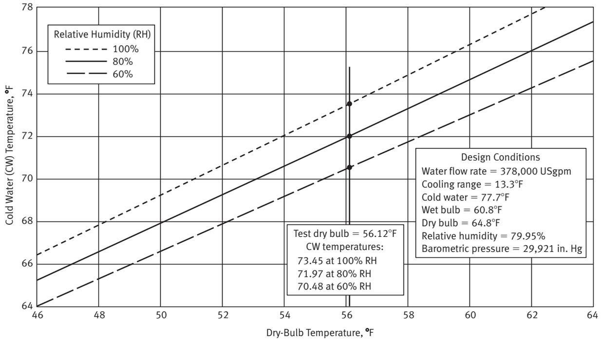
**Fig. F1-5 Cold Water Temperature Versus Dry-Bulb Temperature**
