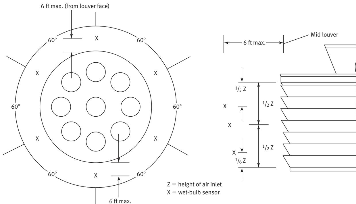
Mechanical Draft — Crossflow, Induced Draft Fans, Circular Configuration
