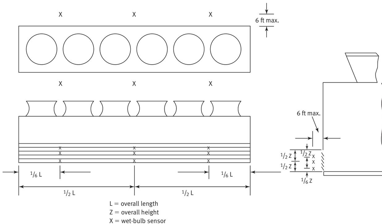
Mechanical Draft — Crossflow, Induced Draft Fans, Rectangular Configuration
