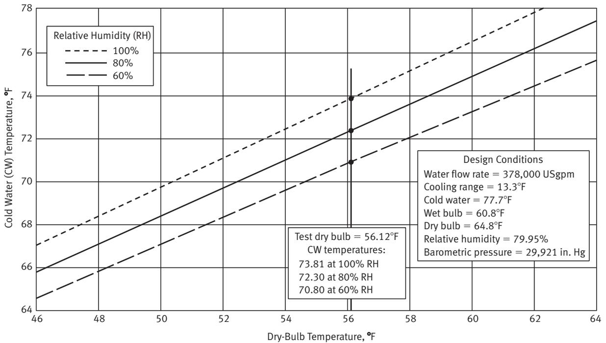
**Fig. F1-6 Cold Water Temperature Versus Dry-Bulb Temperature**
