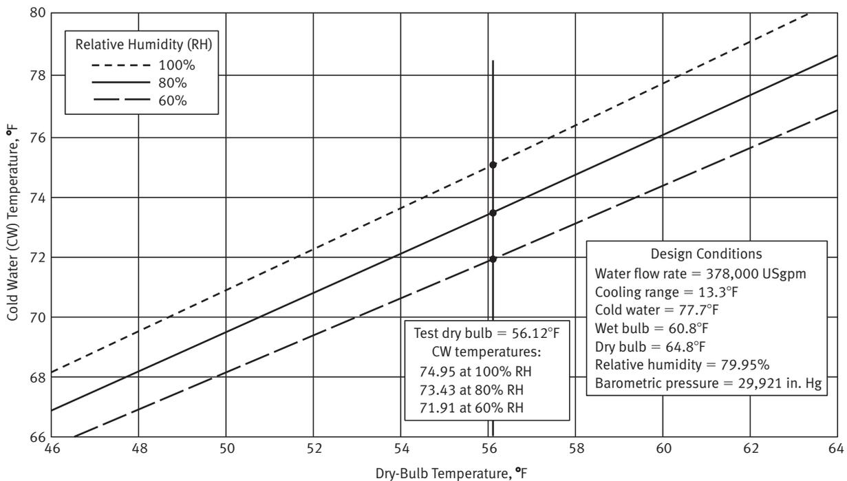
**Fig. F1-8 Cold Water Temperature Versus Dry-Bulb Temperature**
