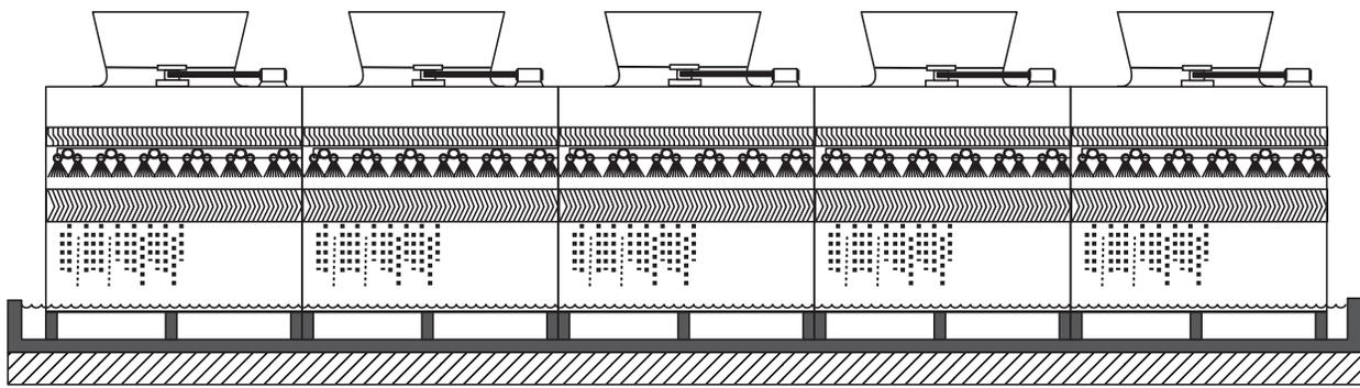
**Fig. J3 Mechanical Draft: Counterflow Cooling Tower**
