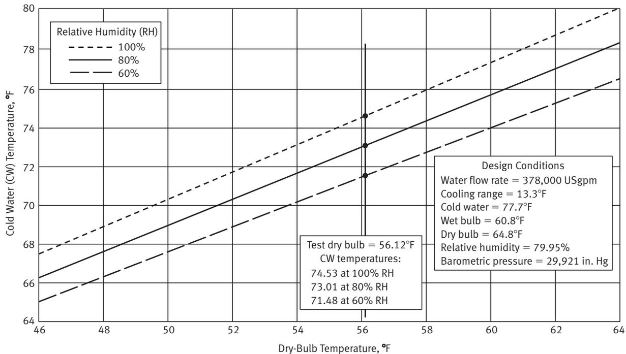
**Fig. F1-7 Cold Water Temperature Versus Dry-Bulb Temperature**
