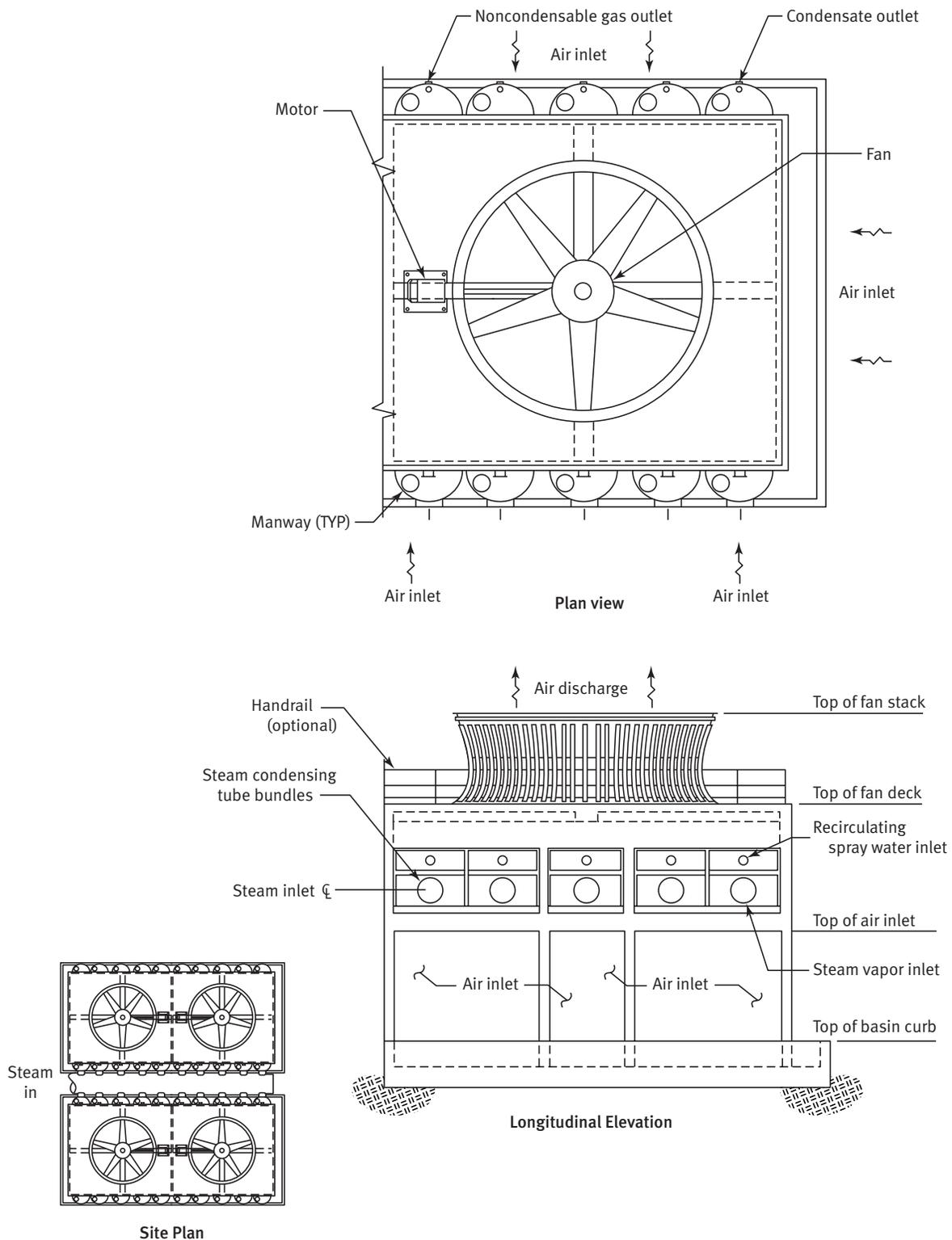
Fig. J12 Closed-Circuit Evaporative Cooler — Counterflow Design
