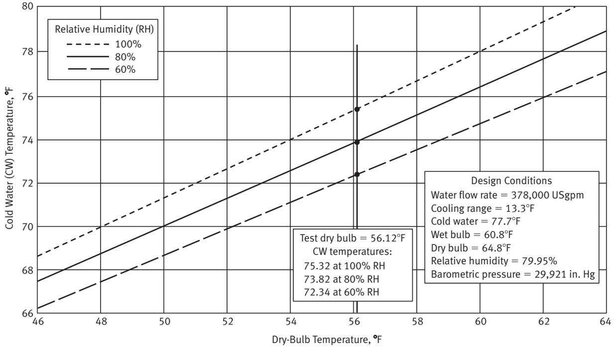
**Fig. F1-9 Cold Water Temperature Versus Dry-Bulb Temperature**
