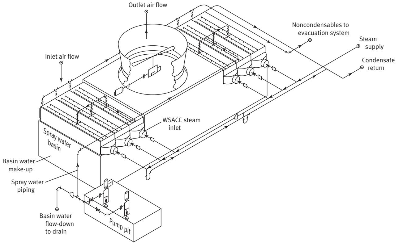
**Fig. J13 Wet Surface Air-Cooled Steam Condenser (WSACC)**
