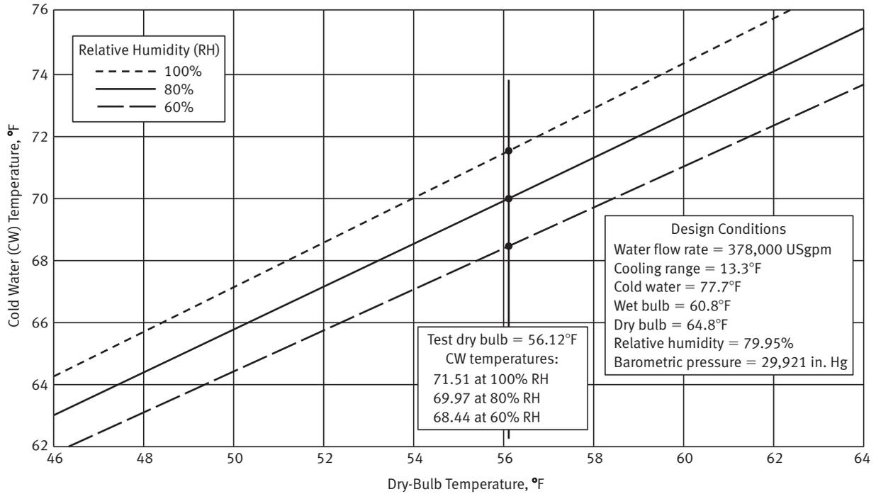
**Fig. F1-1 Cold Water Temperature Versus Dry-Bulb Temperature**
