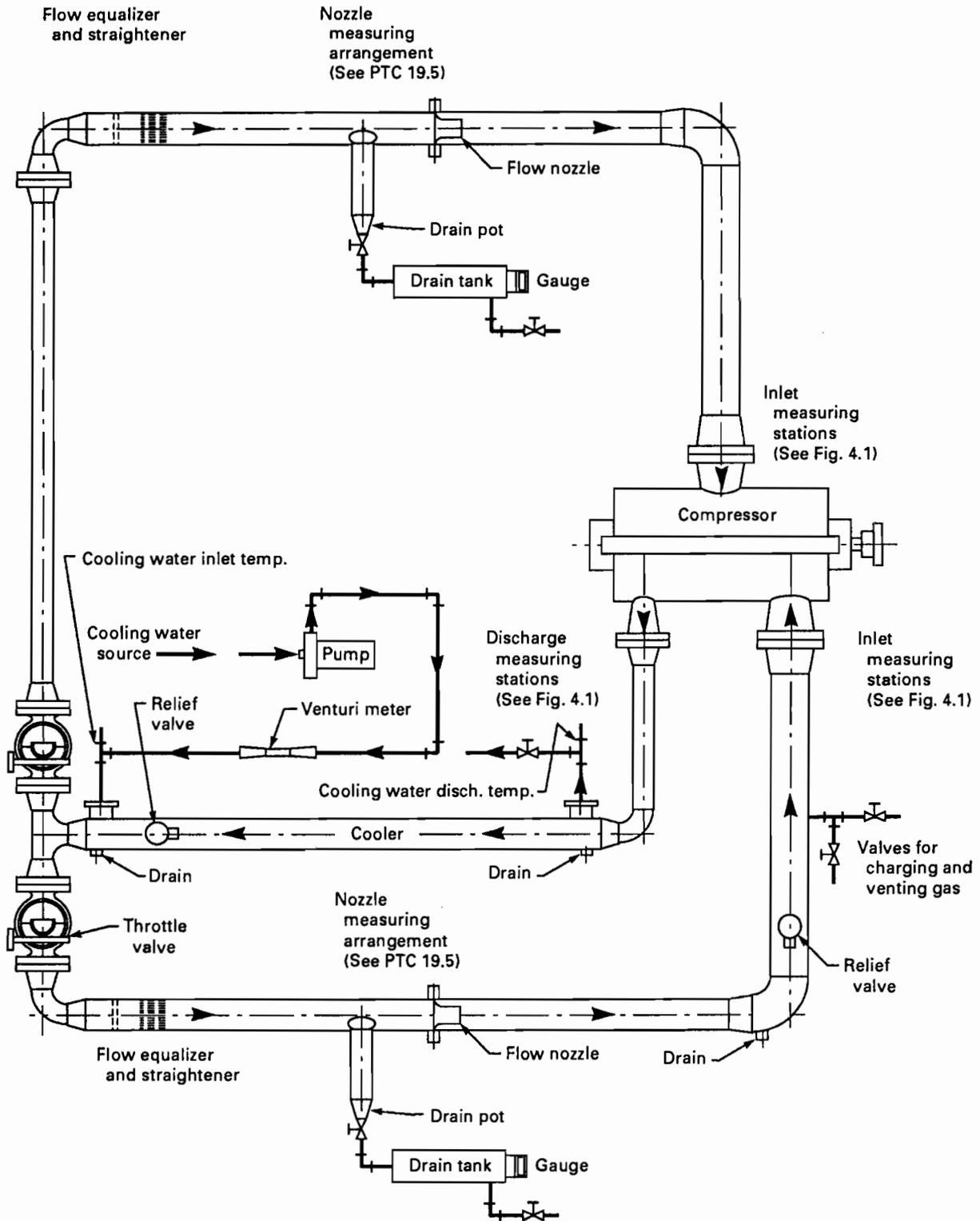
FIG. 4.7 TYPICAL CLOSED LOOP WITH SIDESTREAM
