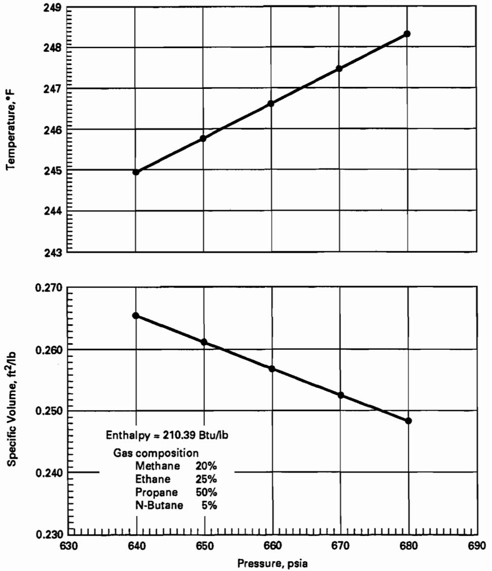
FIG. C.6.2 TEMPERATURE/SPECIFIC VOLUME vs. PRESSURE, CONSTANT ENTHALPY
