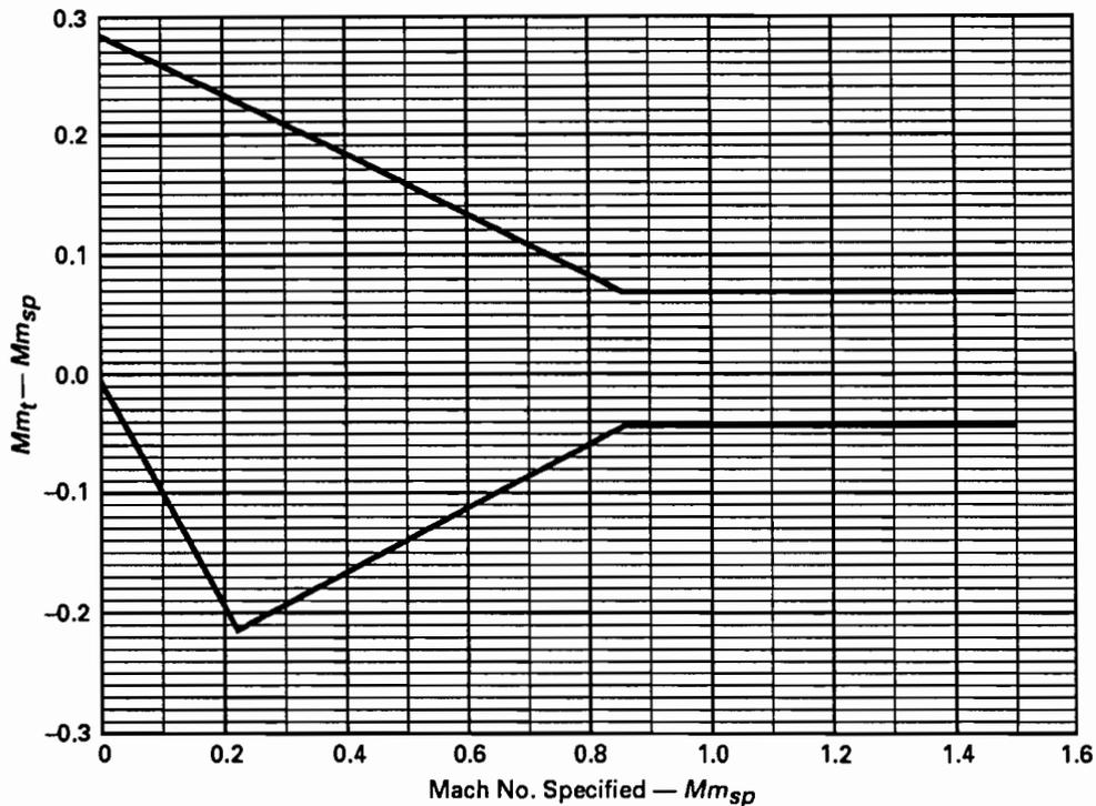
FIG. 3.3 ALLOWABLE MACHINE MACH NUMBER DEPARTURES, CENTRIFUGAL COMPRESSORS
