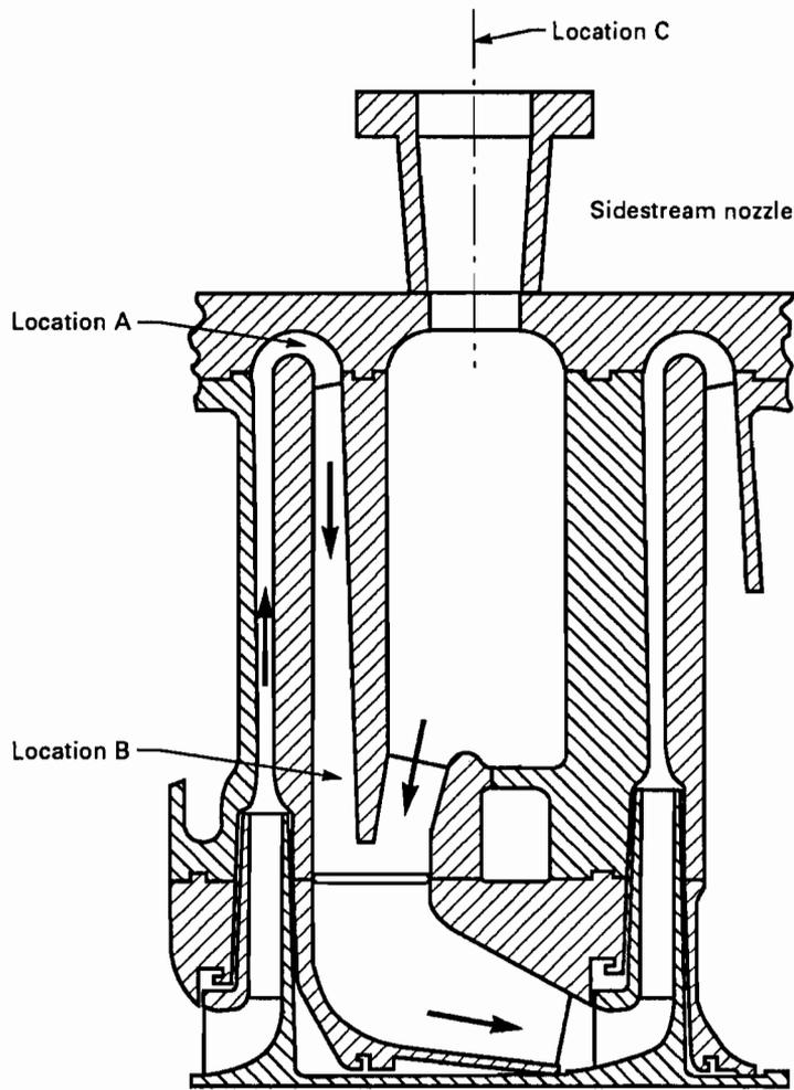
GENERAL NOTE: Mainstream instrumentation to be located between stations A and B.
