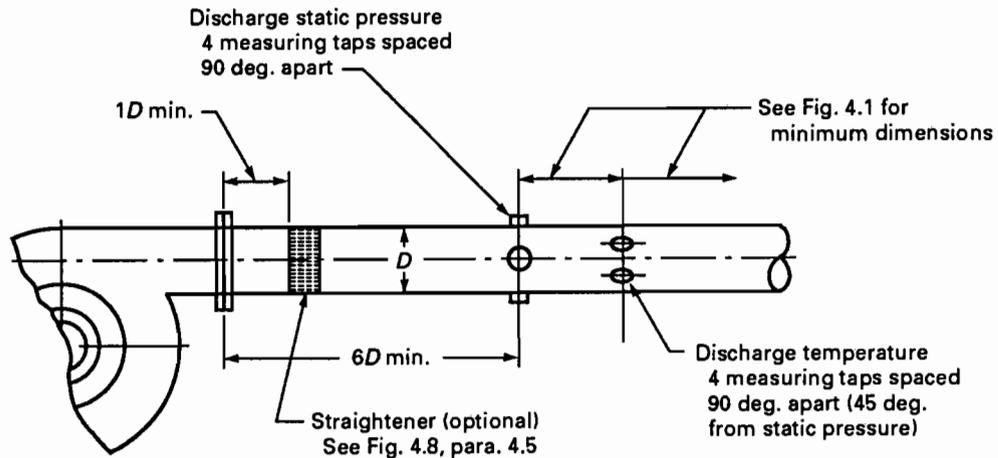
FIG. 4.5 DIFFUSING VOLUTE DISCHARGE WITH NONSYMMETRIC FLOW
