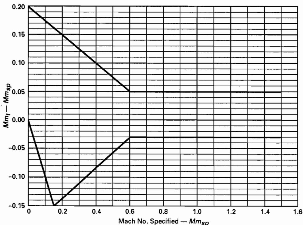
FIG. 3.4 ALLOWABLE MACHINE MACH NUMBER DEPARTURES, AXIAL COMPRESSORS
