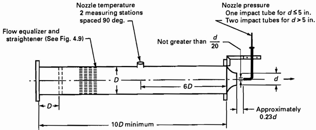
SPECIAL NOTE:  $d$  not more than  $0.6D$  for any nozzle arrangement
