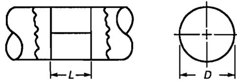
(a) Simple-Vane Flow Straightener
