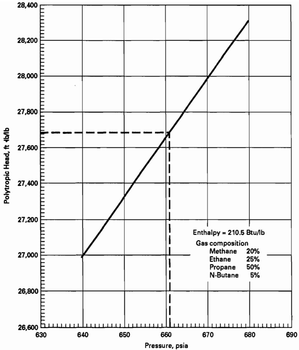
**FIG. C.6.1 POLYTROPIC HEAD vs. PRESSURE,
