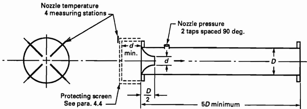
FIG. 4.9 INLET NOZZLE ON AN OPEN LOOP
