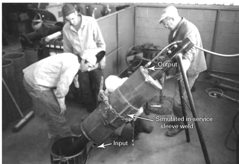
Fig. I-1 Procedure and Welder Qualification Test Assembly for an In-Service Fillet Weld
