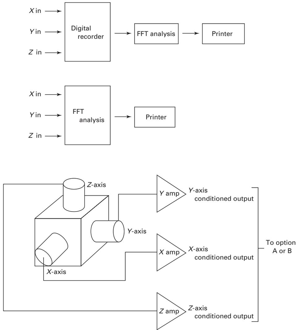
**Fig. C-1 Diagram of Sensor Arrangement and Instrumentation Configuration**
