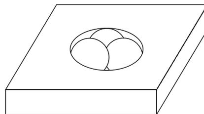
**Fig. G-2 Three-Sphere Kinematic Seat**
