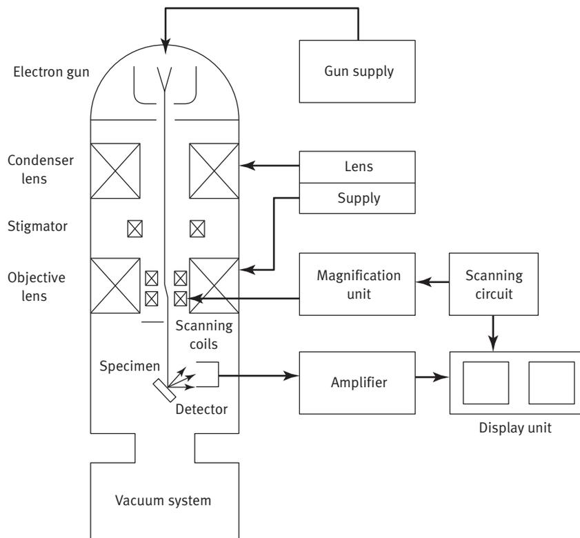
the specimen surface. A schematic diagram of an SEM is shown in Fig. C-9. Similarly, as stated above, Fig. C-9 is only a basic schematic of the principal components of an SEM and should not be interpreted as inclusive of all SEM designs. A number of different lens designs and electron sources are possible.
