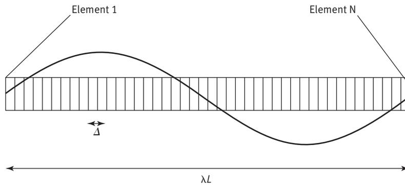
**Fig. 8-3 Demonstration of the Detector Array With Element Spacing  $\Delta$  and the Measurement of the Smallest Spatial Wavelength,  $\lambda R$  Covering Five Pixels**
