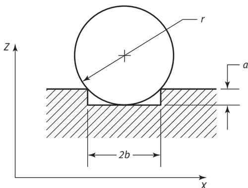
**7-4.2.5 The Maximum Stylus Tip Radius,  $r_{\max}$ , for Grooves.** When measuring a narrow negative step, a groove, it may be necessary to choose a small stylus tip radius and small cone angle to ensure that the tip contacts the bottom of the groove (See Fig. 7-2). If the groove depth is small enough that the groove shoulders contact only the spherical tip and not the cone flank, the maximum tip radius  $r$  that will reach the bottom of the groove is as follows:
