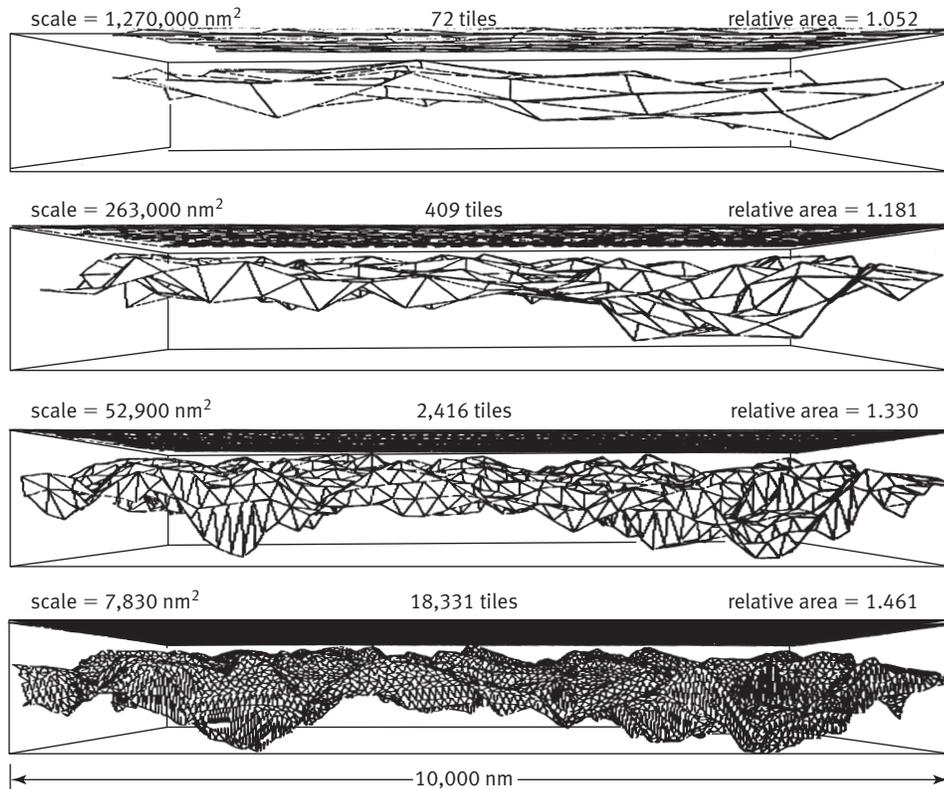
GENERAL NOTE: The triangular tiles, or patches, are shown in outline. The total area measured by the tiles increases as the scale of observation (tile area) decreases. The nominal areas covered by each tiling exercise are represented on the ceiling of each box. The measured area can be calculated as the scale times the number of tiles. Note that there is some distortion of the tiles in the display. In each tiling exercise the tiles all have the same area, which is the scale.
