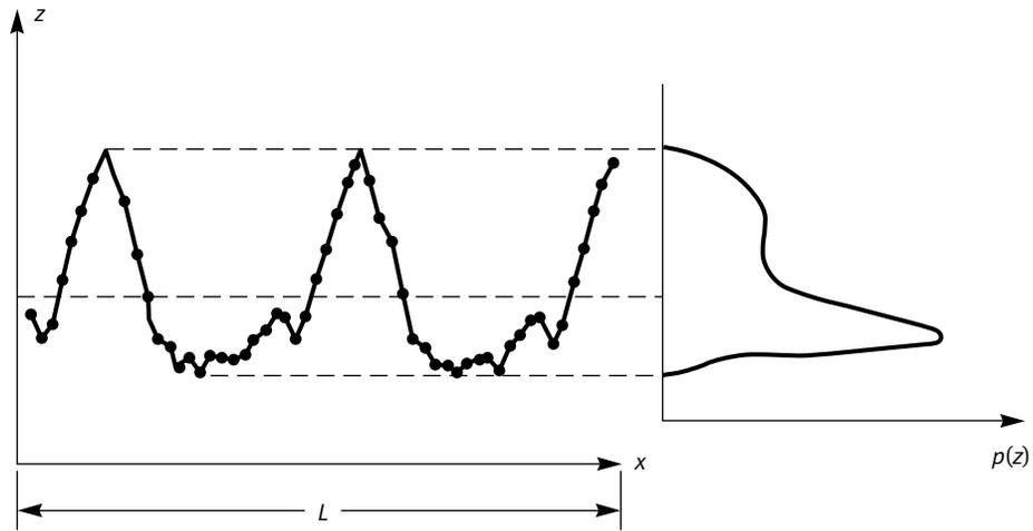
**Fig. 1-16 The Profile Bearing Length**
