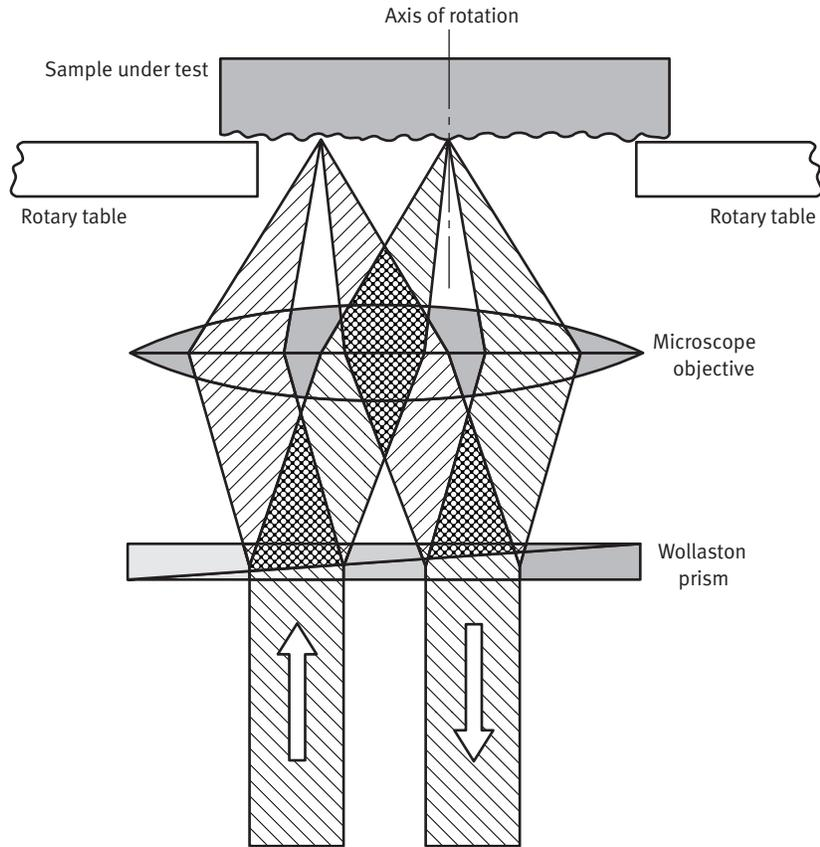
**Fig. C-4 Multiple Beam Interferometer**
