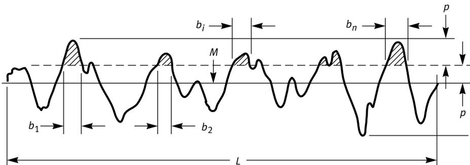
**Fig. 1-17 The Bearing Area Curve and Related Parameters**
