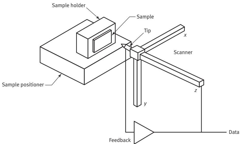
**Fig. E-5 Schematic Diagram of an Atomic Force Microscope With an Optical Lever Sensor**
