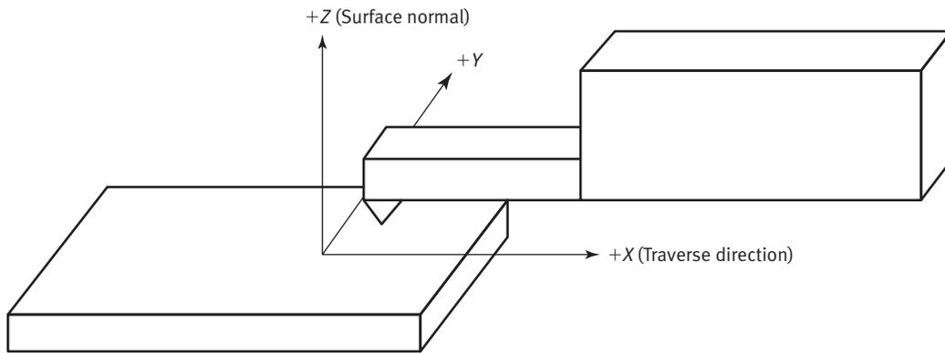
**Fig. 3-2 Conical Stylus Tip**
