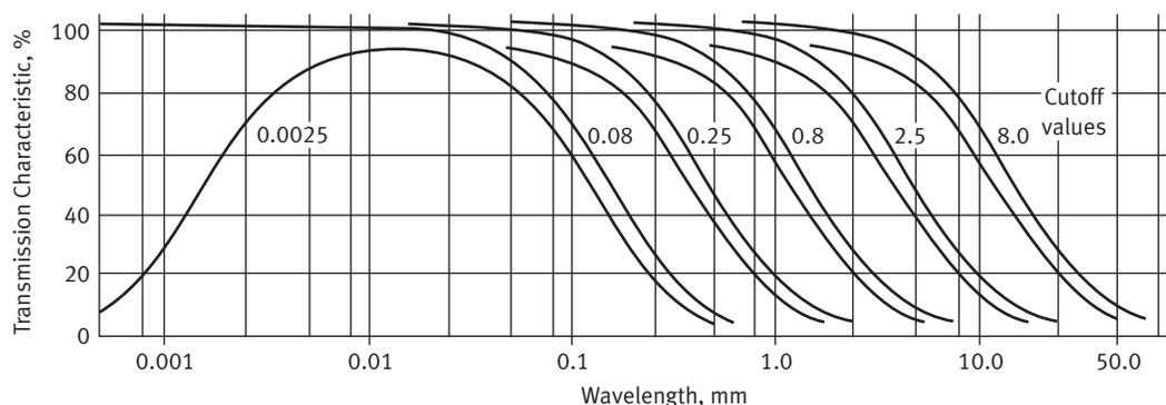
GENERAL NOTE: The double curve for each cutoff is to address the tolerances associated with a given 2RC filter implementation.
