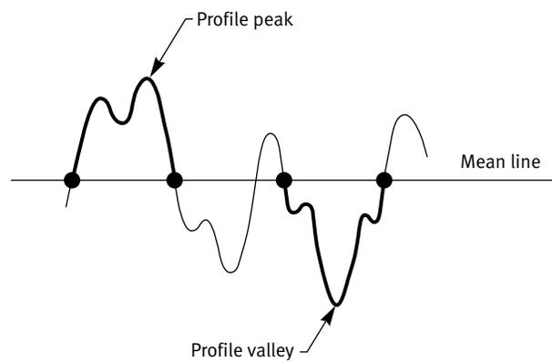
Fig. 1-7 Surface Profile Measurement Lengths
