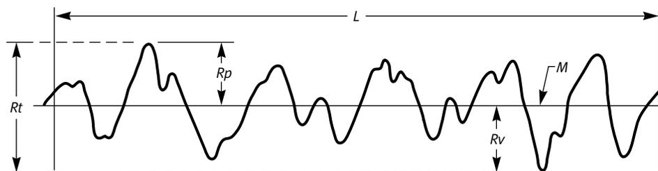
Fig. 1-10 Surface Profile Containing Two Sampling Lengths,  $l_1$  and  $l_2$ , Also Showing the  $R_{p_i}$  and  $R_{t_i}$  Parameters
