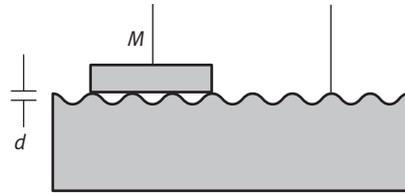
Fig. F-2 Principle of Capacitance Between Parallel Plates
