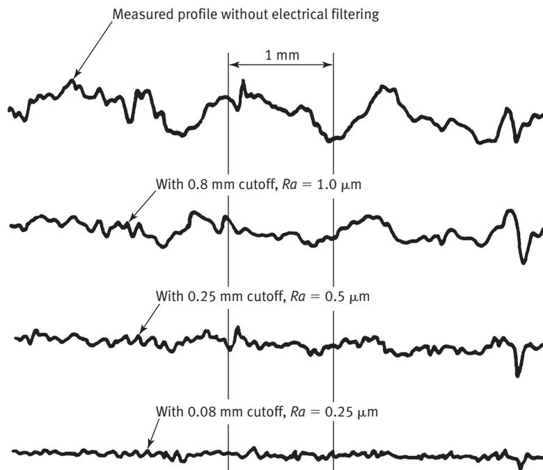
GENERAL NOTE: Profiles have unequal vertical and horizontal magnifications.
