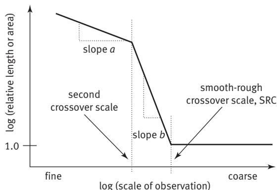
GENERAL NOTE: The crossover scales are scales where there is a change in slope, indicating a change in fractal dimension. In this case the second crossover scale indicates a change to a lower complexity at finer scales ( $-\text{slope } a < -\text{slope } b$ ).
