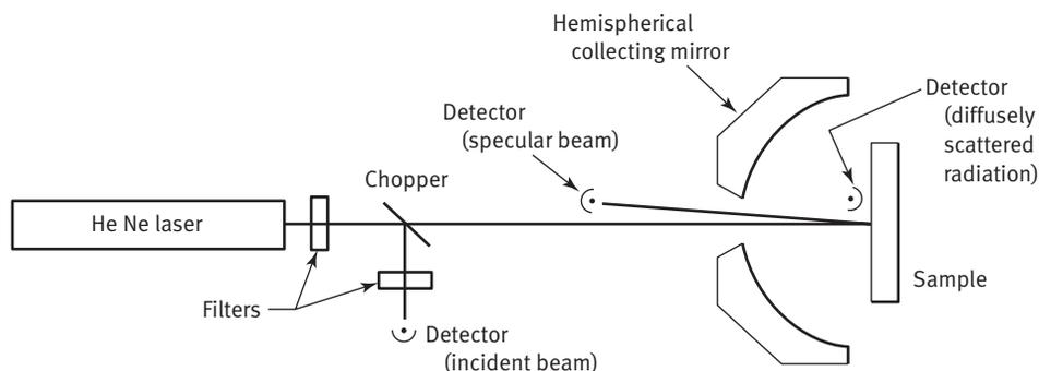
As is generally the case with roughness measuring instruments, the  $Rq$  value measured by TIS is a bandwidth limited quantity [see para. F-4(e)]. That is, it measures roughness over a limited range of spatial wavelengths. For TIS, the shortest measurable spatial wavelengths are approximately equal to the wavelength of light. The longest measurable spatial wavelengths are determined by either the illumination spot size or the angular aperture defining the specular beam.
