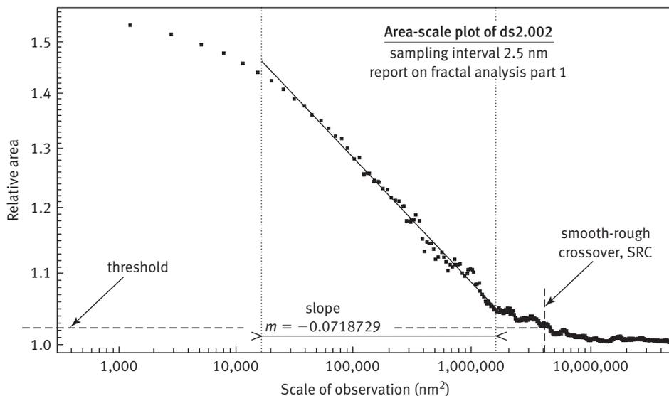
GENERAL NOTE: The smooth-rough crossover is about  $3 \times 10^6$  nm<sup>2</sup>, for a threshold in relative area of 1.02. The area-scale fractal complexity,  $Asfc = -1000$  (slope), is about 71.87 and the area-scale fractal dimension,  $Das = 2 - 2$  (slope), is about 2.144. This plot also serves as an example of a standard report of a geometric property versus scale, in which the comments in italics are optional.
