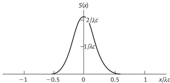
listed in para. 9-3.1. The roughness long-wavelength cutoff  $\lambda c$  is the wavelength of the sinusoidal profile for which 75% of the amplitude is transmitted by the profile filter.
