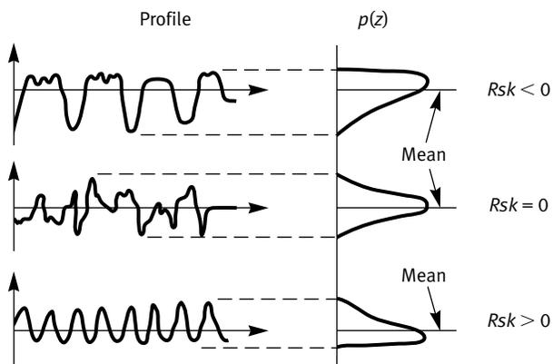
GENERAL NOTE: Three surfaces with different skewness. Also shown are the amplitude density functions (histograms) of surface height.
