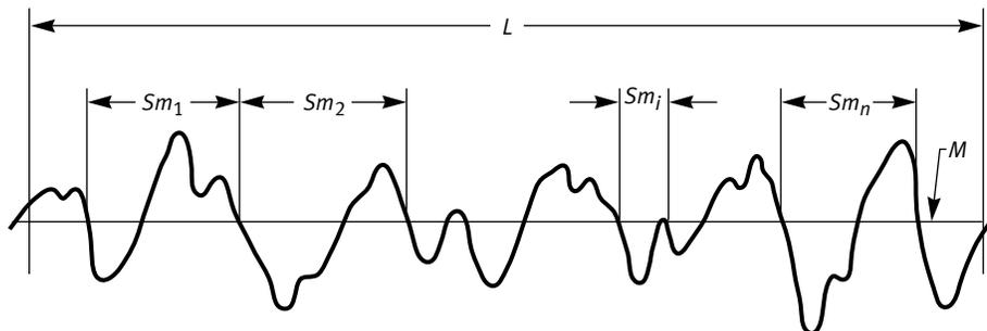
**Fig. 1-14 The Peak Count Level, Used for Calculating Peak Density**
