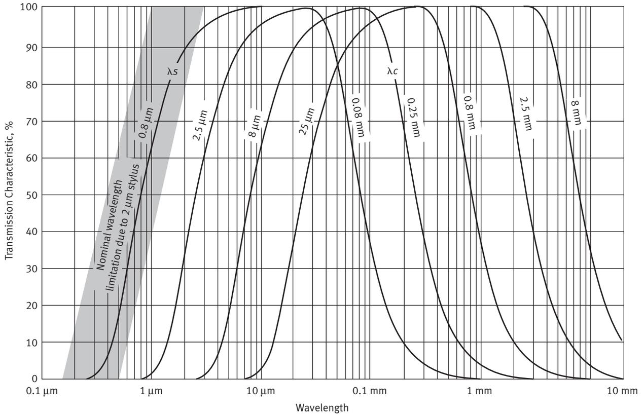
**Fig. 9-3 Weighting Function of the Gaussian Profile Filter**
