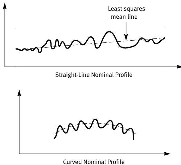
**Fig. 1-5 Filtering a Surface Profile**
