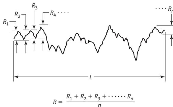
**Fig. D-2 Average Spacing of Roughness Peaks**
