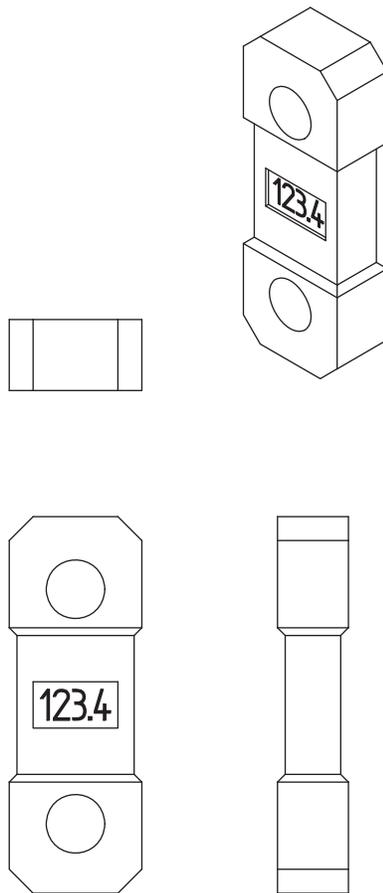
**Fig. 26-6.1.1-3 Shackle With Load-Indicating Pin**
