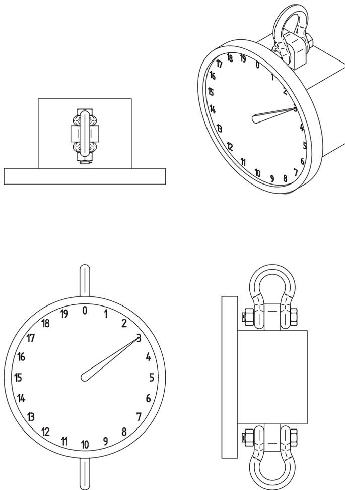
**Fig. 26-6.1.1-2 Link Style Load-Indicating Device**
