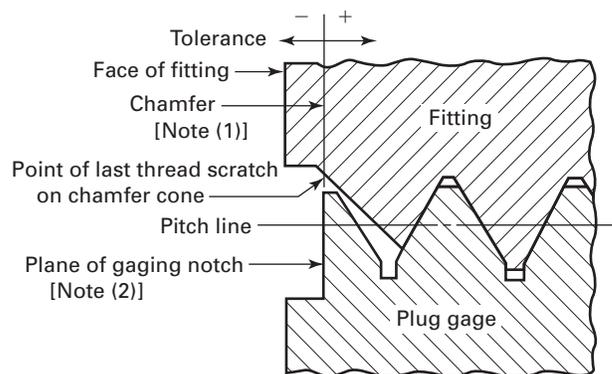
GENERAL NOTE: Enlarged view showing chamfered internal thread of basic size with chamfer exceeding the major diameter.
