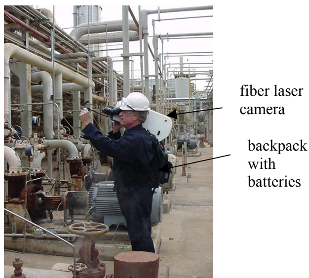
Figure ES 4-3. Scanning Refinery Components with Fiber Laser
