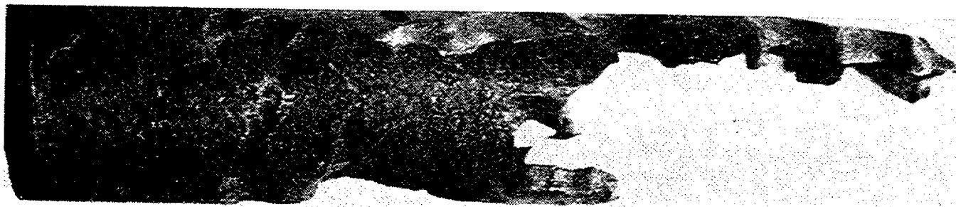
Figure 90—Severely corroded equalizer tube from gas-lift valve.
