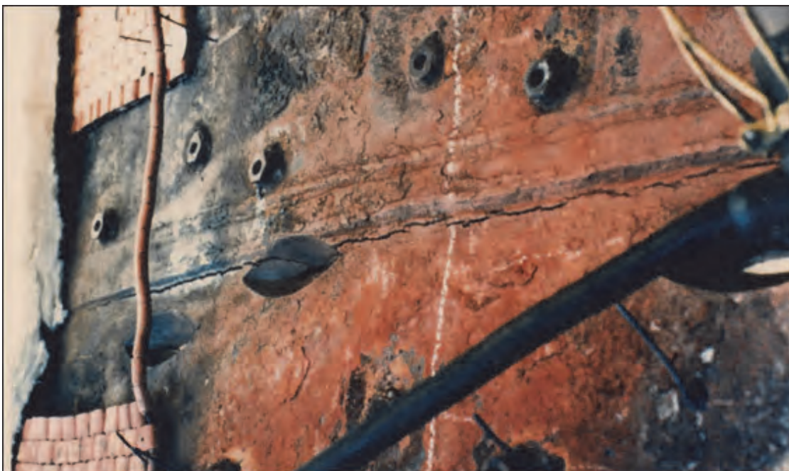
Figure 6—Typical Cracking Observed at Skirt-to-Bottom Head Weld
