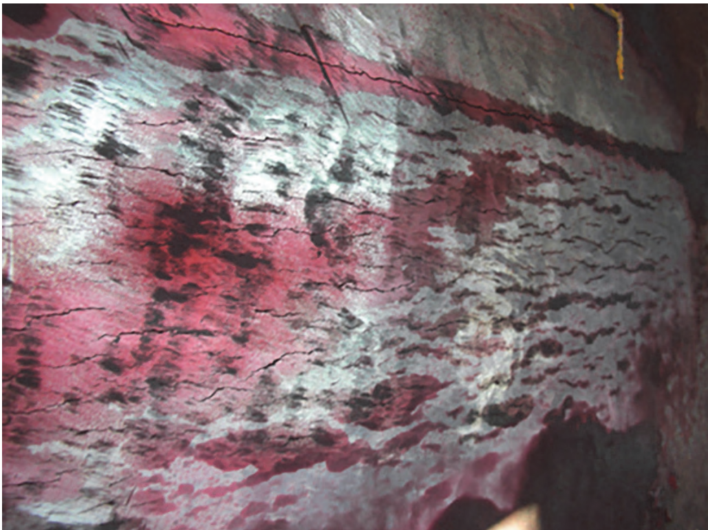
Figure 9b—External Surface Bulge Cracks
