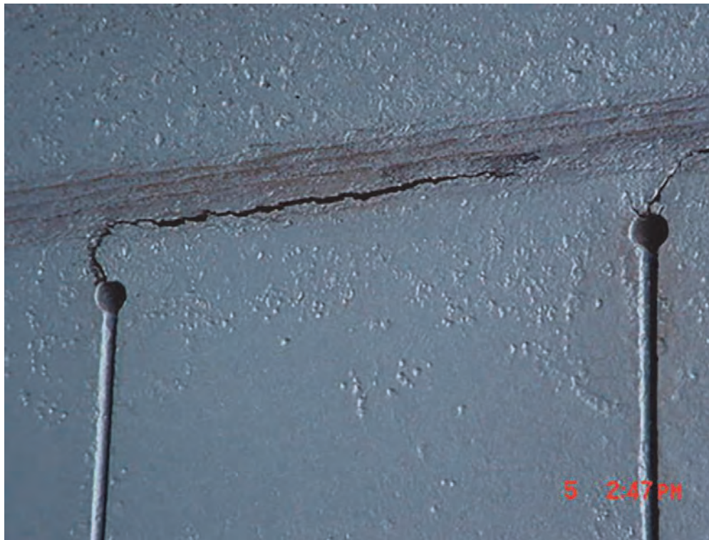
Figure 7—Keyhole Skirt-to-Bottom Head Weld Cracks
