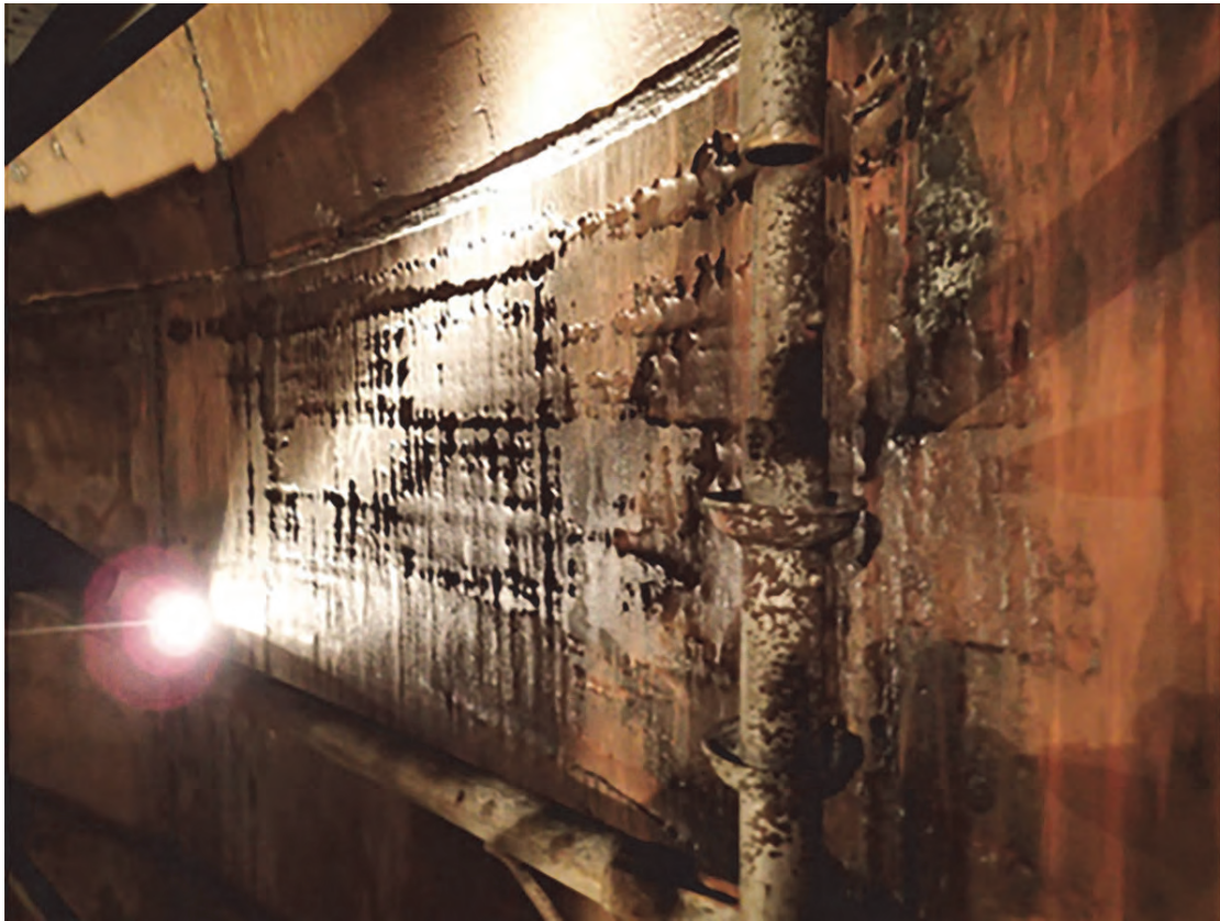
Figure 11—Corrosion of 12Cr Cladding in a Coke Drum Upper Section
