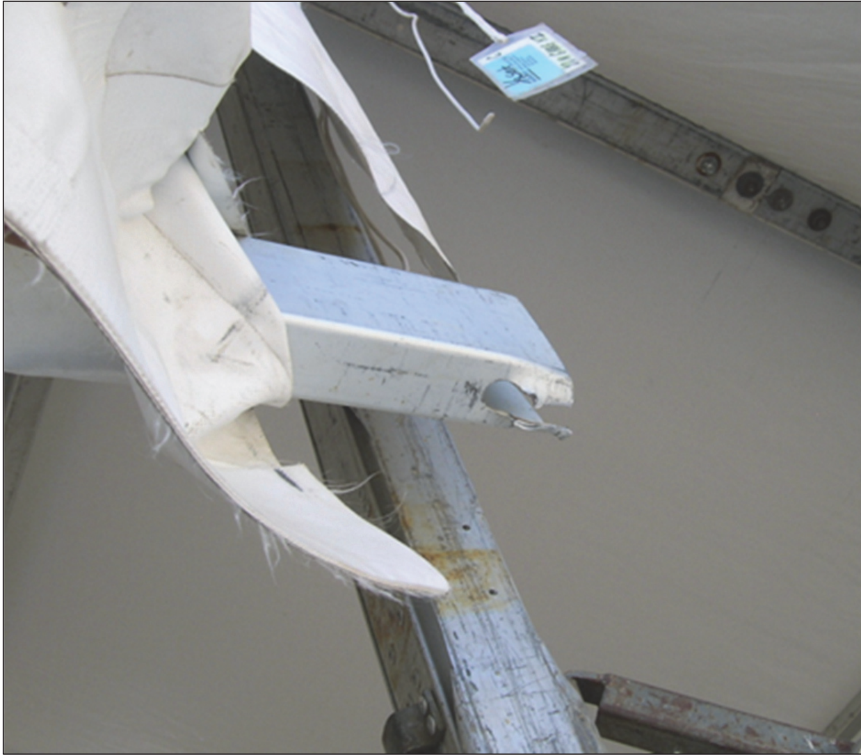
Figure 70. Detail of Failed Horizontal Member – Test C01
