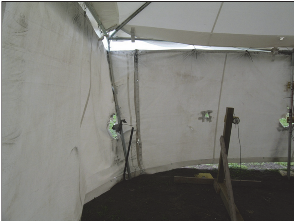
Figure 37. Bent Frame on Light Frame Tent Post Test B06
