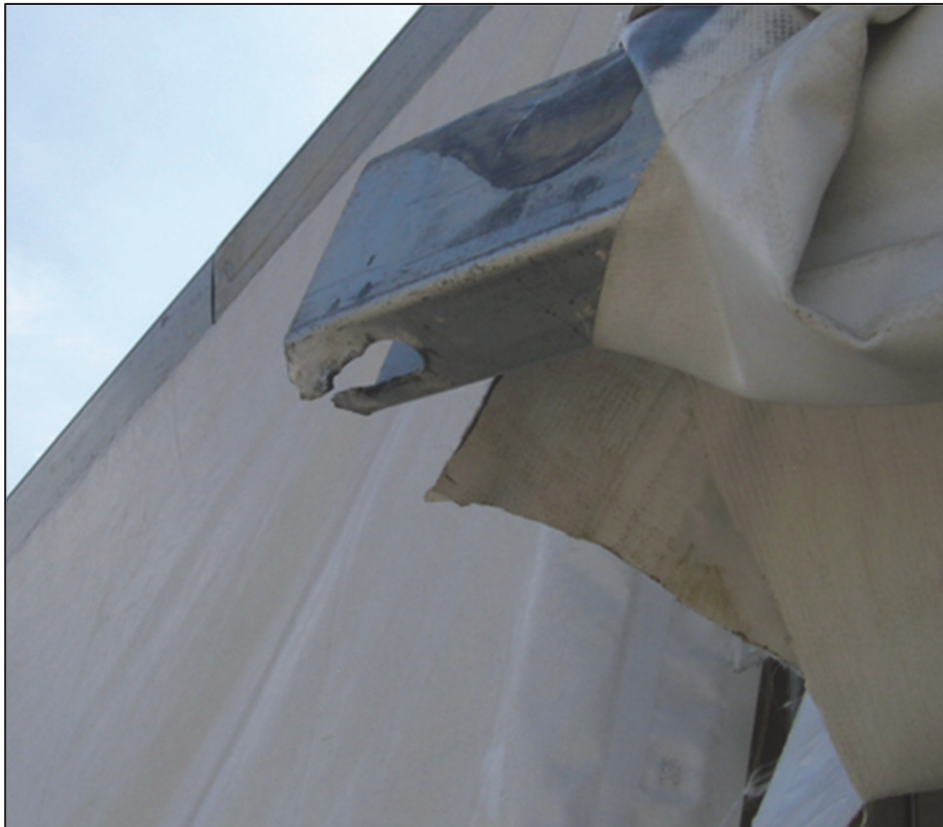
Figure 69. Failed Bolted Connection of Framed Tent – Test C01
