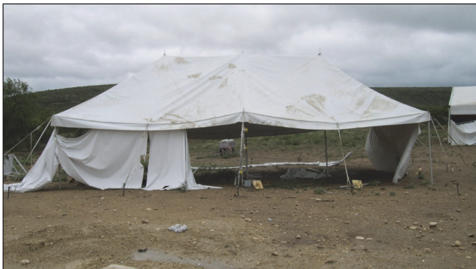
Figure 75. Damage to Pole Tent – Test C02
