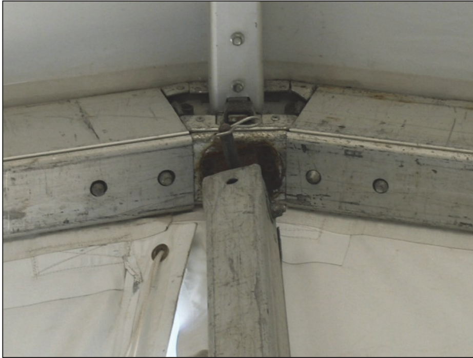
Figure 68. Damage to Framing Joint – Test C01
