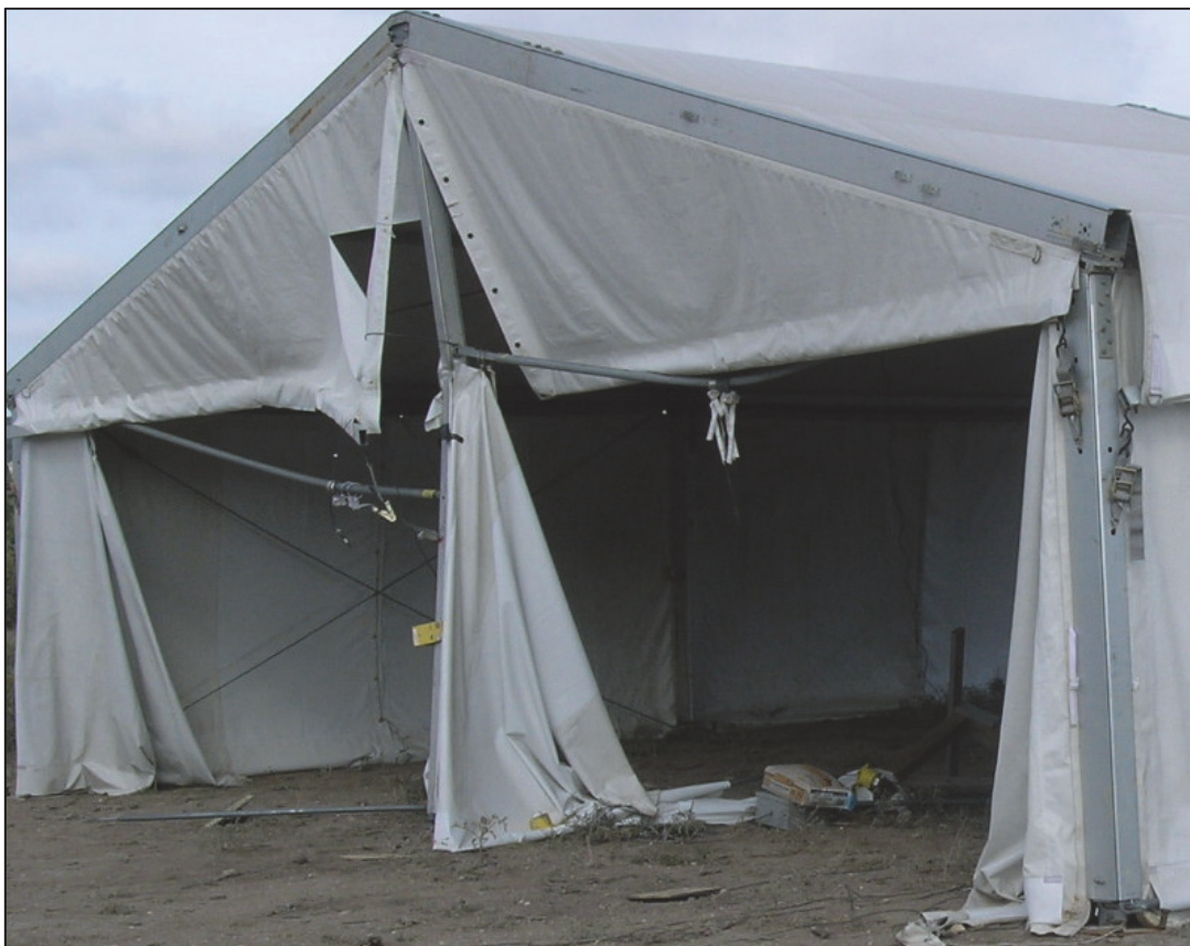
Figure 66. Damage to Front of Framed Tent – Test C01
