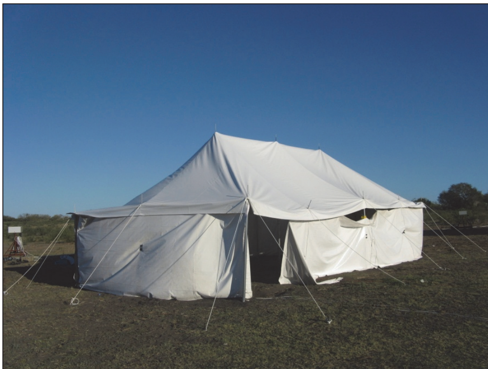
Figure 13. Damage to Non-Wind Rated Pole Tent with Sides, Test A03
