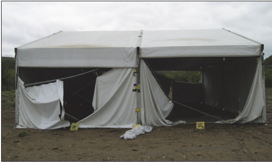
Figure 78. Damage to Side of Framed Tent – Test C2
