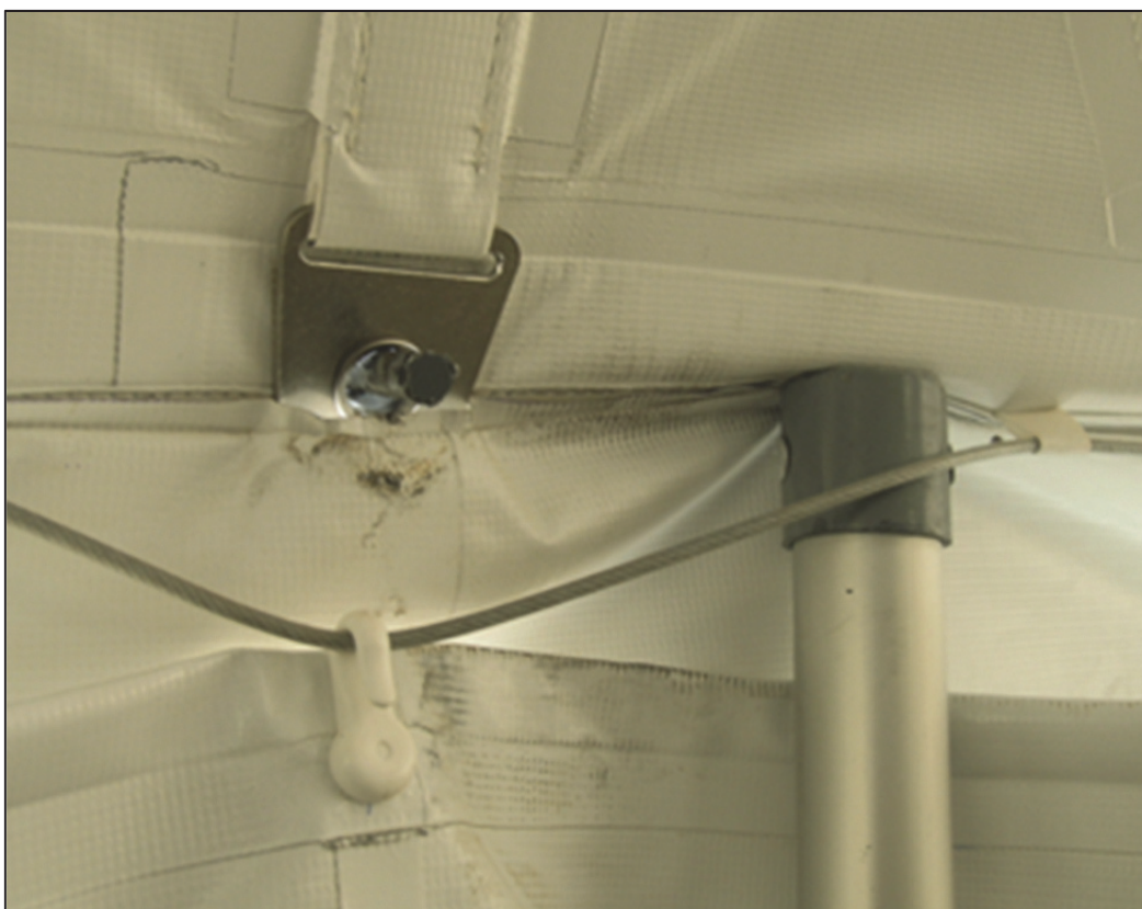
Figure 64. Example of Failed Connector at Top of Side Pole
