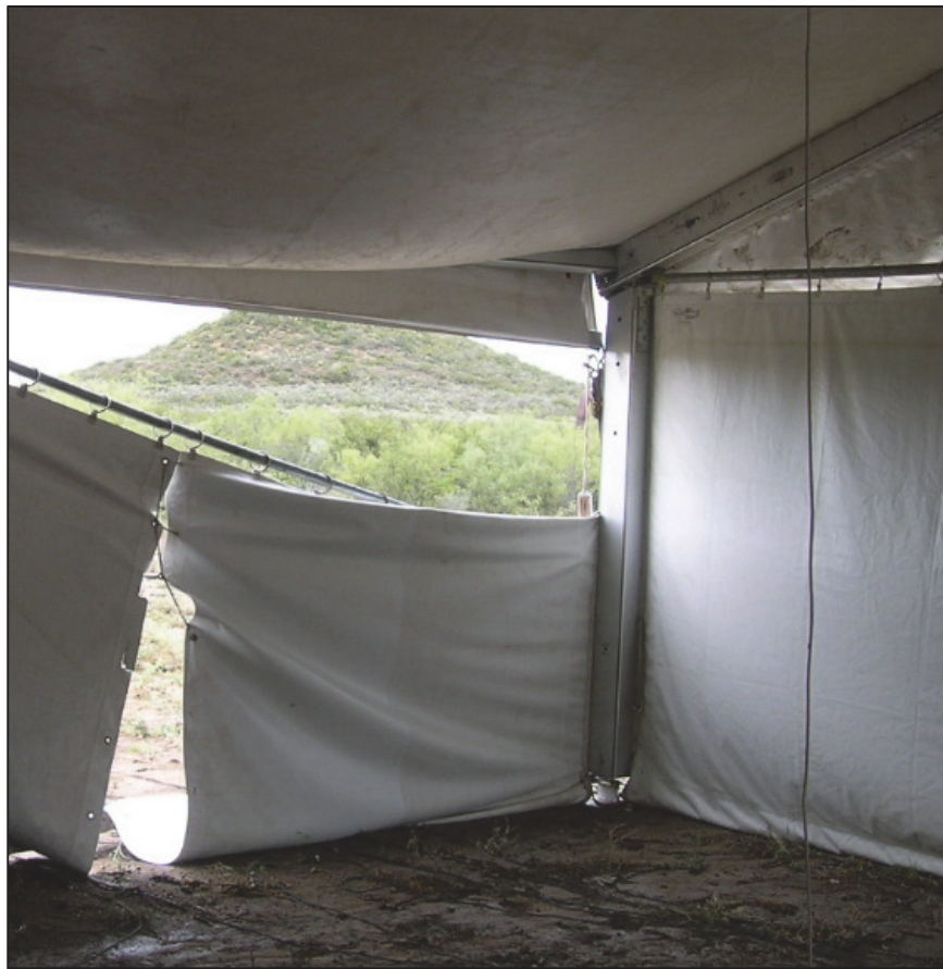
Figure 79. Damage to Rear of Framed Tent – Test C02
