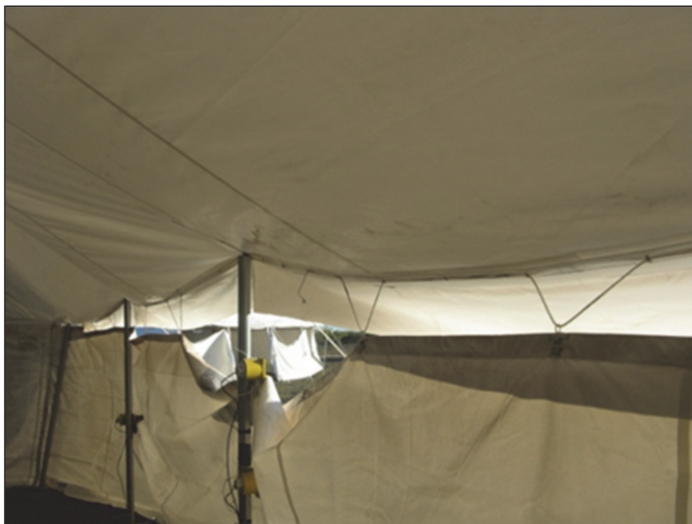
Figure 14. Rope to Wall Panel Connection, Non-Wind Rated Pole Tent w/ Sides, Test A03
