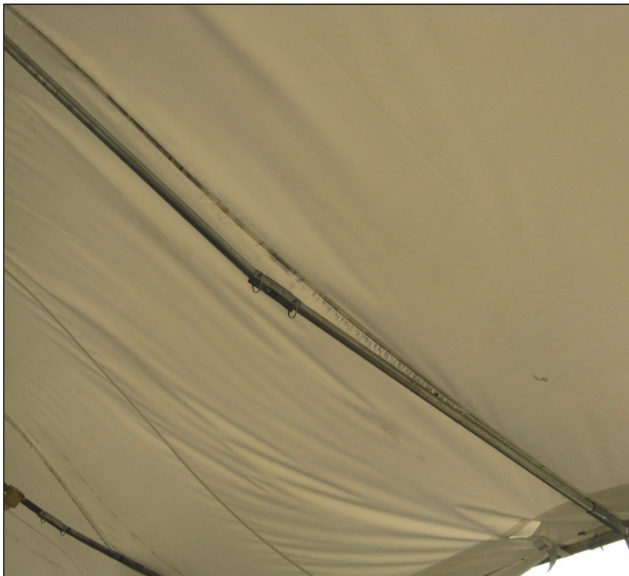
Figure 16. Damage to Hinge of Roof Frame Member, Light Frame Tent, Test A03
