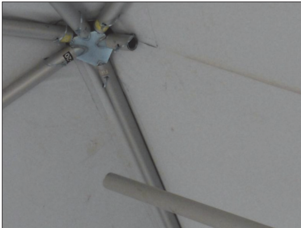
Figure 84. Failure of Roof Frame Connector – Test C02
