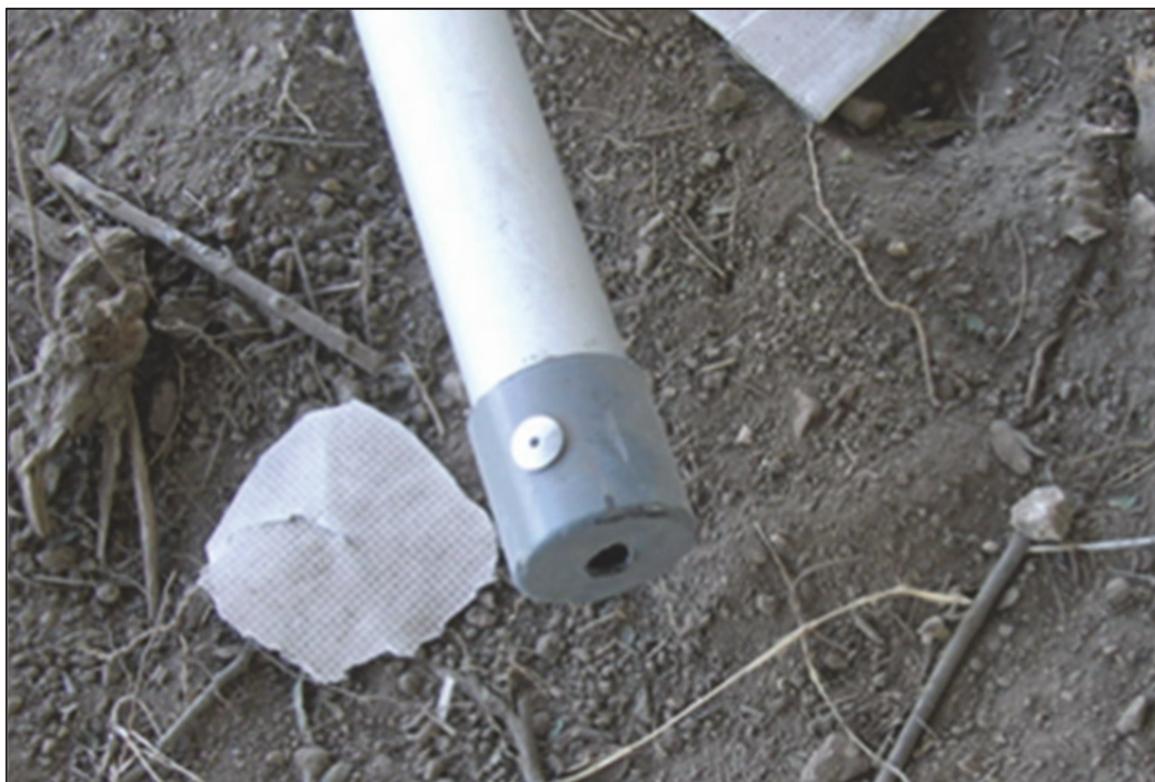
Figure 63. Damage to Connector at Top of Perimeter Pole
