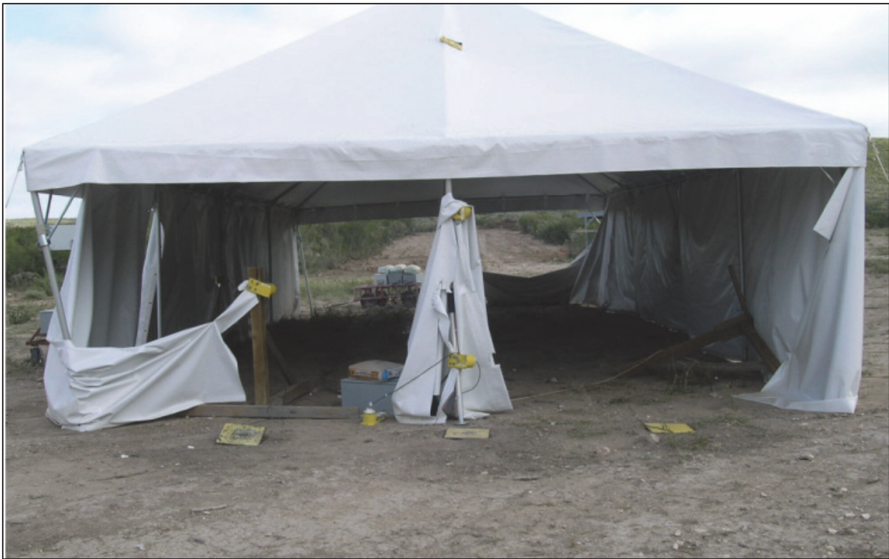
Figure 72. Damage to Front of Light Framed Tent – Test C01
