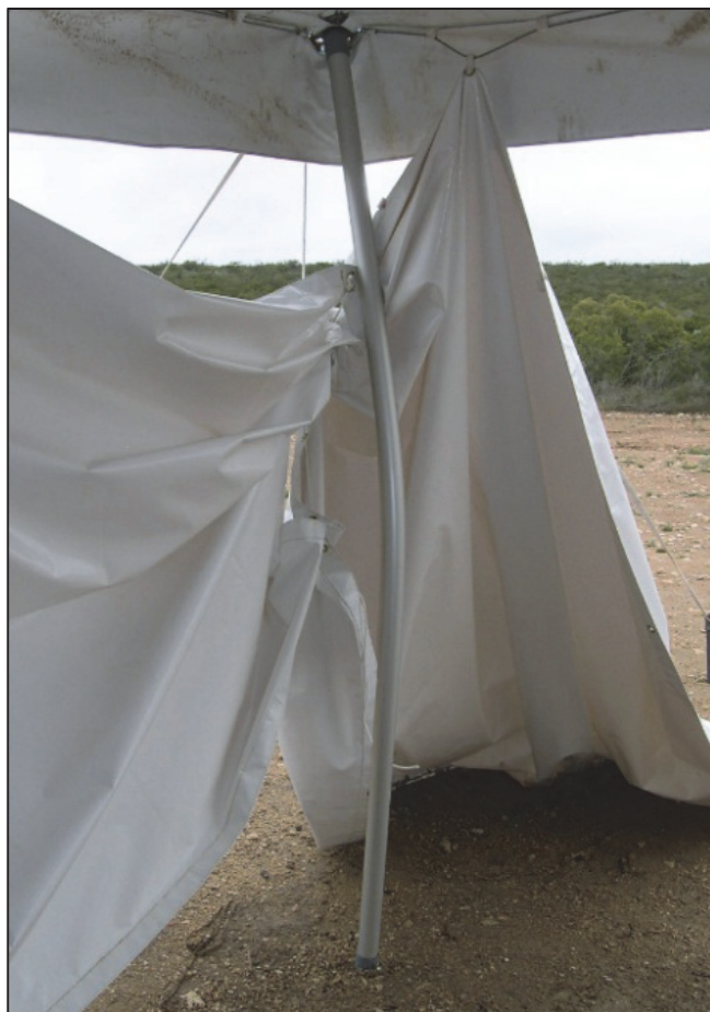
Figure 76. Bent Pole on Pole Tent – Test C02
