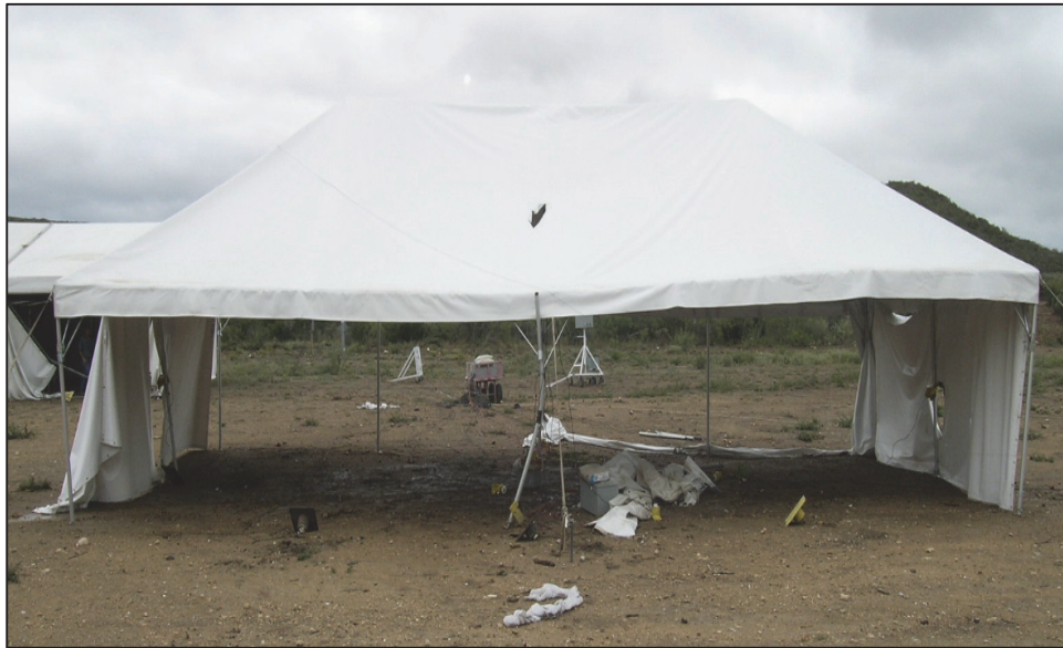
Figure 81. Damage to Light Framed Tent – Test C02
