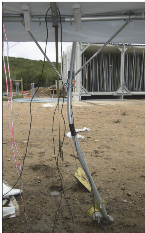
Figure 82. Bending of Side Frame – Test C02
