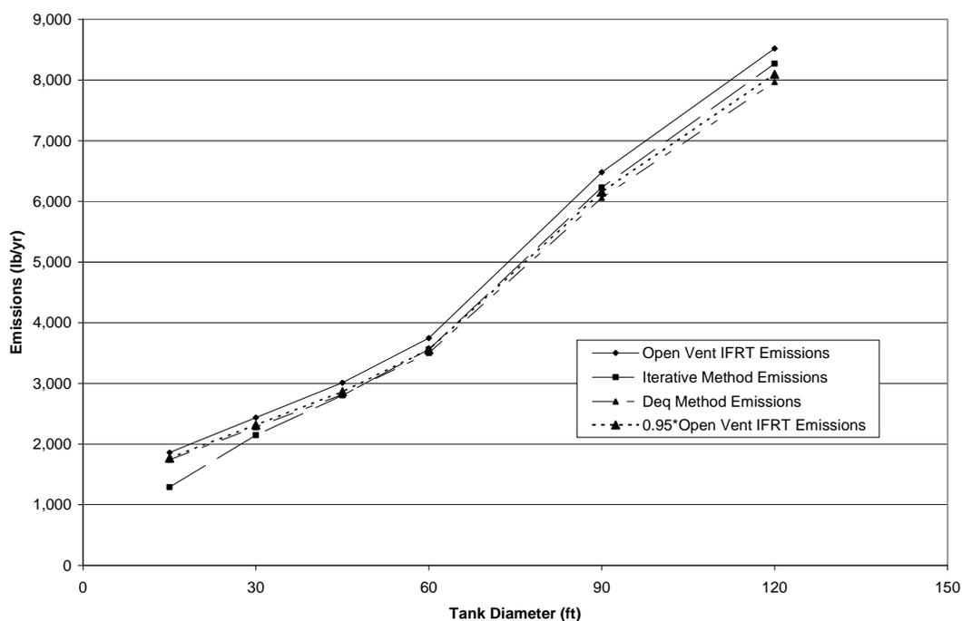
Figure 6—RVP 13 Gasoline Equivalent-Diameter vs Iterative Method 15 Days Between Turnovers
