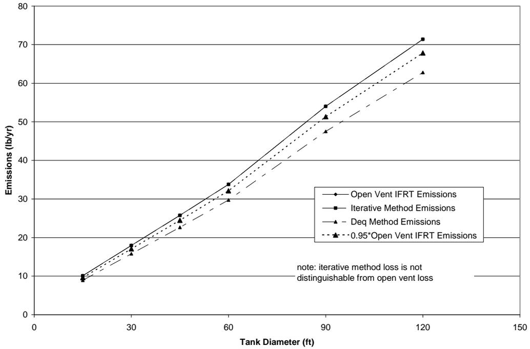
Figure 11—Diesel Equivalent-diameter vs Iterative Method 5 Days Between Turnovers
