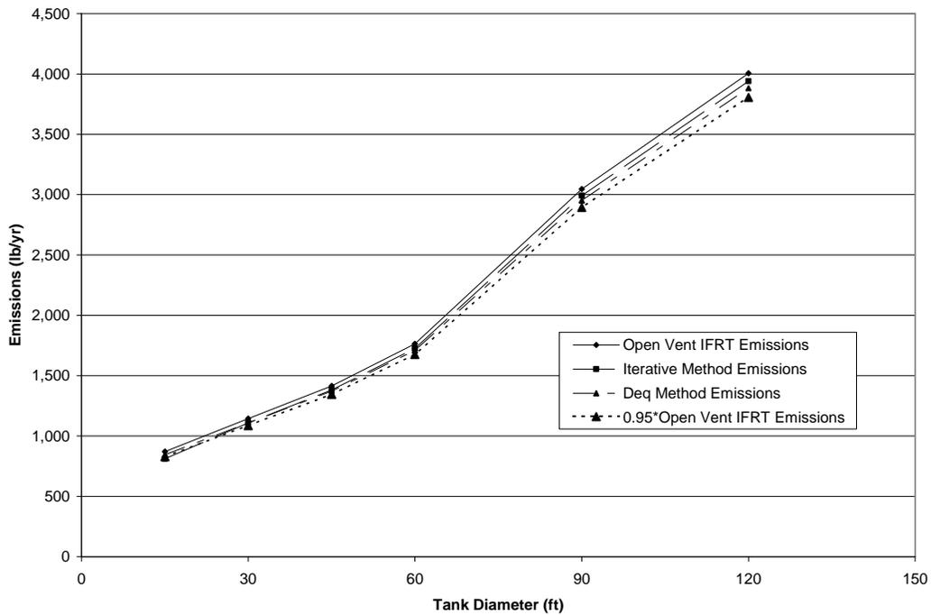
Figure 8—RVP 7 Gasoline Equivalent-diameter vs Iterative Method 5 Days Between Turnovers
