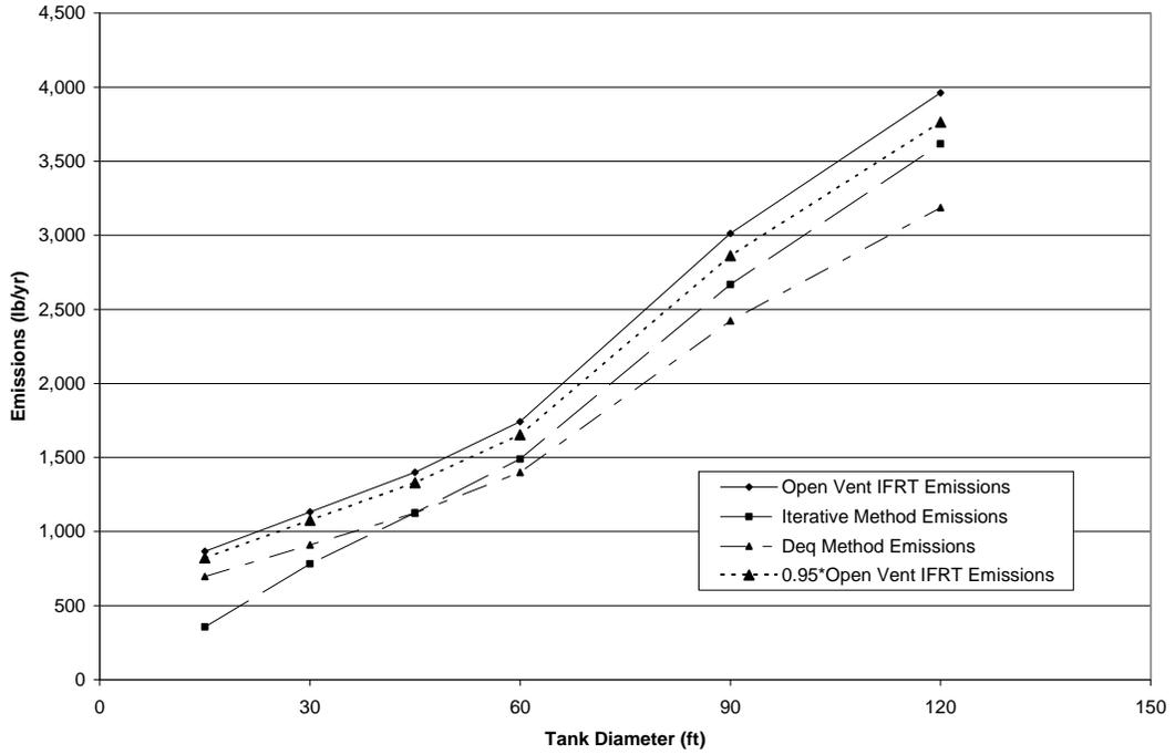
Figure 10—RVP 7 Gasoline Equivalent-diameter vs Iterative Method 90 Days Between Turnovers
