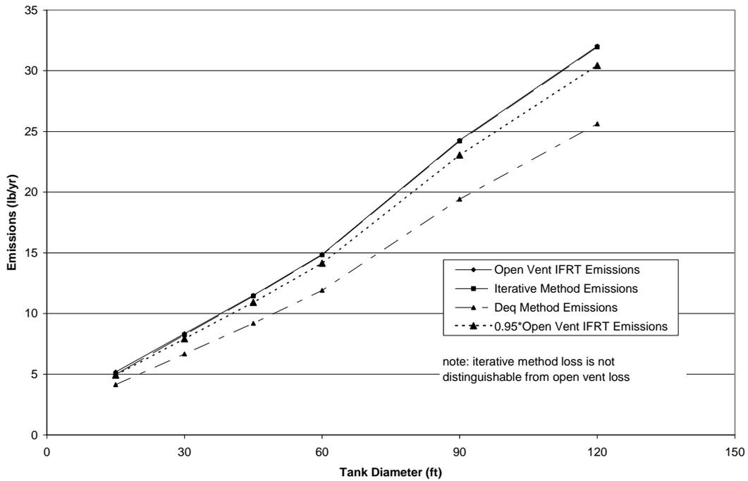
Figure 12—Diesel Equivalent-diameter vs Iterative Method 15 Days Between Turnovers
