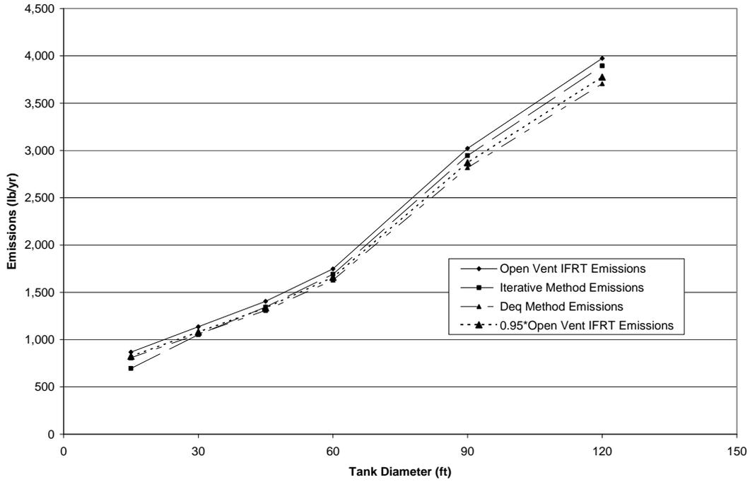
Figure 9—RVP 7 Gasoline Equivalent-diameter vs Iterative Method 15 Days Between Turnovers
