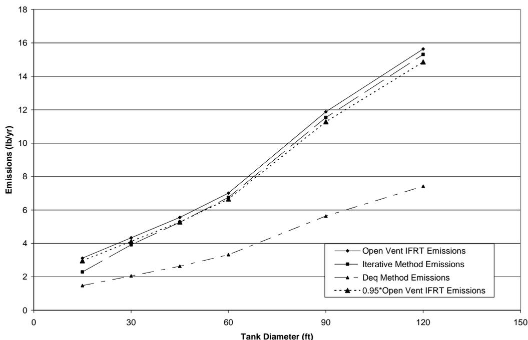
Figure 13—Diesel Equivalent-diameter vs Iterative Method 90 Days Between Turnovers
