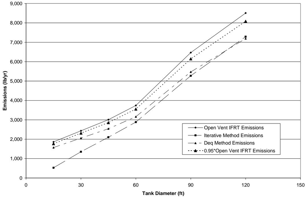
Figure 7—RVP 13 Gasoline Equivalent-diameter vs Iterative Method 90 Days Between Turnovers
