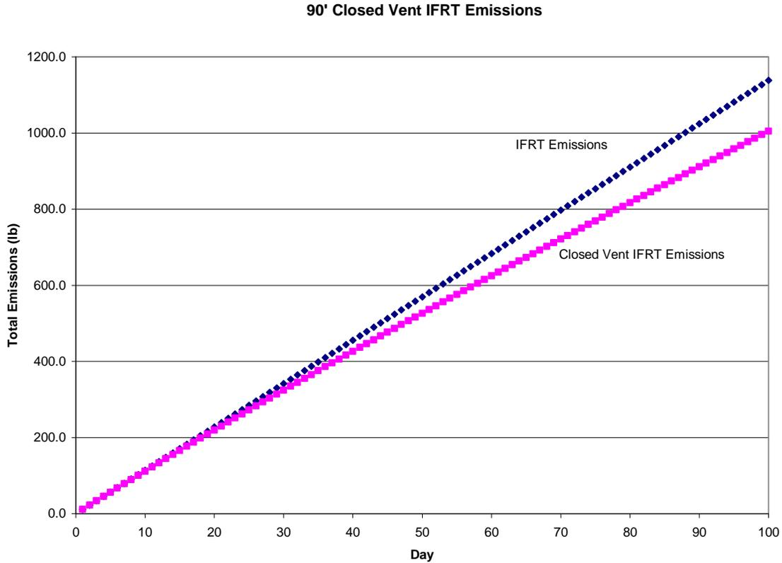
Figure 3—The Effect on Emissions of Adding Closed Vents to an IFRT
