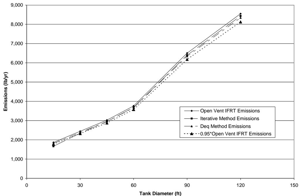
Figure 5—RVP 13 Gasoline Equivalent-Diameter vs Iterative Method 5 Days Between Turnovers
