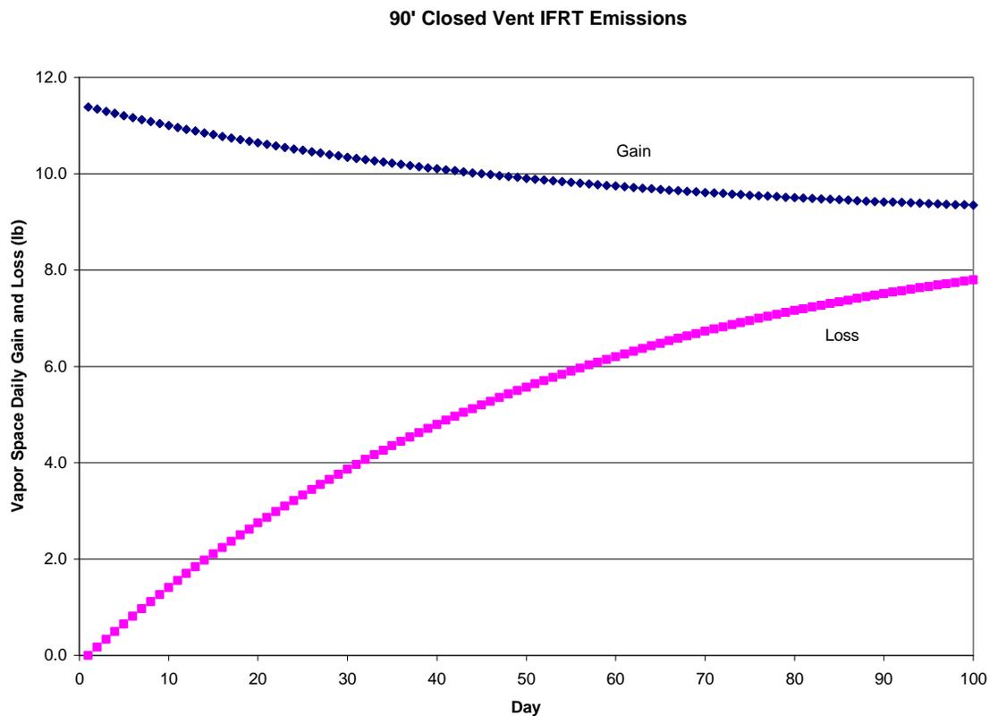
Figure 2—Gain and Loss of Vapors from the Vapor Space
