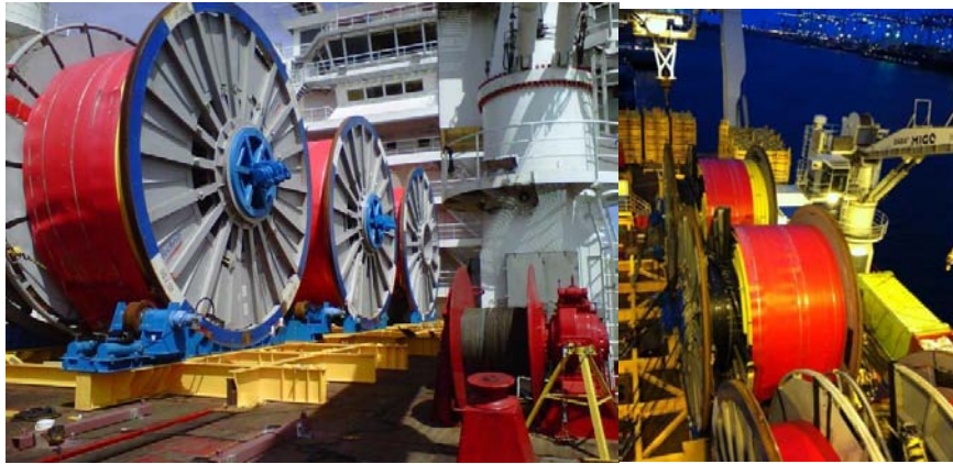
Figure 16—Typical Installation Reels Setup
