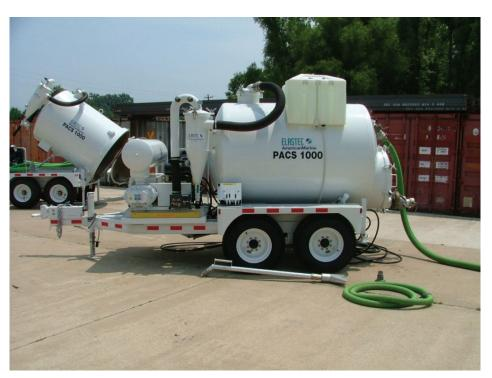
Figure 5.3 Use of Portable Vacuum System to Recover Oil
