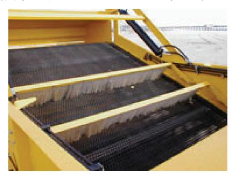
Figure 5.22 Rotating Screen with Brushes to Breakup Sand Accumulations
