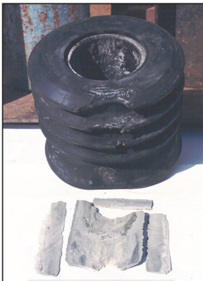
Figure 11—Photo from Large-scale Experiment Showing Damage to Wiper Plug Caused by Solids on Low Side of Casing
