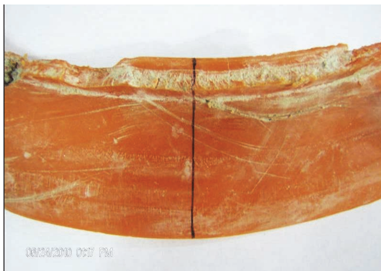
Figure 34—Using an Appropriate Cutting Tool, Cut Line Down on Fin Section
