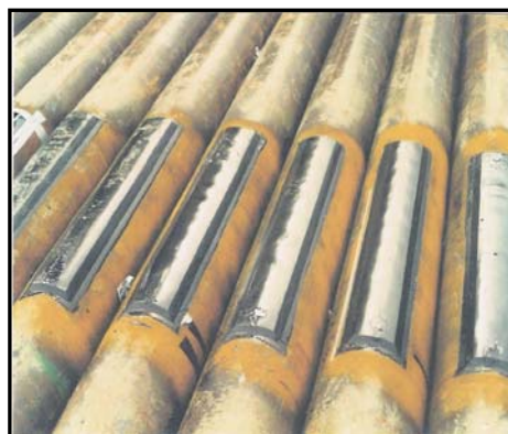
Figure 11—Example of Centralizers Bonded Directly onto the Pipe
