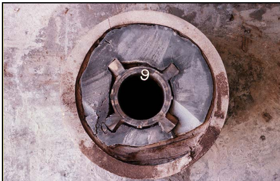
Figure 17—Swirl-inducing Centralizer in a Deviated, Enlarged Hole with Permeability
