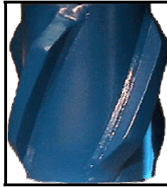
Figure 8—Example of Steel Spiral Solid Centralizer
