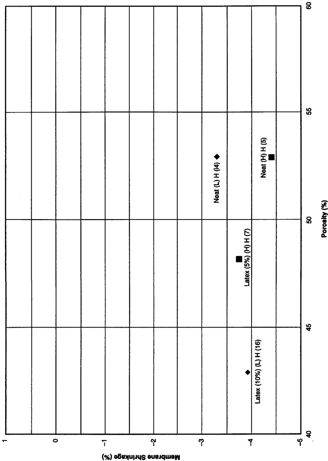
Figure 13—Porosity and Membrane Shrinkage
