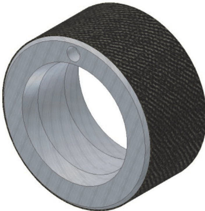
Figure 2—Drill Stem Element Test Specimen with a Material Coating
