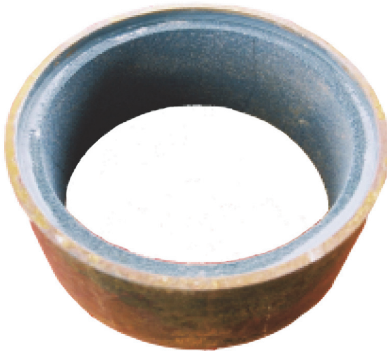
Figure 5—Aluminum Oxide Abrasive Cylinder Mounted in a Piece of Casing
