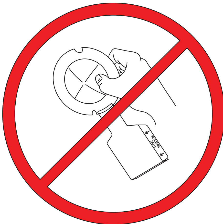
Figure A.3—Improper Handling of a Rupture Disk
