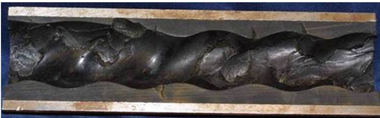
Figure I.10 — Torn/chunked stator (provided courtesy of CFER Technologies)
