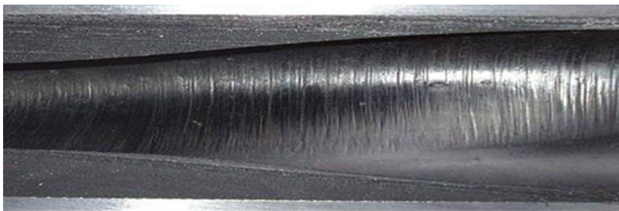
Figure I.12 — Stator worn (provided courtesy of Kudu Industries)
