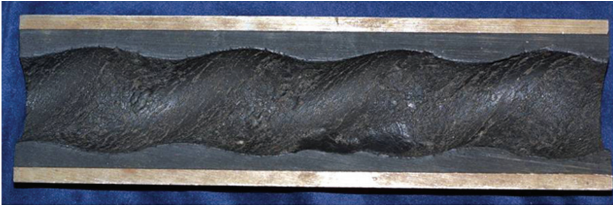
Figure I.6 — Burned/overheated stator (provided courtesy of CFER Technologies)
