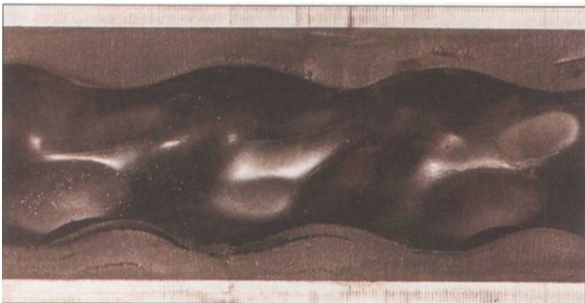
Figure I.5 — Blistered stator (provided courtesy of Weatherford)
