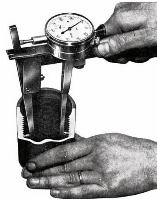
Figure 12—Typical Internal-Thread Taper Gauge for Threads in Sizes Smaller than 4 1 / 2
