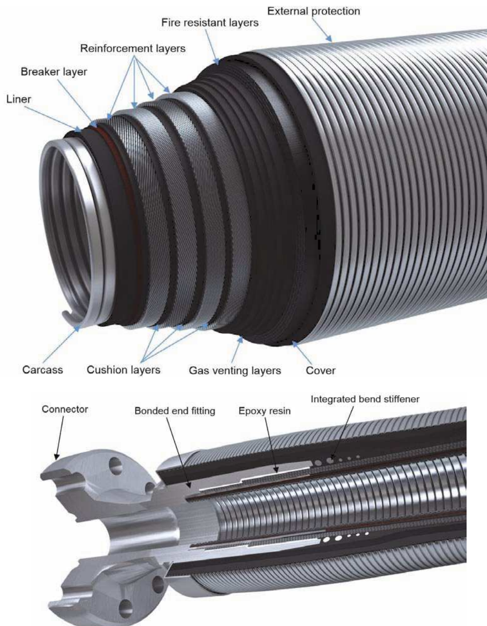
Figure 1a—Typical Bonded Flexible Pipe—Flowline and Riser
