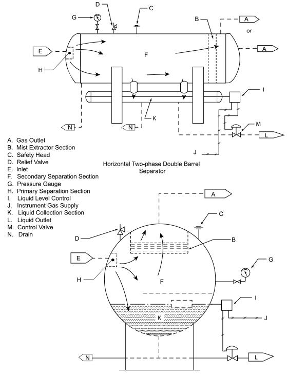
Spherical Two-phase Seperator
