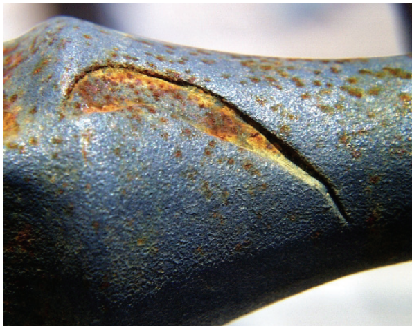
Forging Overfill Fold
