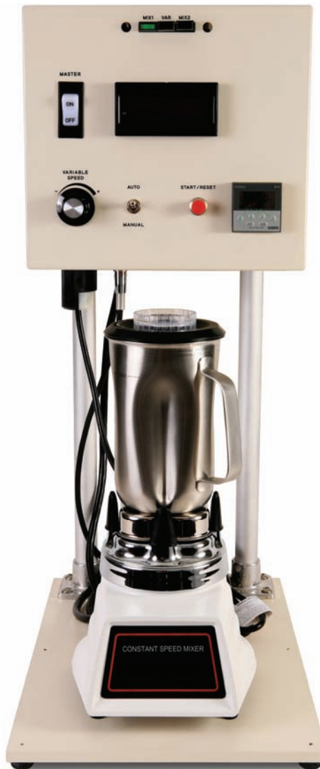
Figure 1 — Example of a typical cement-mixing device
