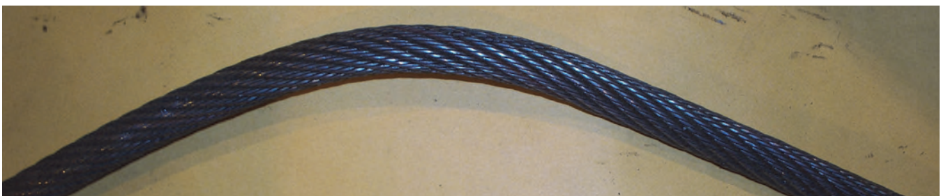
Figure 25—Example of a Permanent Bend in a Wire Rope
