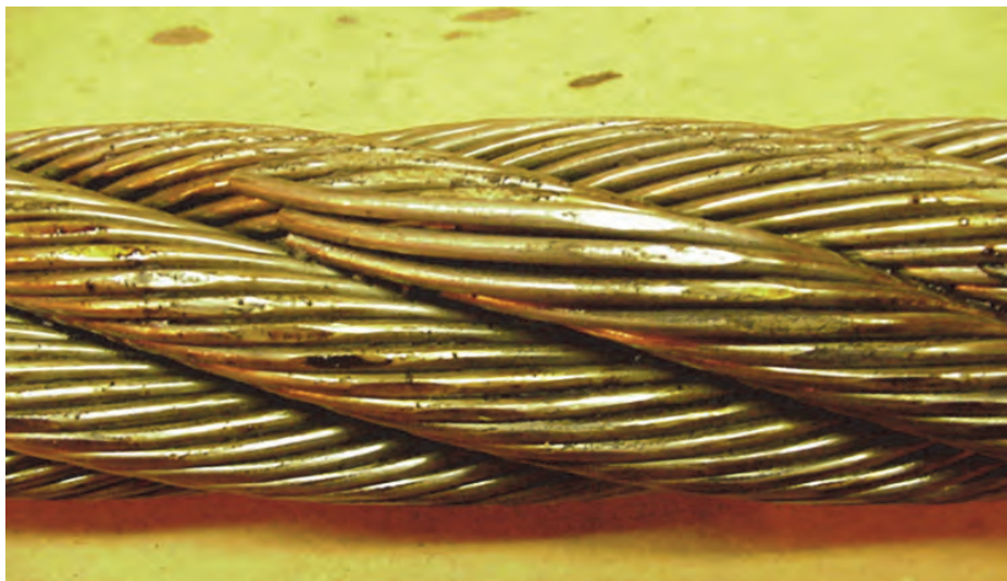
Figure 17—Example of Valley Wire Breaks that are Displaced from their Unbroken Position
