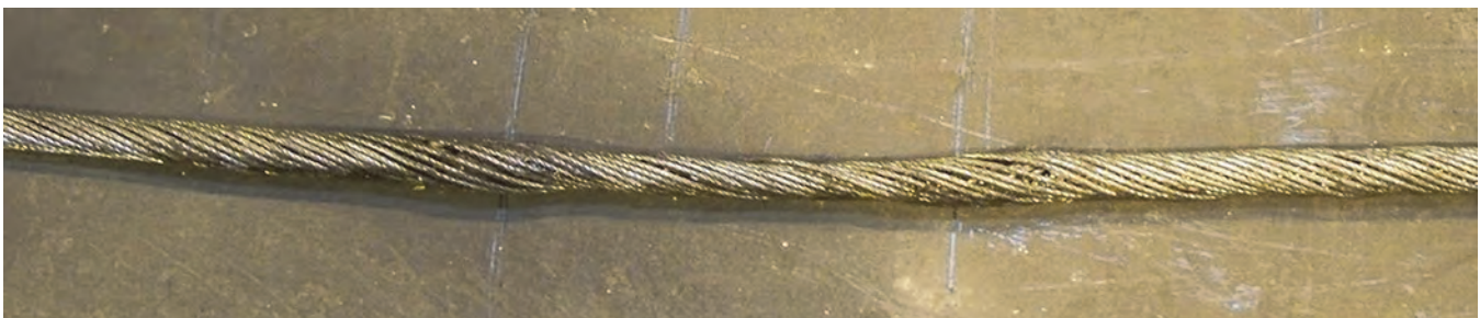
Figure 29—Example of Loss of Core Support Resulting in Localized Diameter Reduction
