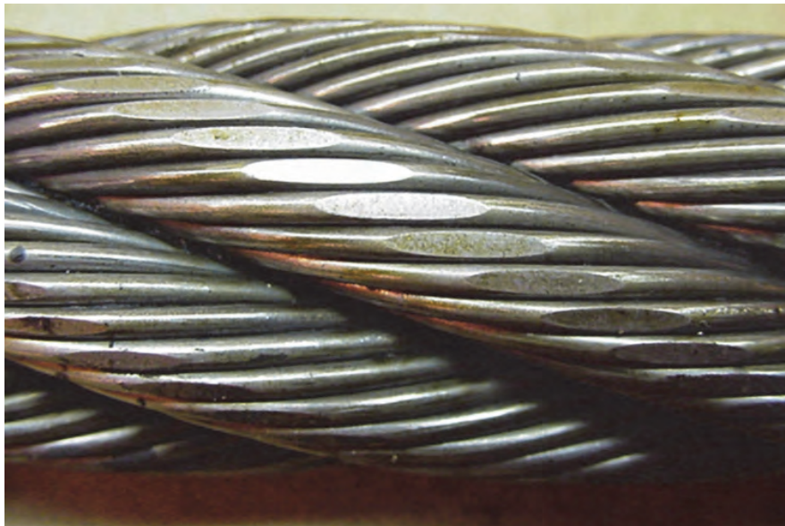
Figure 14 —Example of Abrasion of the Outer Wires
