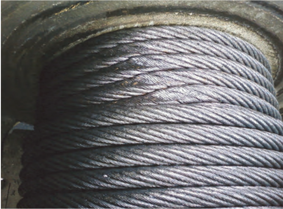
Figure 19—Example of Pattern of Drum Crushing
