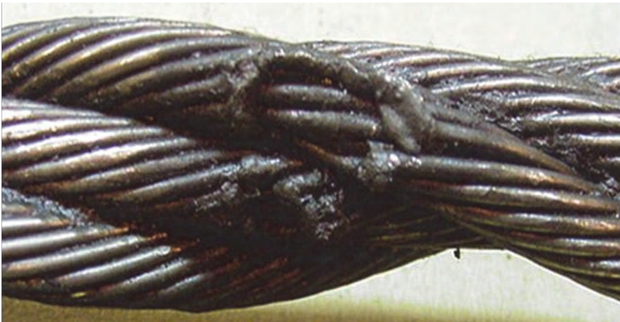
Figure 30—Example of Electrical Arc Causing Severe Wire Rope Damage
