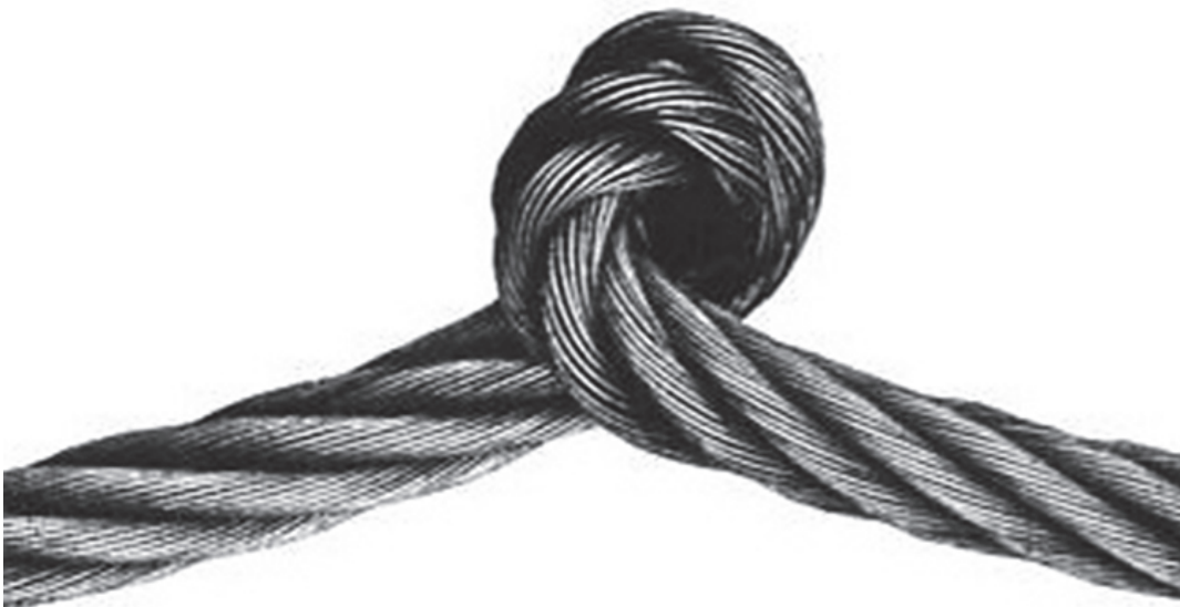
Figure 24—Example of a Kink in a Wire Rope
