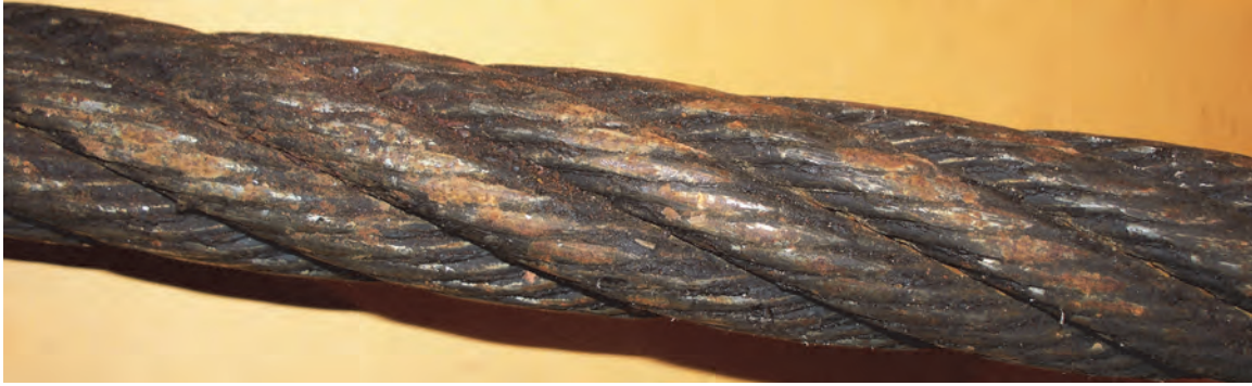
Figure 21—Example of Surface Corrosion on a Wire Rope
