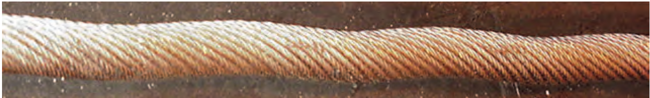
Figure 26—Example of Waviness in a Wire Rope
