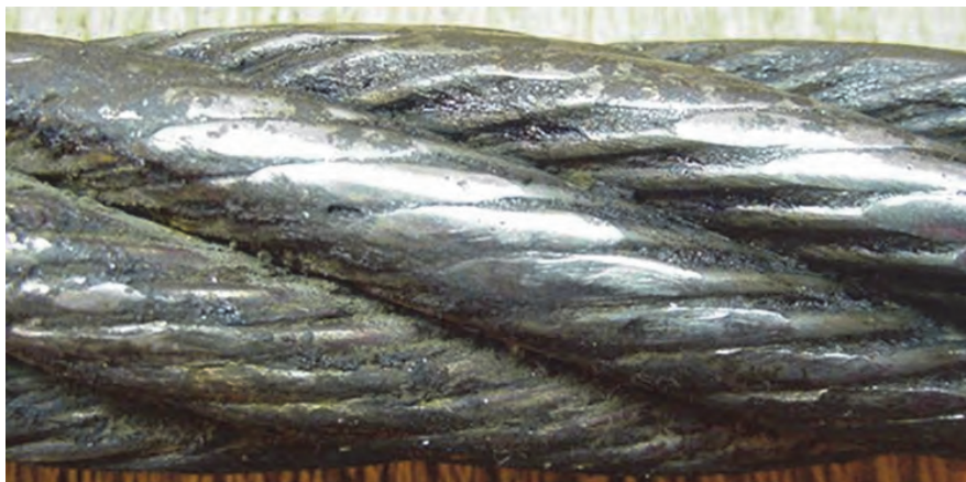
Figure 15 —Example of Peening of the Outer Wires
