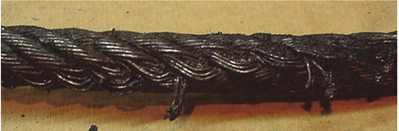
Figure 18—Example of External Damage Resulting in Broken Wires
