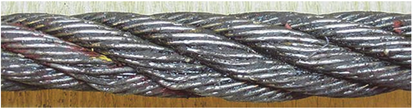
Figure 20—Example of Crushing on a Wire Rope
