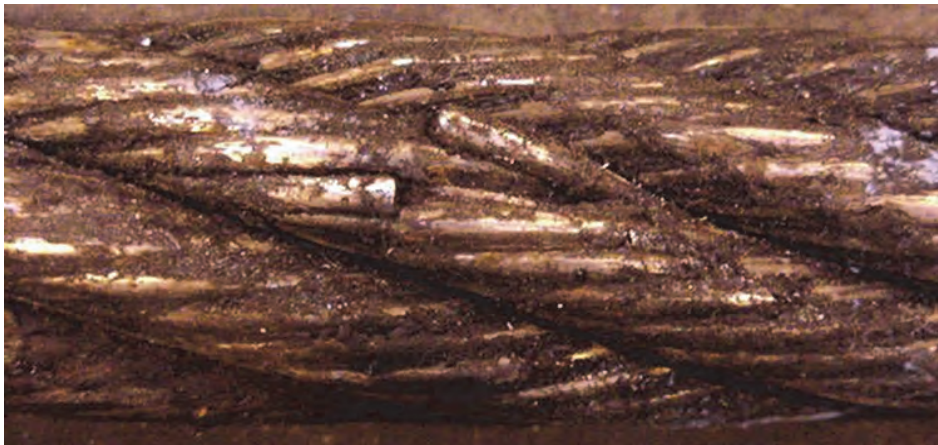
Figure 16—Example of Single Broken Wire on the Crown of a Wire Rope
