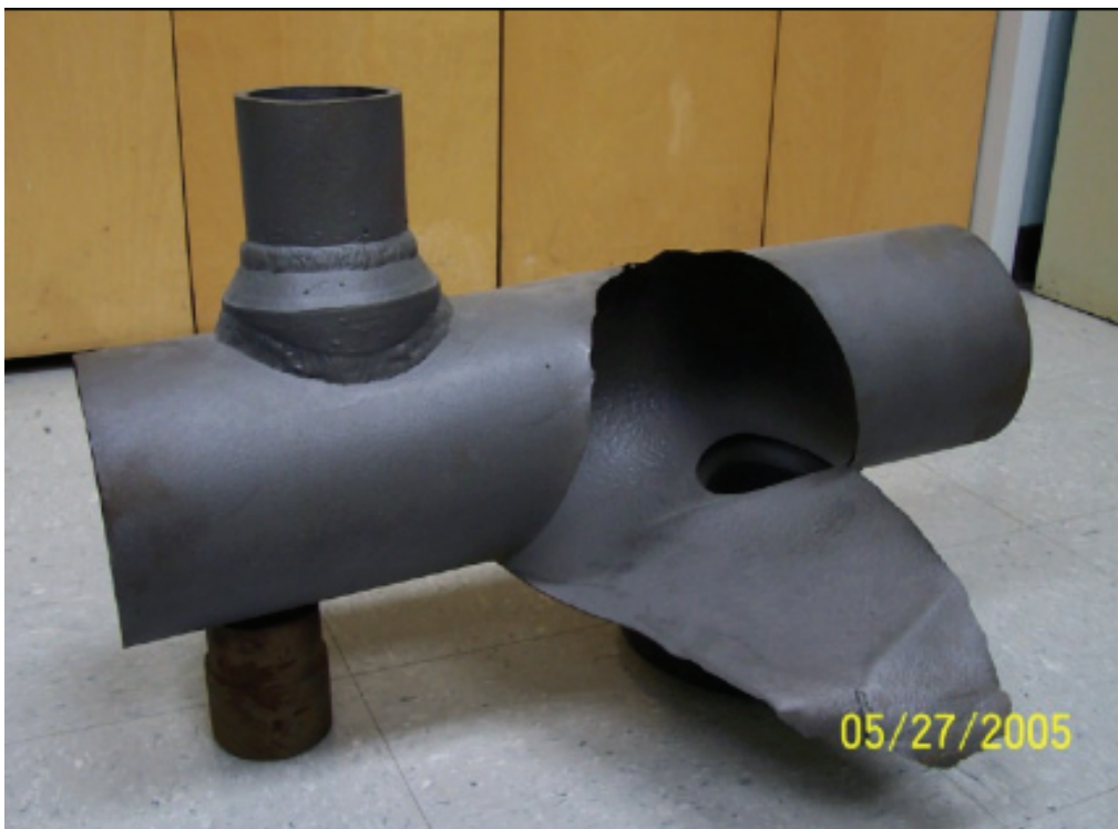
Figure 1—NPS 8 Carbon Steel Piping Failed Due to Sulfidation Corrosion ( H_2 Free)
