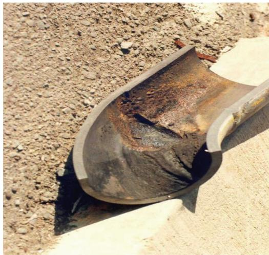
**Figure 12—Erosion-Corrosion of Carbon Steel Piping Elbow**
