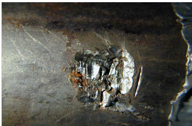
Figure D.22—Gouges with Large Transverse Component
