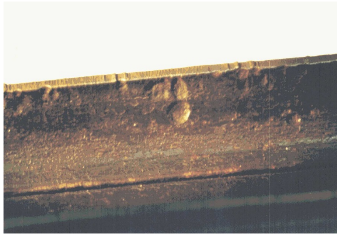
Figure D.5—Carbon Dioxide Pitting in Hang-off Tubing
