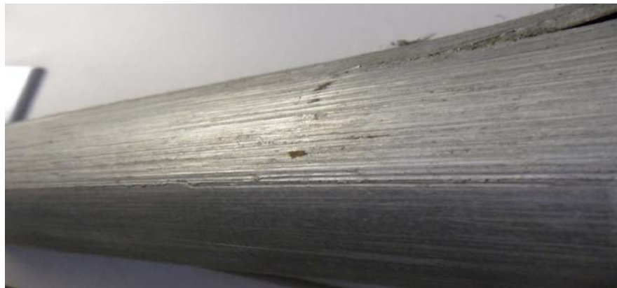
Figure D.24—Scoring Marks on the Tube Outside Diameter
