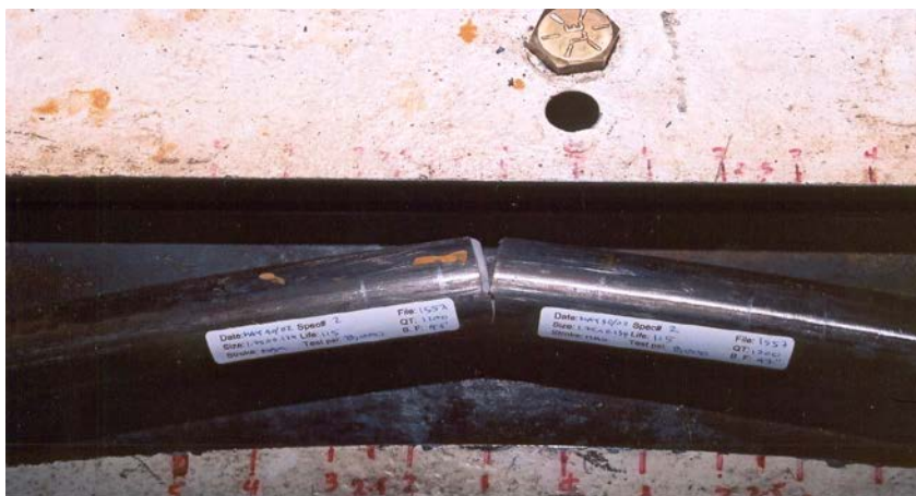
Figure D.11—Fatigue Crack Originating with High Pressure Inside the Tubing
