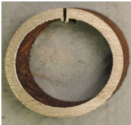
Figure D.29—Burst at Thin Wall Area in Tubing
