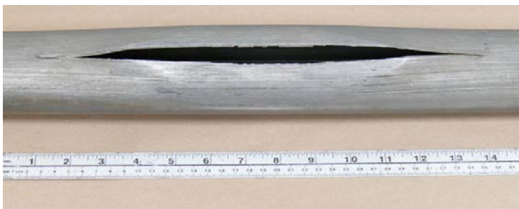
Figure D.29—Burst at Thin Wall Area in Tubing
