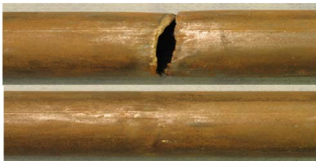
Figure D.15—Separation Caused by Tensile Overload Under Flexure
