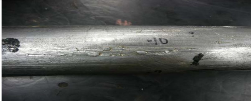
Figure D.27—Wear with Galling
