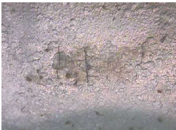
Figure D.2—Pitting that Occurred from Acid During Storage (Transversely Oriented Fatigue Cracks in Base of Pitting Inside Tubing at Location of Storage Corrosion) (Continued)
