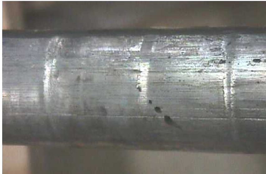
Figure D.40—Injector Ring Damage
