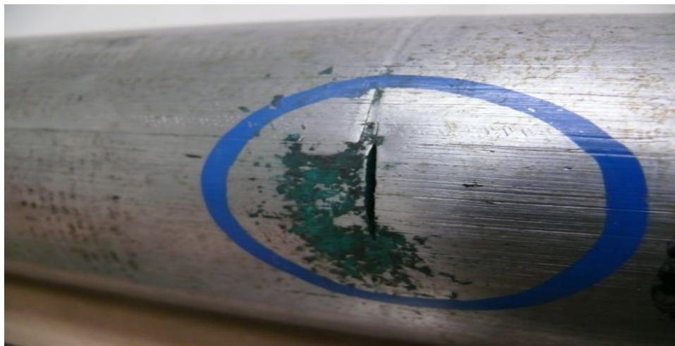
Figure D.39—Gripper Block Mark with Fatigue Crack
