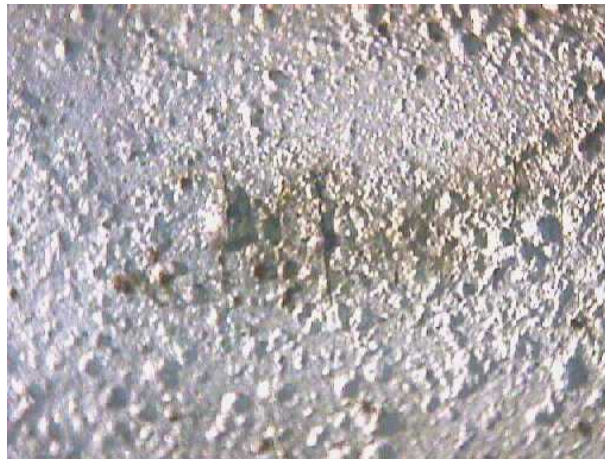
Figure D.2—Pitting that Occurred from Acid During Storage (Transversely Oriented Fatigue Cracks in Base of Pitting Inside Tubing at Location of Storage Corrosion)
