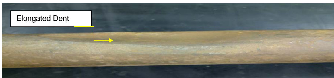
Figure D.35—Elongated Dent
