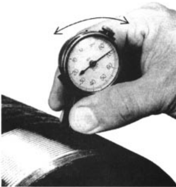
Figure 24—External/Internal Thread Height Gauge Applied to a Thread (Arcing Lines Show Direction of Rocking Motion)
