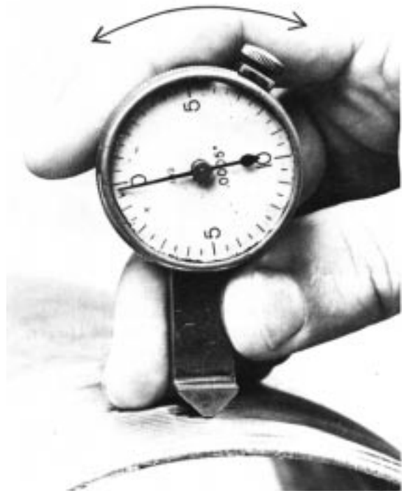
Figure 25—Balanced-Dial Type Gauge Applied to Thread Showing Small Error in Thread Height
