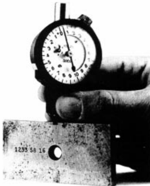
Figure 21—Height Gauge Applied to Setting Standard (Balanced-Type)
