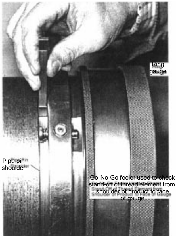
Figure 55—Extreme-Line Thread Ring Gauge Installed Hand-Tight and Seal Ring Advanced (Note use of Go-No-Go Gauge)
