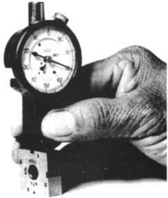
Figure 23—Continuous-Dial Type Gauge Applied to a Setting Standard
