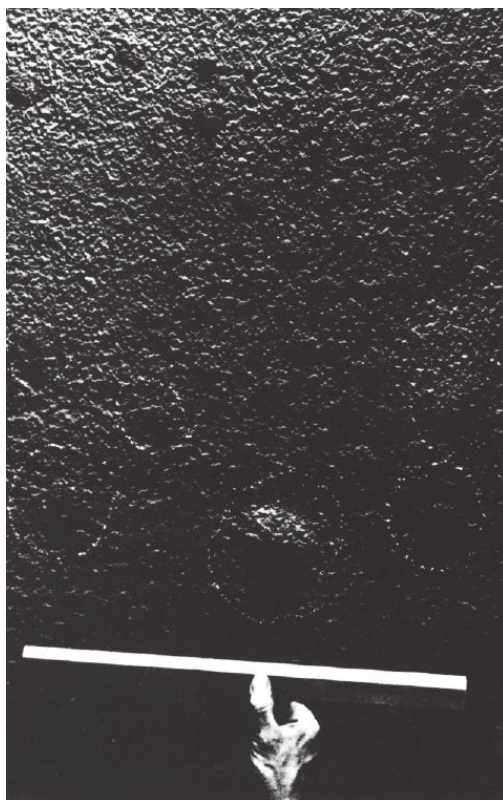
Figure 41—Small Hydrogen Blisters on Shell Interior
