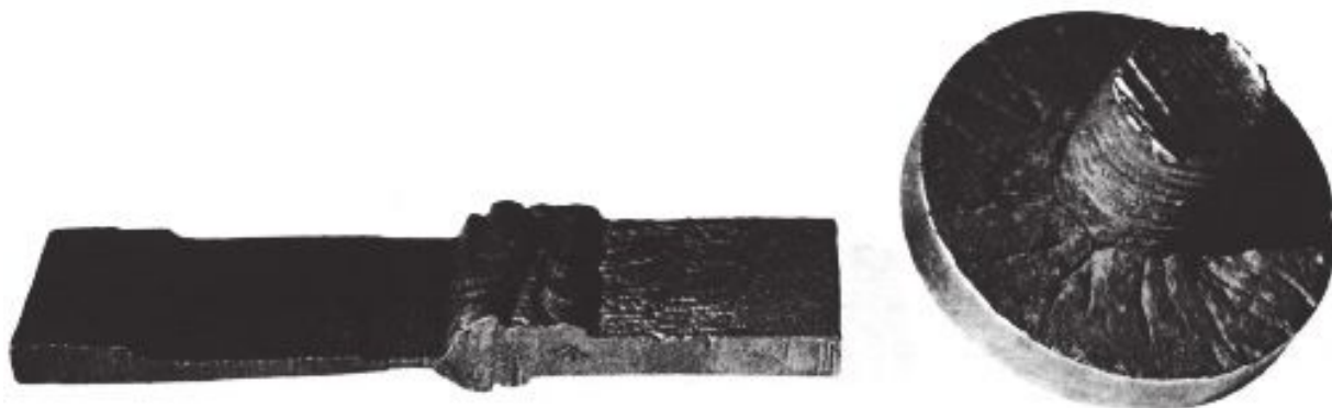
Figure 40—Caustic Stress Corrosion Cracks
