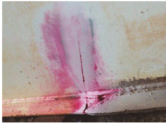
Figure 29—Cracks in Tank Shell Plate
