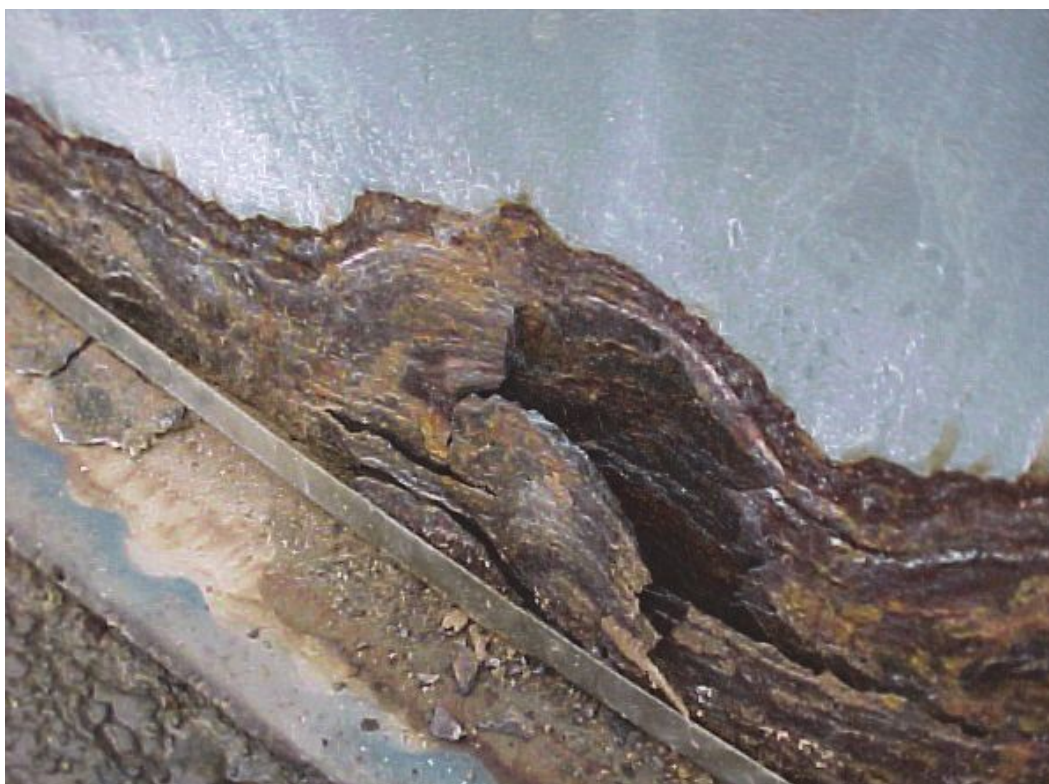
Figure 38—Close-up of Corrosion Under Insulation
