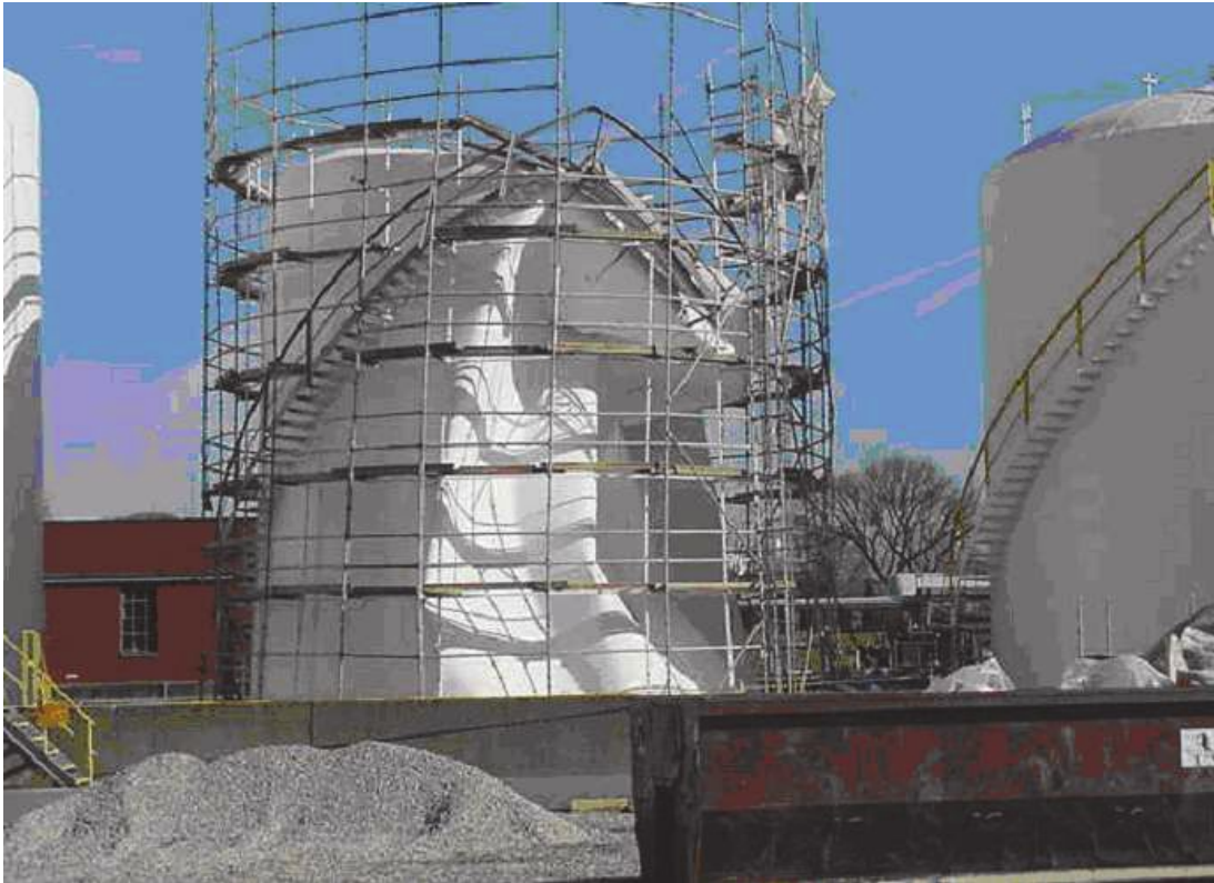
Figure 43—Tank Failure Caused by Inadequate Vacuum Venting
