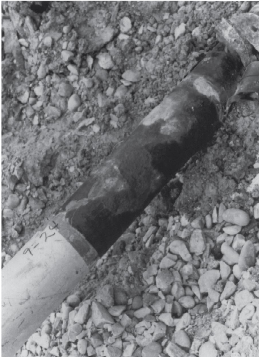
Figure 28—Underground Piping Corrosion Beneath Poorly Applied Tape Wrap
