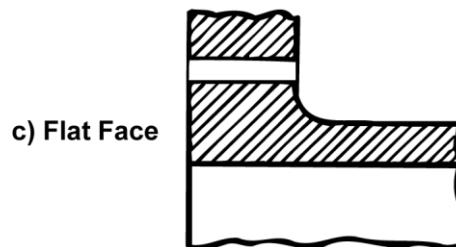
Figure 12—Flange Facings Commonly Used in Refinery and Chemical Plant Piping
