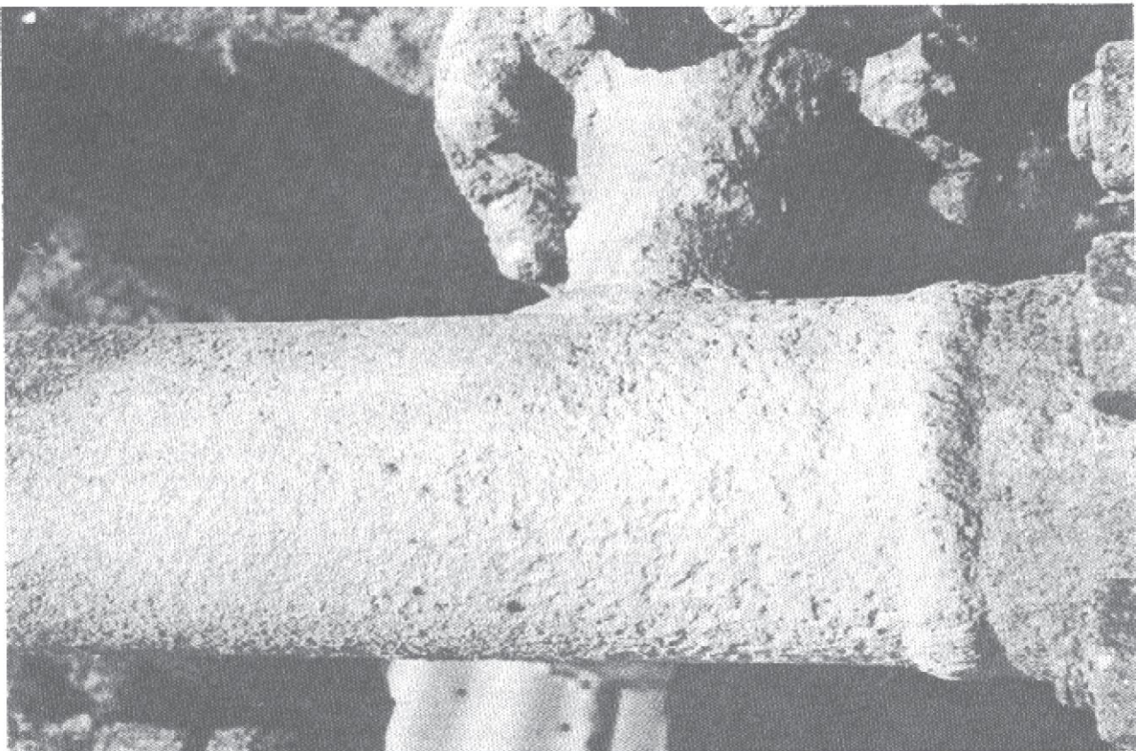
Figure 21—Severe Atmospheric Corrosion of Piping
