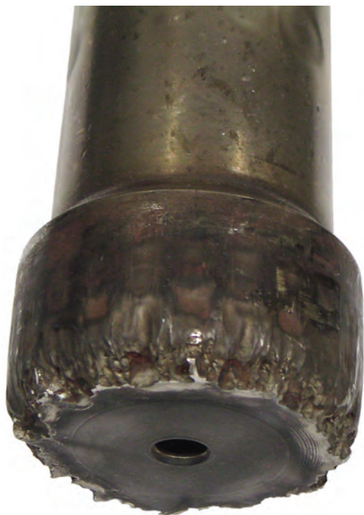
Figure 10—Cavitation Damage to Valve Plug
