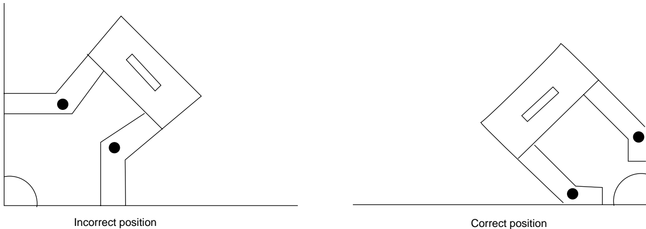
Figure 55—Incorrect and Correct Electromagnetic Yoke Setup for T and Y Joint Connections
