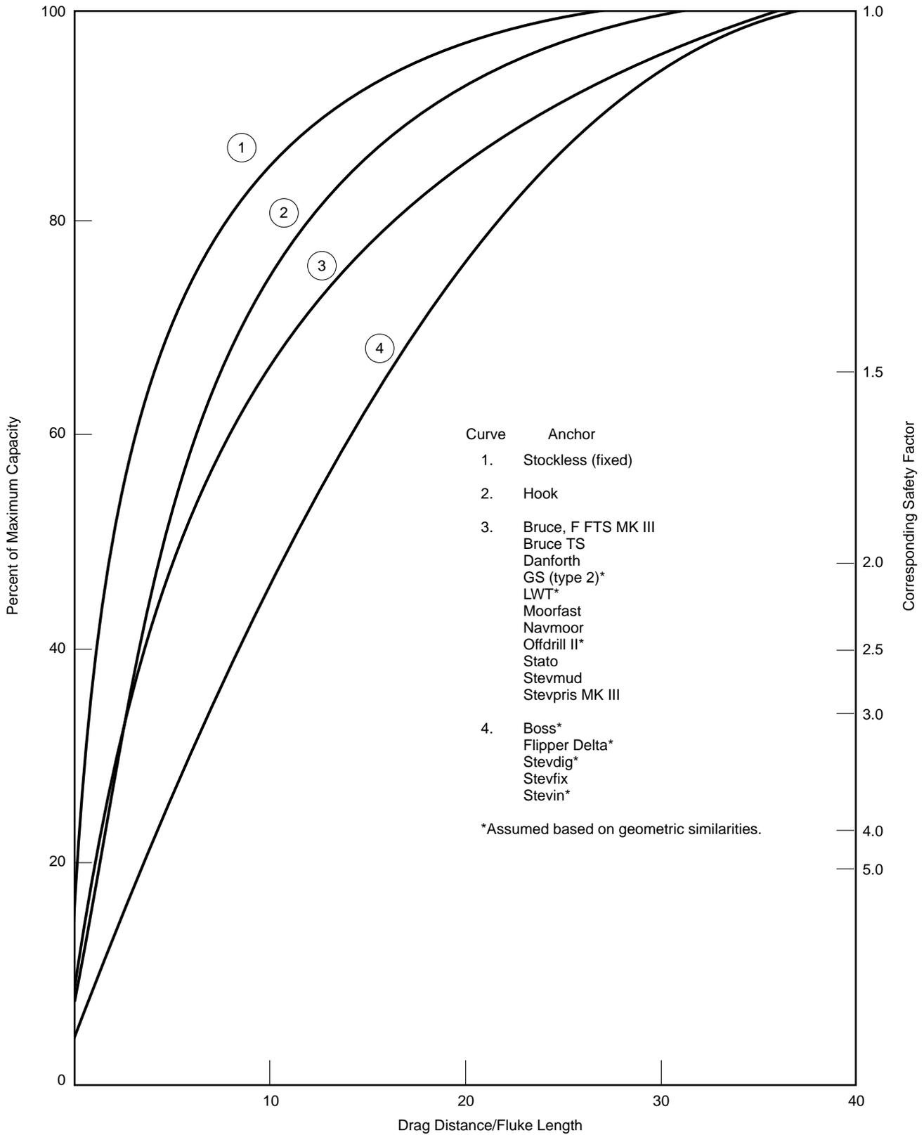
Figure D.6—Percent Holding Capacity versus Drag Distance in Soft Clay
