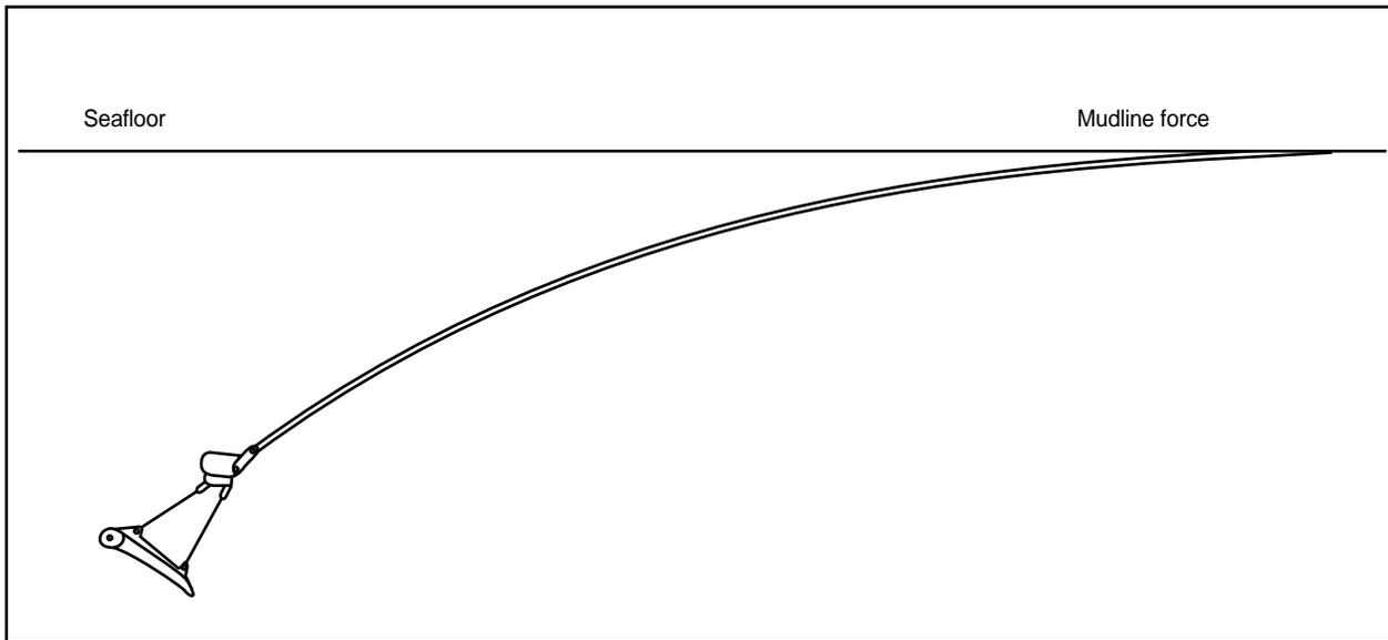
Figure E.5—Schematic of Anchor Line Configuration During Embedment
