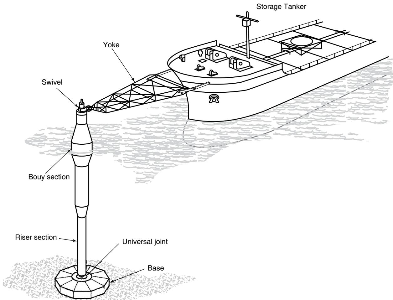
Figure 10—Single Anchor Leg Mooring (SALM) with Tubular Riser and Yoke
