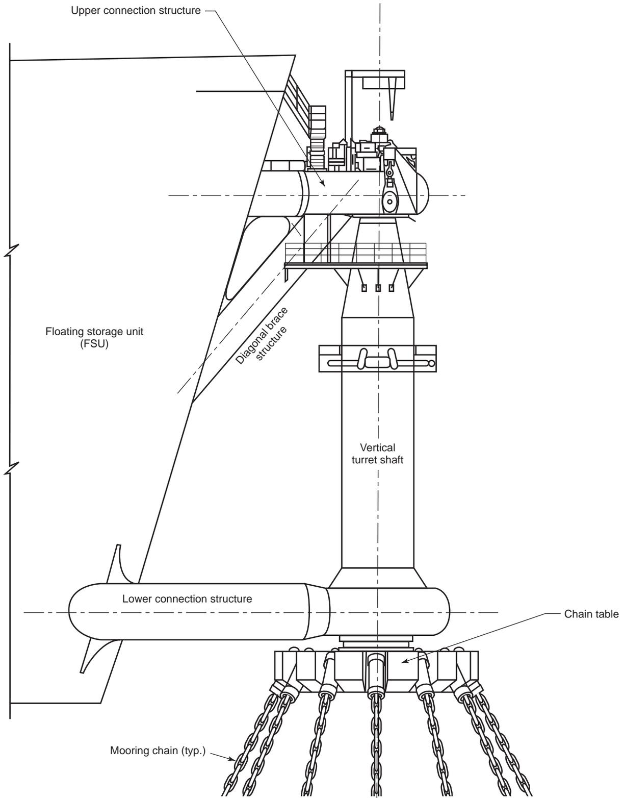
Figure 4—Typical External Turret Mooring Arrangement
