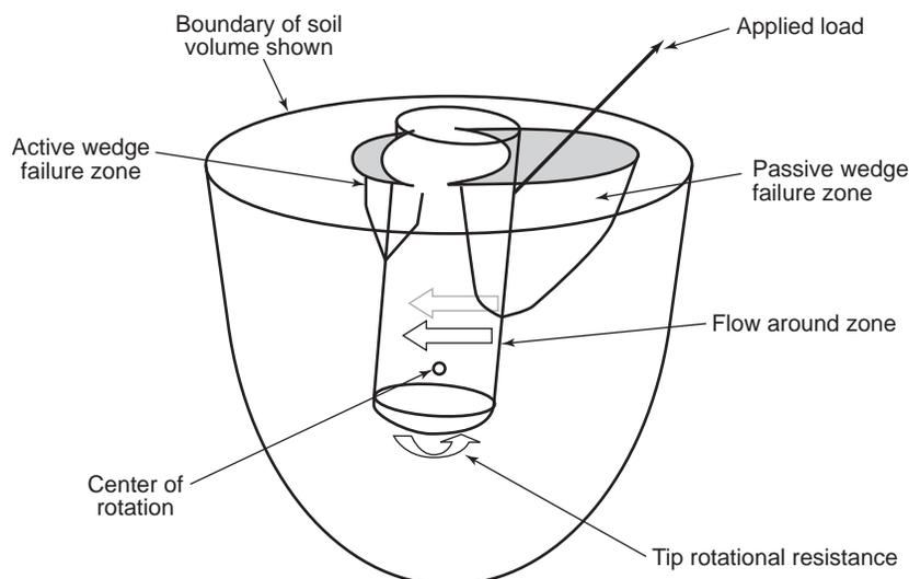
Figure E.1—Three-Dimensional View of a Possible Failure Mechanism
