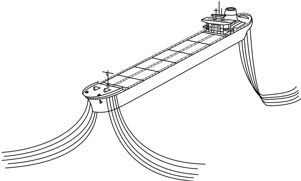
Figure 3—Differential Compliance Anchoring System (DICAS)
