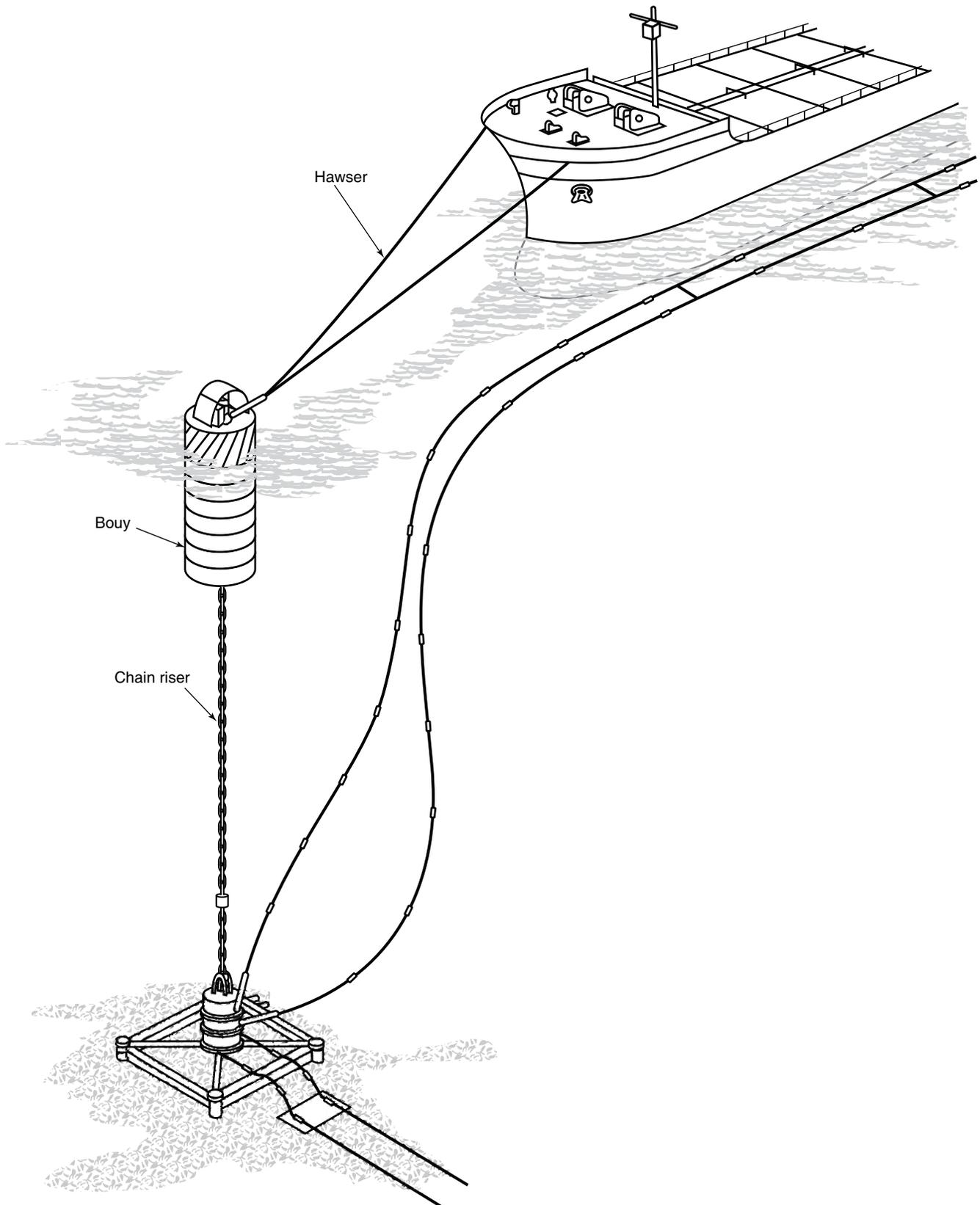
Figure 11—Single Anchor Leg Mooring (SALM) with Chain Riser and Hawser
