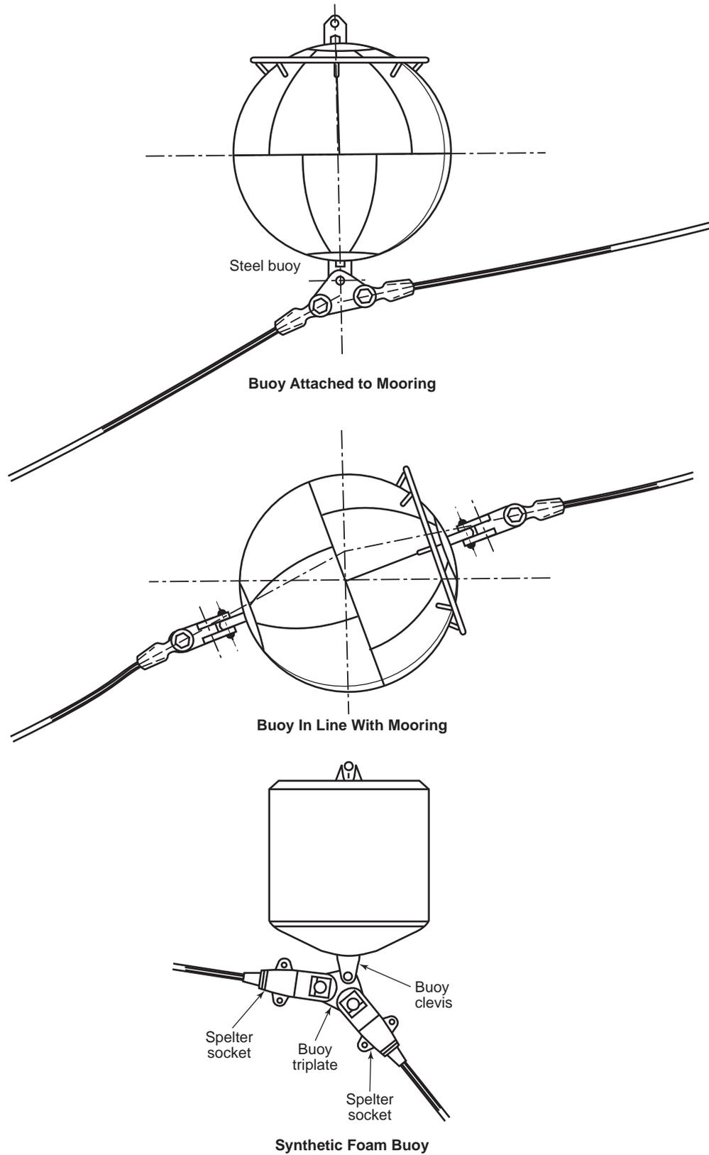
Figure A.5—Submersible Buoy Configurations
