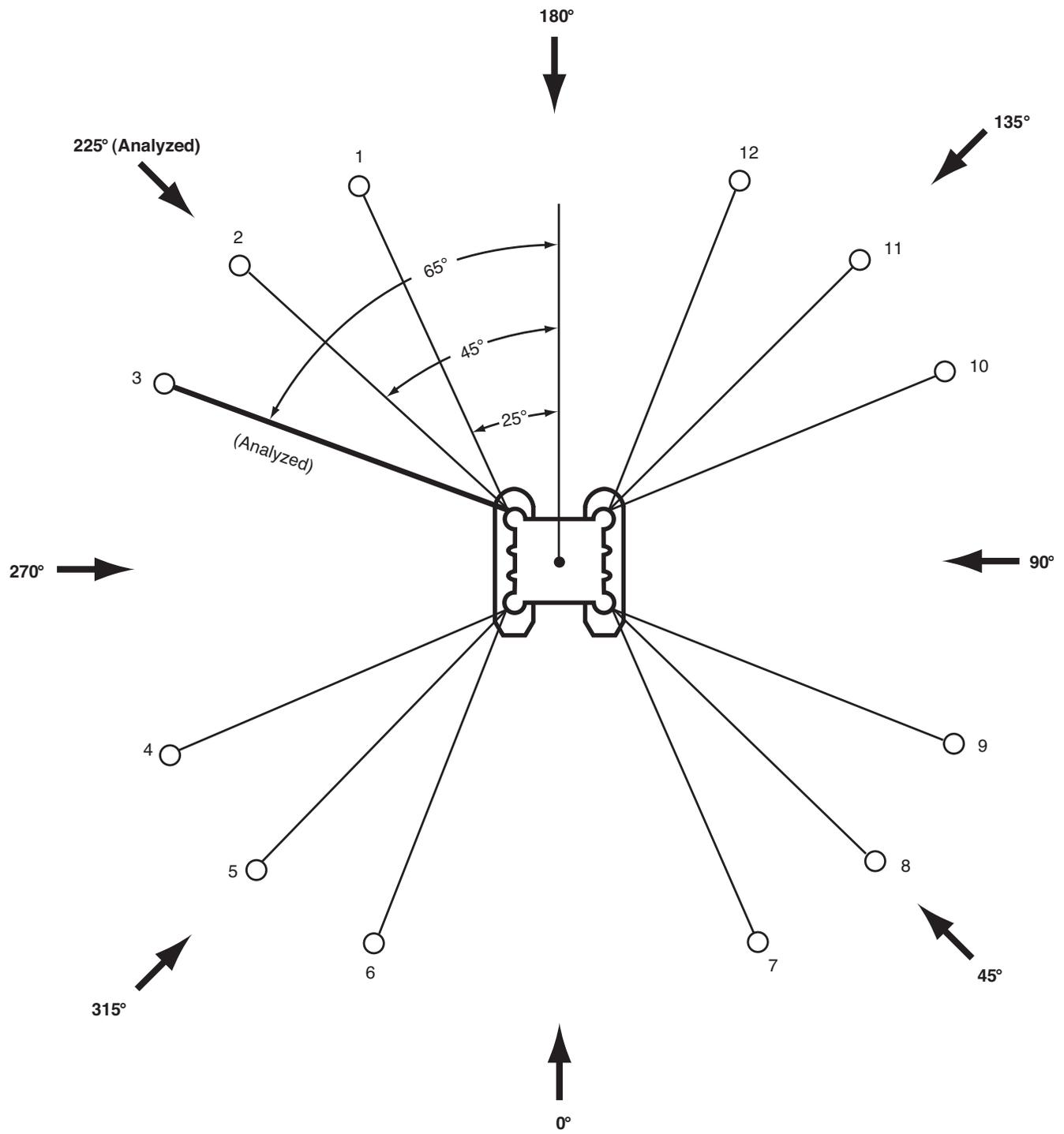
Figure J.4—Mooring System and Environmental Directions
