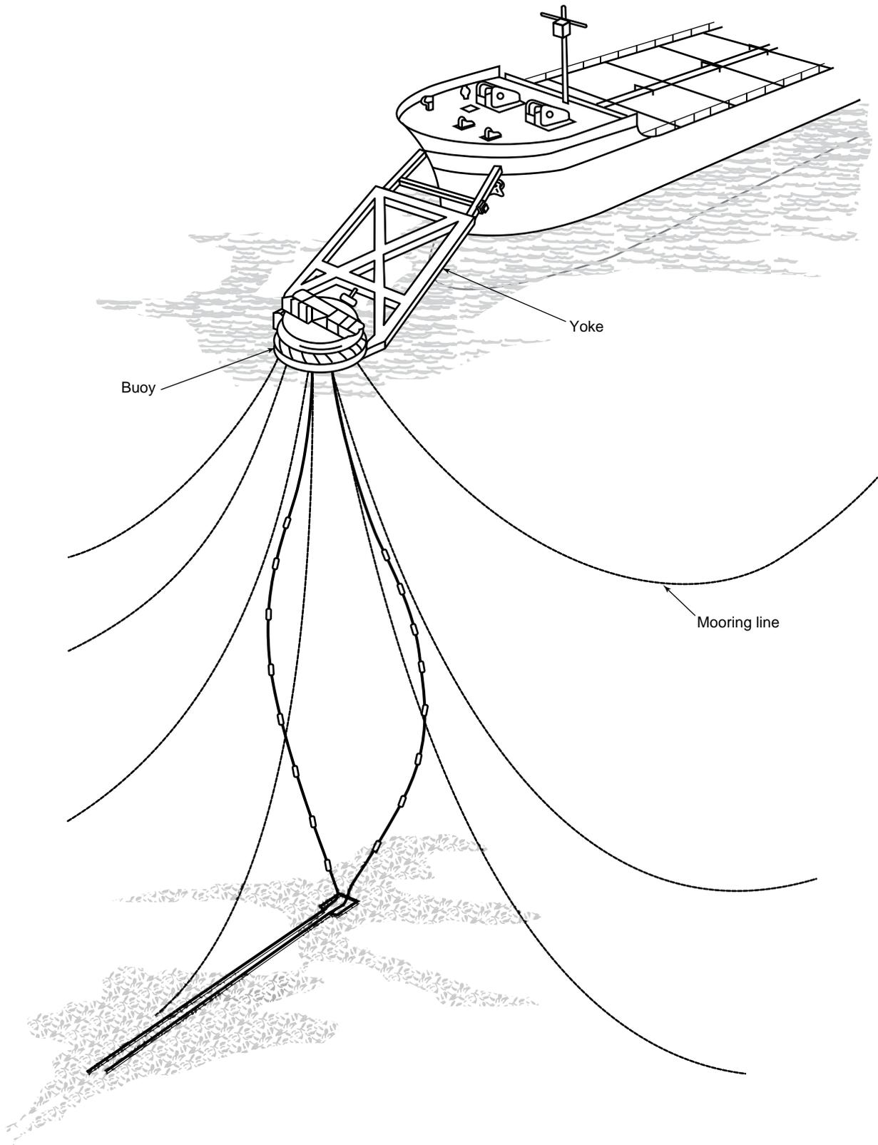
Figure 8—Catenary Anchor Leg Mooring (CALM) with Fixed Yoke
