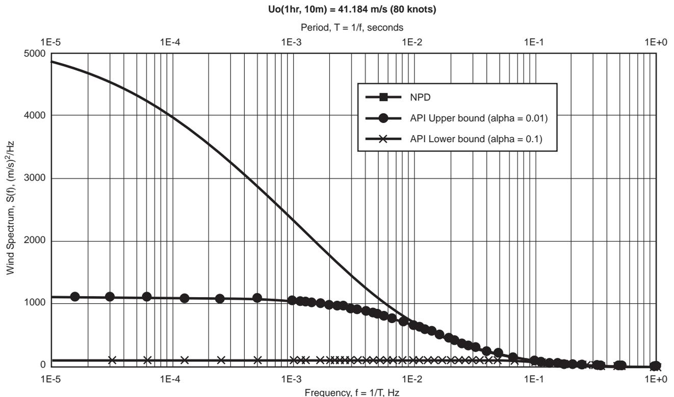
Figure I.18—Difference in Wind Spectra Increases with Increasing Natural Period
