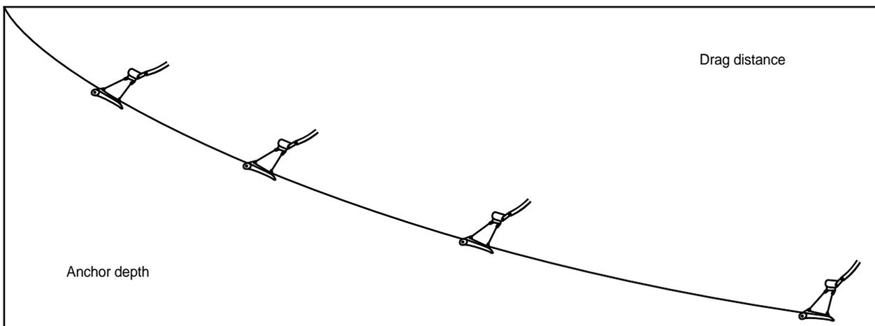
Figure E.6—Anchor Trajectory and Fluke Orientation During Installation
