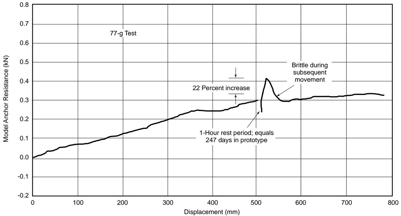
Figure D.5—Effect of Anchor Soaking
