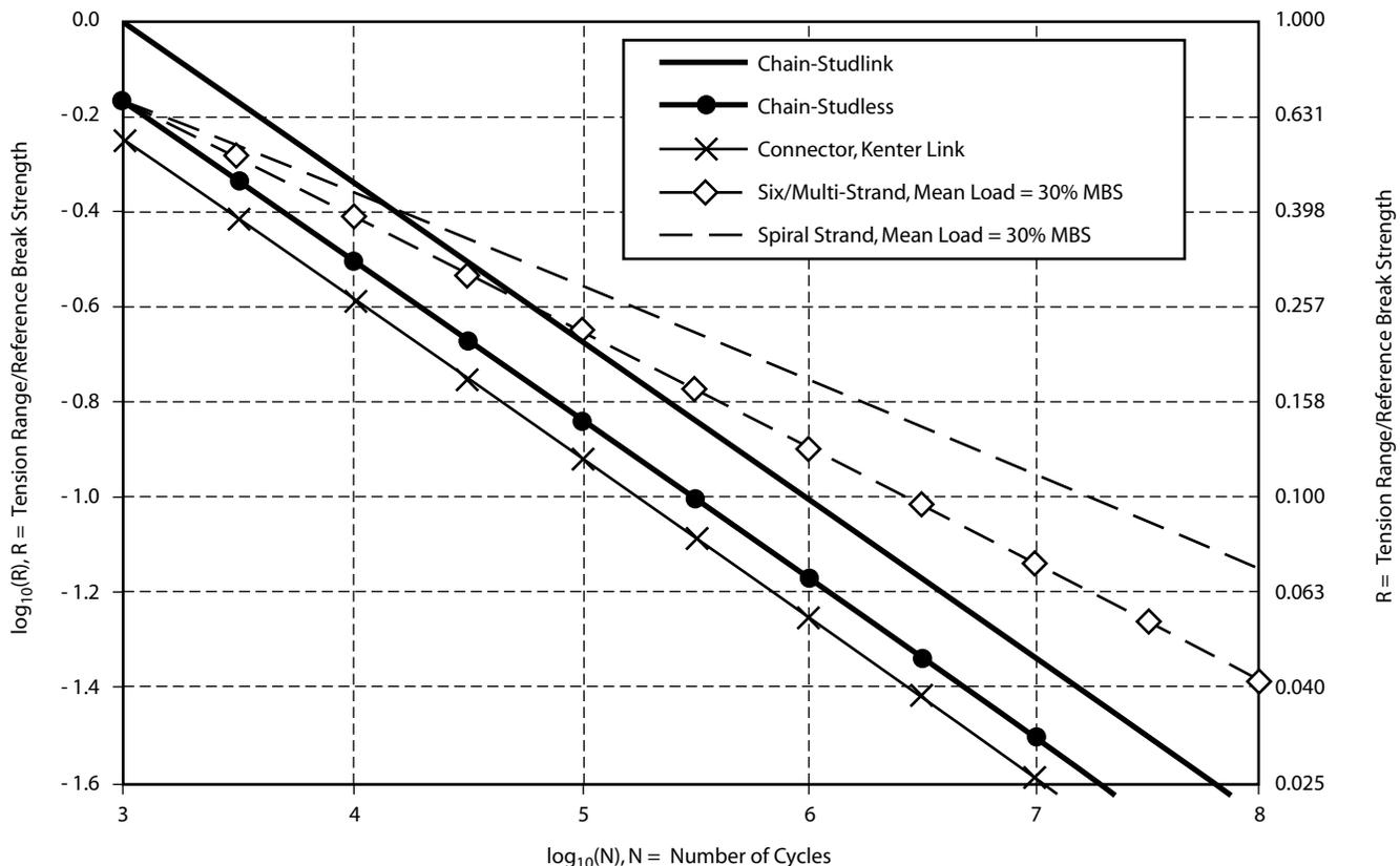
Figure 13—Mooring Fatigue Design Curves
