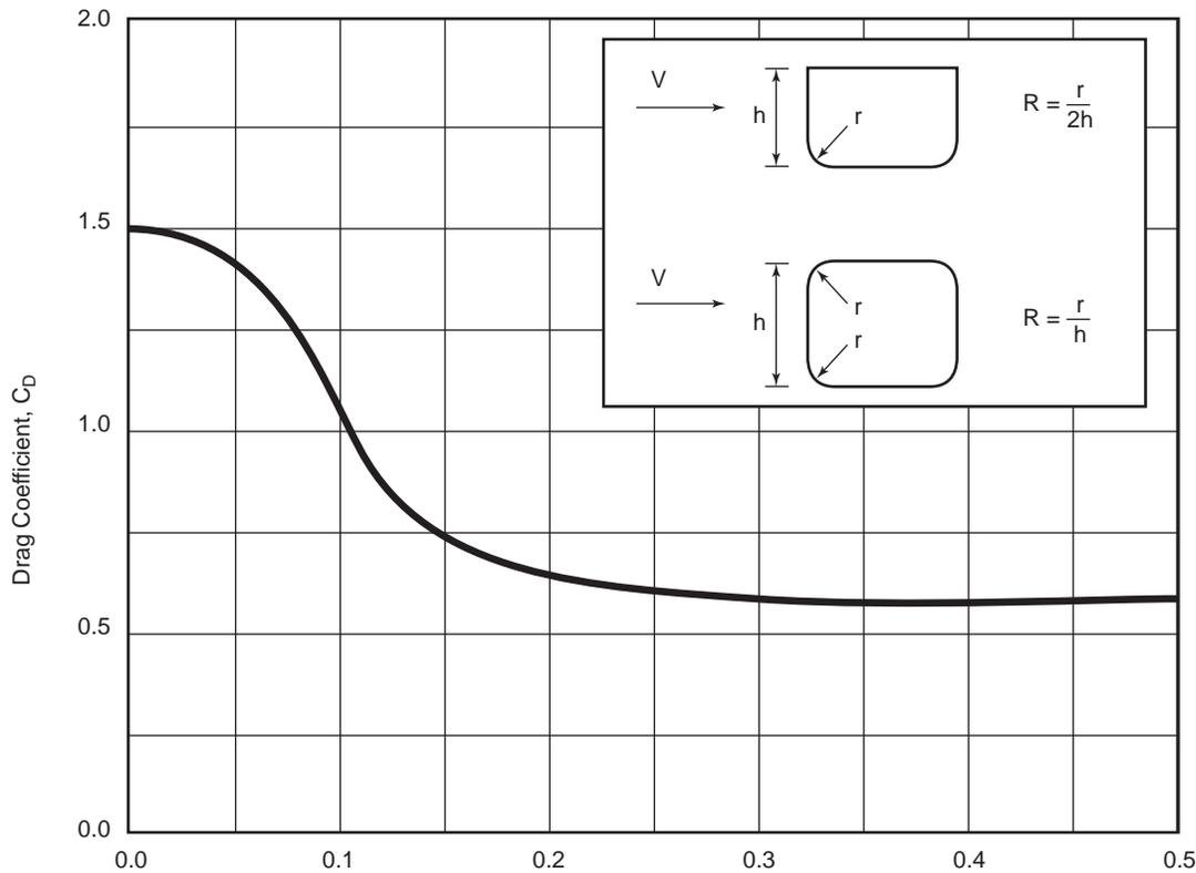
Figure C.1—Semi-submersible Current Drag Coefficient for Members Having Flat Surfaces
