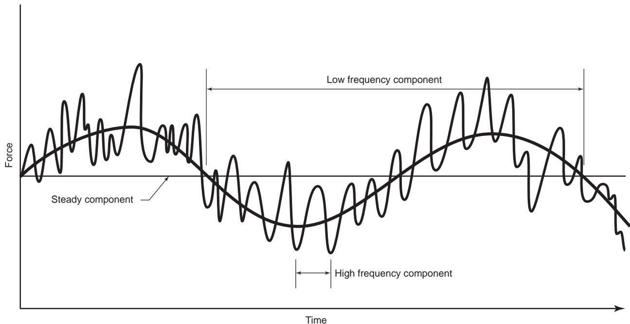
Figure C.2—Wave Force Components
