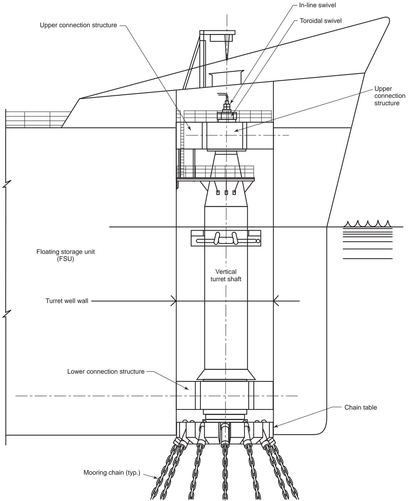
Figure 5—Typical Internal Turret Mooring Arrangement
