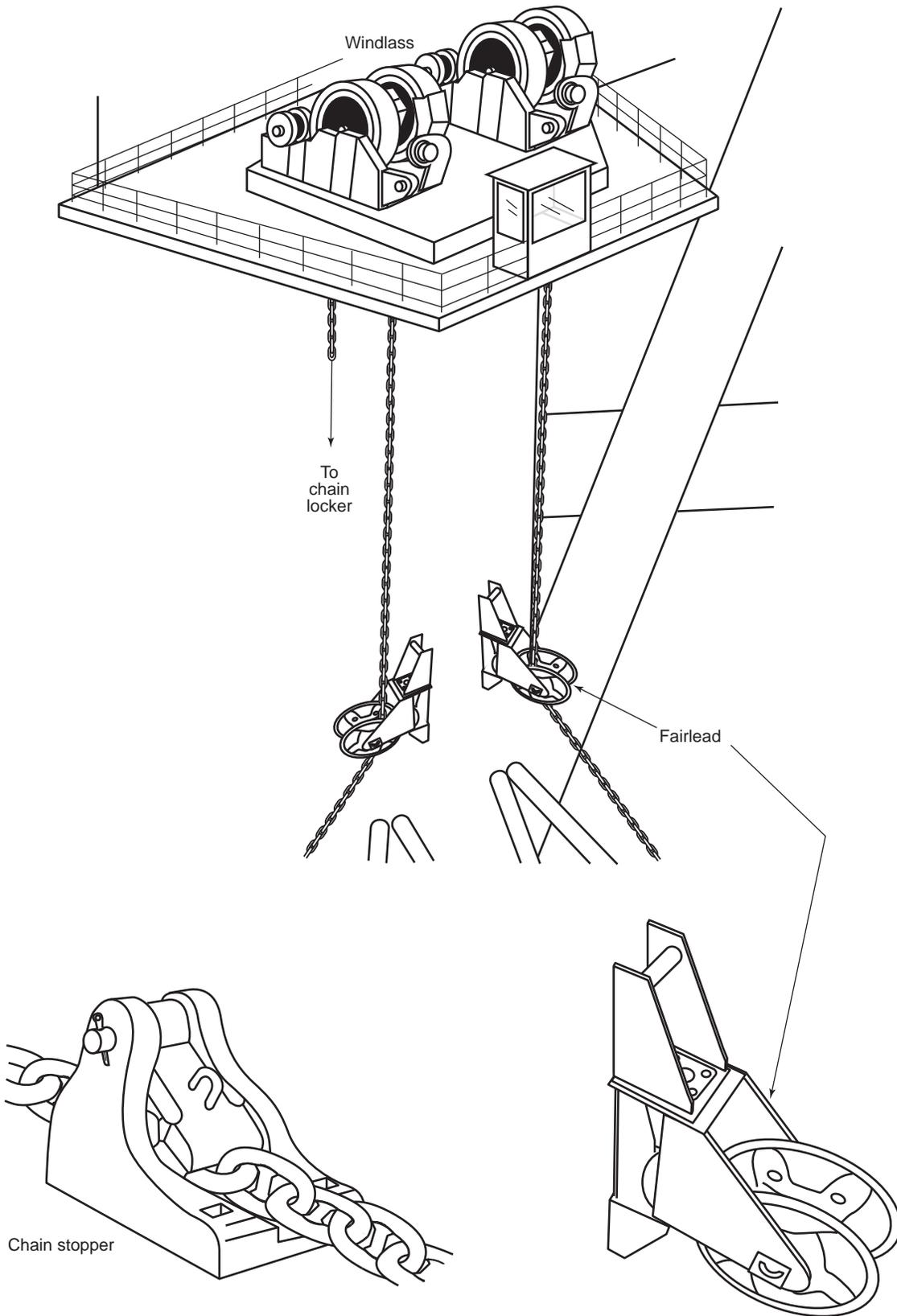
Figure A.8—Winching Equipment for Chain
