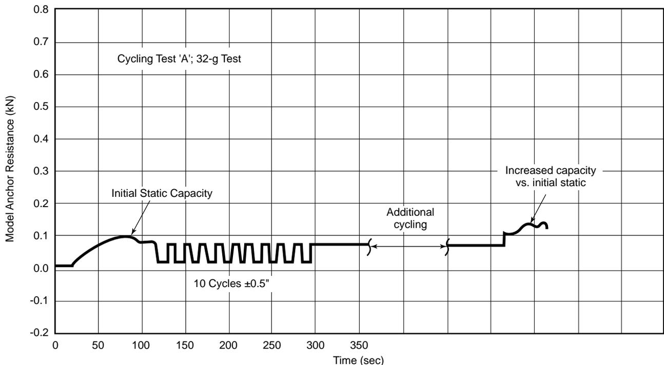
Figure D.4—Effect of Cyclic Loading
