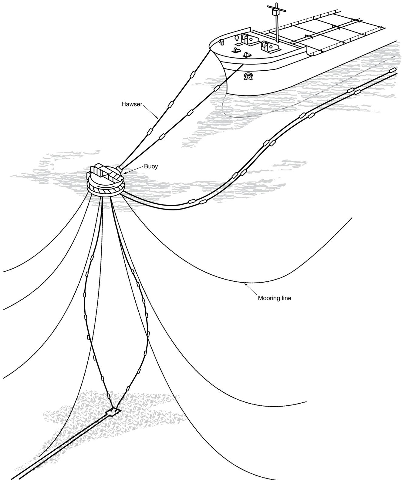
Figure 7—Catenary Anchor Leg Mooring (CALM) with Hawsers
