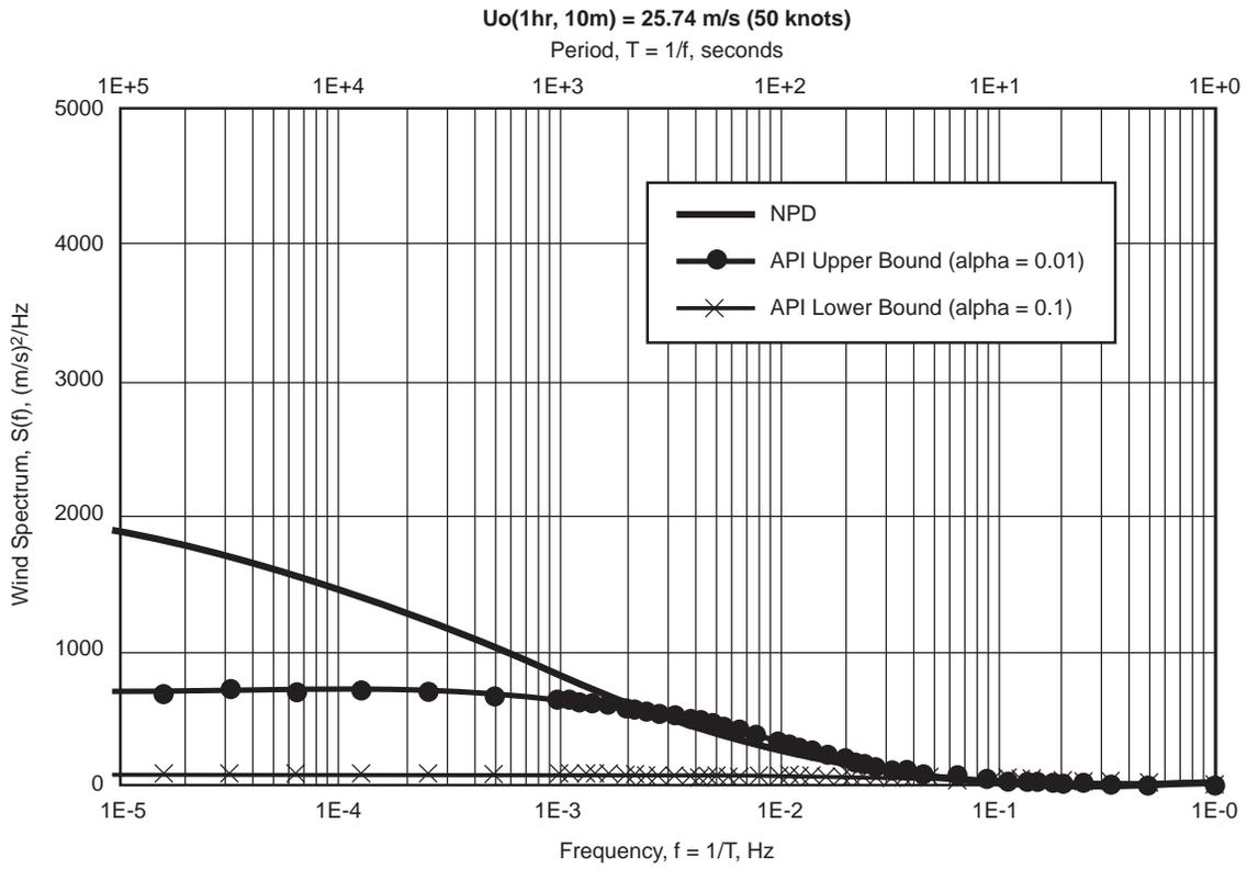
Figure B.2—Comparison of API and NPD Spectrum for 50-Knot Wind
