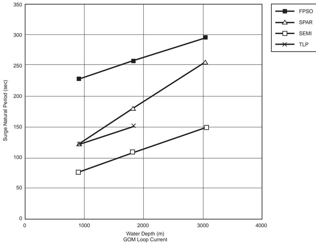
Figure I.4—Surge Natural Period Increases with Water Depth—Loop Current
