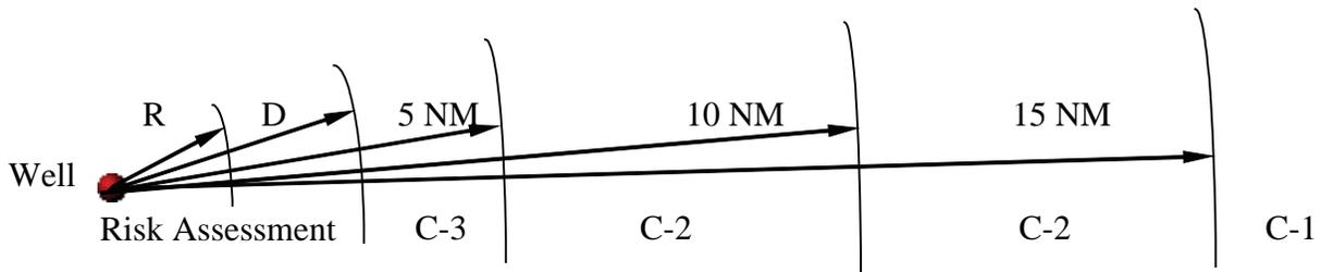
Note:  $d$  = distance to well center.  $R$  = mooring radius = distance between well and most distant anchor;  $D$  = mooring diameter =  $2R$
