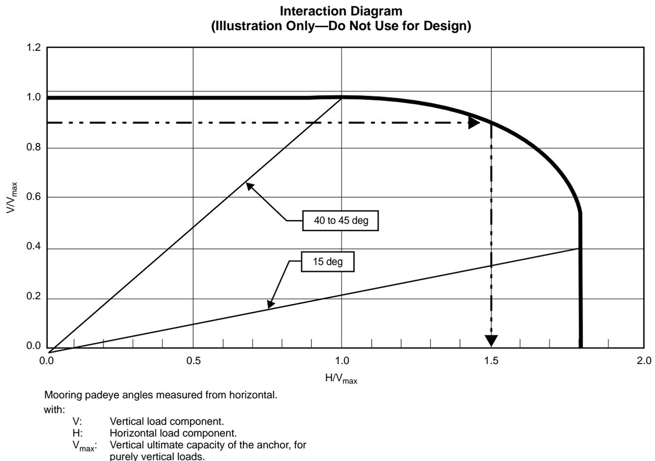
Figure E.3—Example of Failure Interaction Diagram
