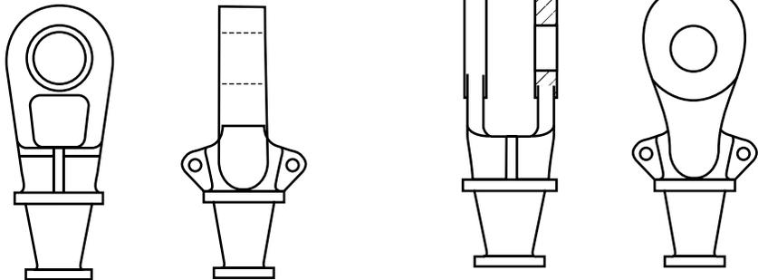
Figure A.3—Wire Rope Socket for Permanent Mooring
