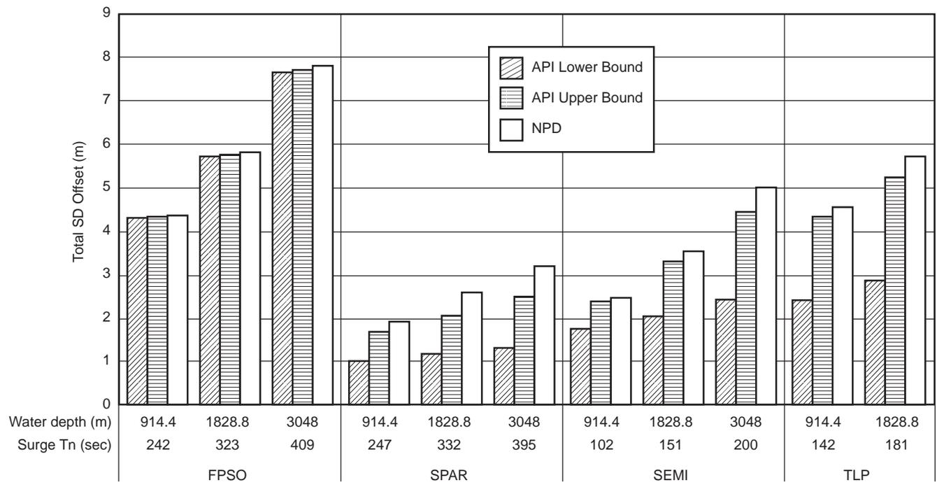
Figure I.20—Sensitivity of Wind Spectrum on Total SD Offset—Hurricane Condition
