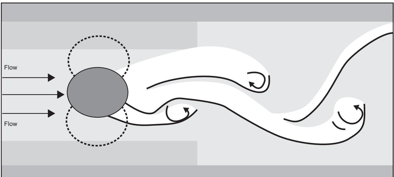
Figure H.1—Eddies in the Downstream Wake of a Cylinder
