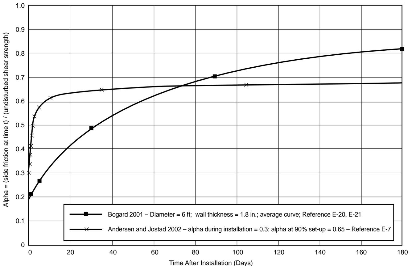
Figure E.2—Example of Increase in Adhesion Factor with Time
