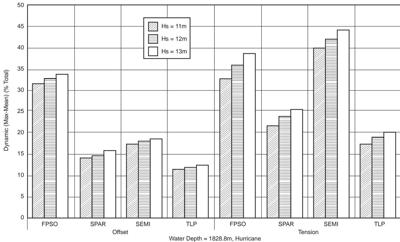
Figure I.21—Sensitivity of Wave Height for Hurricane Condition
