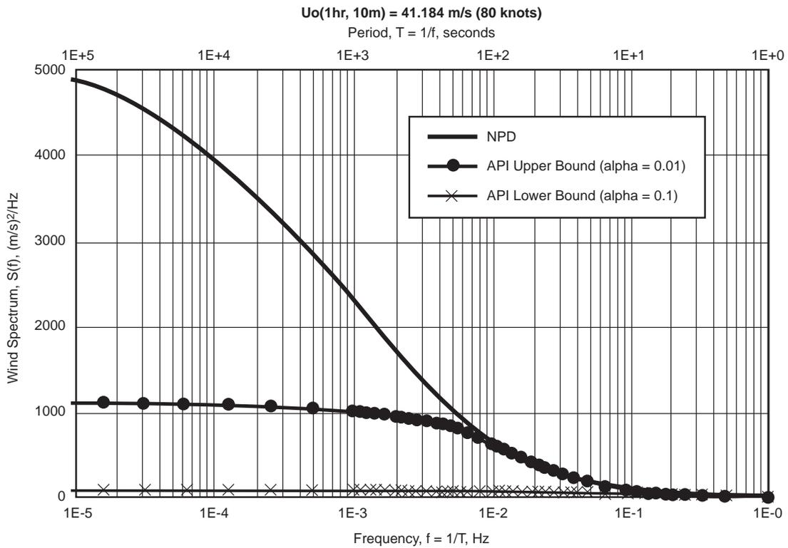
Figure B.3—Comparison of API and NPD Spectrum for 80-Knot Wind
