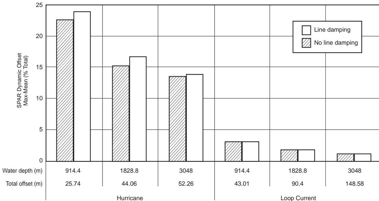
Figure I.9—Effect of Neglecting Line Damping for SPAR
