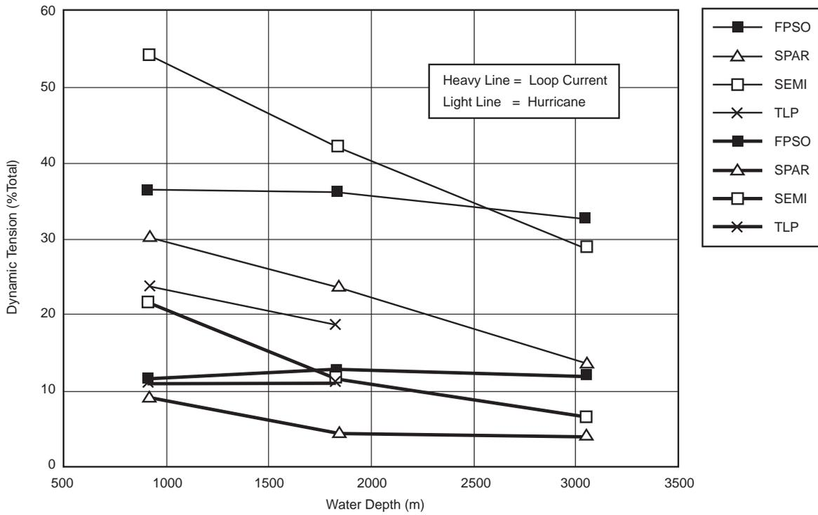
Figure I.2—Dynamic Tension for Most Loaded Mooring Line or Tendon
