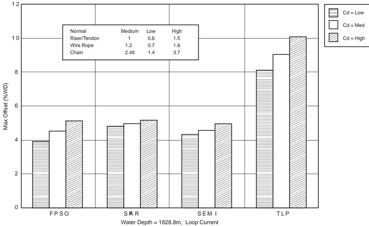
Figure I.11—Effect of Current Drag Coefficient on Vessel Offset—Loop Current
