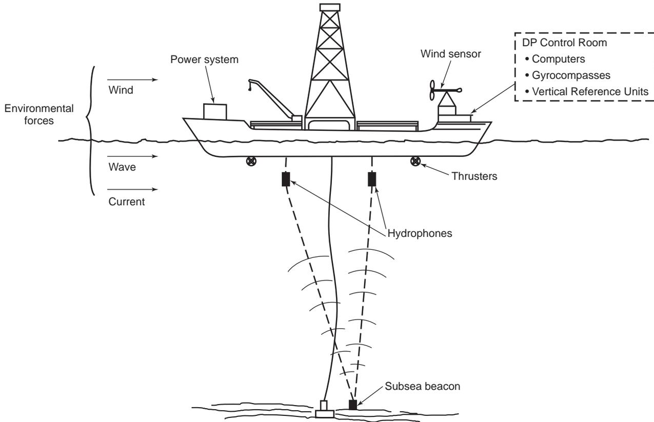
Figure 14—Major Elements of a Dynamic Positioning System
