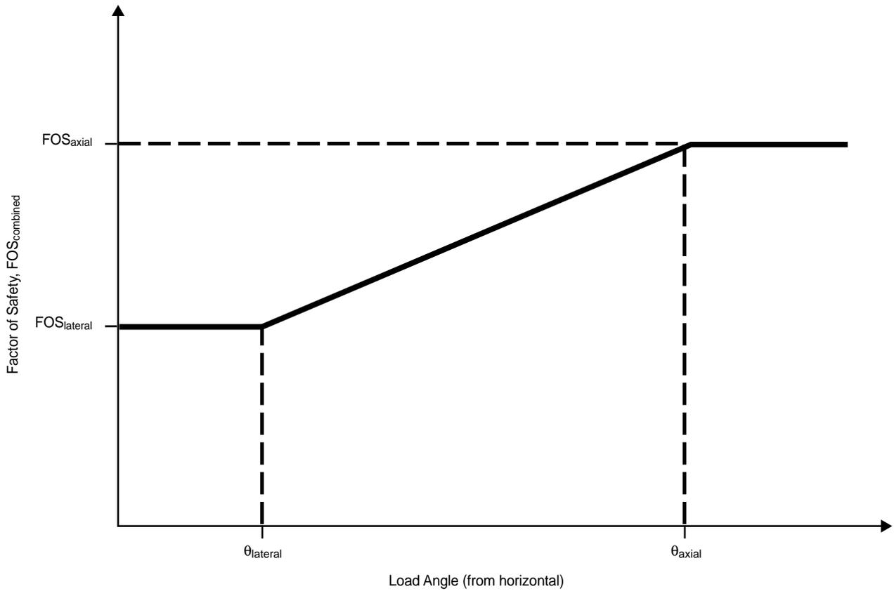
Figure E.4—Calculation of Required Safety Factor as a Function of Failure Mode
