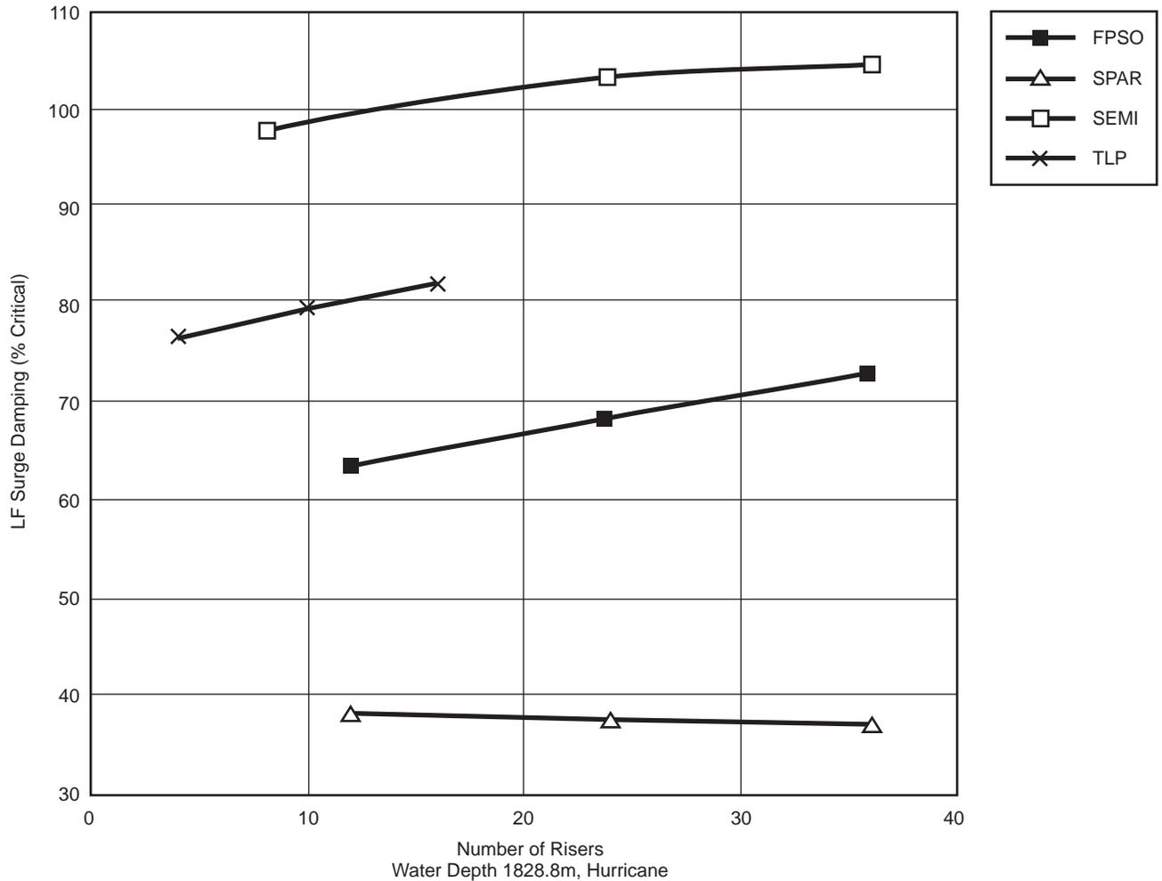
Figure I.8—Effect of Risers on Low Frequency Surge Damping
