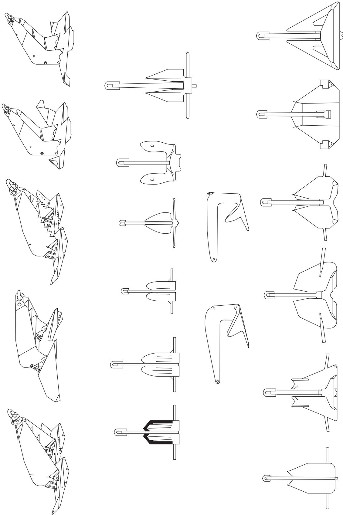
Figure D.1—Typical Drag Embedment Anchors
