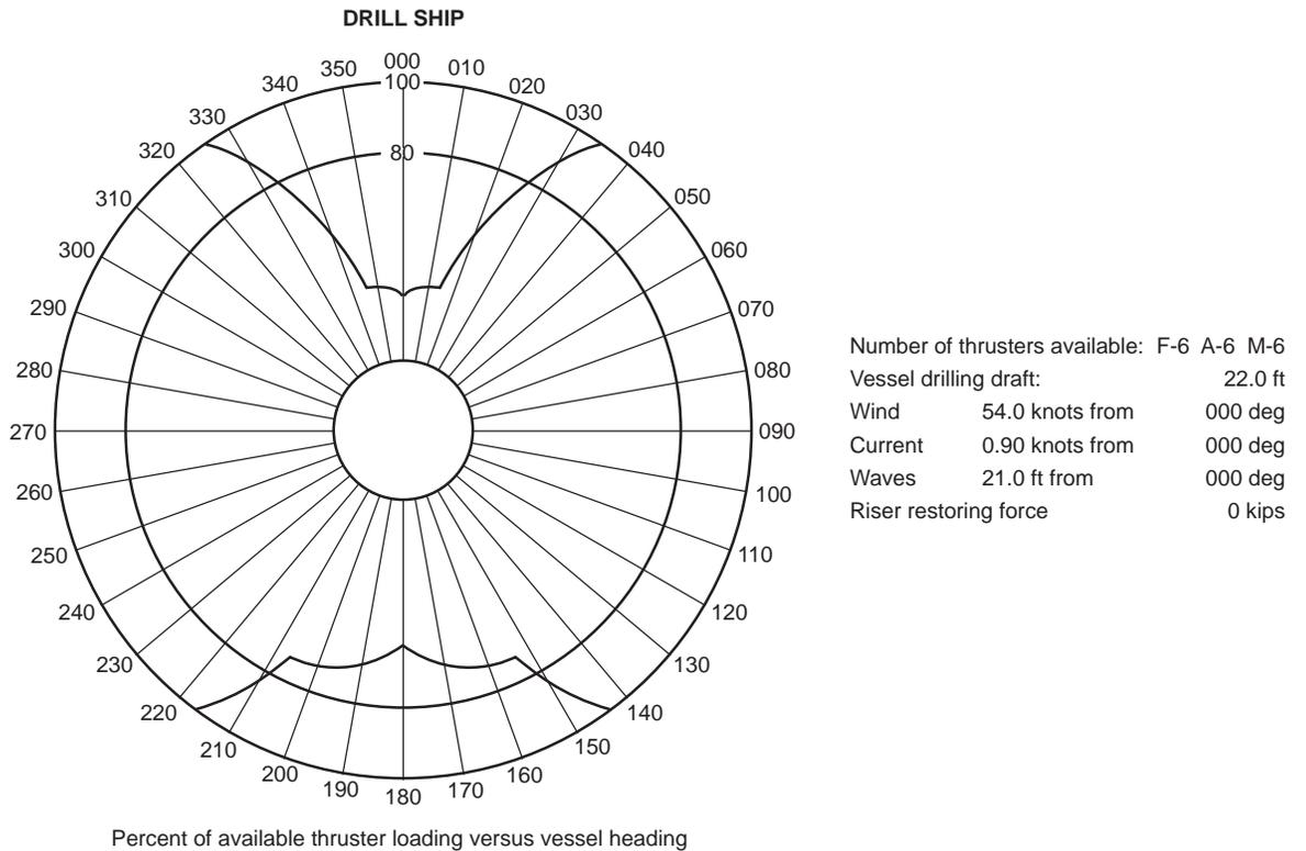
Figure 15—Dynamic Positioning Capacity Rosettes
