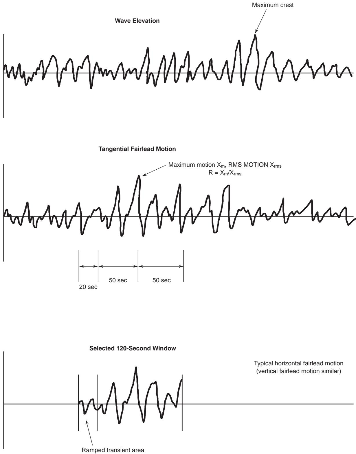
Figure J.3—Selection of Input Motion
