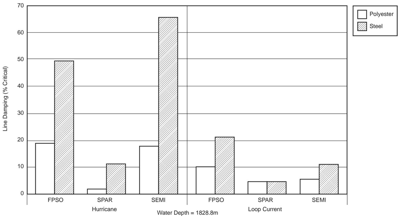
Figure I.24—Comparison of Line Damping for Steel and Polyester Mooring
