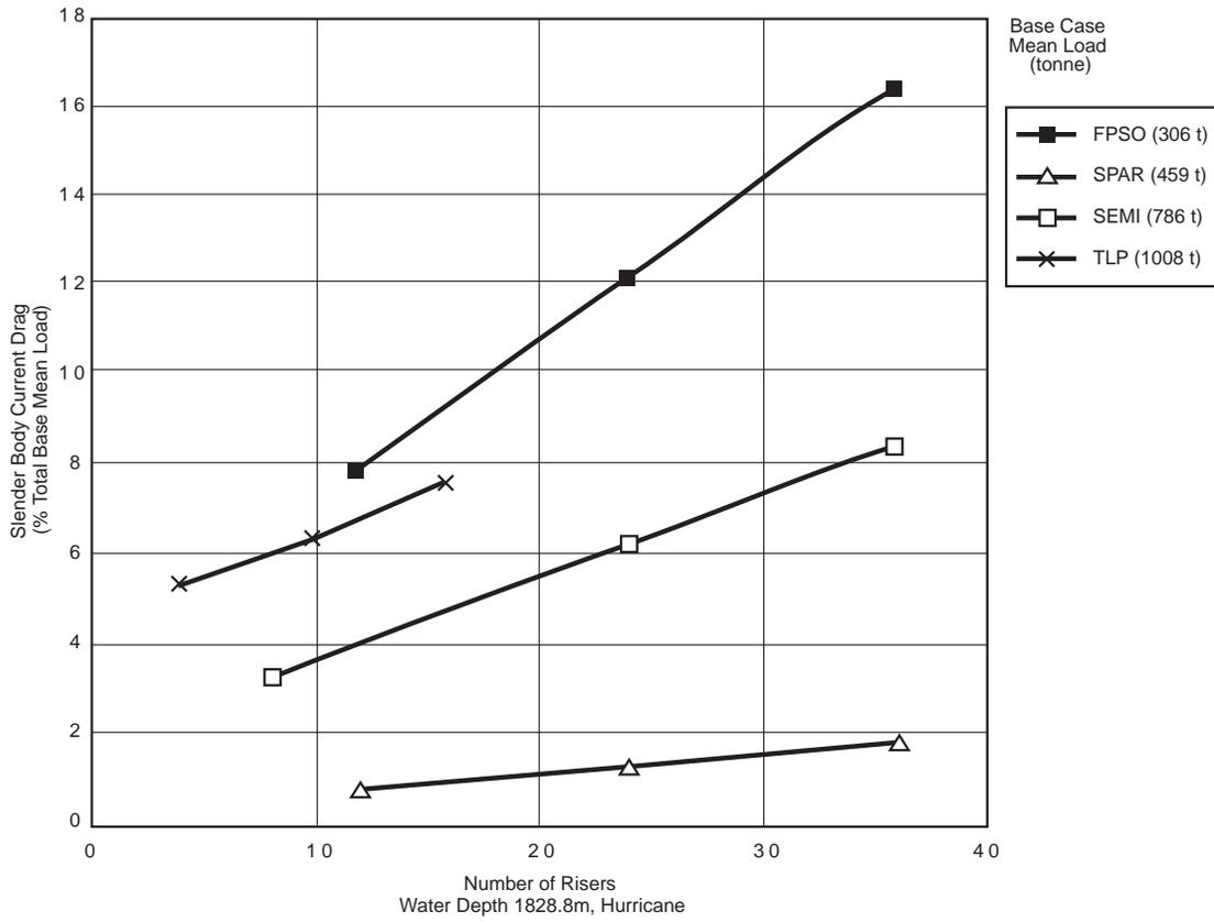
Figure I.10—Effect of Risers on Current Load from Slender Bodies
