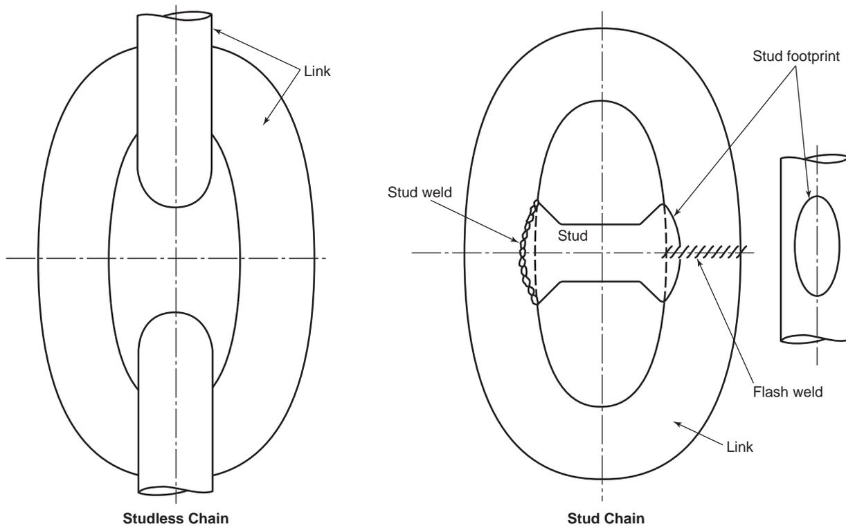
Figure A.1—Stud and Studless Chain
