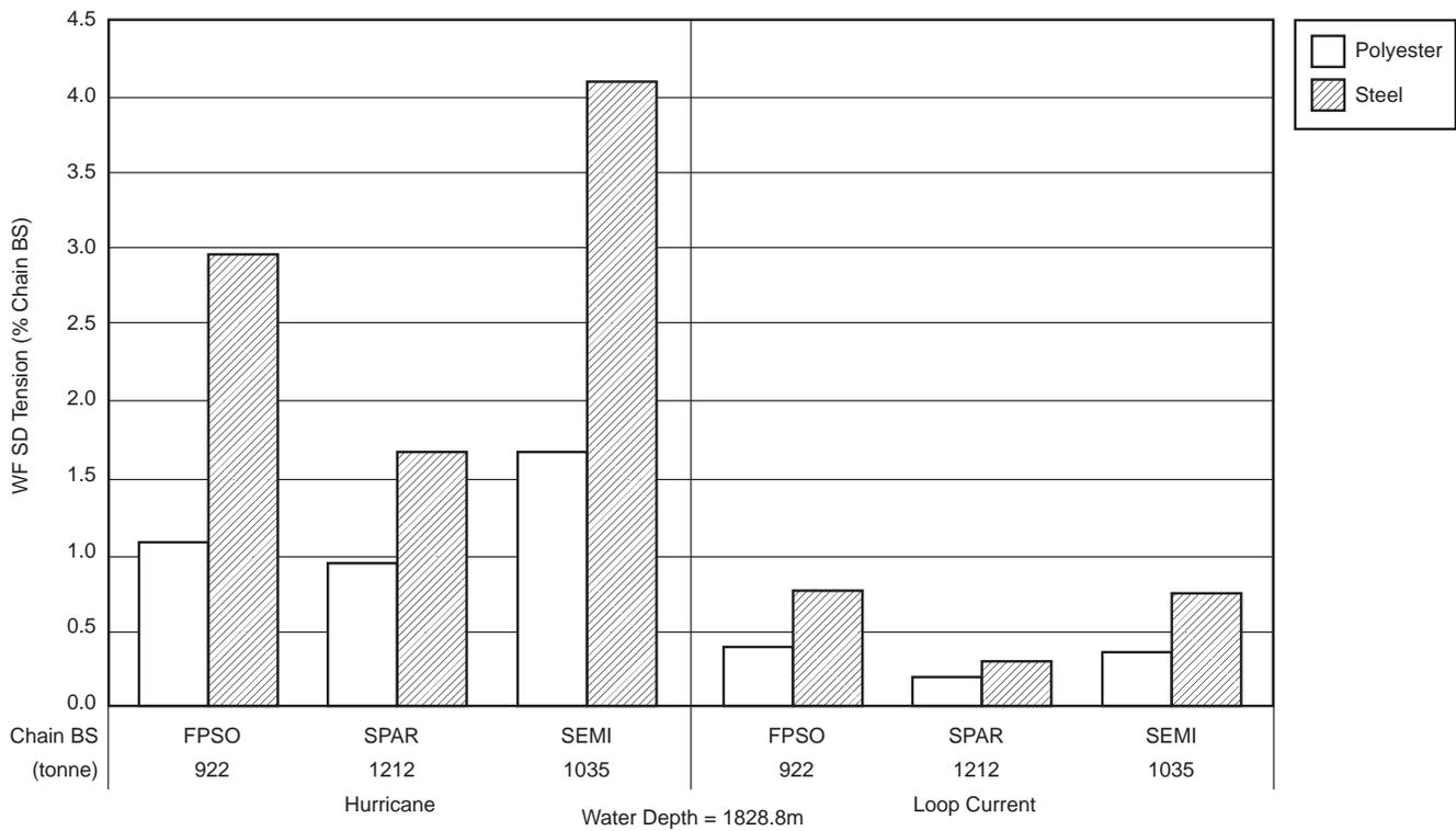
Figure I.23—Comparison of Wave Frequency Tensions for Steel and Polyester Mooring
