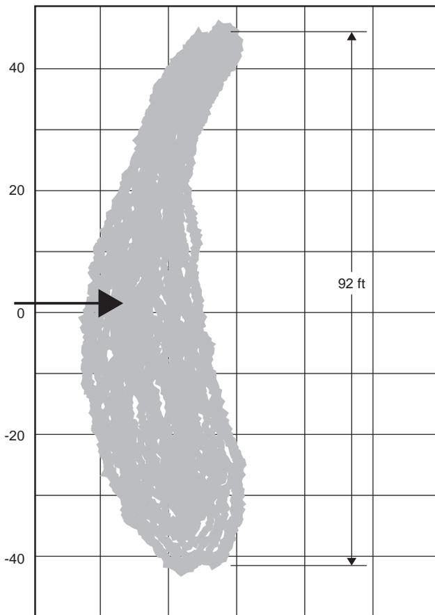
Figure H.2—Motion Trajectory of a Spar Experiencing VIM
