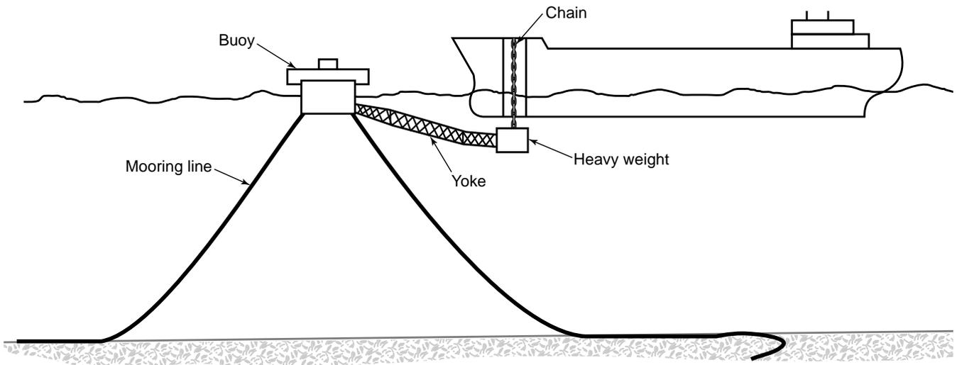
Figure 9—Catenary Anchor Leg Mooring (CALM) with Soft Yoke
