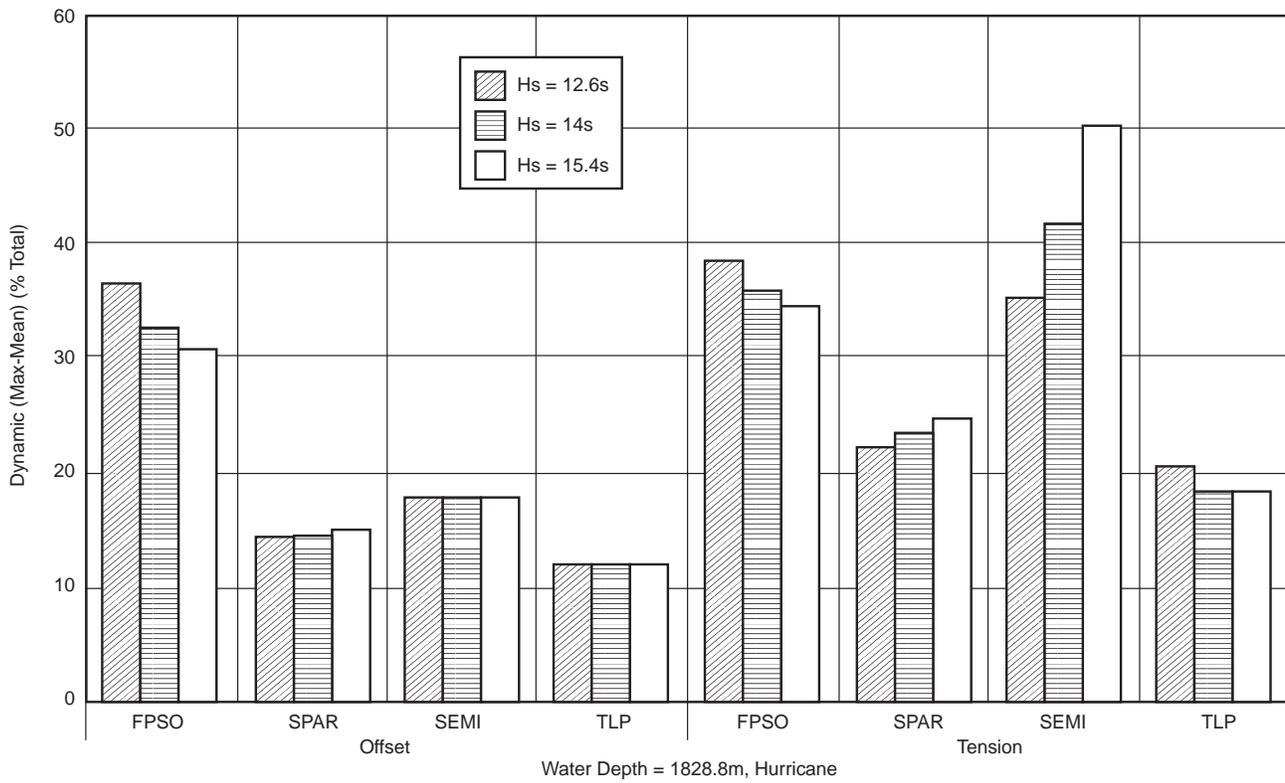
Figure I.22—Sensitivity of Wave Peak Period for Hurricane Condition
