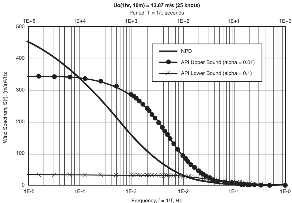
Figure B.1—Comparison of API and NPD Spectrum for 25-Knot Wind
