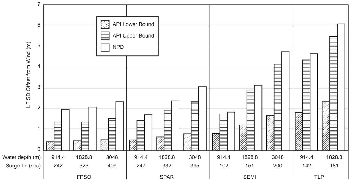
Figure I.19—Sensitivity of Wind Spectrum on SD Offset from Wind—Hurricane Condition
