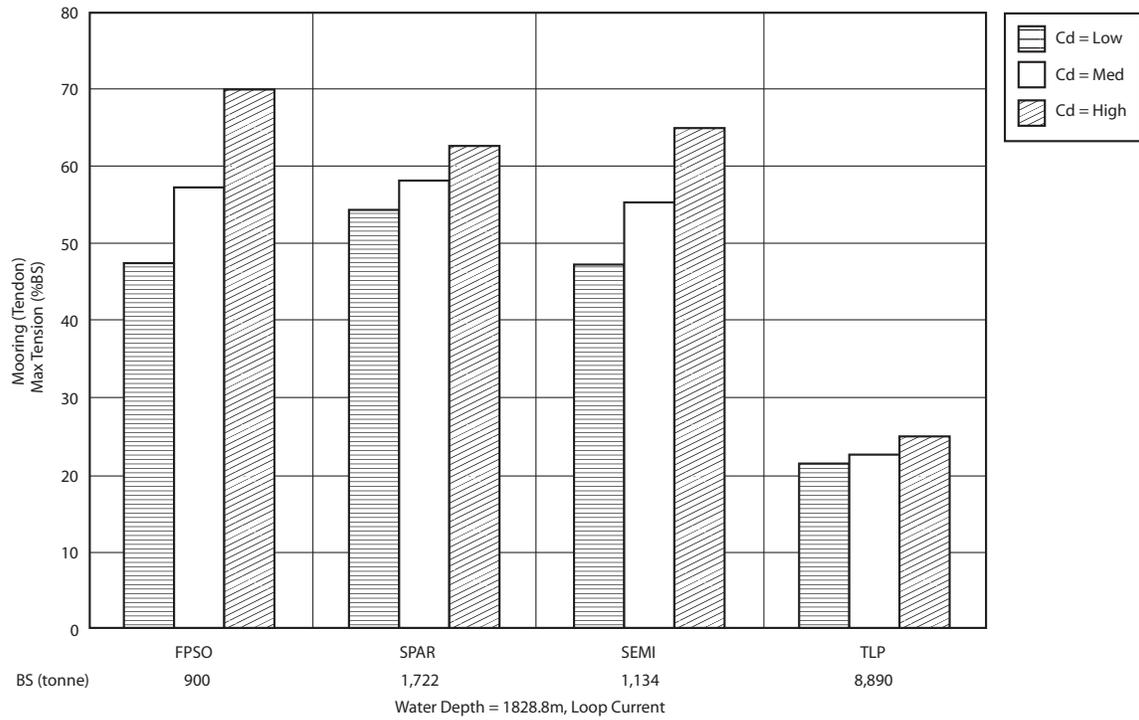
Figure I.12—Effect of Current Drag Coefficient on Line Tension—Loop Current
