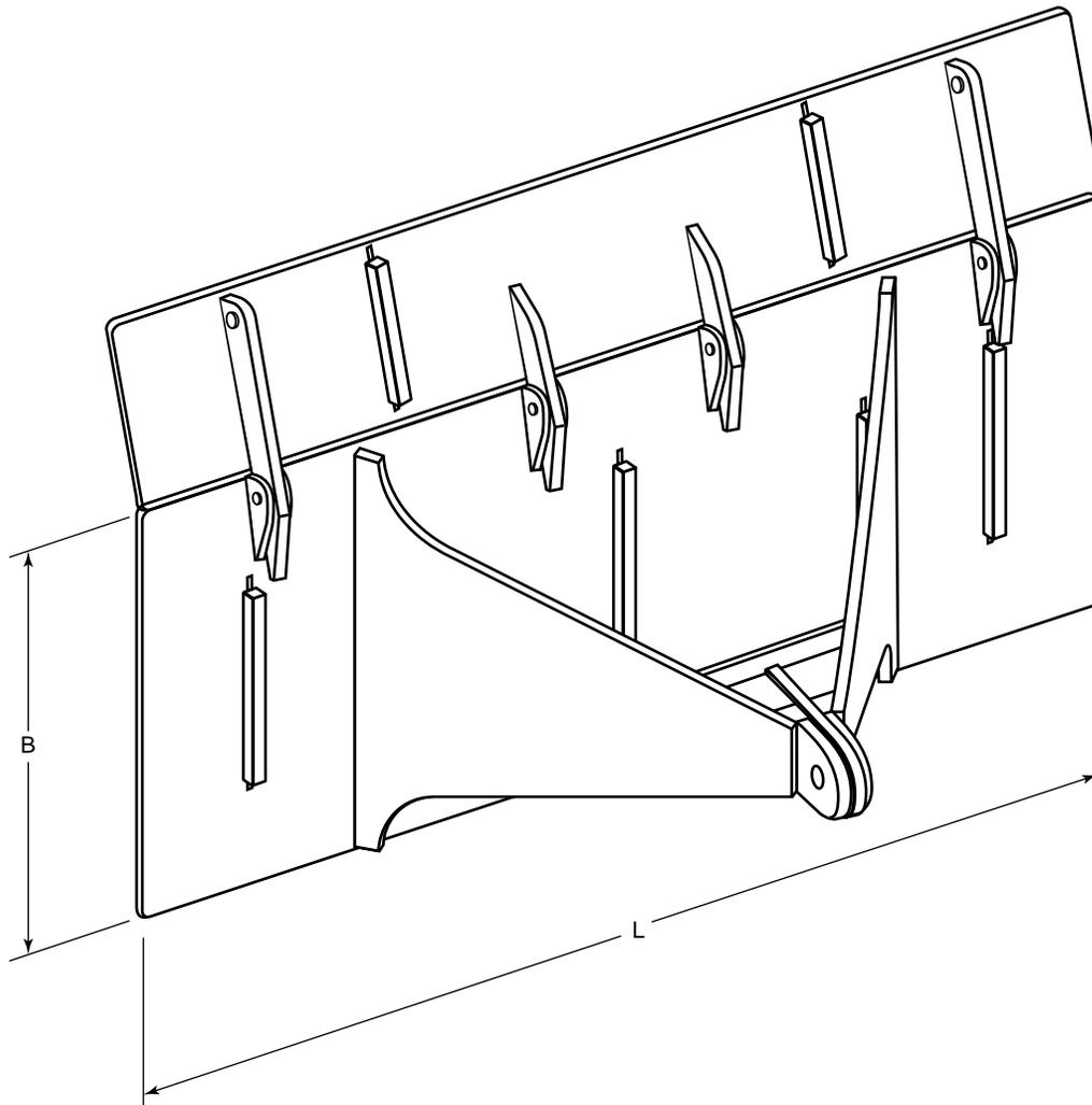
Figure E.7—Definition of Anchor Fluke Width,  $B$ , and Length,  $L$
