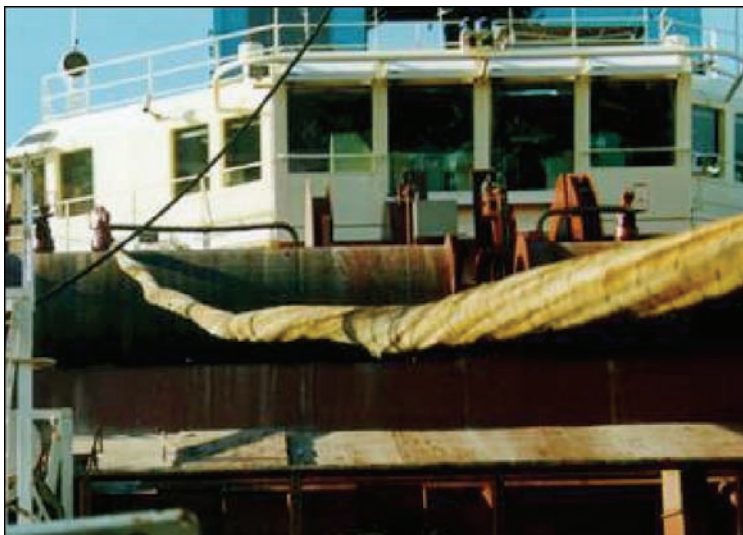
Figure 45—Rope Twisting During Installation
