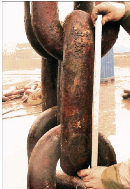
Figure 32—Example of Chain Link Subjected to Out-of-Plane Bending
