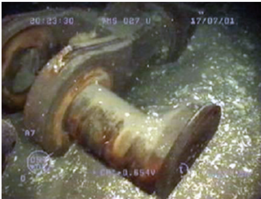
Figure 35—Wire Rope Socket Disconnected Due to Detachment of Retaining Pin
