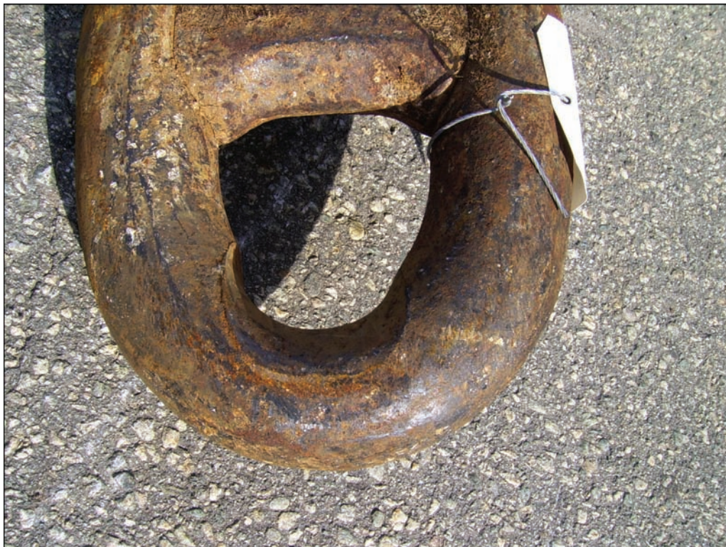
Figure 31—Chain Diameter Reduction Due to Excessive Interlink Wear
