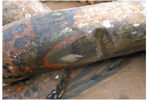
b) Wear notch from contact with hawse
