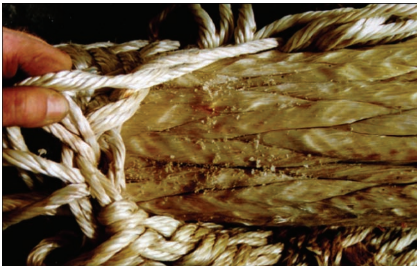
Figure 42—Marine Growth Detected Between the Jacket and Load Carrying Fiber
