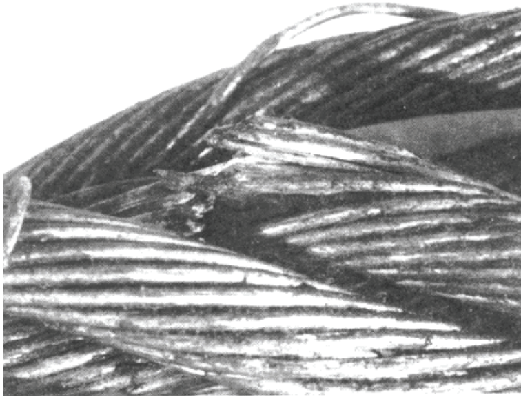
Figure 11—Locally Grouped Broken Wires
