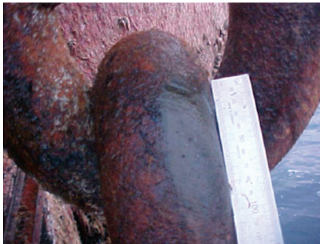
Figure 27—Example of Chain Wear from Sitting in a Fairlead Pocket
