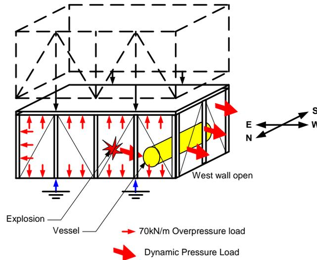
Figure C.6.7-1—Blast in a Compartment
