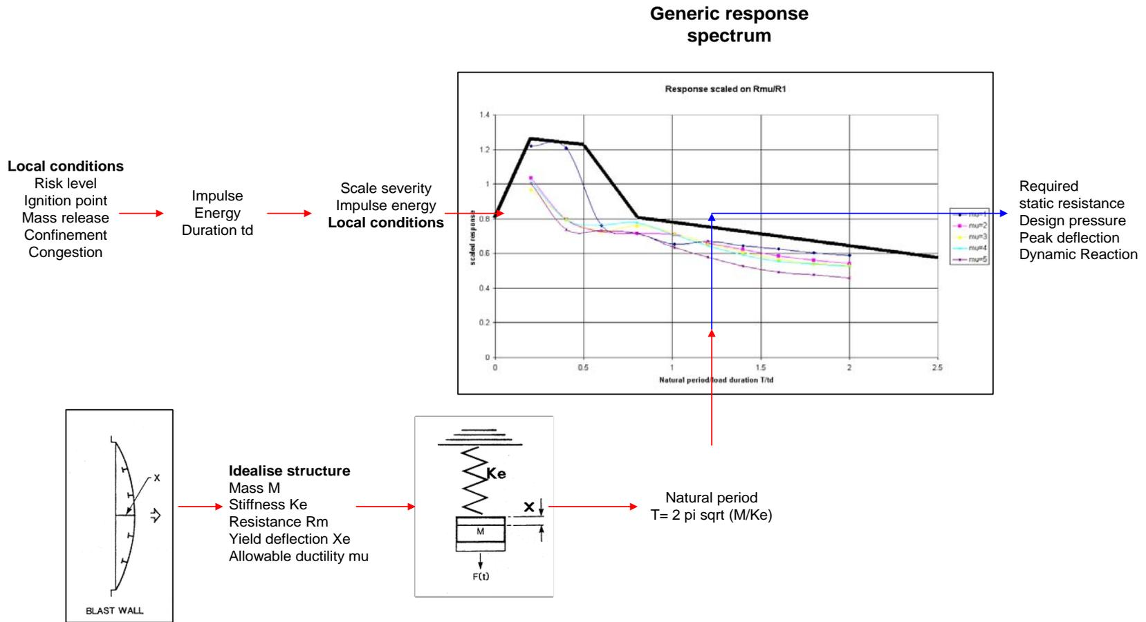
Figure C.6.6-1—Generic Response Spectra for a Hydrocarbon Blast
