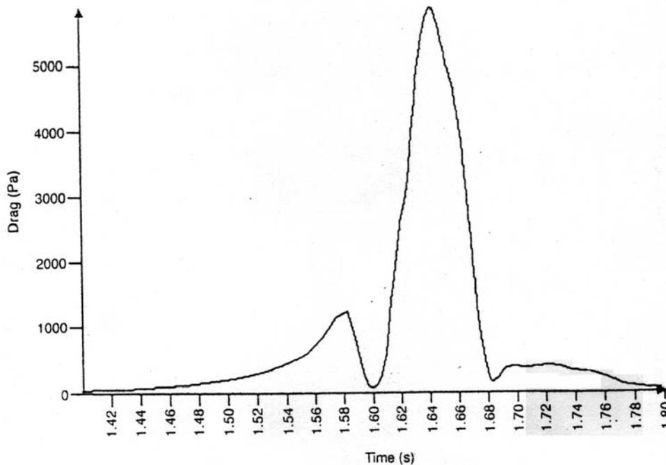
Figure C.6.7-2—Drag Loading on Piping – Typical Time-History
