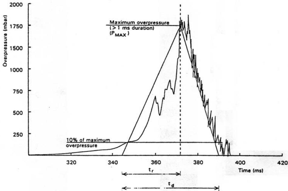
Figure C.6.5-1—Idealized Pressure Trace for a Hydrocarbon Blast
