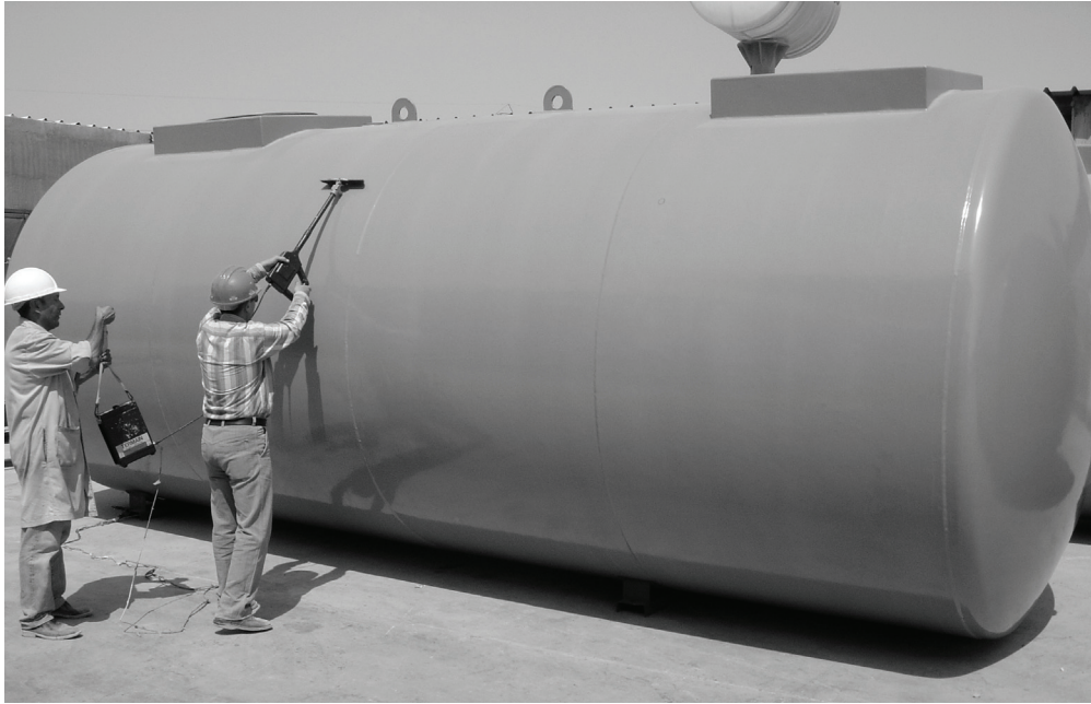
Figure 6—Typical “Holiday” Test for Steel USTs
