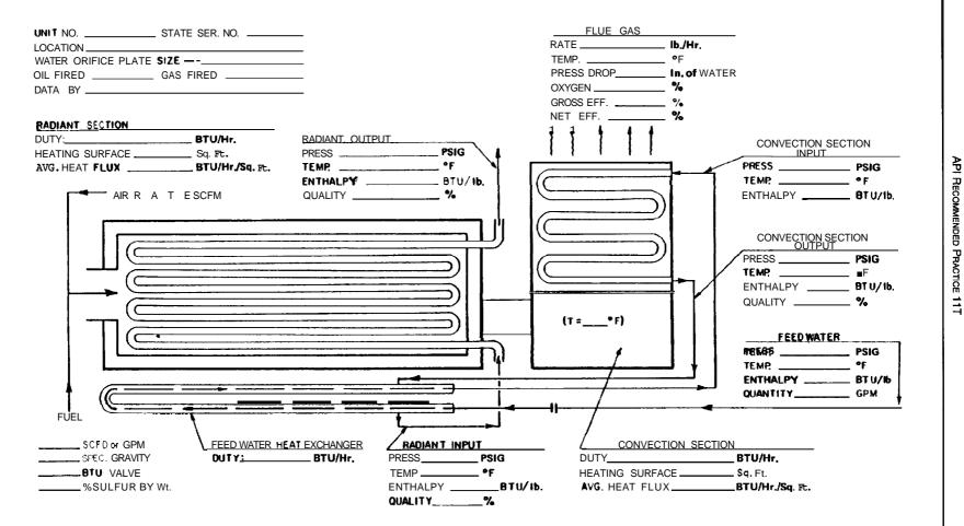
Figure 1 — Example Heat Balance Performance Data Sheet
