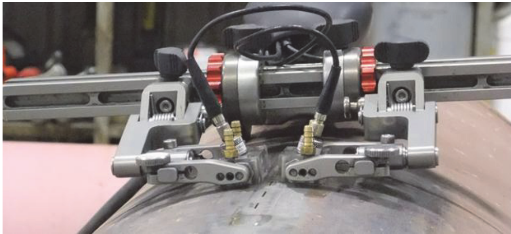
Figure K.2—Time-of-Flight Diffraction Head for Seam Weld Inspection
