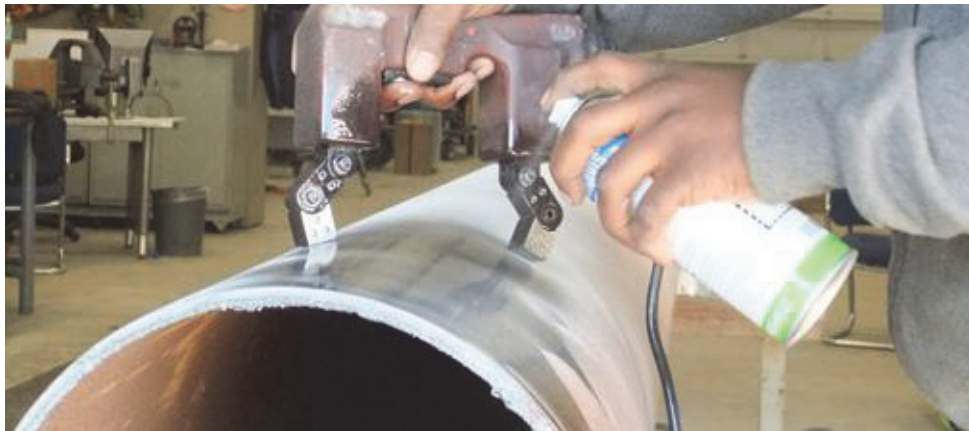
Figure K.1—Example of a Magnetic Particle Inspection
