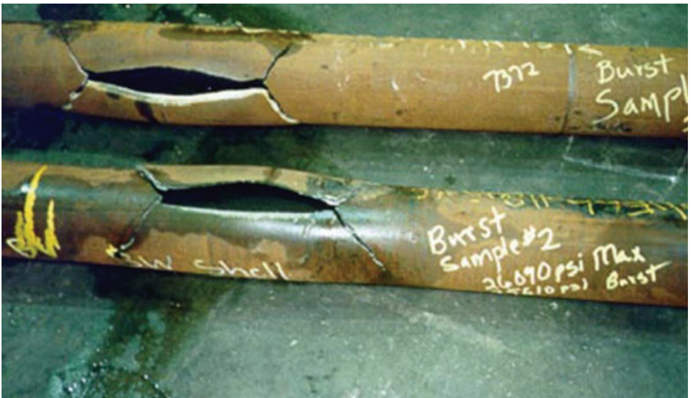
Figure A.2—Brittle Burst Sample
