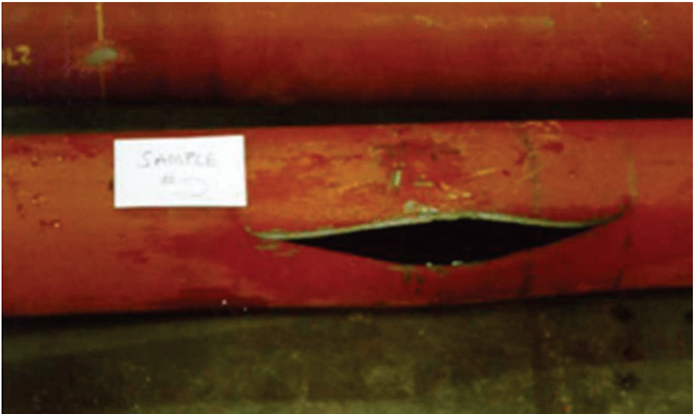
Figure A.1—Ductile Burst Sample
